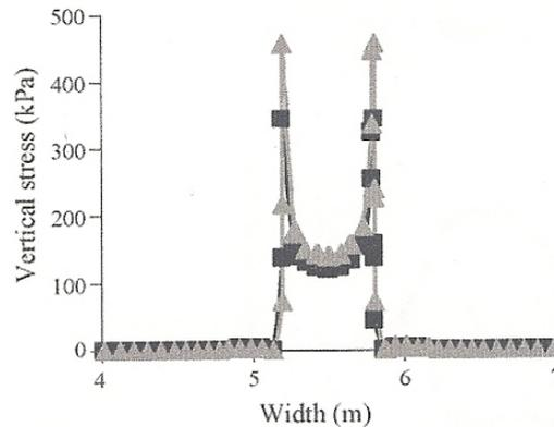
**Figure 2.8 Calculated vertical stress distributions on a clay surface with a very rigid plate using a uniform applied stress  $q = 150$  kPa (black squares) and a higher value 180 kPa (grey triangles) (Cui et. al., 2006)**
