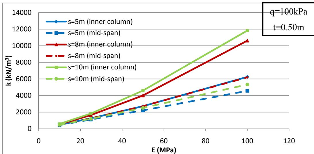
Figure 4.3 k vs E for various spacings under the columns and mid-spans
