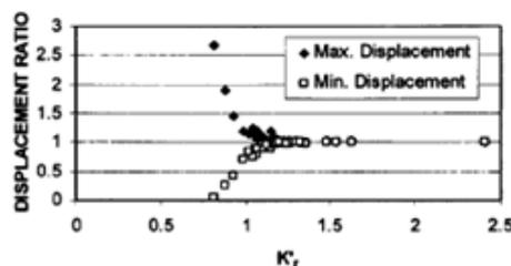
**Figure 2.9 Results for concentratedly loaded square footings vertical displacement (Tabsh and Al-Shawa, 2005)**
