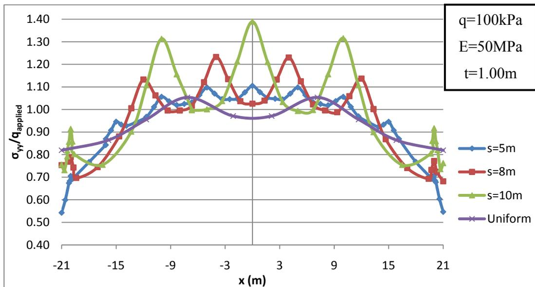
**Figure 4.25 Normalized contact stress distribution for various column spacings for  $t = 1.00$  m**
