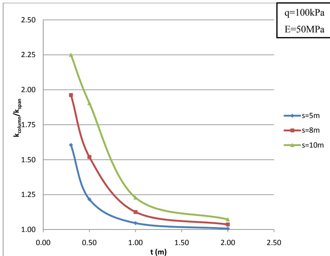
**Figure 4.22  $k_{\text{column}}/k_{\text{span}}$  vs  $t$  for various column spacings**
