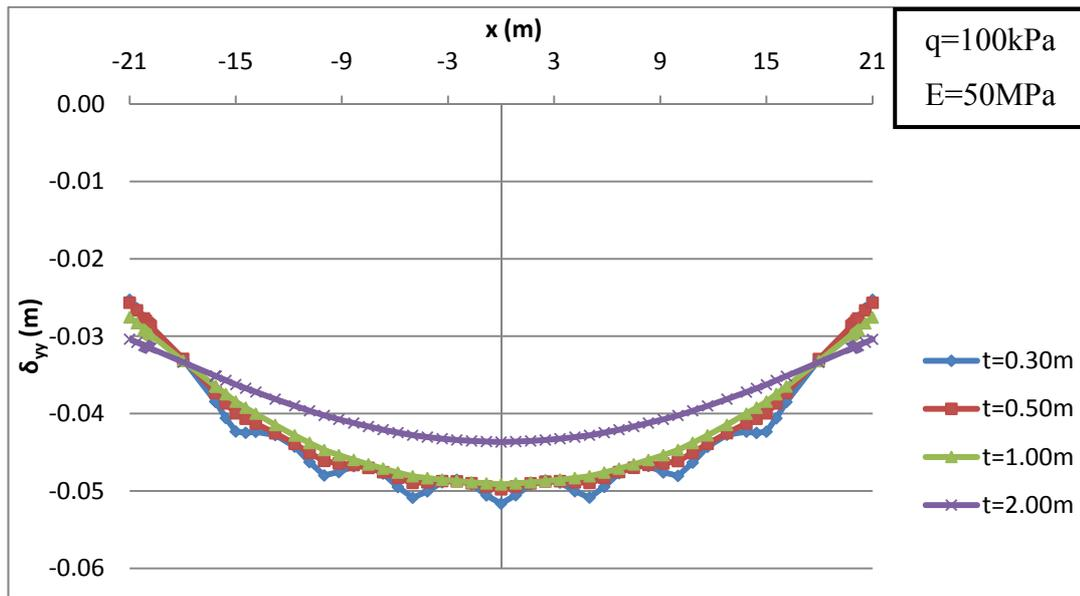
**Figure 3.21 Comparison of settlement distribution of Pattern B -  $s = 5$  m for Cases 2-1, 2-2, 2-3 and 2-4**
