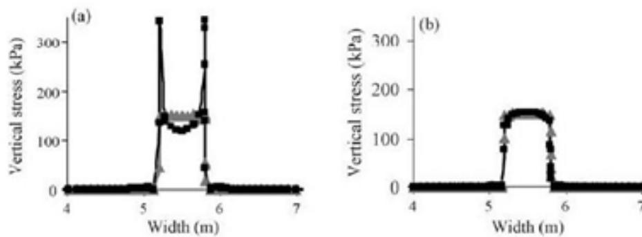
**Figure 2.6 Calculated vertical stress distributions on the soil surface with a very soft plate (grey triangles) or a very rigid plate (black squares) on (a) a clay, (b) a sand (Cui et. al., 2006)**
