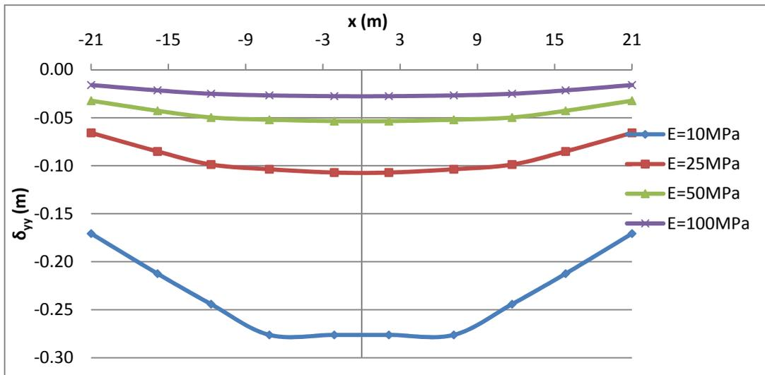
**Figure 3.6 Comparison of settlement distribution of Pattern A for Cases 1-1, 1-2, 1-3 and 1-4**
