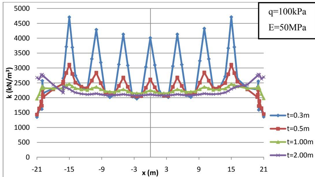
**Figure 3.22 Comparison of modulus of subgrade reaction distribution of Pattern B -  $s = 5$  m for Cases 2-1, 2-2, 2-3 and 2-4**
