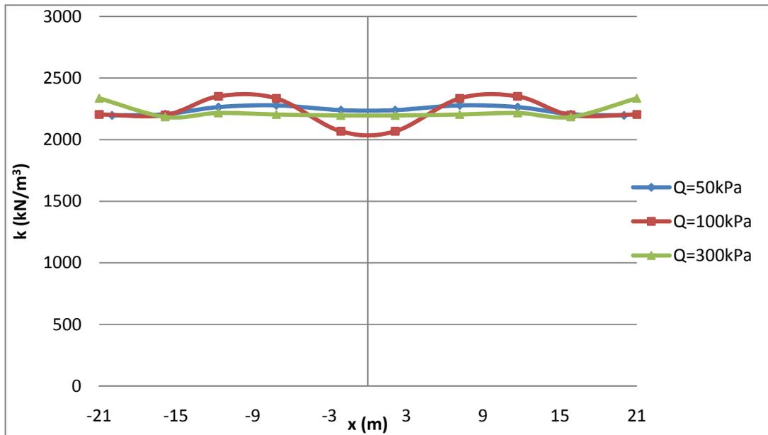
**Figure 3.14 Comparison of modulus of subgrade reaction of Pattern A for Cases 3-1, 3-2 and 3-3**
