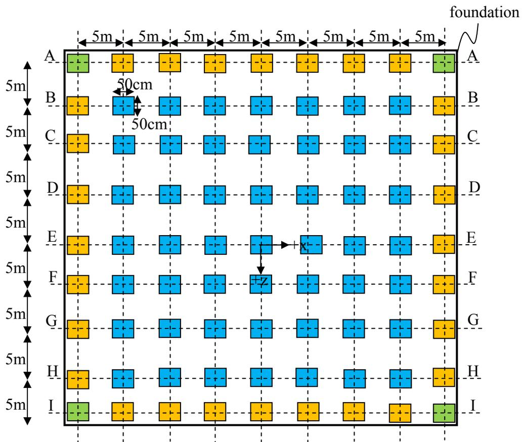
Figure 3.15 Plan view of the foundation model of Pattern B -  $s = 5 \text{ m}$
