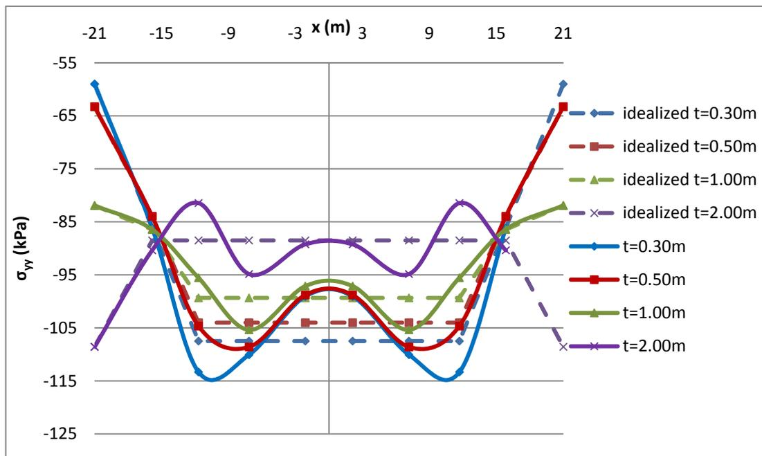
**Figure 3.9 Comparison of contact stress distribution of Pattern A for Cases 2-1, 2-2, 2-3 and 2-4**
