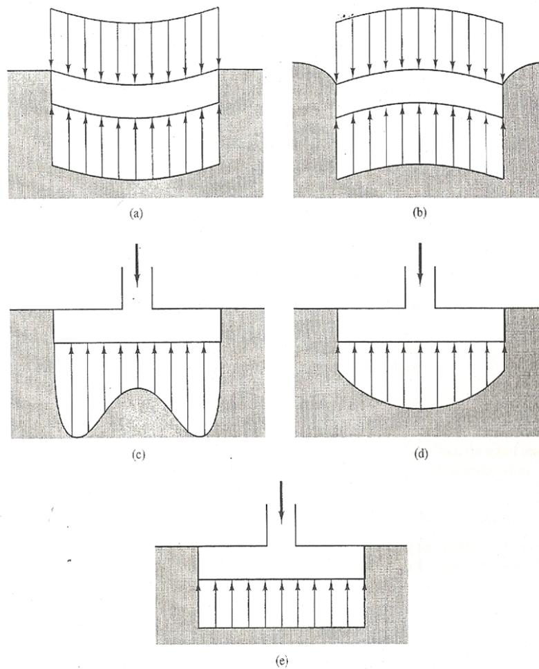
**Figure 2.4 Distribution of bearing pressure along the base of shallow foundations subjected to concentric vertical loads: (a) flexible foundation on clay, (b) flexible foundation on sand, (c) rigid foundation on clay, (d) rigid foundation on sand and (e) simplified distribution (Taylor, 1948 by Coduto, 2001)**
