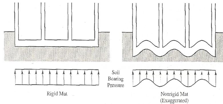
**Figure 2.1 The rigid method assumes there are no flexural deflections in the mat, so the distribution of soil bearing pressure is simple to define. However, these deflections are important because they influence the bearing pressure distribution (Coduto, 2001)**
