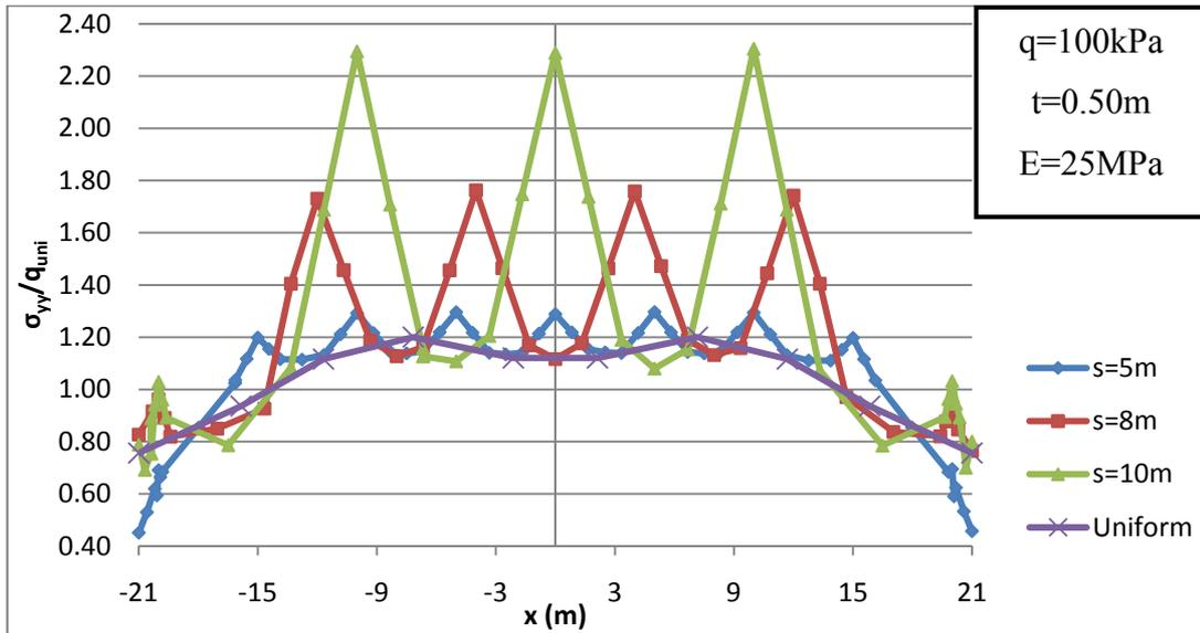
**Figure 4.12 Normalized contact stress distribution for various column spacings for E = 25 MPa**
