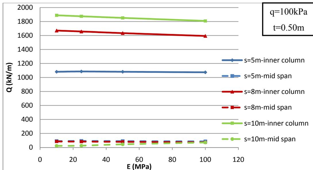
Figure 4.4 Q vs E for various spacings under the columns and mid-spans
