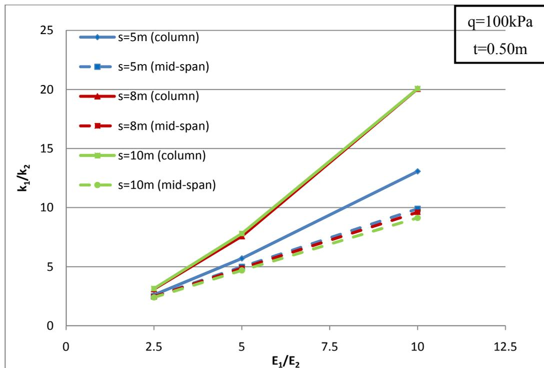
**Figure 4.10 Relation between  $k_1/k_2$  and  $E_1/E_2$  for various column spacings under column and mid-spans**
