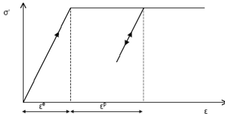
**Figure 2.3 Basic idea of an elastic perfectly plastic model (PLAXIS 3D Foundation Manual, 2007)**
