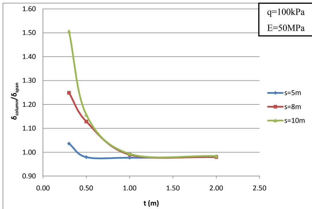
**Figure 4.21  $\delta_{\text{column}}/\delta_{\text{span}}$  vs  $t$  for various column spacings**
