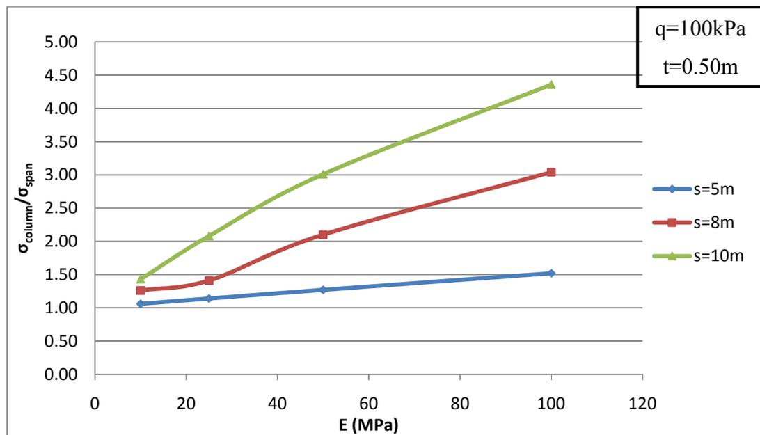
**Figure 4.6  $\sigma_{\text{column}}/\sigma_{\text{span}}$  vs E for various column spacings**
