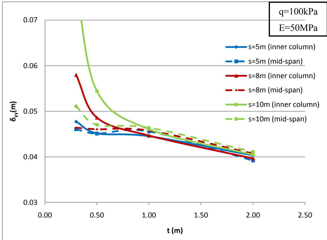
**Figure 4.16  $\delta_{yy}$  vs  $t$  for various column spacings under the columns and mid-spans**
