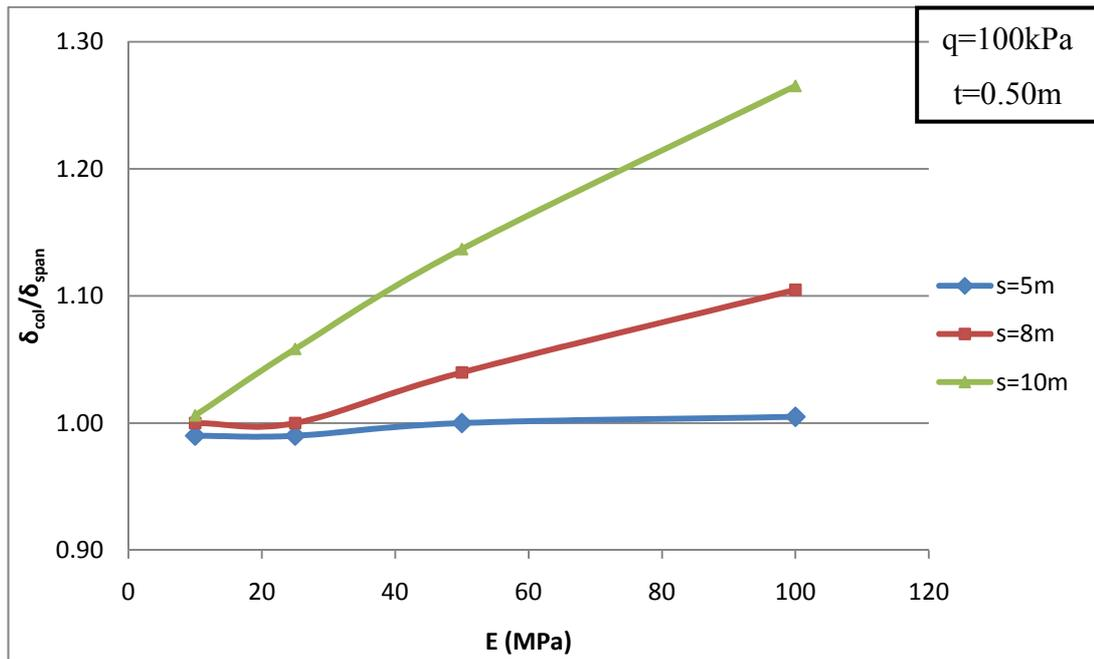
**Figure 4.7  $\delta_{column}/\delta_{span}$  vs E for various column spacings**
