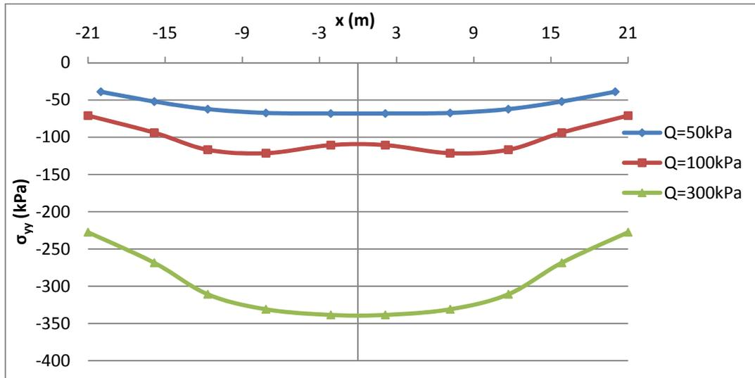
**Figure 3.12 Comparison of contact stress distribution of Pattern A for Cases 3-1, 3-2 and 3-3**
