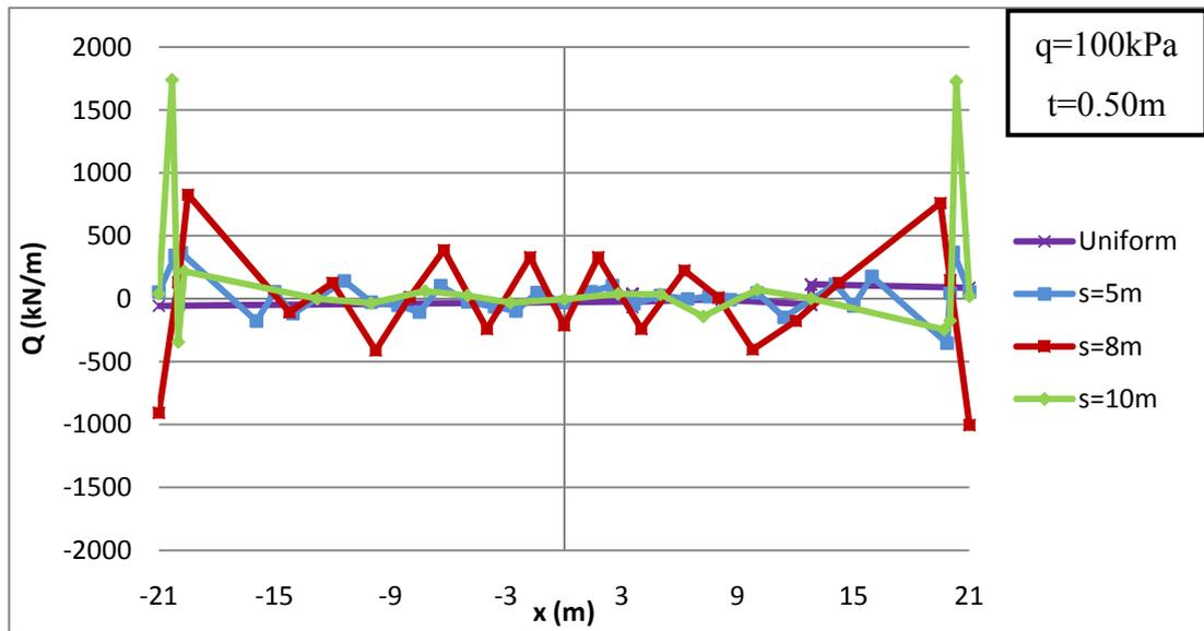
**Figure 4.31 Shear force distributions for pattern A and pattern B**
