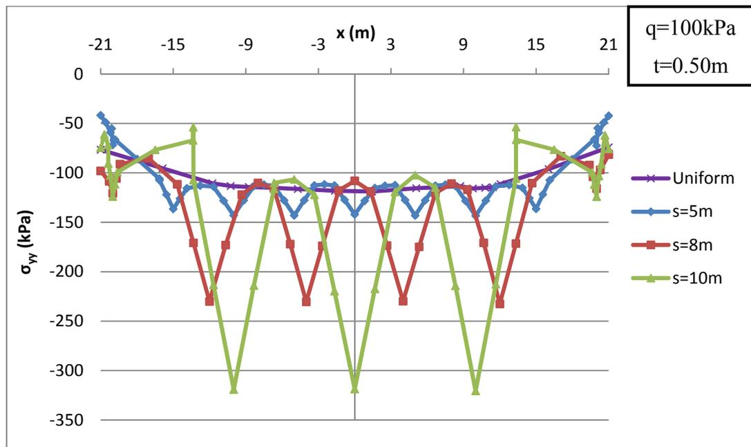
**Figure 4.28 Contact stress distributions for pattern A and pattern B**
