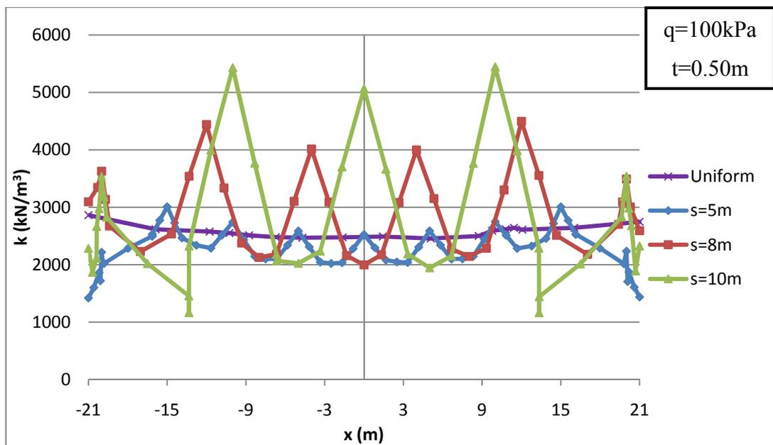
Figure 4.30 Modulus of subgrade reaction distributions for pattern A and pattern B
