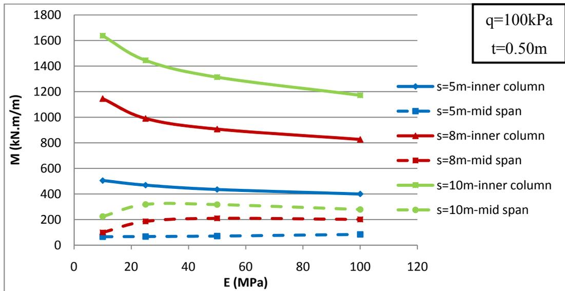
**Figure 4.5 M vs E for various spacings under the columns and mid-spans**
