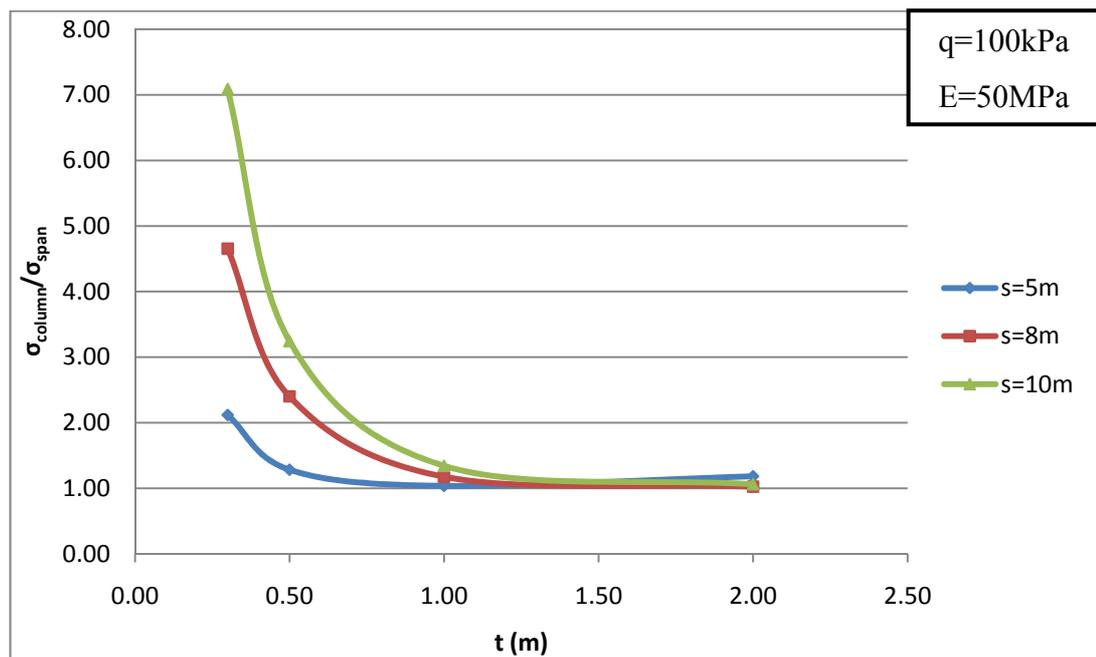
**Figure 4.20  $\sigma_{\text{column}}/\sigma_{\text{span}}$  vs  $t$  for various column spacings**
