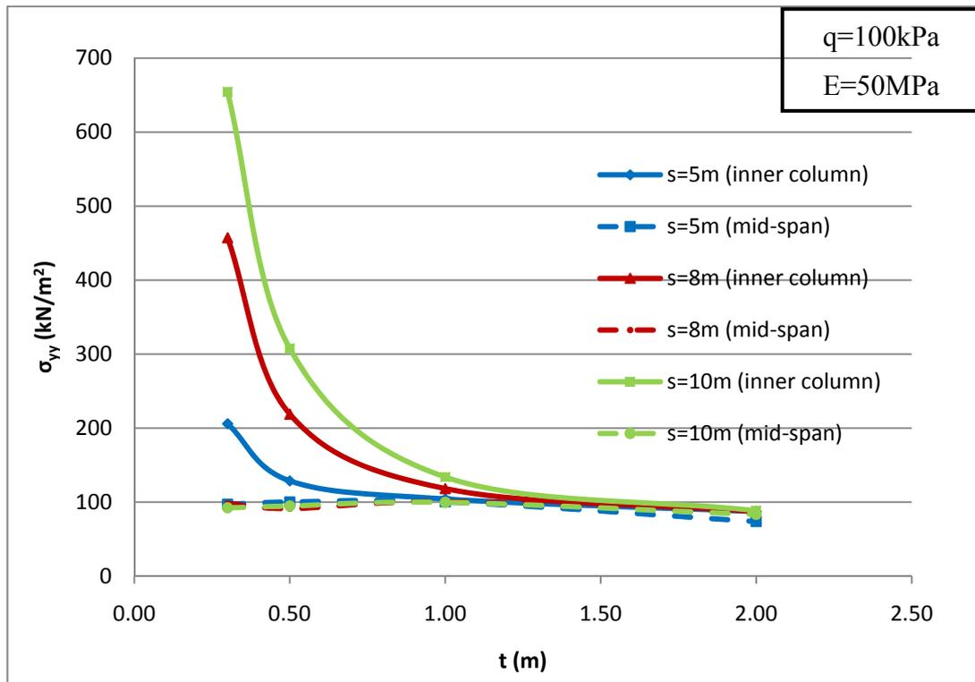
**Figure 4.15  $\sigma_{yy}$  vs  $t$  for various column spacings under the columns and mid-spans**
