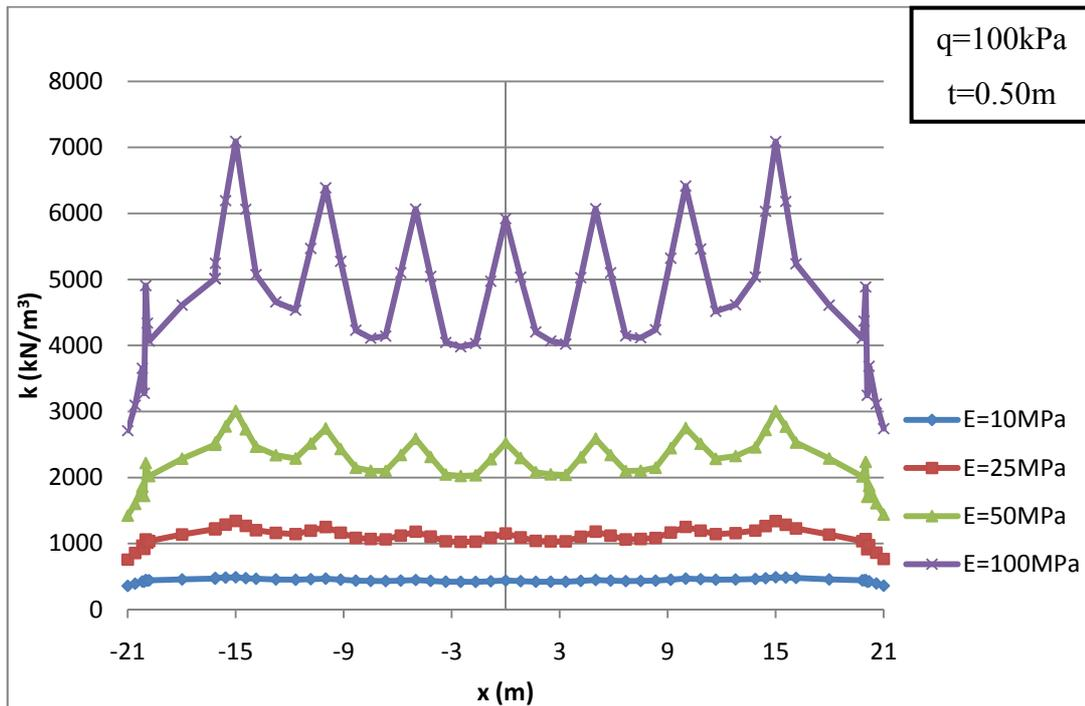
**Figure 3.19 Comparison of modulus of subgrade reaction distribution of Pattern B-s = 5 m for Cases 1-1, 1-2, 1-3 and 1-4**
