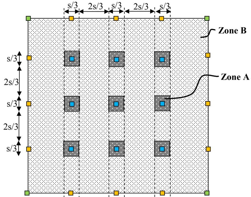
**Figure 4.14 Zones for contact stress distribution for variation in foundation thickness of Pattern B –  $s = 10$  m**
