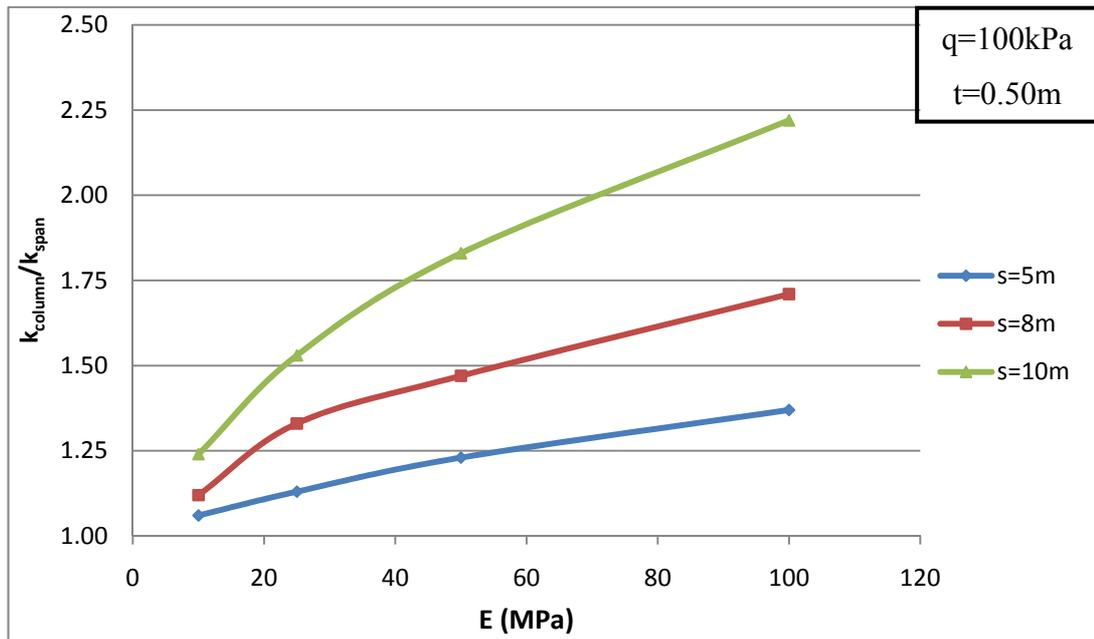
**Figure 4.8  $k_{\text{column}}/k_{\text{span}}$  vs E for various column spacings**
