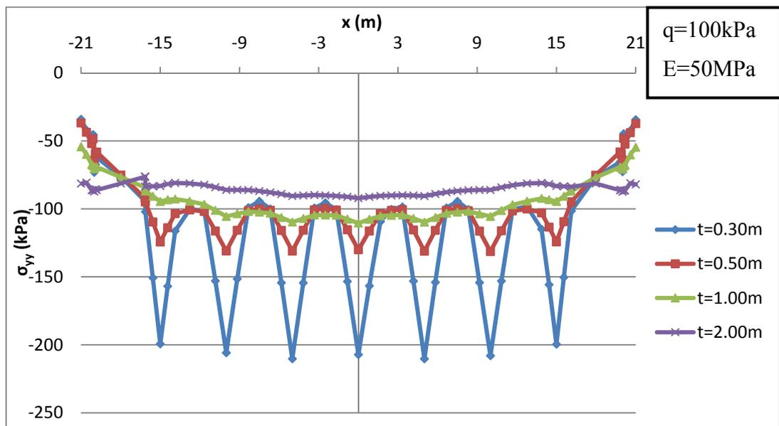
**Figure 3.20 Comparison of contact stress distribution of Pattern B -  $s = 5$  m for Cases 2-1, 2-2, 2-3 and 2-4**
