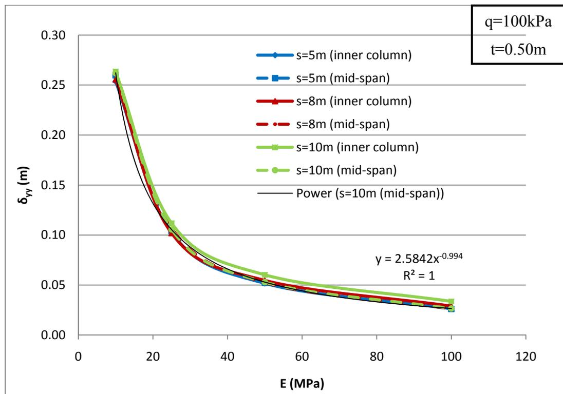
**Figure 4.2  $\delta_{yy}$  vs E for various spacings under the columns and mid-spans**
