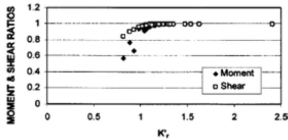
**Figure 2.12 Results for concentrically loaded square footings for shear and moment (Tabsh and Al-Shawa, 2005)**
