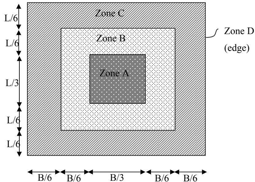
**Figure 3.8 Modulus of subgrade reaction distribution over the mat foundation for Pattern A**
