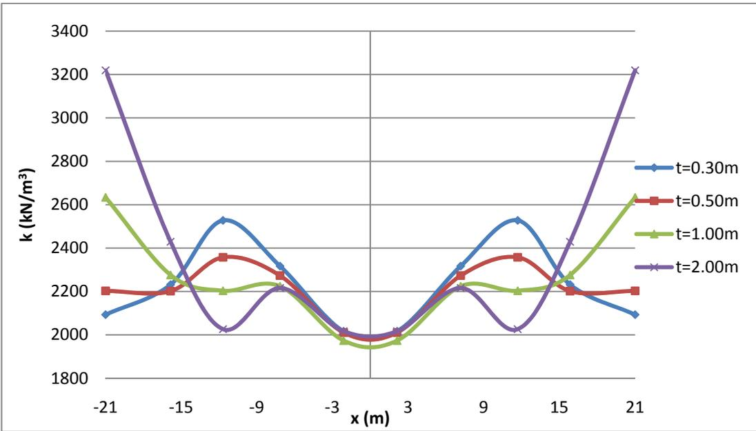
**Figure 3.11 Comparison of modulus of subgrade reaction of Pattern A for Cases 2-1, 2-2, 2-3 and 2-4**
