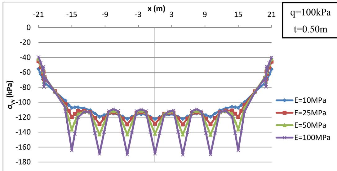
**Figure 3.17 Comparison of contact stress distribution of Pattern B-s = 5m for Cases 1-1, 1-2, 1-3 and 1-4**
