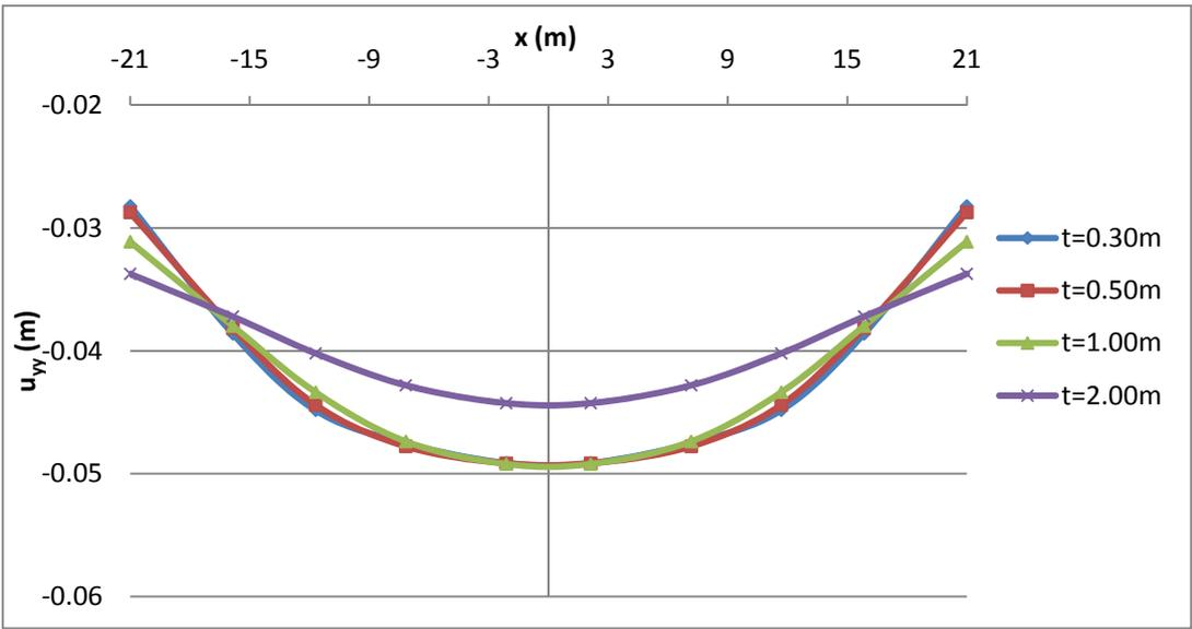
**Figure 3.10 Comparison of settlement distribution of Pattern A for Cases 2-1, 2-2, 2-3 and 2-4**
