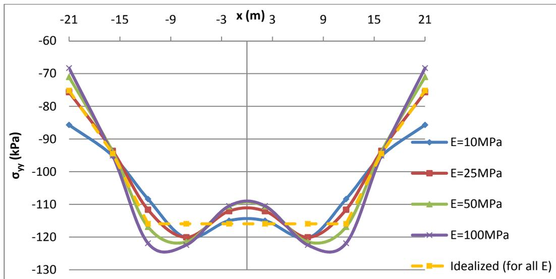
**Figure 3.5 Comparison of contact stress distribution of Pattern A for Cases 1-1, 1-2, 1-3 and 1-4**
