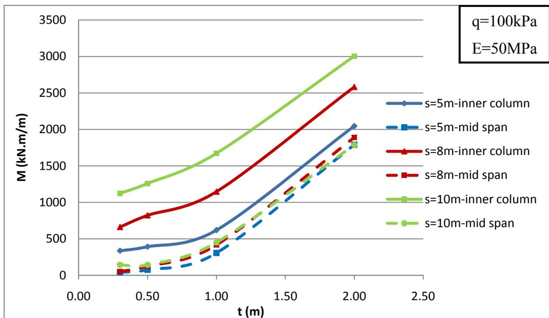
**Figure 4.19 M vs t for various column spacings under the columns and mid-spans**
