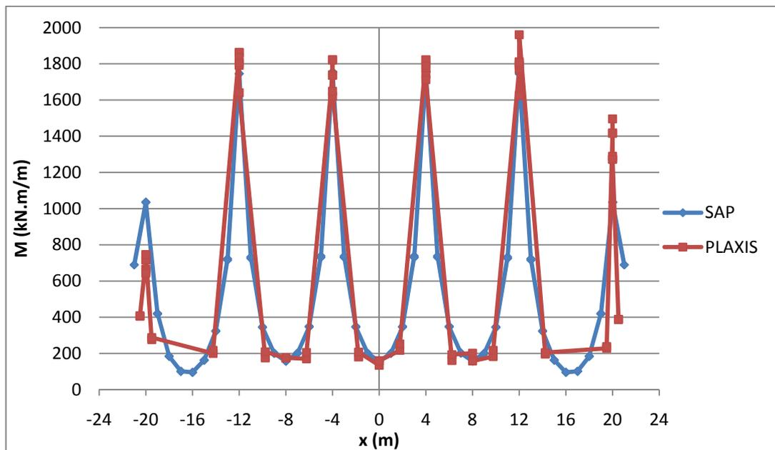
**Figure 4.34 Comparison of bending moment distributions obtained from PLAXIS and SAP**
