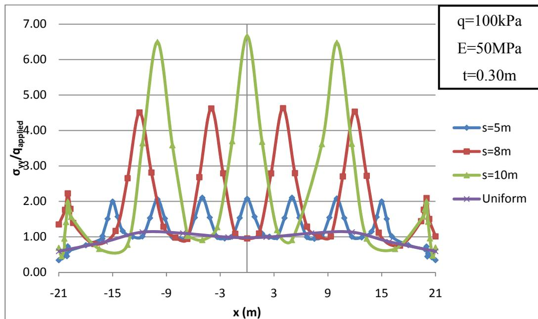
**Figure 4.23 Normalized contact stress distribution for various column spacings for  $t = 0.30 \text{ m}$**
