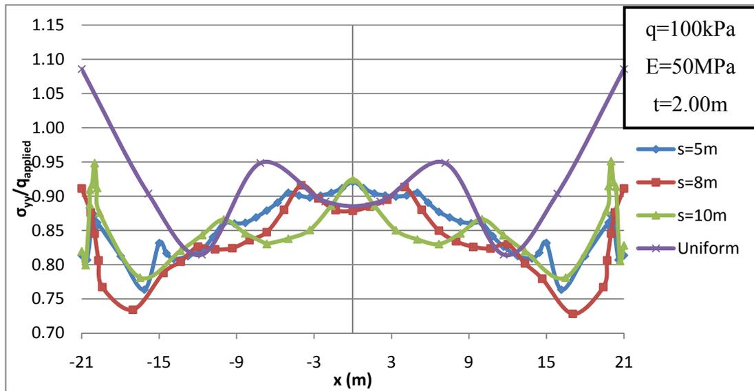
**Figure 4.26 Normalized contact stress distribution for various column spacings for  $t = 2.00$  m**
