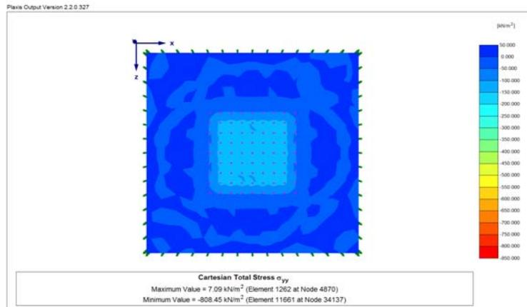
**Figure 3.16 Contact stress distribution of Pattern B-s = 5 m for Case 1-3**
