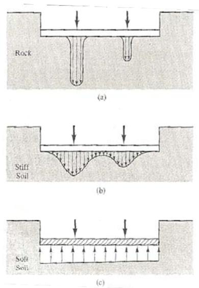
**Figure 2.2 Distribution of bearing pressure under a mat foundation; (a) on bedrock or very hard soil; (b) on stiff soil; (c) on soft soil (Adapted from Teng, 1962 by Coduto, 2001)**
