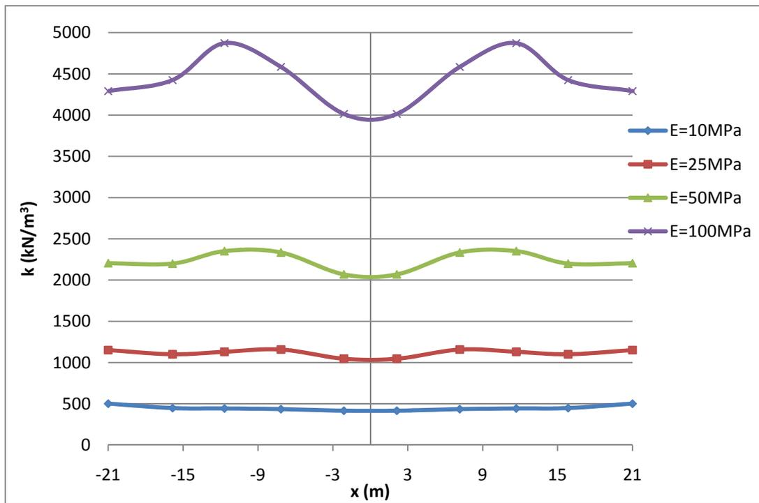
**Figure 3.7 Comparison of modulus of subgrade reaction of Pattern A for Cases 1-1, 1-2, 1-3 and 1-4**
