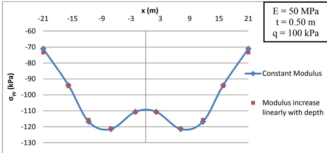
**Figure 3.1 Comparison of contact stress distribution between constant E and variable E depending on depth (500 kPa / m) analysis in Mohr-Coulomb model**
