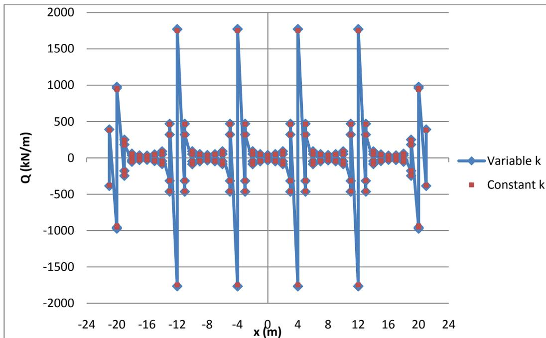
**Figure 4.35 Comparison of shear force distribution between *Variable k* and *Constant k* analyses**
