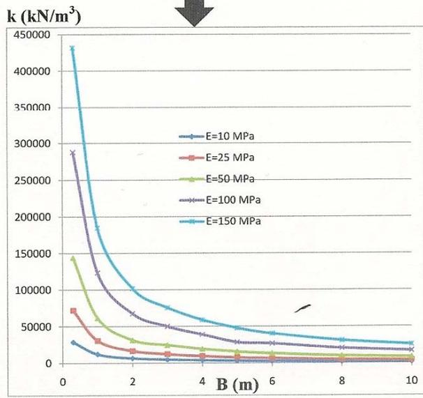
Figure 3.15 Relationship between B, E and k of Pattern A
