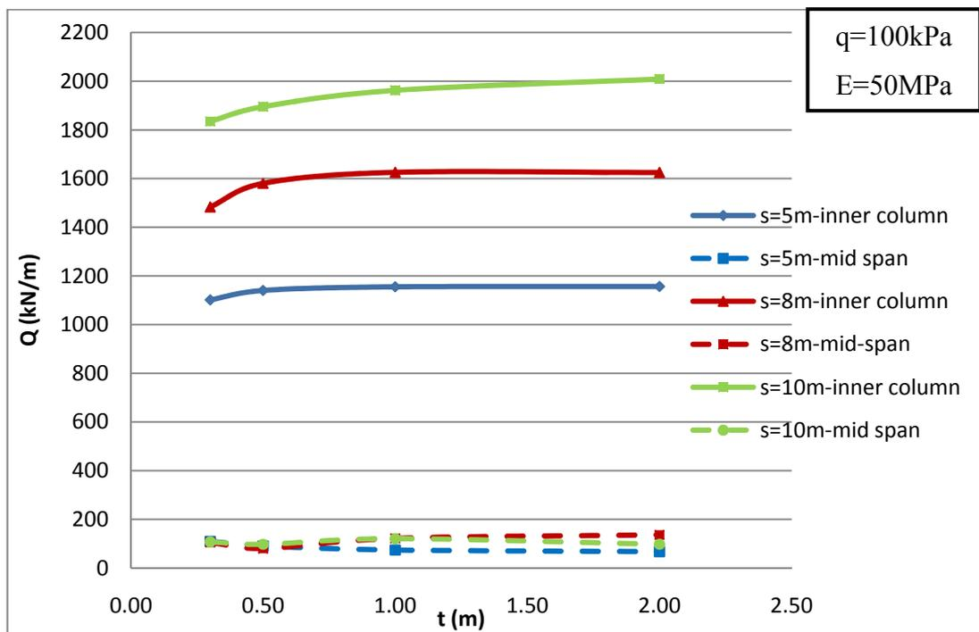
**Figure 4.18 Q vs t for various column spacings under the columns and mid-spans**
