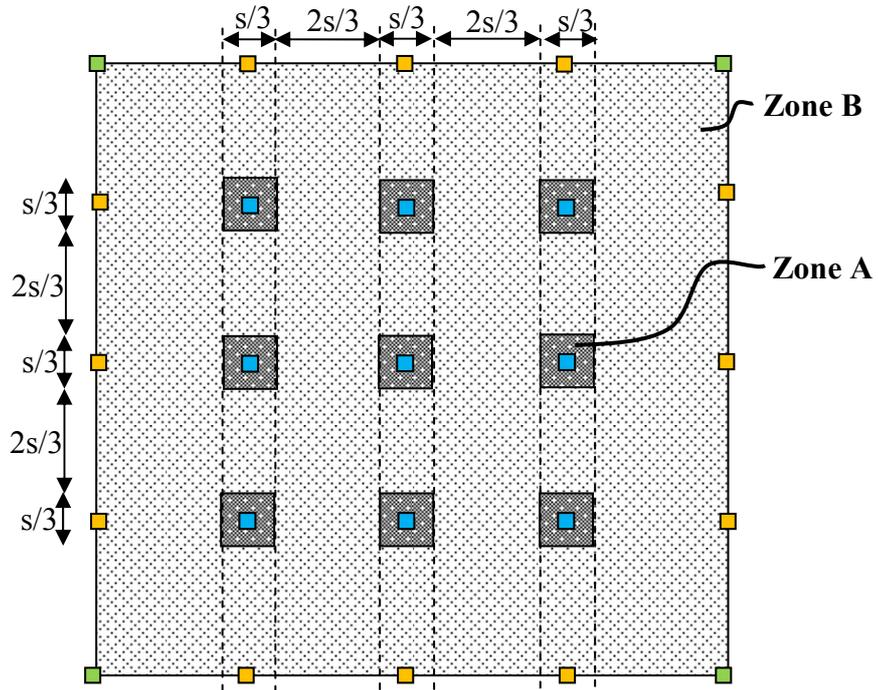
Figure 4.27 Zones for contact stress distribution for variation in foundation thickness of Pattern B –  $s = 10$  m
