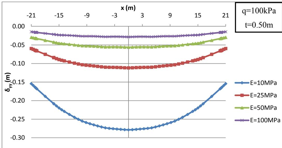
**Figure 3.18 Comparison of settlement distribution of Pattern B-s = 5 m for Cases 1-1, 1-2, 1-3 and 1-4**
