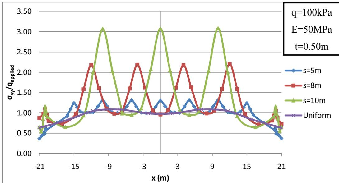
**Figure 4.24 Normalized contact stress distribution for various column spacings for  $t = 0.50$  m**
