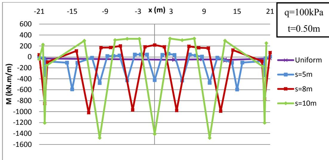
**Figure 4.32 Bending moment distributions for pattern A and pattern B**
