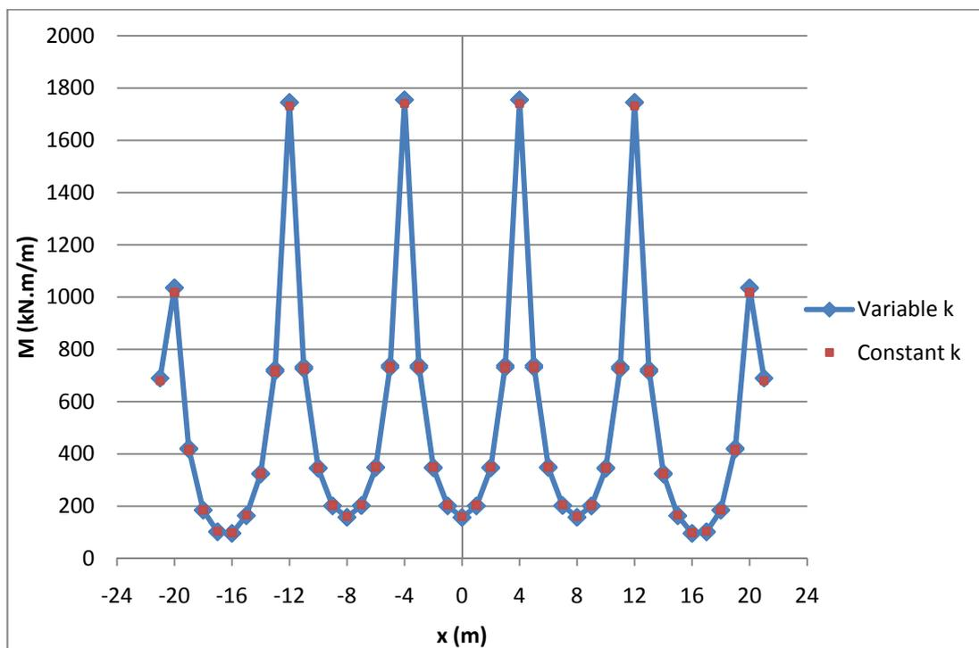
**Figure 4.36 Comparison of bending moment distribution between *Variable k* and *Constant k* analyses**
