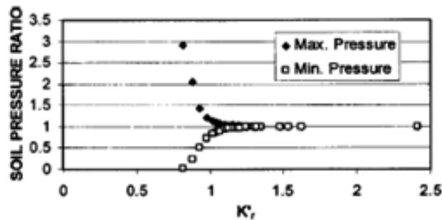
**Figure 2.5 Results for concentratedly loaded square footings soil pressure (Tabsh and Al-Shawa, 2005)**
