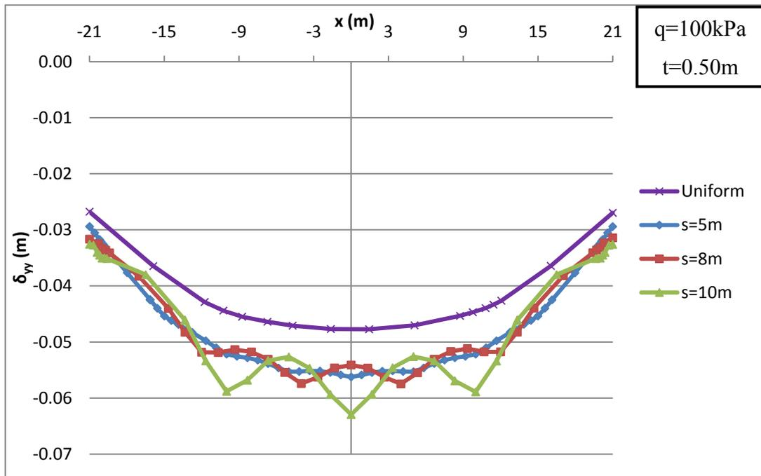
Figure 4.29 Settlement distributions for pattern A and pattern B
