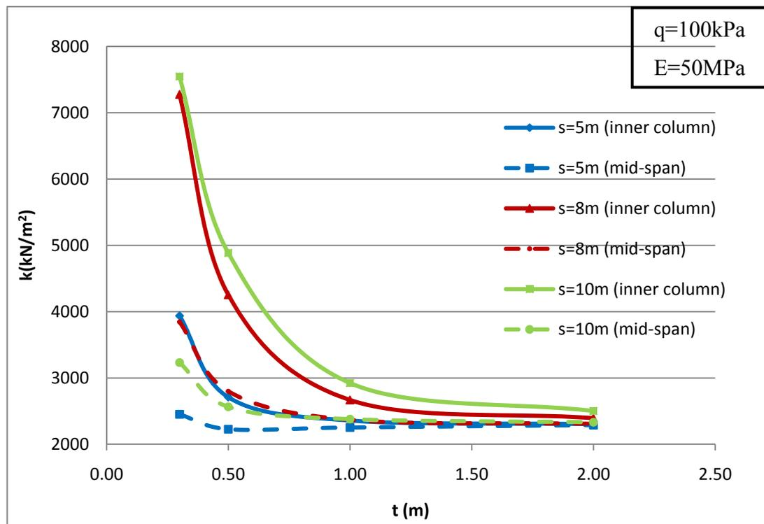
**Figure 4.17 t vs k for various column spacings under the columns and mid-spans**
