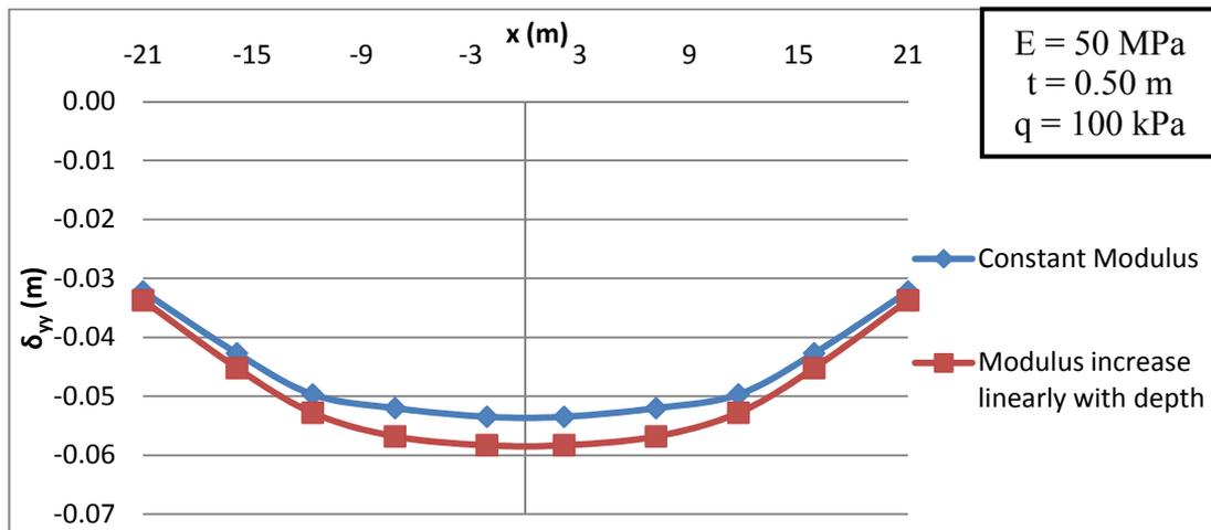
**Figure 3.2 Comparison of settlement distribution between constant E and variable E depending on depth (500 kPa / m) analysis in Mohr-Coulomb model**
