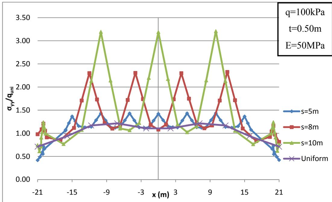
**Figure 4.13 Normalized contact stress distribution for various column spacings for E = 50 MPa**
