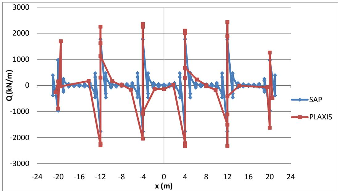
**Figure 4.33 Comparison of shear force distributions obtained from PLAXIS and SAP**
