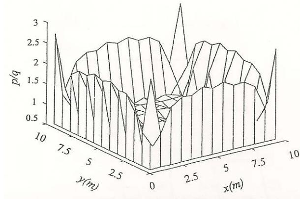
**Figure 2.7 Contact pressure distribution beneath a square plate on a stratum (Wang et. al. ,2003)**
