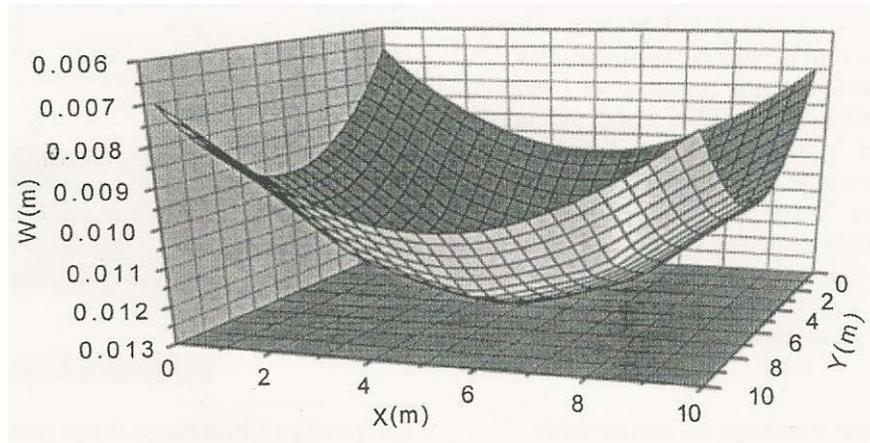
**Figure 2.11 Three dimensional deformation of a square plate on a stratum
