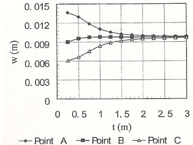
**Figure 2.10 Variation of plate deformation with the plate thickness (Wang et. al. ,2003)**
