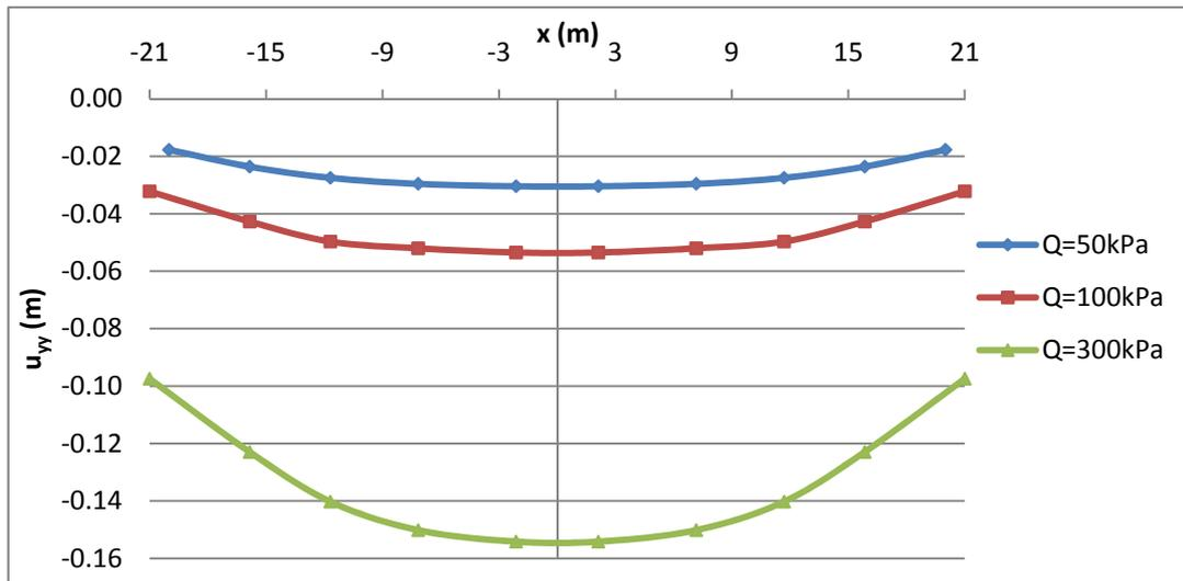
**Figure 3.13 Comparison of settlement distribution of Pattern A for Cases 3-1, 3-2 and 3-3**
