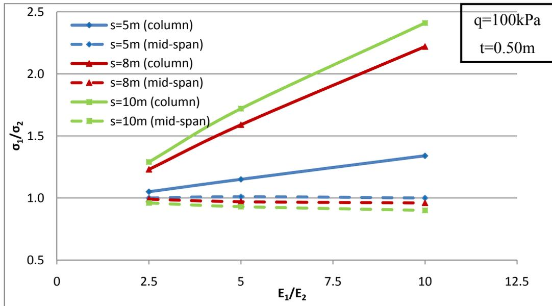
**Figure 4.9 Relation between  $\sigma_1/\sigma_2$  and  $E_1/E_2$  for various column spacings under column and mid-spans**
