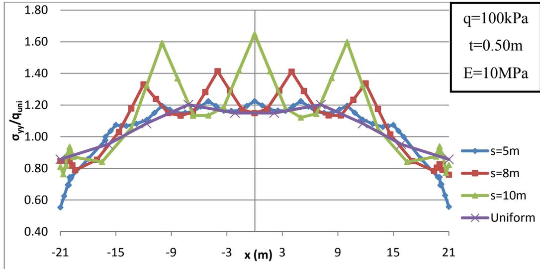
**Figure 4.11 Normalized contact stress distribution for various column spacings for E = 10 MPa**
