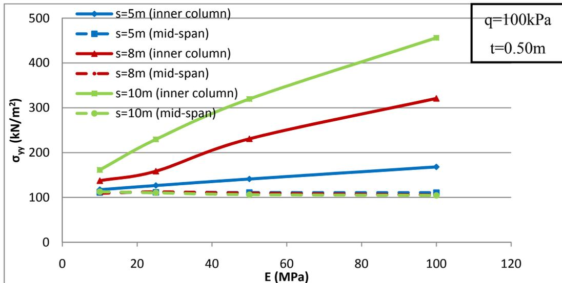
Figure 4.1  $\sigma_{yy}$  vs  $E$  for various spacings under the columns and mid-spans
