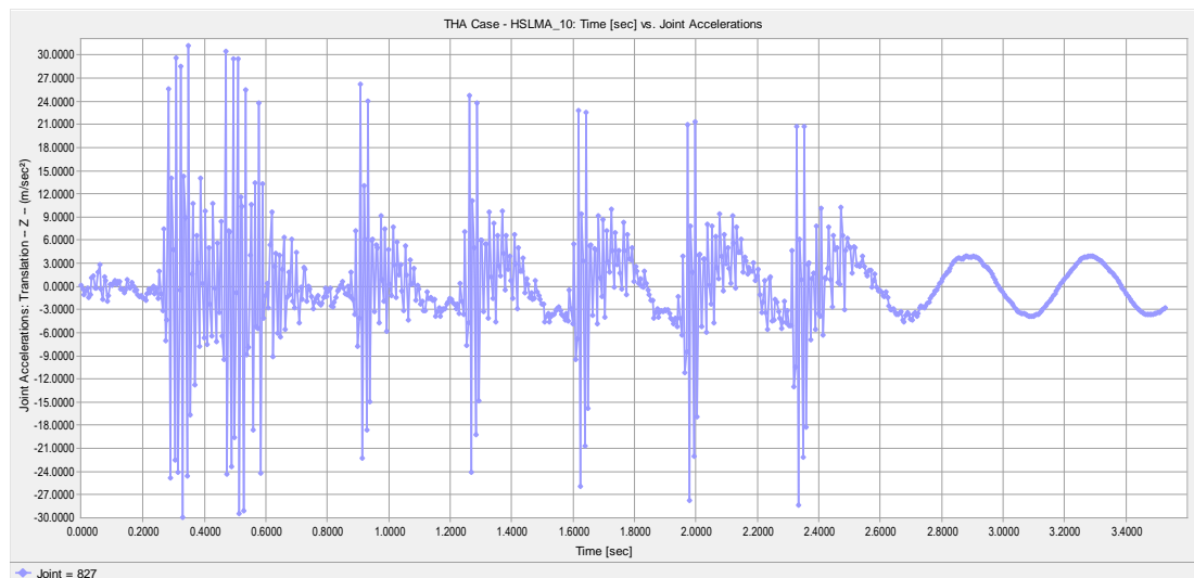
Figure A.48 Joint Acceleration vs. Time graph of the bridge having 24.5 m span length, 1.30 m girder height, 700 MPa ballast stiffness for 76.08 m/s vehicle speed.
