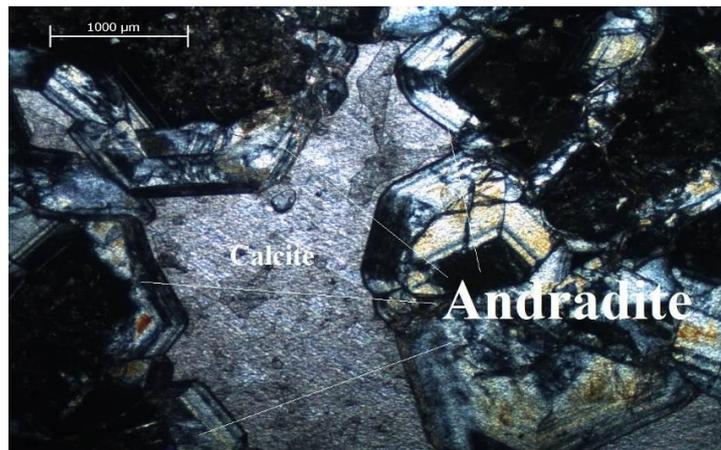
Figure 4.16. Zoned andradite crystals in the early calc-silicate alteration, and calcite infill (Sample taken from 262.2 m depth of ES-9).
