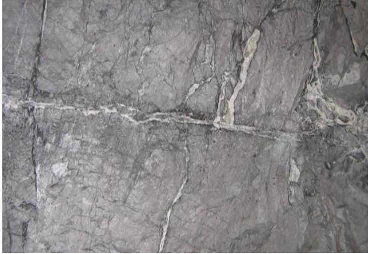
Figure 3.2. Recrystallized limestone with calcite veins and veinlets
