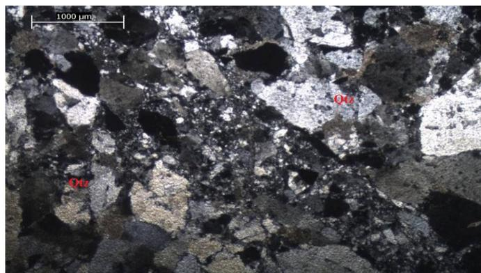
Figure 4.8 Coarse-grained, anhedral quartz crystals of silicified rock (Sample taken from 270.1 m depth of ES-9 (Qtz:Quartz)).
