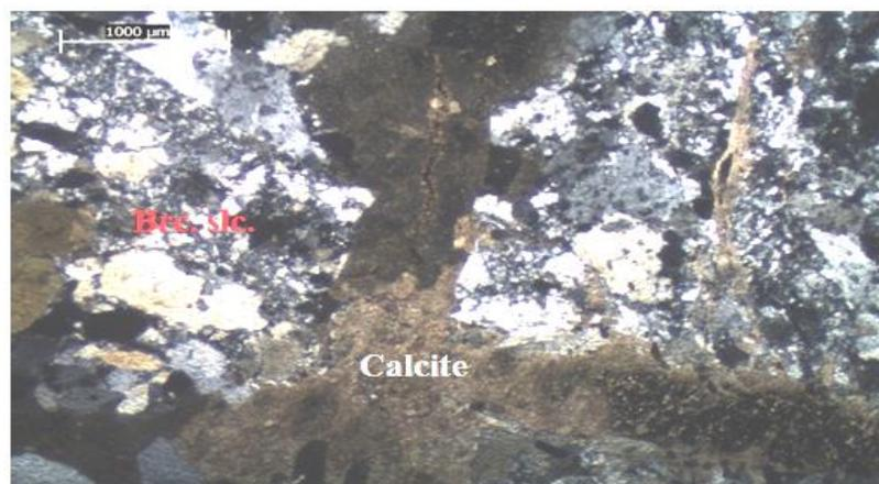
Figure 4.12. Hydrothermal breccia and early silicification cut by calcite veinlets. (Sample taken from 270.1 m depth of ES-9. Bre. Slc.:Brecciated silicified rock)
