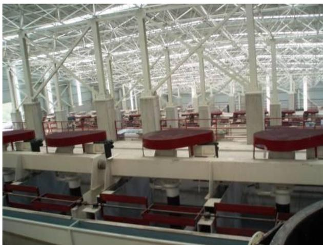
Figure 1.5. Ore dressing plant for ore production by Eczacıbaşı ESAN Madencilik.
