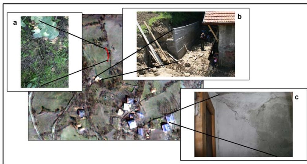
Figure 4.10. The anomalies investigated through the field surveys, the photos are overlaid to the remote sensing image of the region a. A fracture representation of the region b. The protection wall of a house in the region c. The cracks inside the house
