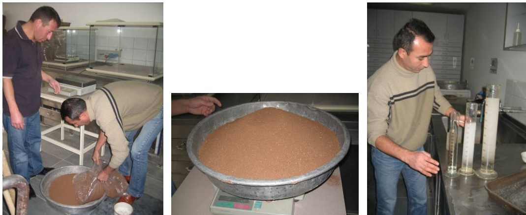
Figure 3.8 Addition of water to the sample in order to obtain the optimum water content
