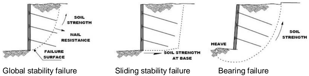
Figure 1.10 External failure modes (FHWA, 2003)
