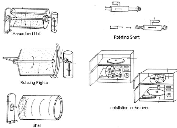
**Figure 1** A removable rotary drum for microwave ovens
