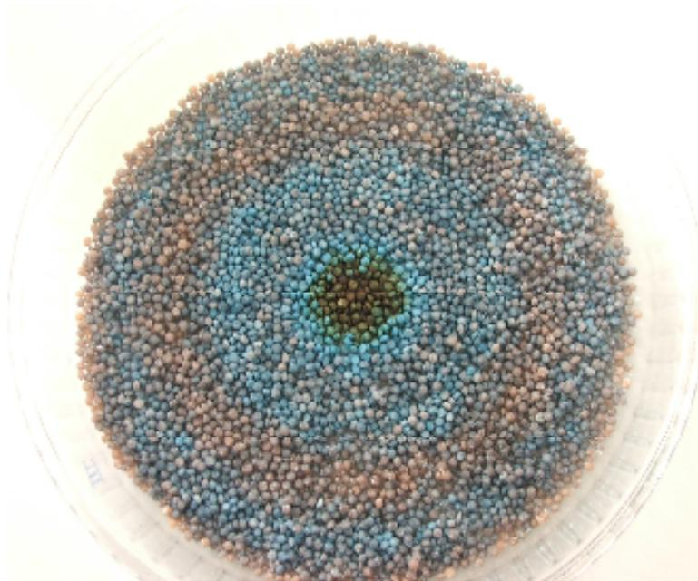
**Figure 30** Electromagnetic field distribution over the turntable
