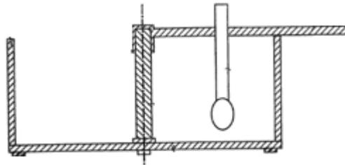
**Figure 3** A vertical stirrer fixed on a rotating shaft for microwave ovens
