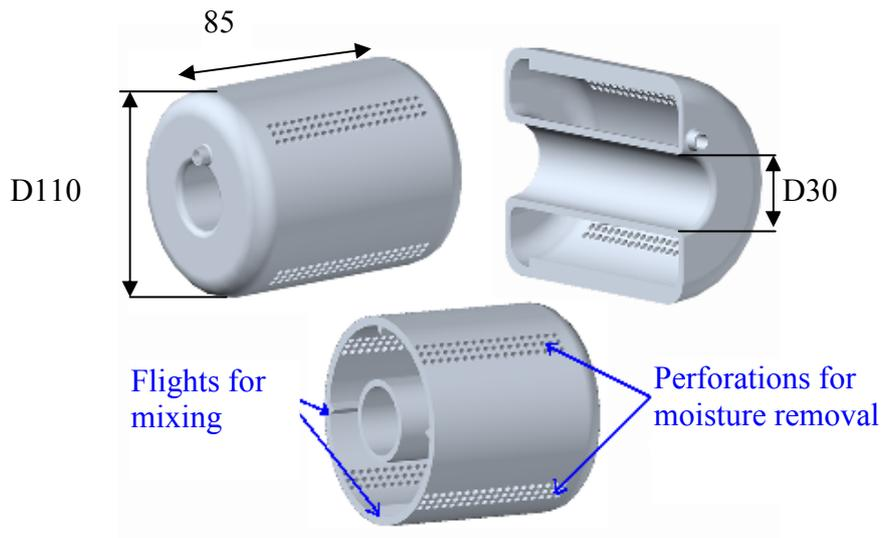
**Figure 13** The Rotating Drums
