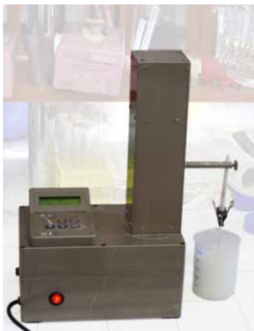
Figure 3.2-1 Dip coating apparatus
