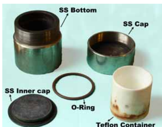
Figure 3.4-1 Autoclave setup for hydrothermal treatment of TiO 2
