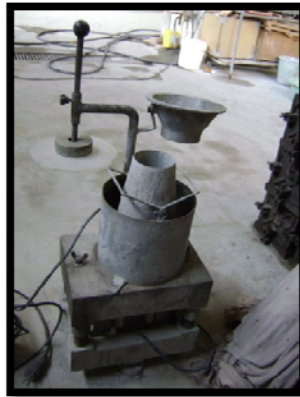
Figure 3.5 Illustration of Vebe test of concrete
