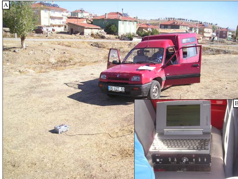
Figure 5.23. Photo A: A view from the microtremor measurement at the Mob-49 site. Photo B: the amplifier (black box) and the laptop used during recording ambient noise.
