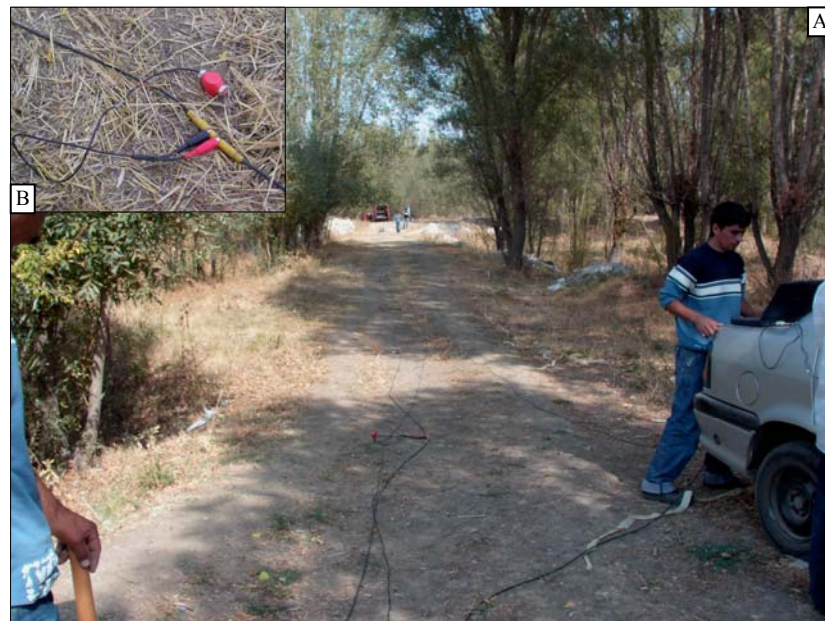
Figure 5.3. Photo A: A view of the Seis-2 site showing the general configuration of the surface wave method applied at the sites, photo B: a view of the 4.5 Hz geophones that were connected to the seismograph through a spread cable.
