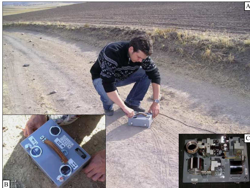
Figure 5.22. Photo A: A view from the microtremor measurement at the Mob-89 site. Photo B: a close view of the UP-255s seismometer, Photo C: a view of the inside of the seismometer.
