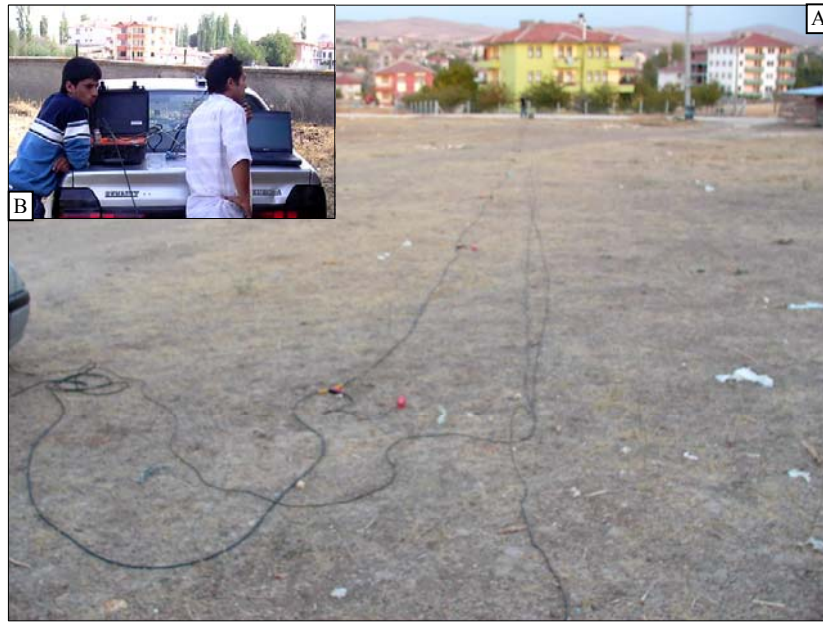
Figure 5.4. Photo A: A view of the surface wave measurement configuration from site Seis-19. Photo B: a view of the equipment used for data acquisition, monitoring and storage.
