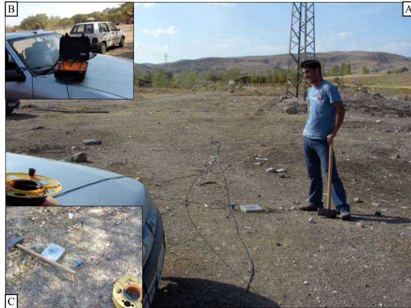
Figure 5.5. Photo A: A view showing the application of the MASW method. Photo B: ABEM RAS 24 seismograph. Photo C: The MASW equipment (sledge hammer, striker plate and trigger geophone).
