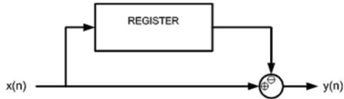
Figure 14: Subtraction block of Sinc filter.
