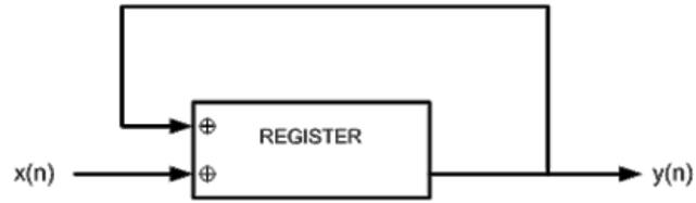
Figure 13: Addition block of Sinc filter.
