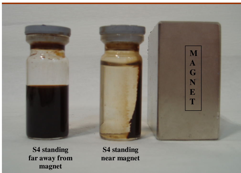
Figure 3.25 Magnetic property of S4, in situ prepared PMAA coated magnetite agglomerates under ultrasonic agitation
