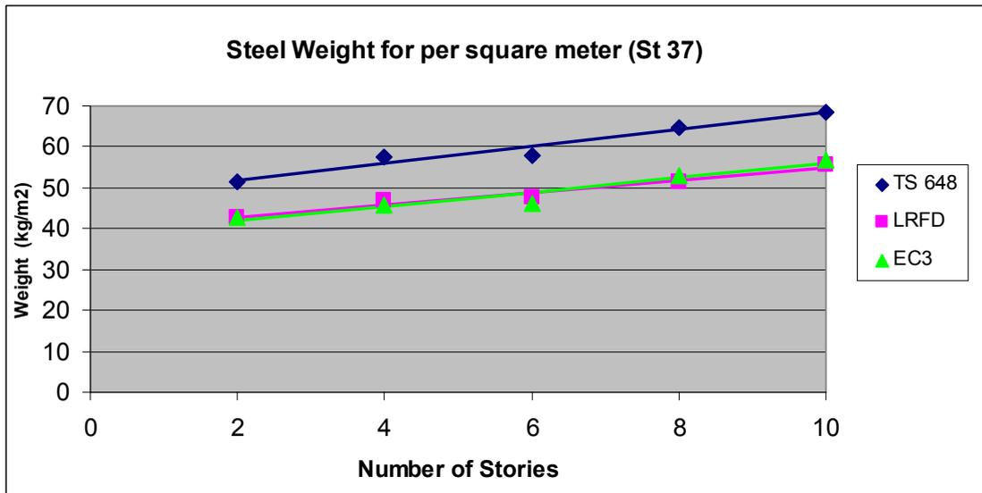
Figure 11.5 Weight of steel used on 1 m<sup>2</sup>
