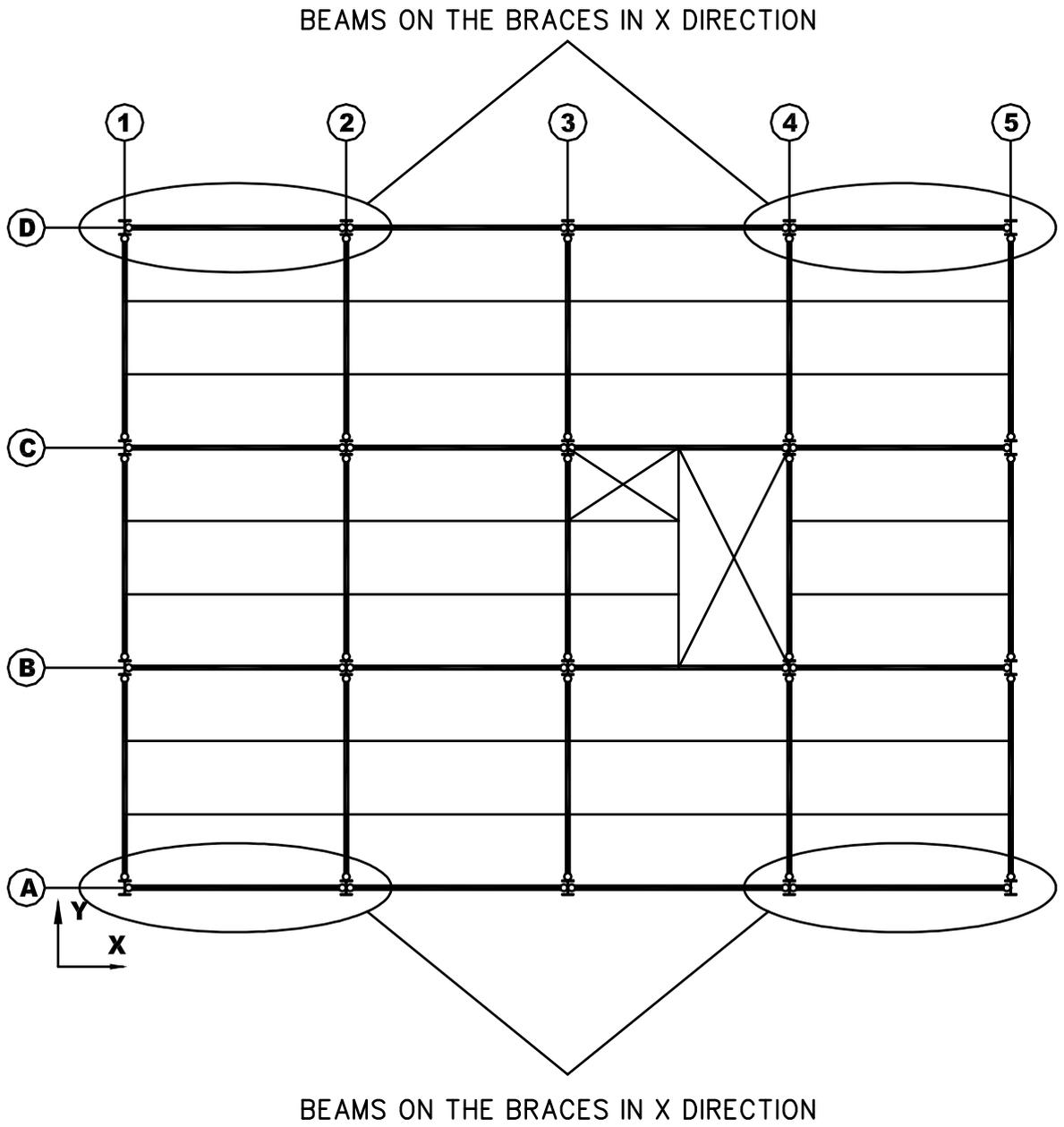
Figure 11.3 Beams connected to the braces in X direction view
