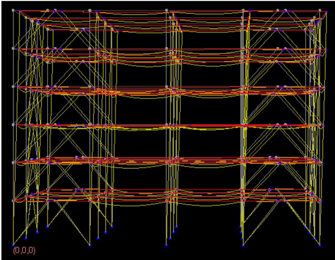
Figure 10.6 Deformed Shape of LARSA Model
