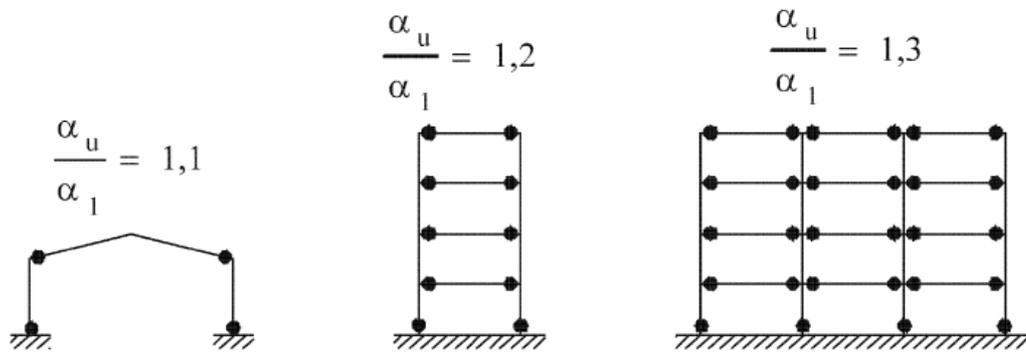
Figure 9.4 Moment resisting frames
