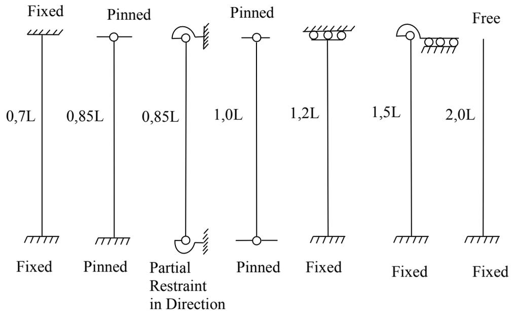
Figure 5.3 Buckling Lengths ( $L_{cr}$ ) for compression members
