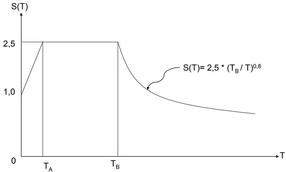
Figure 9.1 Shape of Design Spectrum
