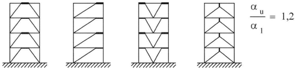
Figure 9.3 Frames with eccentric bracing
