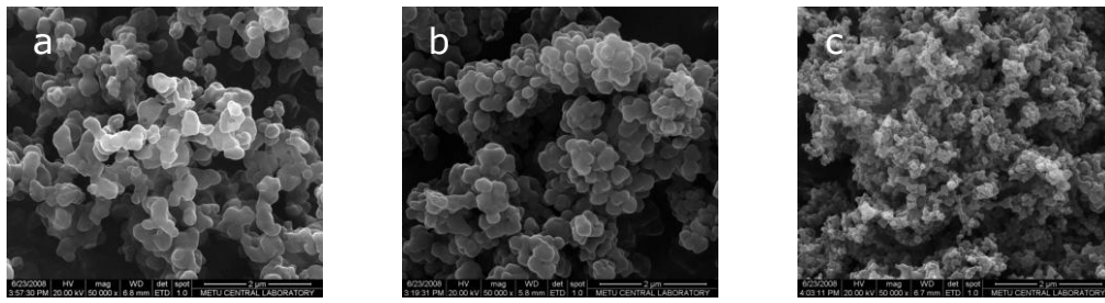
Figure 6 SEM of NPs based on pNIPAM, which was prepared by using various concentrations of crosslinker: (a) 0.22% (b) 0.44% (c) 0.88% (x50 000)
