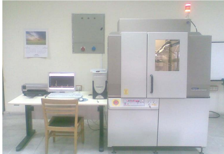
Figure 3.8. Rigaku Multiflex Powder X-ray diffractometer (14)
