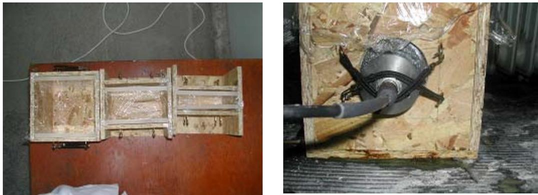
Figure 4.1. The wooden molds used in the experiments and attachment of transducers
