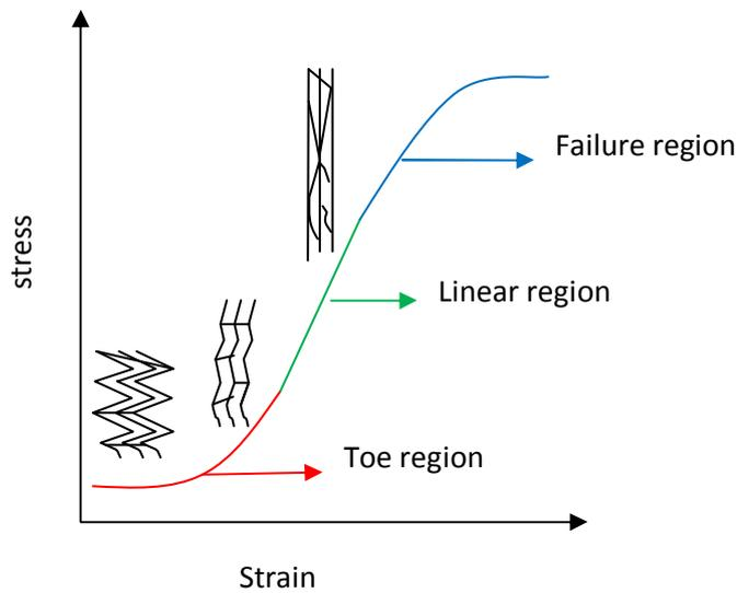
**Figure 1.5.** Characteristic stress strain curve of collagen and the location of the toe region (Adapted from Guelcher and Hollinger, 2006)
