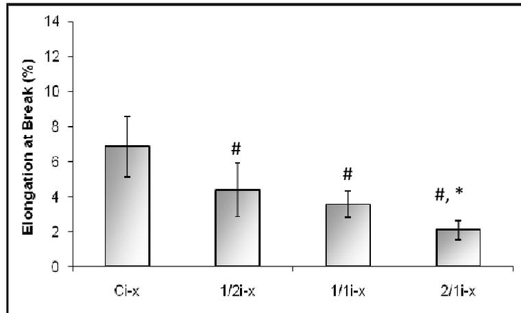
**Figure 3.16.** Comparison of elongation at break values of thin membranes containing only collagen (Ci-x), and different weight ratios of sericin/collagen (1/2i-x, 1/1i-x, 2/1i-x). Data are expressed as mean  $\pm$  SD ( $n \geq 6$ ). #: Significant difference from the group containing only collagen (Ck-x). \*: Significant difference from 1/2i-x.  $p < 0.05$ .
