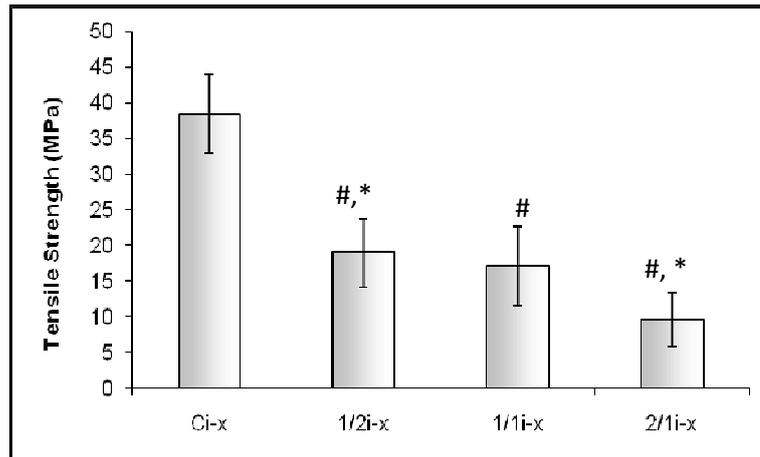
**Figure 3.12.** Comparison of tensile strength values of thin membranes containing only collagen (Ci-x), and different weight ratios of sericin/collagen (1/2i-x, 1/1i-x, 2/1i-x). Data are expressed as mean  $\pm$  SD ( $n \geq 6$ ). #: Significant difference from the group containing only collagen (Ci-x). \*: Significant difference between the dual protein groups.  $p < 0.05$ .
