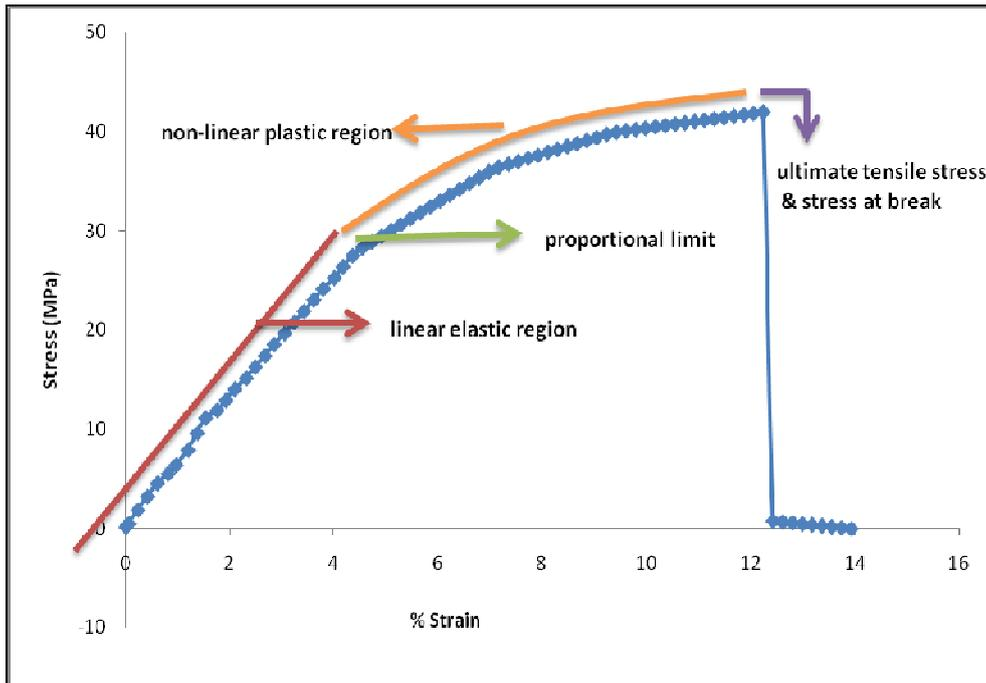
**Figure 3.7.** Representative stress-strain curve for collagen membrane (Ck-x) undergoing brittle failure
