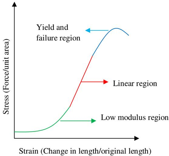
**Figure 1.2.** A typical stress-strain curve for wet skin (adapted from Silver, 1994).
