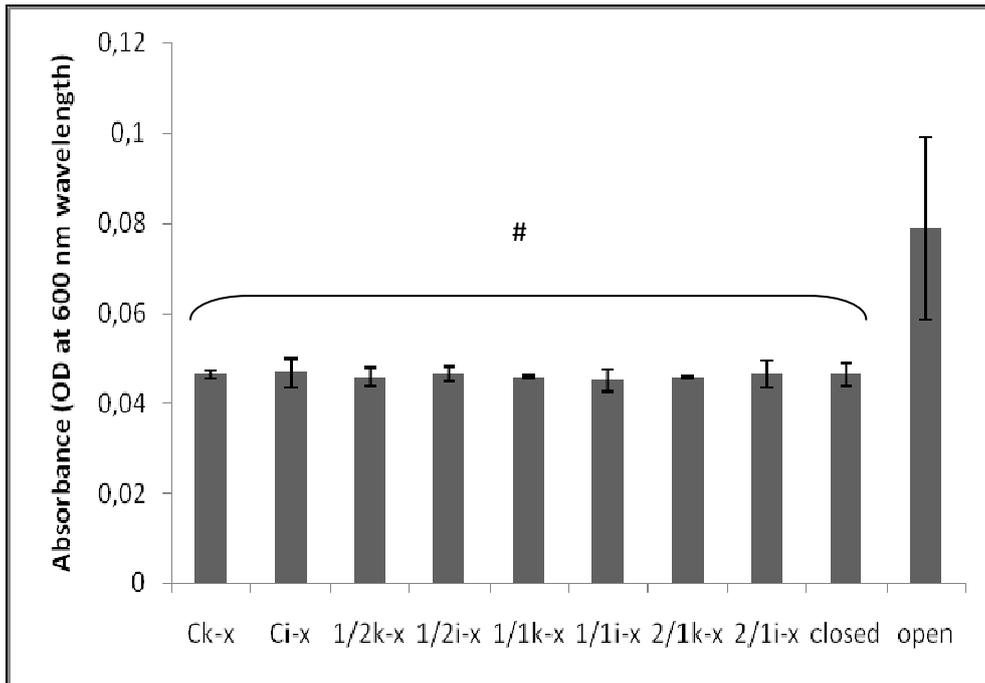
**Figure 3.5.** Absorbance (O.D. at 600 nm) measurement results of nutrient broths covered with thick and thin collagen (Ck-x, Ci-x) and sericin/collagen (1/2k-x, 1/2i-x, 1/1k-x, 1/1i-x, 2/1k-x, 2/1i-x) membranes after one week incubation time at RT. Controls are closed and open groups. Data are expressed as mean  $\pm$  SD (n =3). #: Significant difference from the open control.  $p < 0.05$ .
