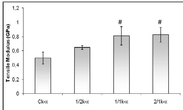
**Figure 3.13.** Comparison of tensile modulus values of thick membranes containing only collagen (Ci-x), and different weight ratios of sericin/collagen (1/2i-x, 1/1i-x, 2/1i-x). Data are expressed as mean  $\pm$  SD ( $n \geq 6$ ). #: Significant difference from the group containing only collagen (Ck-x).  $p < 0.05$ .
