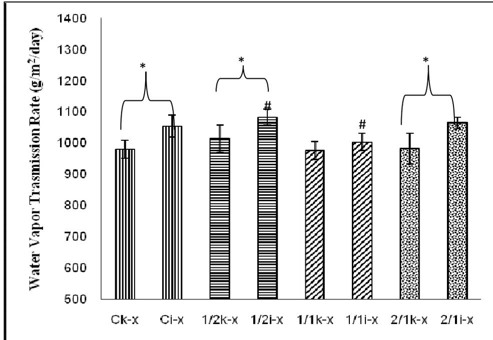
**Figure 3.4.** Comparison of water vapor transmission rates of cross-linked thick and thin collagen (Ck-x, Ci-x) and sericin/collagen (1/2k-x, 1/2i-x, 1/1k-x, 1/1i-x, 2/1k-x, 2/1i-x) membranes. Data are expressed as mean  $\pm$  SD ( $n \geq 4$ ). #: Significant difference between the groups of thin membranes. \*: Pairwise comparisons between thin and thick membranes of the same groups.  $p < 0.05$
