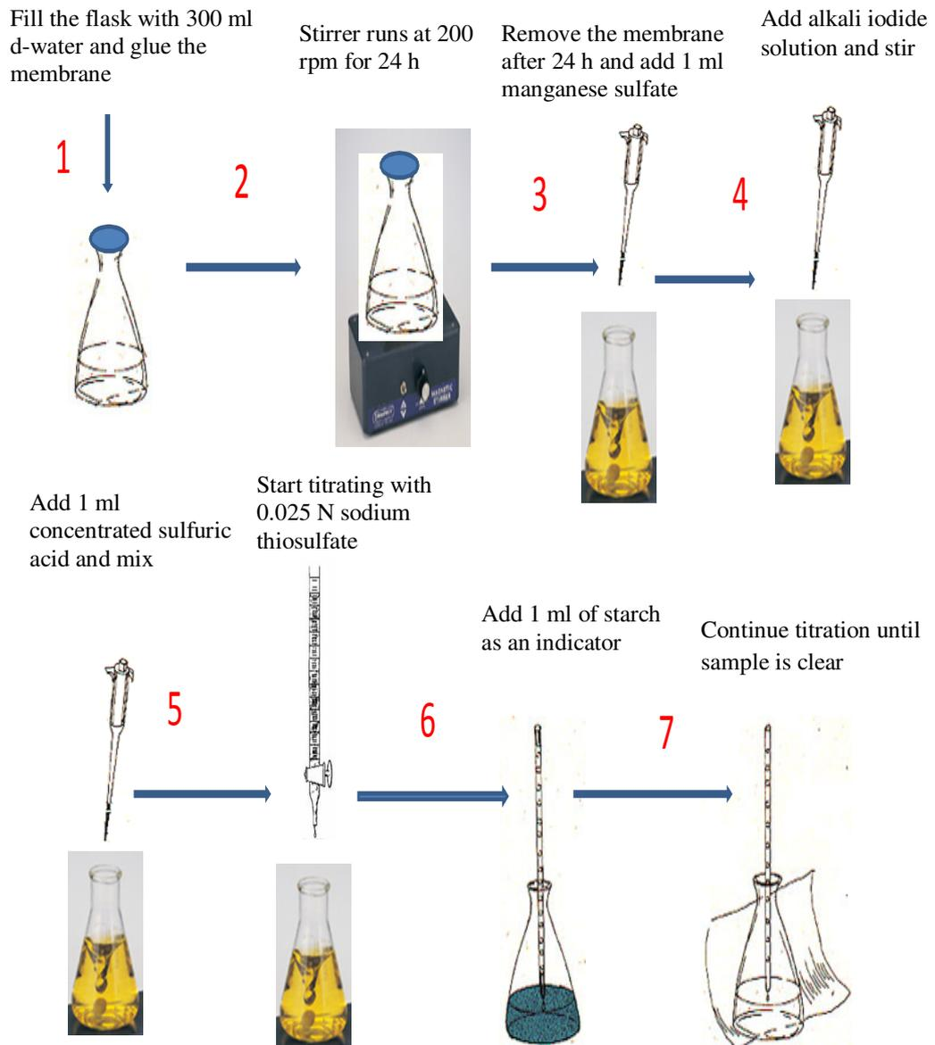
**Figure 2.4.** A schematic representation of the oxygen permeability test
