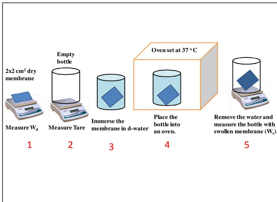
**Figure 2.2.** Experimental setup for testing water absorption of membranes
