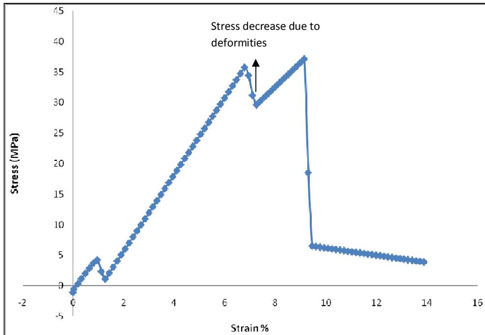
**Figure 3.9.** Stress-strain curve indicating the abrupt decrease in stress obtained for 1/2k-x
