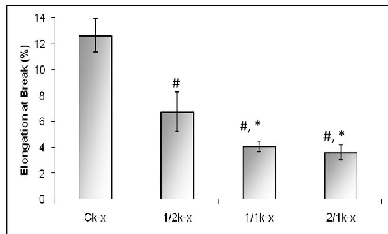
**Figure 3.15.** Comparison of elongation at break values of thick membranes containing only collagen (Ck-x), and different weight ratios of sericin/collagen (1/2k-x, 1/1k-x, 2/1k-x). Data are expressed as mean  $\pm$  SD ( $n \geq 6$ ). #: Significant difference from the group containing only collagen (Ck-x). \*: Significant difference from 1/2k-x.  $p < 0.05$ .
