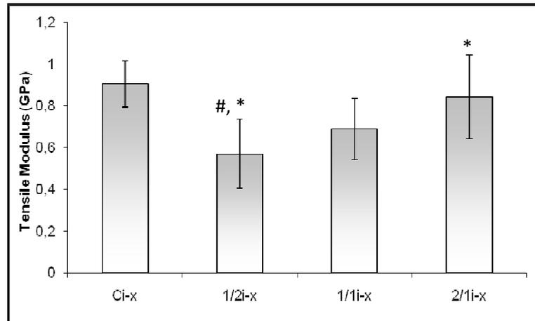
**Figure 3.14.** Comparison of tensile modulus values of thin membranes containing only collagen (Ci-x), and different weight ratios of sericin/collagen (1/2i-x, 1/1i-x, 2/1i-x). Data are expressed as mean  $\pm$  SD ( $n \geq 6$ ). #: Significant difference from the group containing only collagen (Ck-x). \* Significant difference between the dual protein groups:  $p < 0.05$ .
