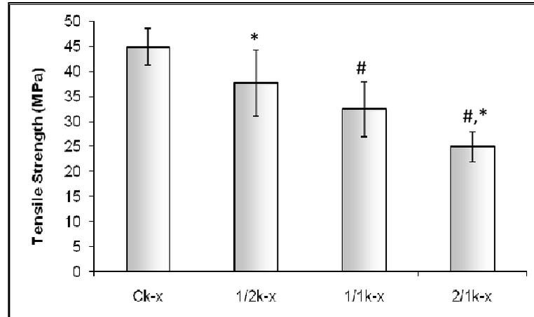
**Figure 3.11.** Comparison of tensile strength values of thick membranes containing only collagen (Ci-x), and different weight ratios of sericin/collagen (1/2k-x, 1/1k-x, 2/1k-x). Data are expressed as mean  $\pm$  SD ( $n \geq 6$ ). #: Significant difference from the group containing only collagen (Ck-x). \*: Significant difference between the dual protein groups.  $p < 0.05$ .
