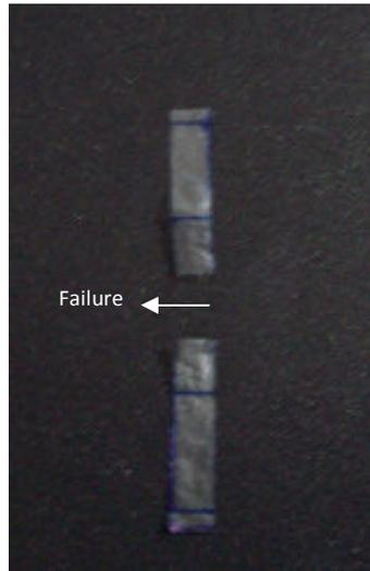
**Figure 3.10.** Successful tensile break occurred in the middle of the gauge length
