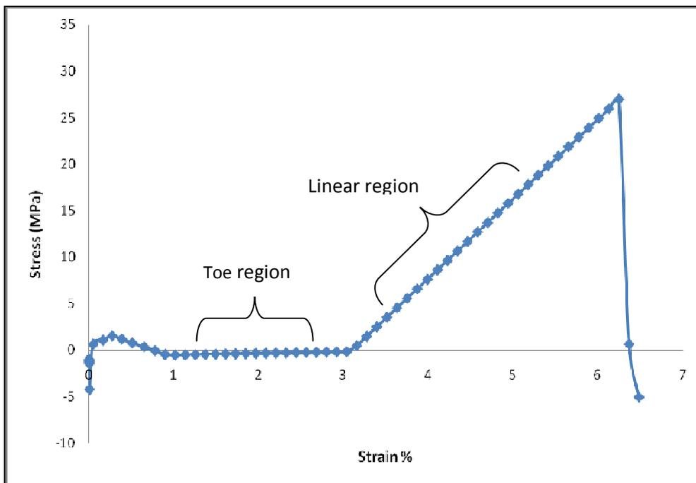
**Figure 3.8.** Stress-strain curve indicating the toe region in membranes obtained for 1/2k-x
