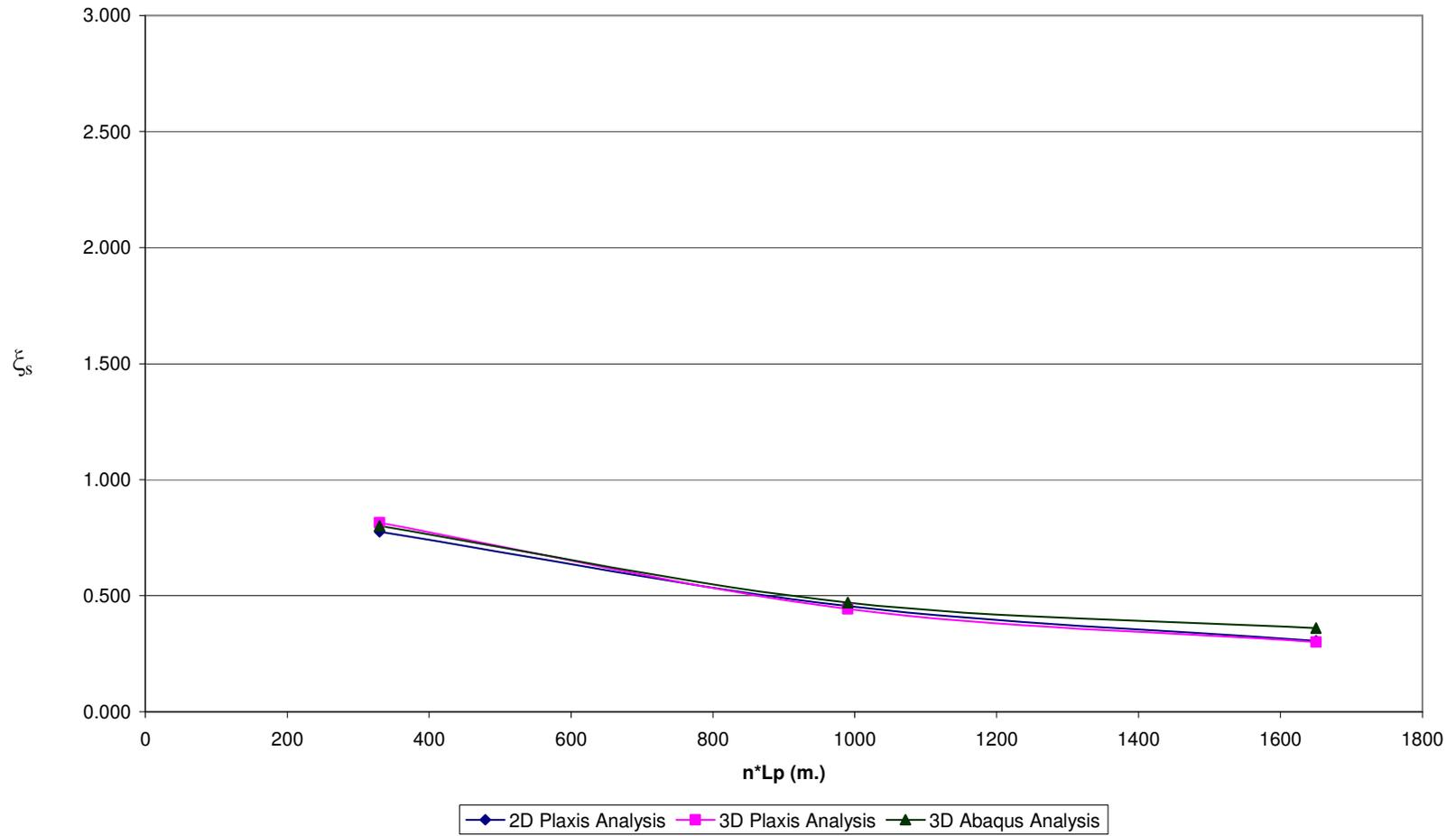
**Fig A.14  $\xi_s$  vs.  $n \cdot L_p$  for Pile Configuration – 3,  $n=33$  &  $V_{ult} / P_{eff} = 20$**
