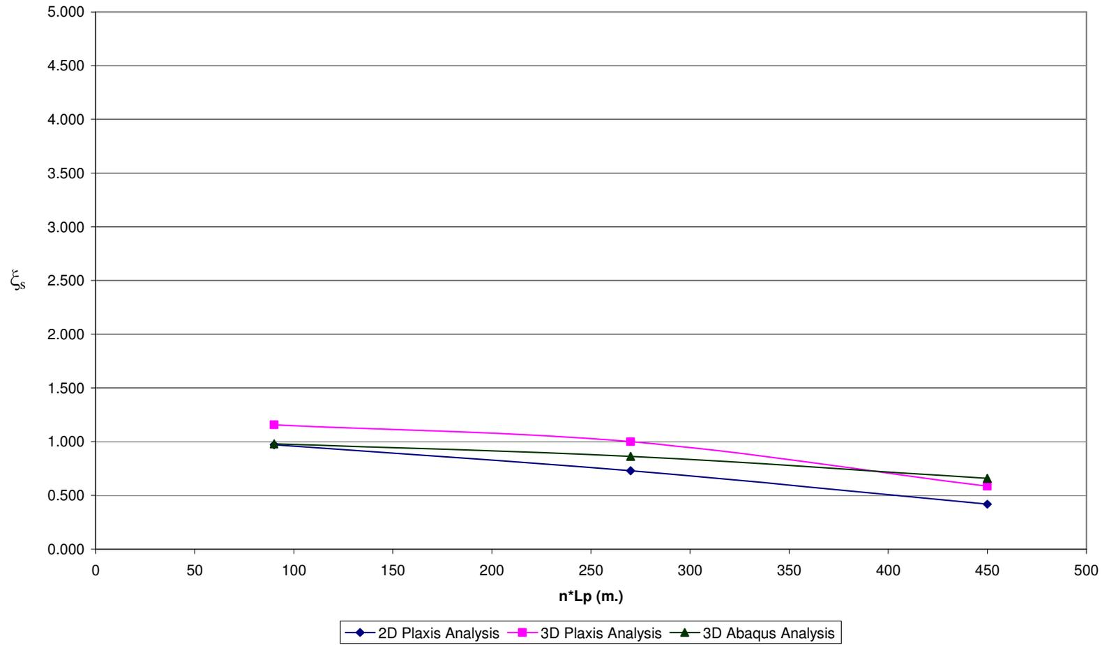
**Fig A.7  $\xi_s$  vs.  $n \cdot L_p$  for Pile Configuration – 2,  $n=9$  &  $V_{ult} / P_{eff} = 5$**
