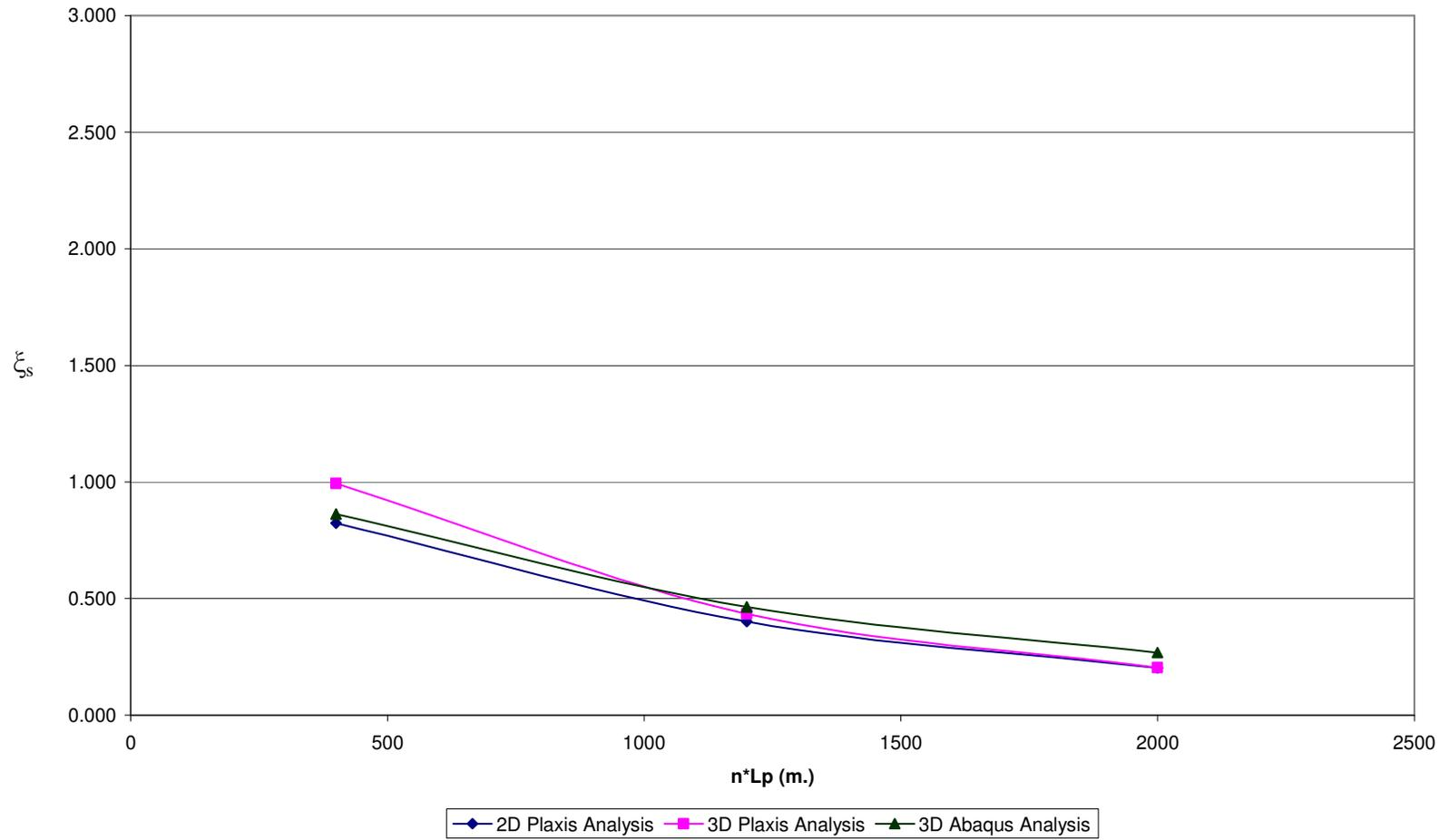
**Fig A.11  $\xi_s$  vs.  $n \cdot L_p$  for Pile Configuration – 3,  $n=40$  &  $V_{ult} / P_{eff} = 5$**
