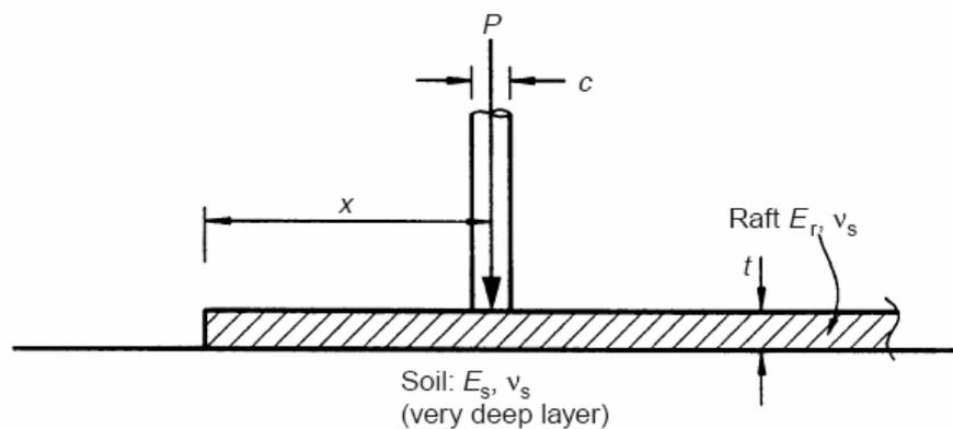
Fig 2.6 Definition of Problem for an Individual Column Load
