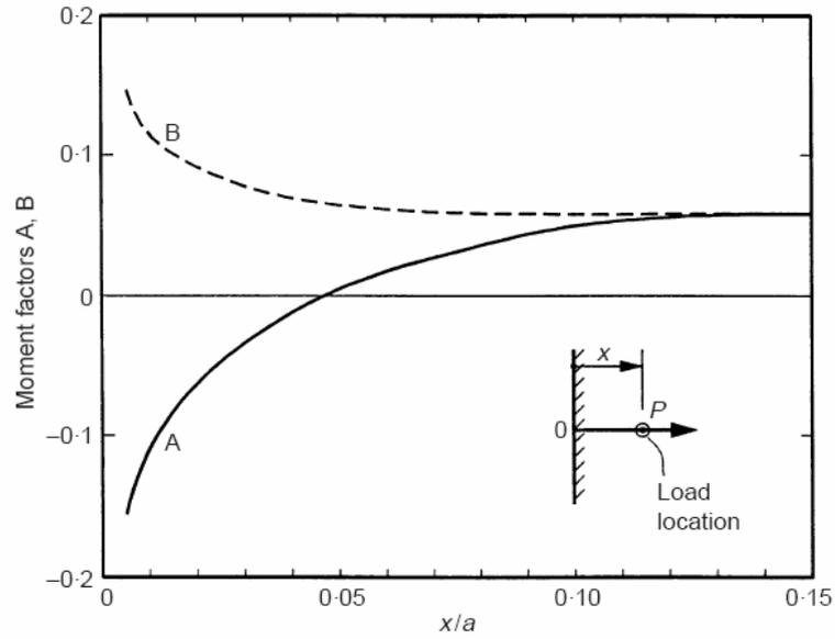
Fig 2.7 Moment Factors A, B for Circular Column
