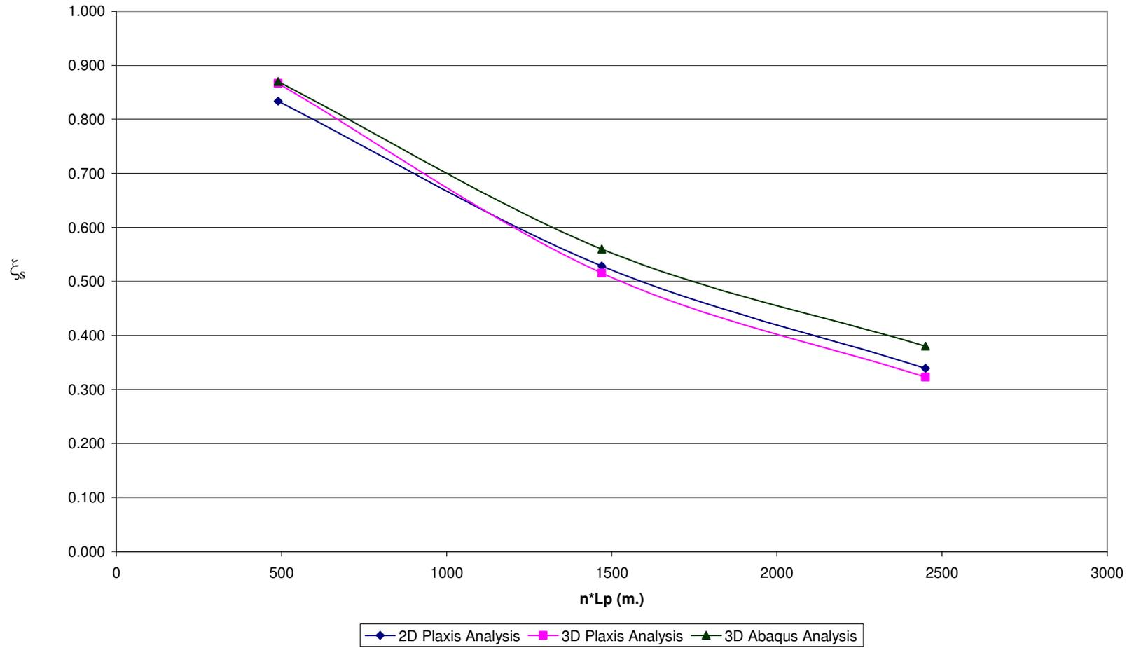
**Fig A.4  $\xi_s$  vs.  $n \cdot L_p$  for Pile Configuration – 2,  $n=49$  &  $V_{ult} / P_{eff} = 20$**
