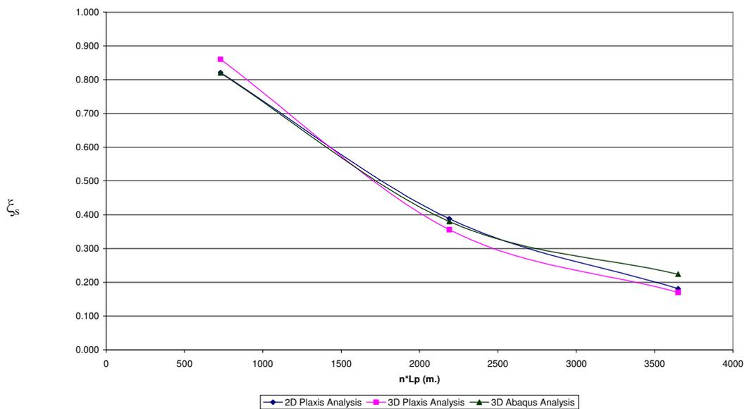
Fig 4.18  $\xi_s$  vs.  $n \cdot L_p$  for Pile Configuration – 3,  $n=73$  &  $V_{ult} / P_{eff} = 5$
