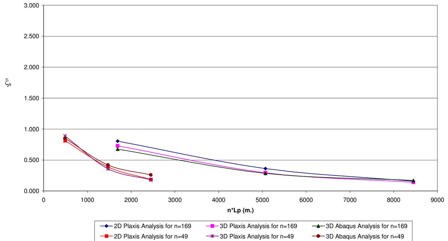
**Fig A.1  $\xi_s$  vs.  $n \cdot L_p$  for Pile Configuration – 1 &  $V_{ult} / P_{eff} = 5$**
