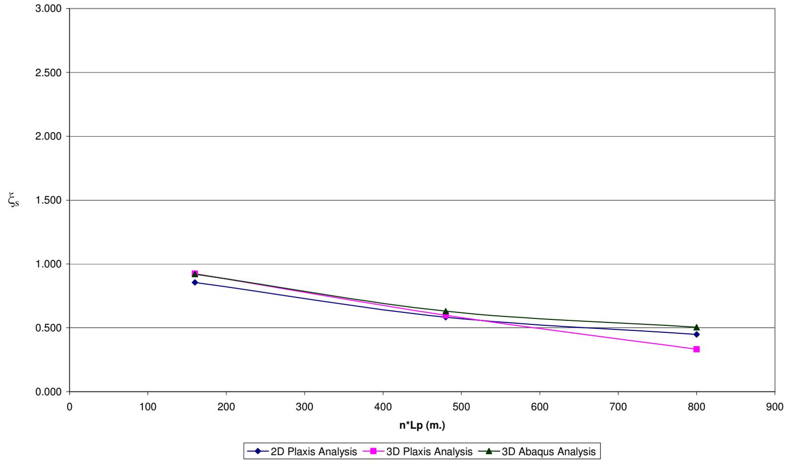
**Fig A.6  $\xi_s$  vs.  $n \cdot L_p$  for Pile Configuration – 2,  $n=16$  &  $V_{ult} / P_{eff} = 20$**
