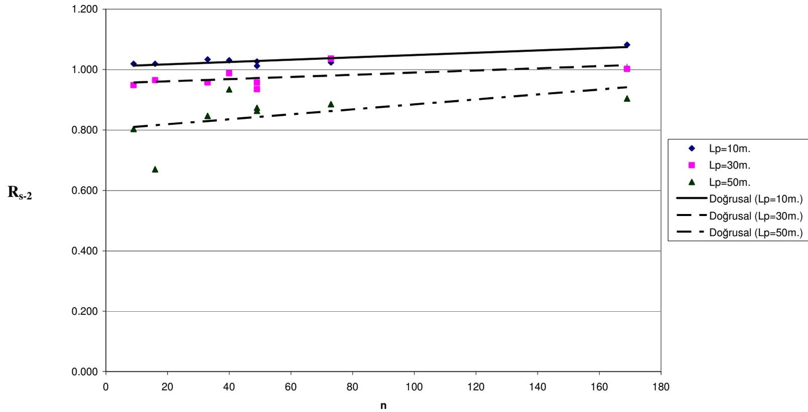
Fig B.4  $R_{s-2}$  for  $V_{ult}/P_{eff} = 20$
