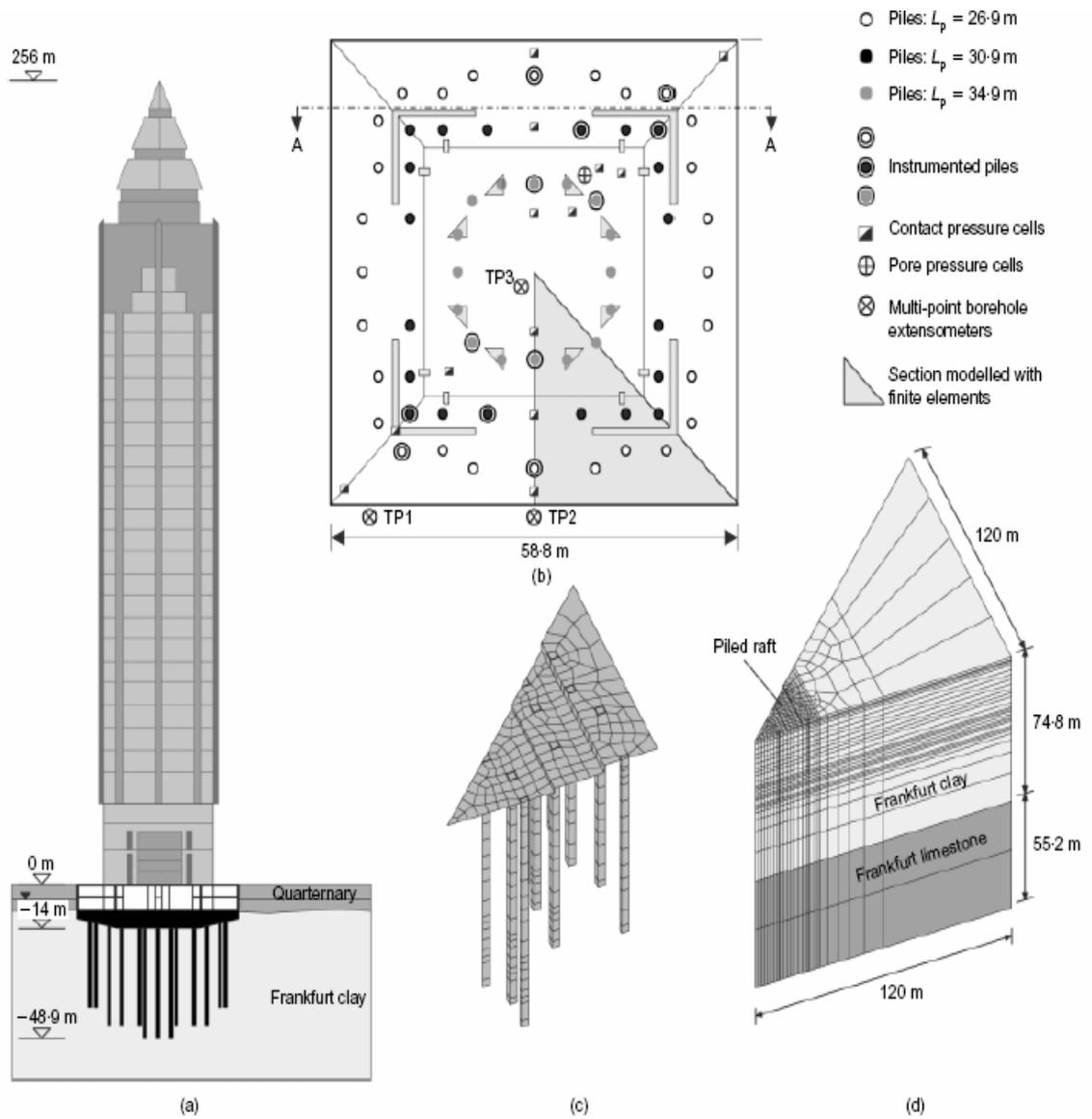
Fig 3.5 (a) General View, (b) Instrumentation Layout, (c) Finite Element Mesh of the Piled Raft, (d) Finite Element Mesh of the System
