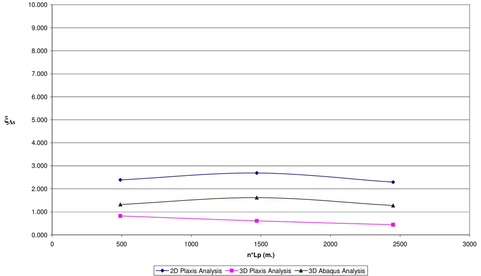
**Fig D.3  $\xi_{As}$  vs.  $n \cdot L_p$  for Pile Configuration – 1,  $n=49$  &  $V_{ult} / P_{eff} = 5$**
