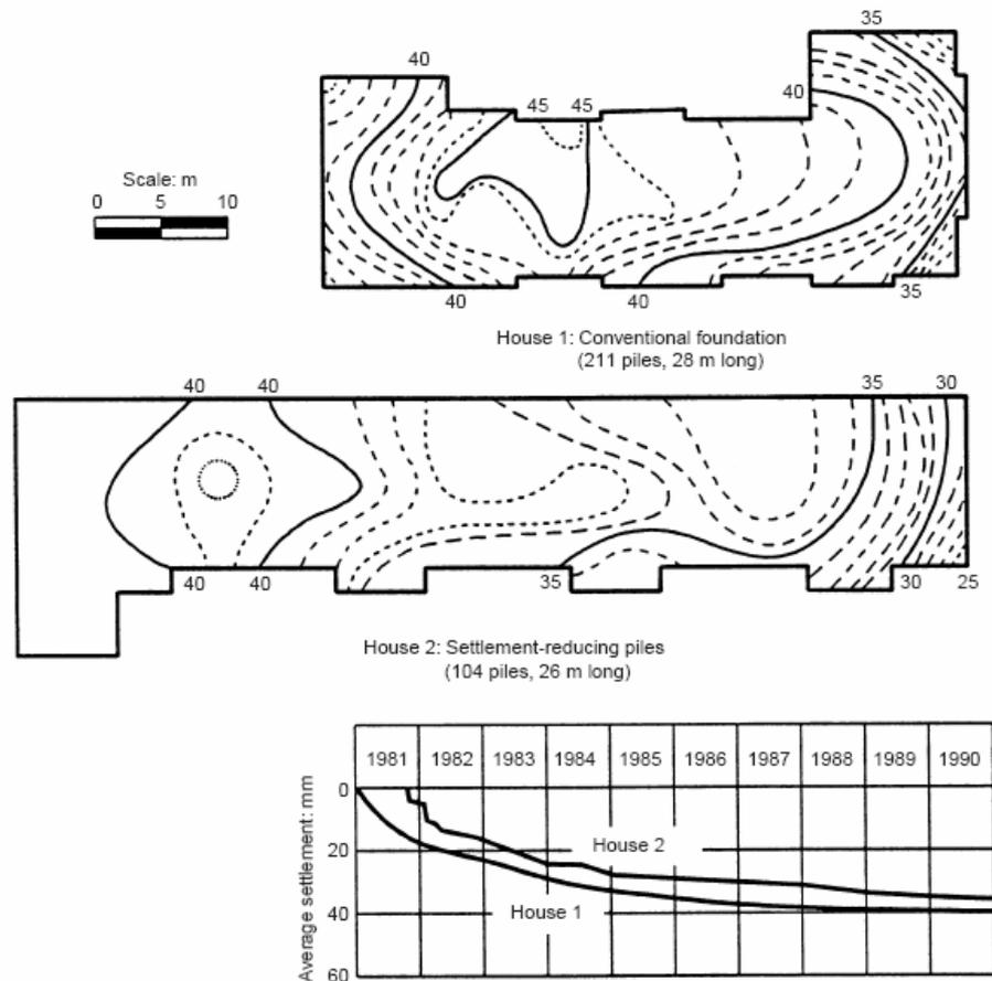
Fig 2.12 Settlement Performance of Two Buildings, one on conventional piles and one on creep piles
