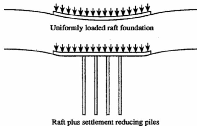
Fig 2.13 Central Piles to Reduce Differential Settlement
