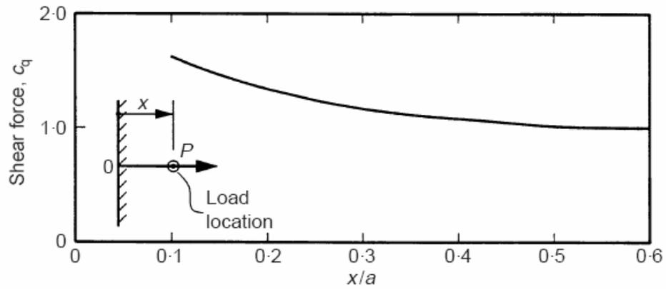
Fig 2.8 Shear Factor , $c_q$ , for Circular Column
