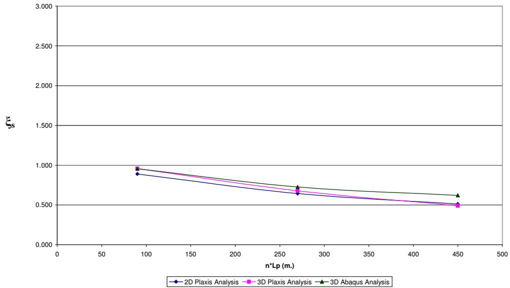
Fig 4.14  $\xi_s$  vs.  $n \cdot L_p$  for Pile Configuration – 2,  $n=9$  &  $V_{ult} / P_{eff} = 20$
