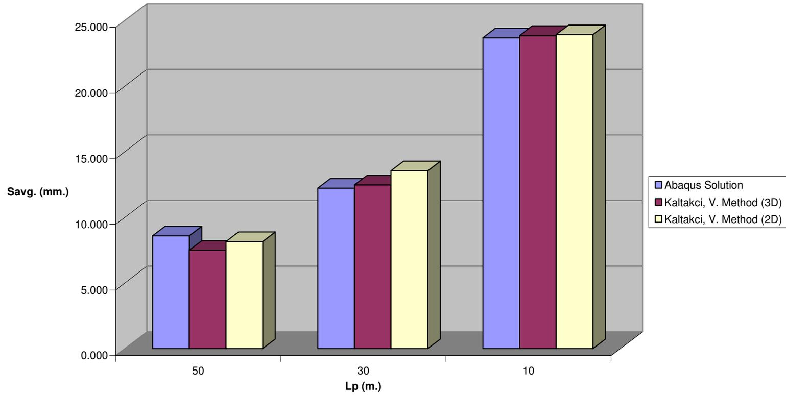
**Fig C.12  $S_{avg}$  vs.  $L_p$  for Pile Configuration -3 ,  $n=73$  &  $V_{ult} / P_{eff} = 20$**
