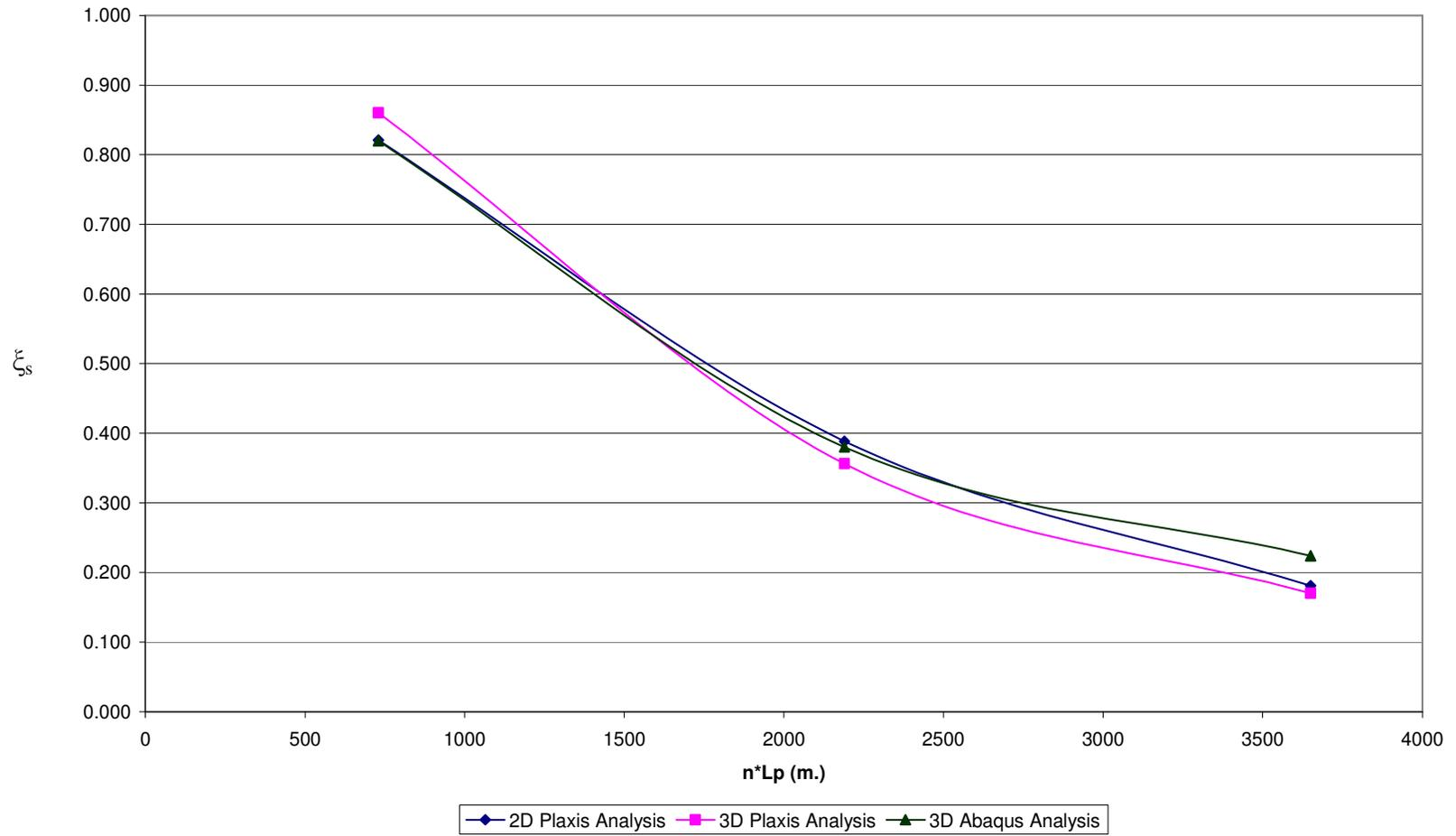
**Fig A.9  $\xi_s$  vs.  $n \cdot L_p$  for Pile Configuration – 3,  $n=73$  &  $V_{ult} / P_{eff} = 5$**
