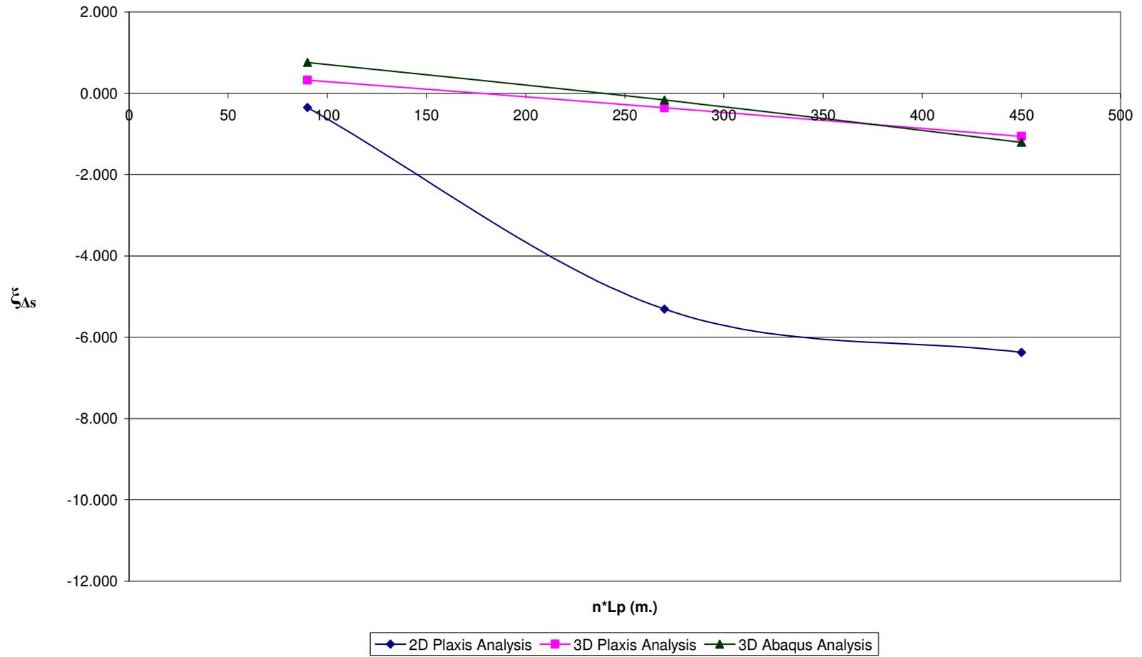
**Fig D.9**  $\xi_{As}$  vs.  $n \cdot L_p$  for Pile Configuration – 2,  $n=9$  &  $V_{ult} / P_{eff} = 5$
