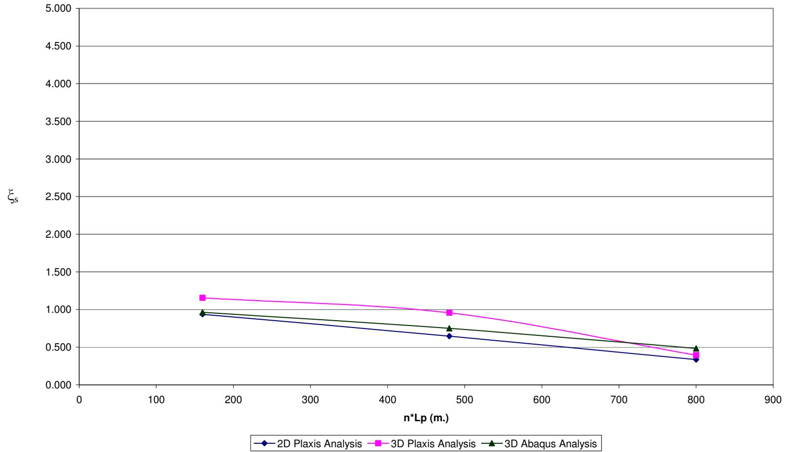
**Fig A.5  $\xi_s$  vs.  $n \cdot L_p$  for Pile Configuration – 2,  $n=16$  &  $V_{ult} / P_{eff} = 5$**
