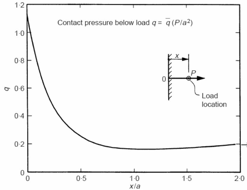
Fig 2.9 Contact Pressure Factor,  $q$
