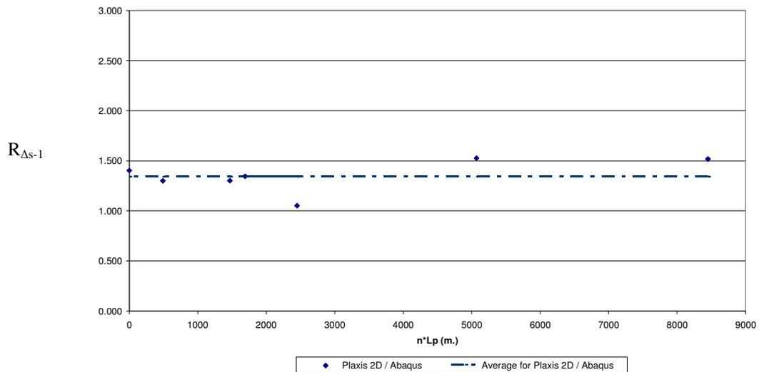
Fig 4.10  $R_{\Delta s-1}$  vs.  $n \cdot L_p$  for Pile Configuration – 1 &  $V_{ult} / P_{eff} = 20$
