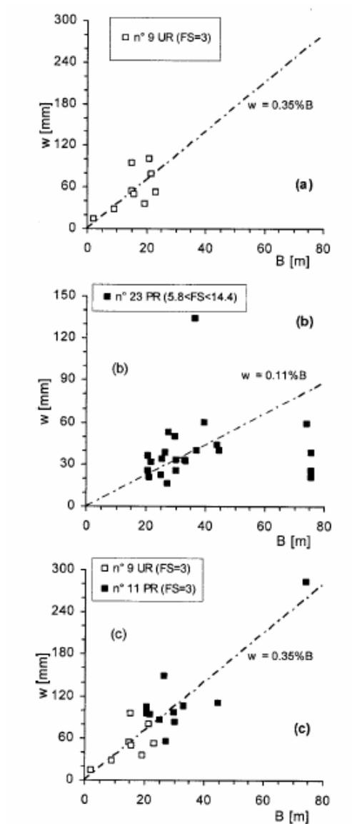
Fig 2.17 Settlement of foundation over stiff clays (a) unpiled raft, (b) piled rafts, (c) unpiled and piled rafts (Sanctis & Mandolini, 2006)
