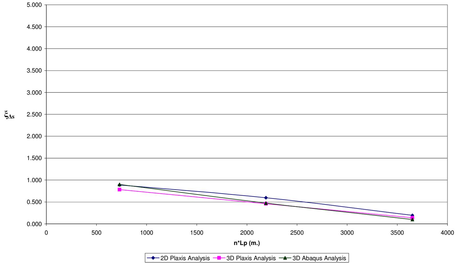
**Fig D.12  $\xi_{\Delta s}$  vs.  $n * L_p$  for Pile Configuration – 3,  $n=73$  &  $V_{ult} / P_{eff} = 20$**
