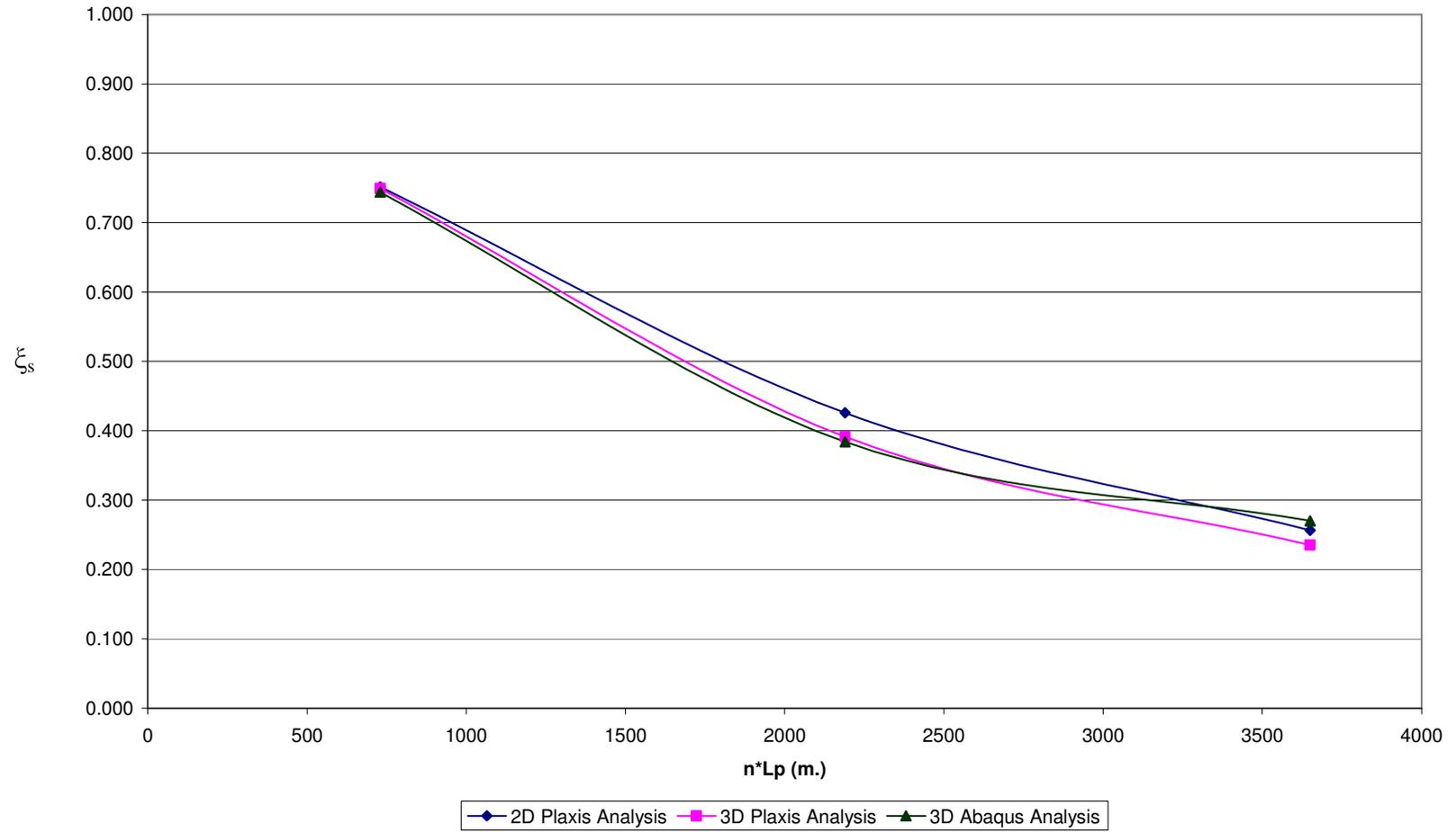
**Fig A.10  $\xi_s$  vs.  $n \cdot L_p$  for Pile Configuration – 3,  $n=73$  &  $V_{ult} / P_{eff} = 20$**
