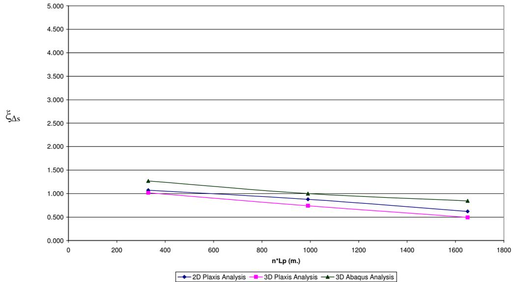
Fig 4.20  $\xi_{\Delta s}$  vs.  $n \cdot L_p$  for Pile Configuration – 3,  $n=33$  &  $V_{ult} / P_{eff} = 20$
