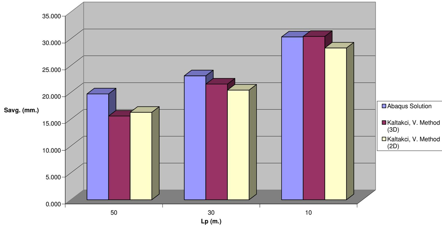
**Fig C.10  $S_{avg}$ . vs.  $L_p$  for Pile Configuration -2 ,  $n=9$  &  $V_{ult} / P_{eff} = 20$**
