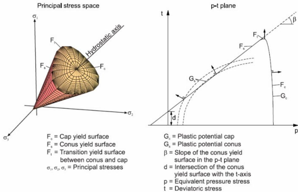
Fig 3.3 Cap Model : Yield Surfaces in Principal Stress Space and p – t plane
