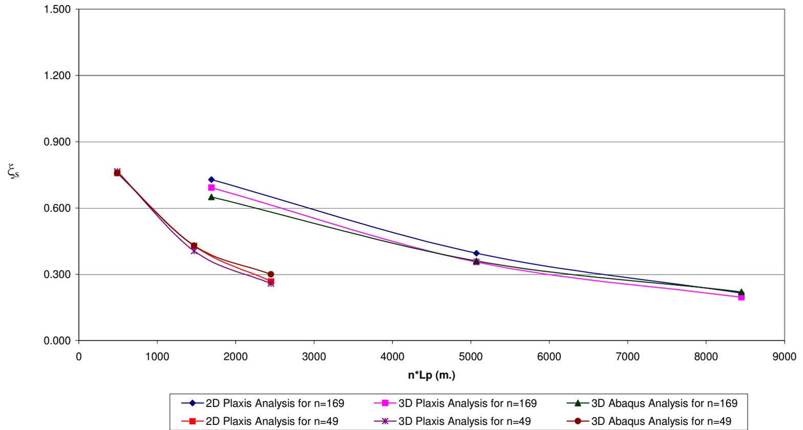
**Fig A.2  $\xi_s$  vs.  $n \cdot L_p$  for Pile Configuration - 1 &  $V_{ult} / P_{eff} = 20$**
