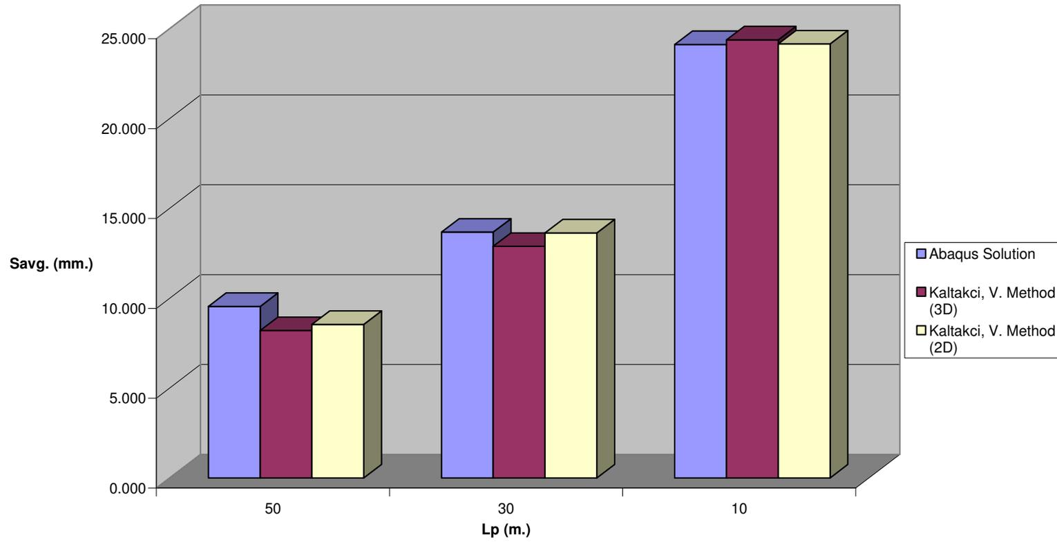
**Fig C.4  $S_{avg.}$  vs.  $L_p$  for Pile Configuration -1 ,  $n=49$  &  $V_{ult} / P_{eff} = 20$**
