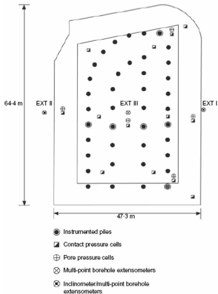
Fig 3.2 Instrumentation Layout of Westend 1
