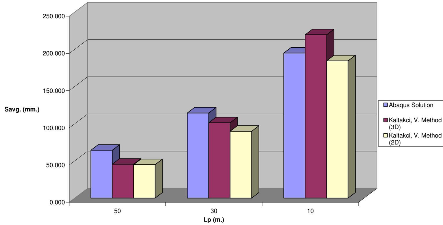
**Fig C.15  $S_{avg}$ . vs.  $L_p$  for Pile Configuration -3 ,  $n=33$  &  $V_{ult} / P_{eff} = 5$**
