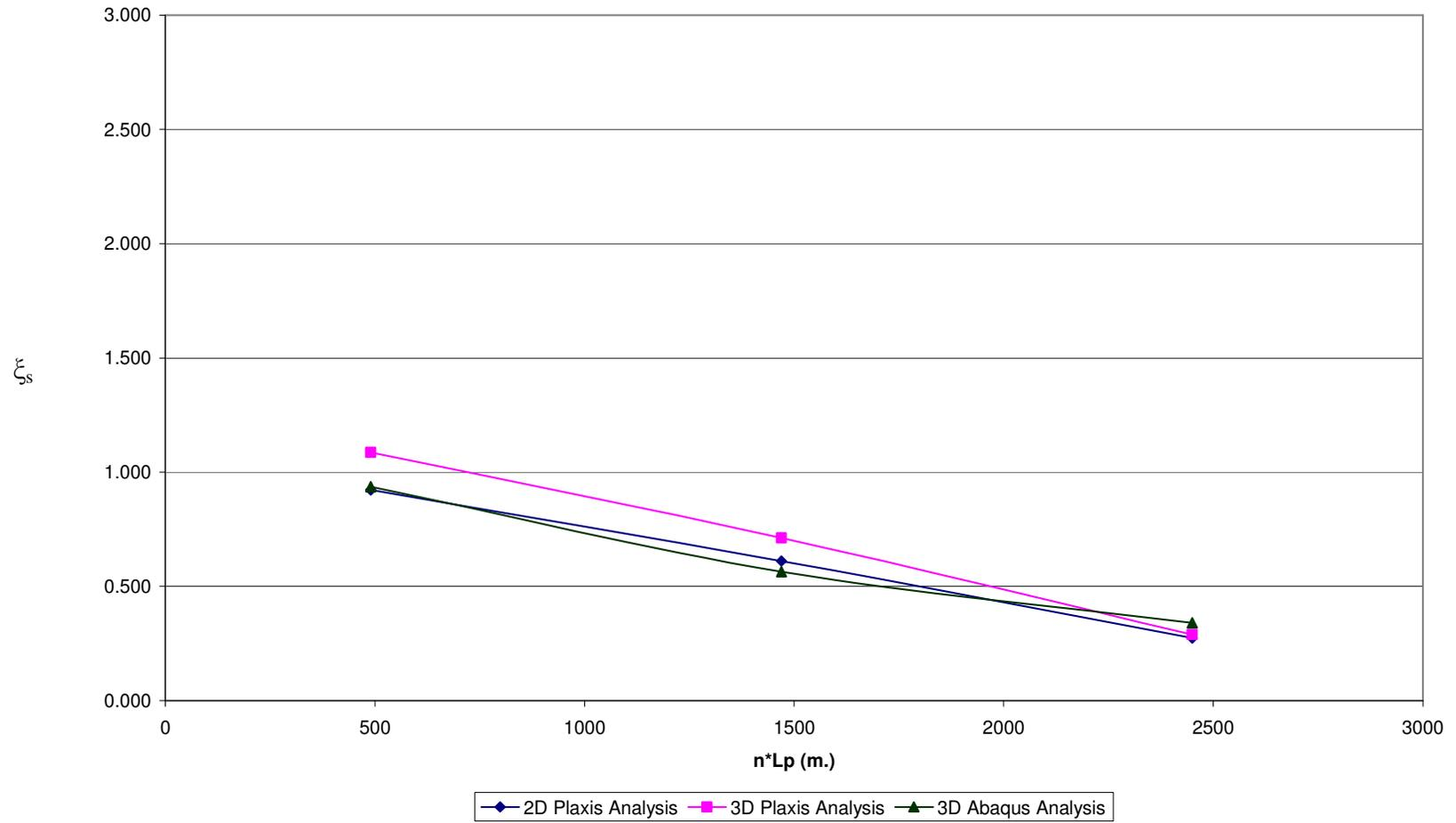
**Fig A.3  $\xi_s$  vs.  $n \cdot L_p$  for Pile Configuration – 2,  $n=49$  &  $V_{ult} / P_{eff} = 5$**
