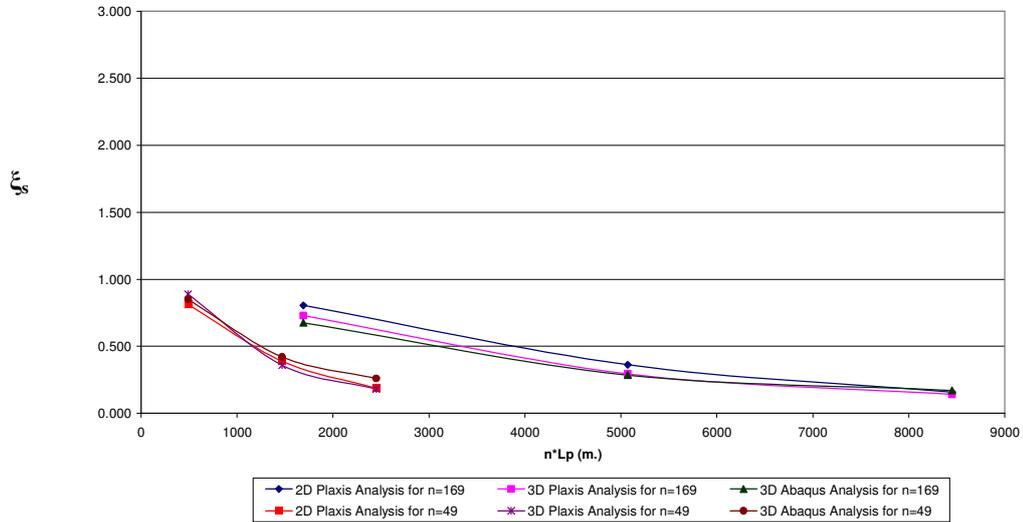
Fig 4.7  $\xi_s$  vs.  $n \cdot L_p$  for Pile Configuration – 1 &  $V_{ult} / P_{eff} = 5$
