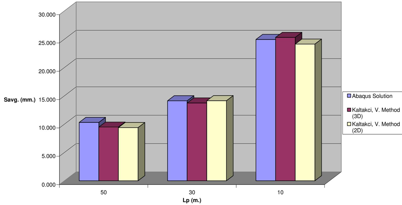
**Fig C.14  $S_{avg}$ . vs.  $L_p$  for Pile Configuration -3 ,  $n=40$  &  $V_{ult} / P_{eff} = 20$**
