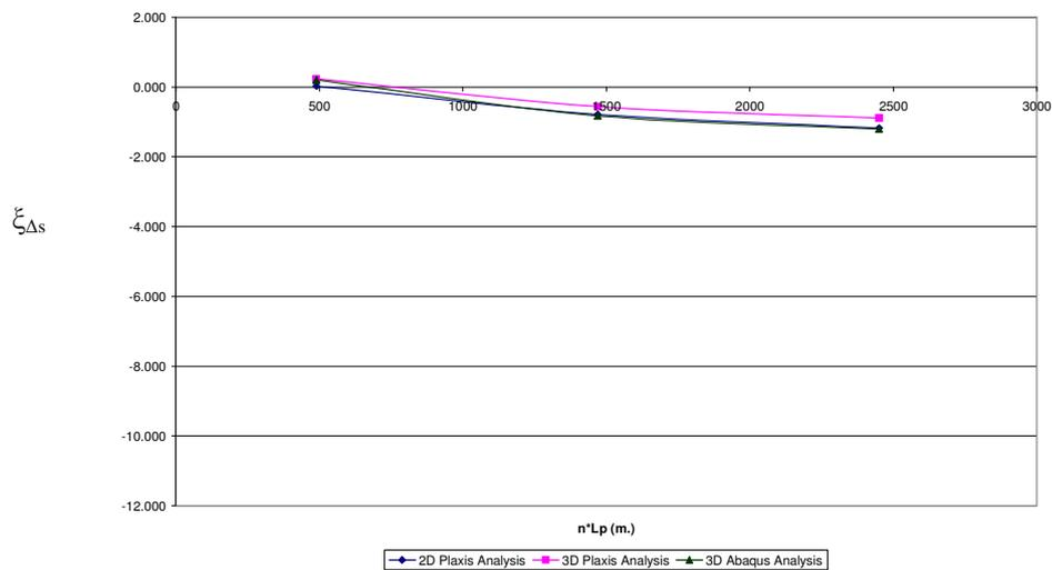
Fig 4.17  $\xi_{\Delta s}$  vs.  $n \cdot L_p$  for Pile Configuration – 2,  $n=49$  &  $V_{ult} / P_{eff} = 20$
