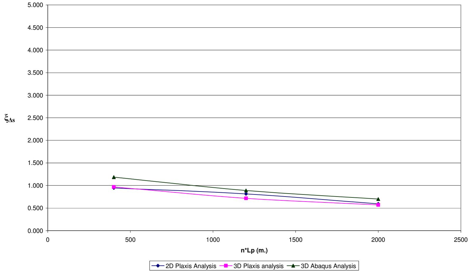
**Fig D.14  $\xi_{\Delta s}$  vs.  $n \cdot L_p$  for Pile Configuration – 3,  $n=40$  &  $V_{ult} / P_{eff} = 20$**
