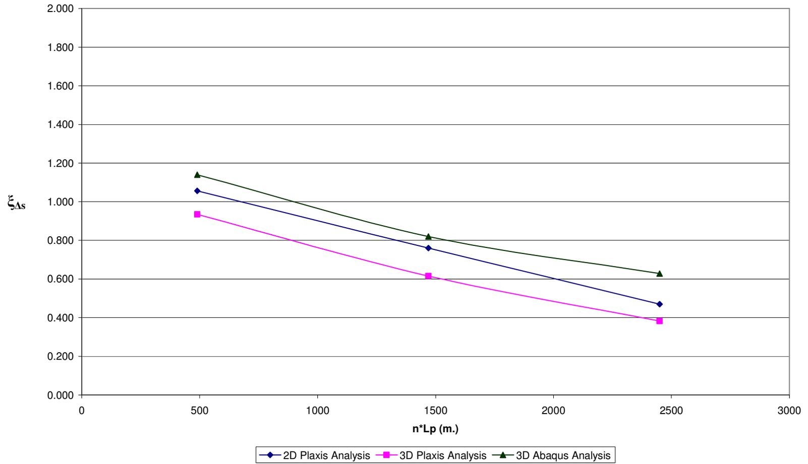
**Fig D.4  $\xi_{As}$  vs.  $n \cdot L_p$  for Pile Configuration – 1,  $n=49$  &  $V_{ult} / P_{eff} = 20$**
