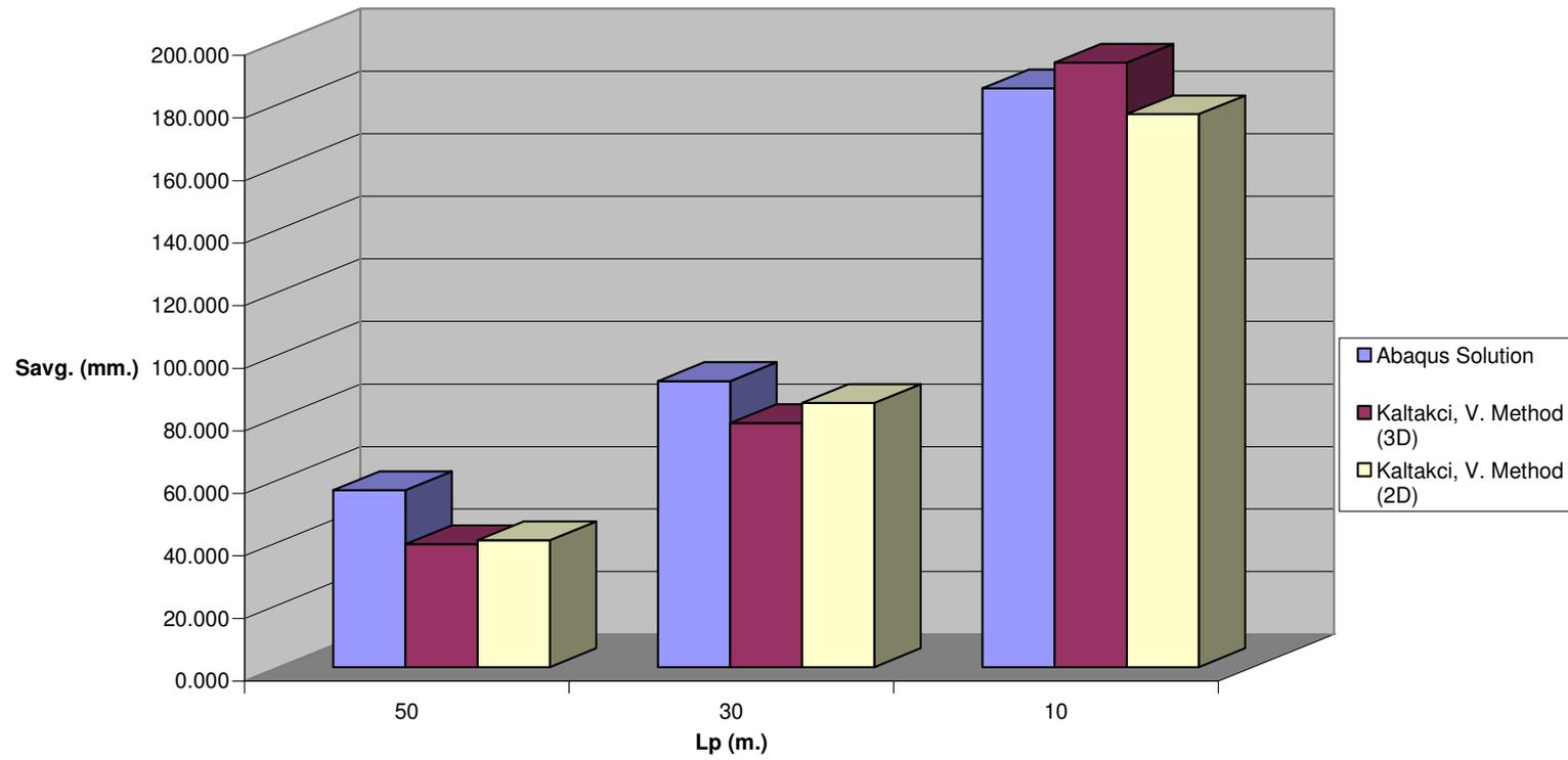
**Fig C.3  $S_{avg.}$  vs.  $L_p$  for Pile Configuration -1 ,  $n=49$  &  $V_{ult} / P_{eff} = 5$**
