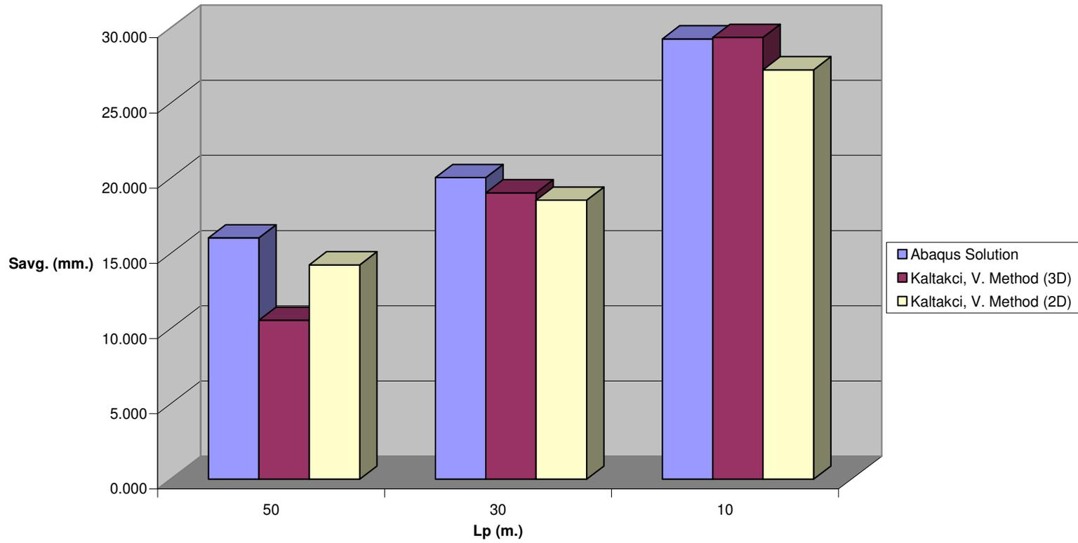
**Fig C.8  $S_{avg}$ . vs.  $L_p$  for Pile Configuration -2 ,  $n=16$  &  $V_{ult} / P_{eff} = 20$**
