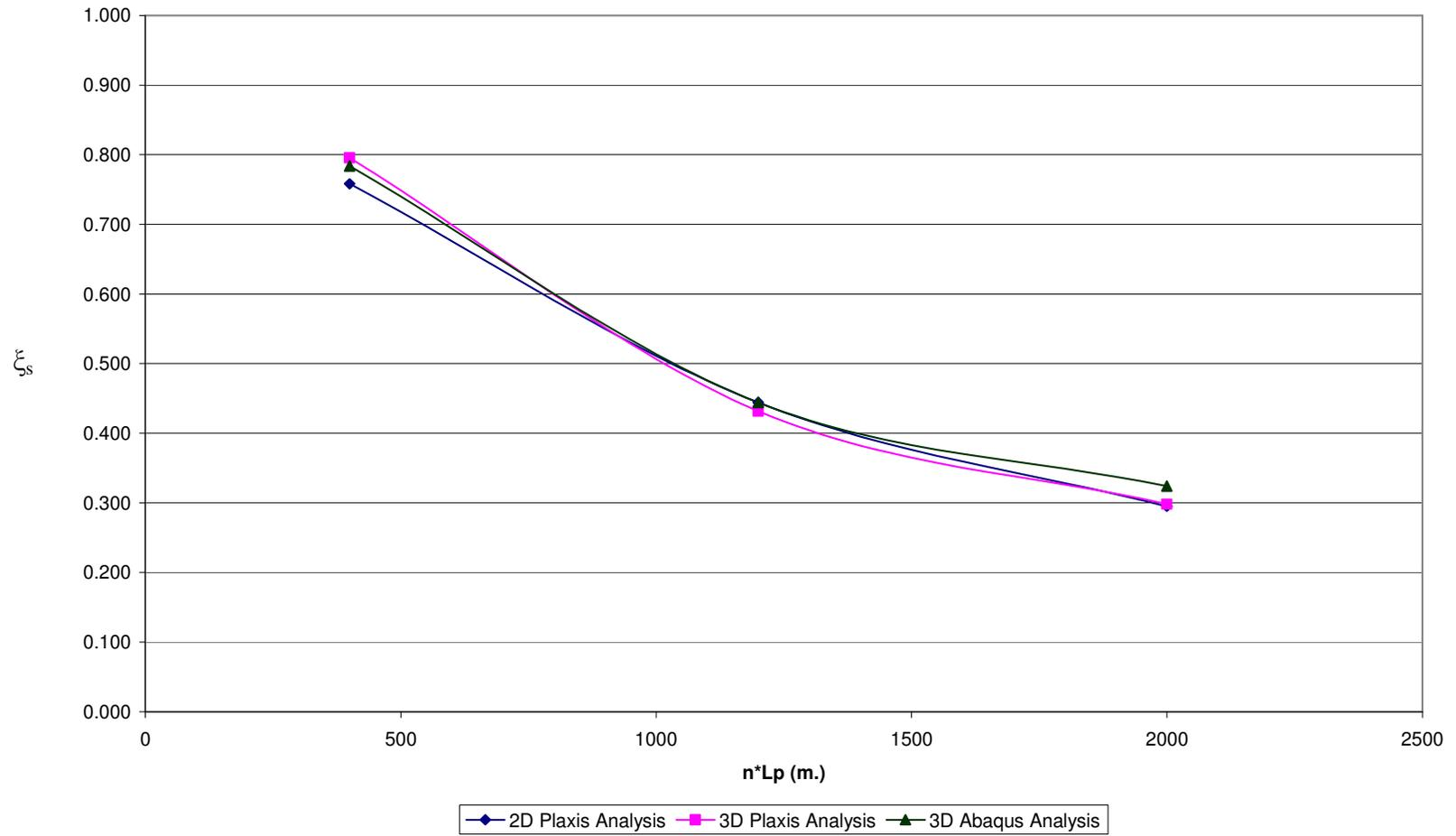
**Fig A.12  $\xi_s$  vs.  $n \cdot L_p$  for Pile Configuration – 3,  $n=40$  &  $V_{ult} / P_{eff} = 20$**
