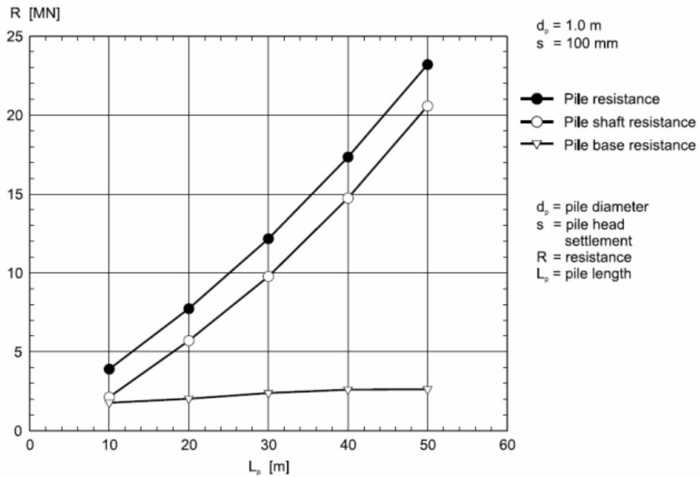
Fig 4.5 Variation of the Ultimate Pile Resistance of a Single Pile with the Pile Length (Reul, 2001)
