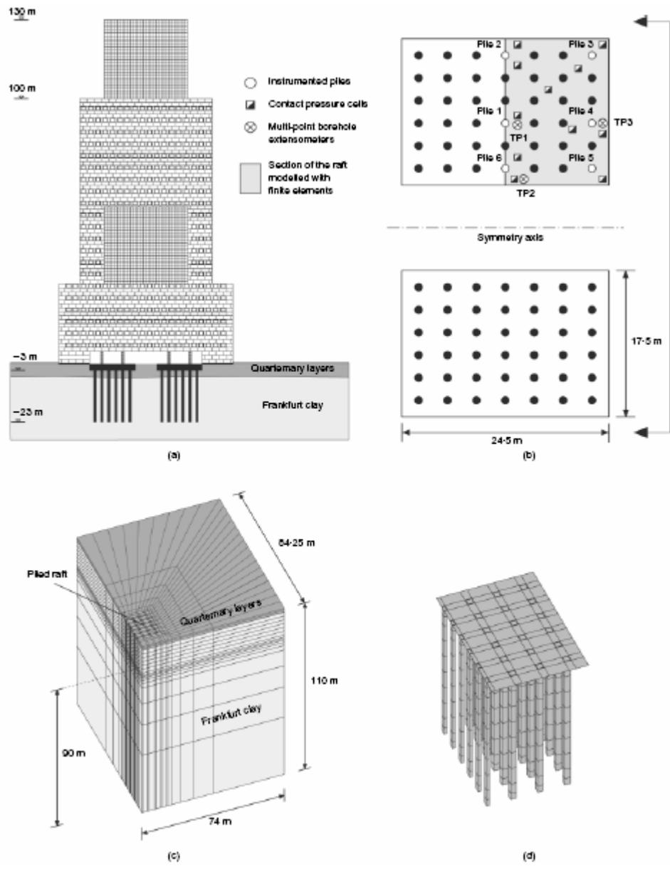
Fig 3.6 (a) Profile View of the Building, (b) Ground Plan of Raft, (c) Finite Element Mesh of System, (d) Finite element mesh of Piled Raft
