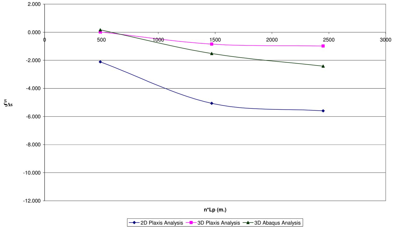
**Fig D.5  $\xi_{\Delta s}$  vs.  $n \cdot L_p$  for Pile Configuration – 2,  $n=49$  &  $V_{ult} / P_{eff} = 5$**
