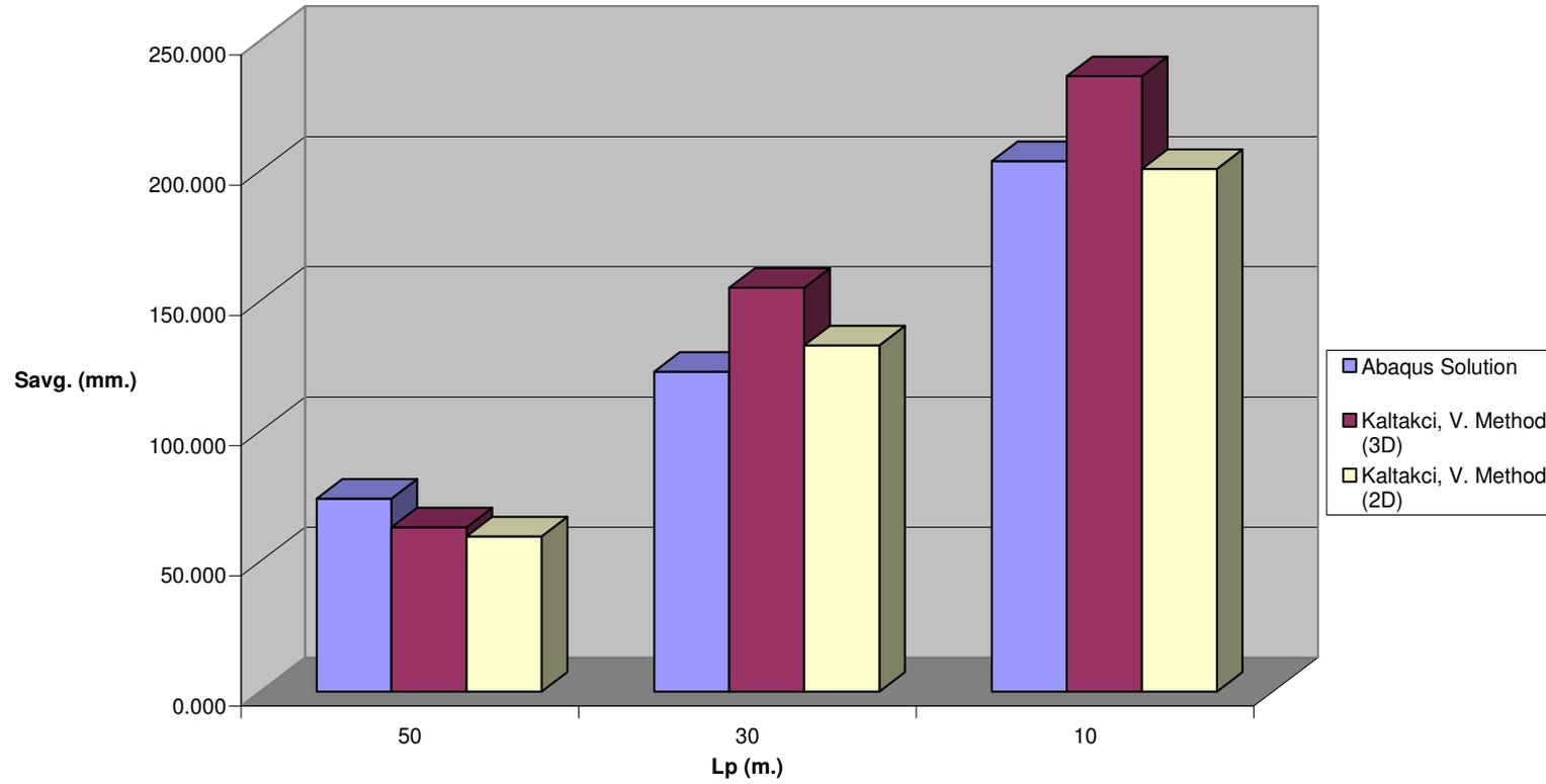
**Fig C.5  $S_{avg}$ . vs.  $L_p$  for Pile Configuration -2 ,  $n=49$  &  $V_{ult} / P_{eff} = 5$**
