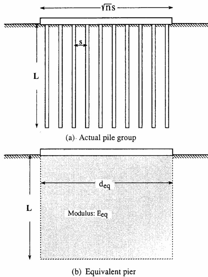
Fig 2.3 Replacement of Pile Group , or Piled Raft, by Equivalent Pier
