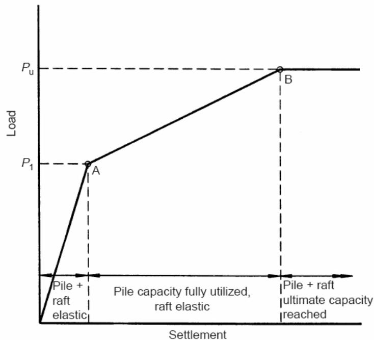
Fig 2.5 Simplified Load – Settlement Ccurve for Preliminary Analysis
