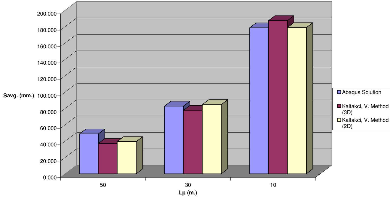
**Fig C.11  $S_{avg}$ . vs.  $L_p$  for Pile Configuration -3 ,  $n=73$  &  $V_{ult} / P_{eff} = 5$**
