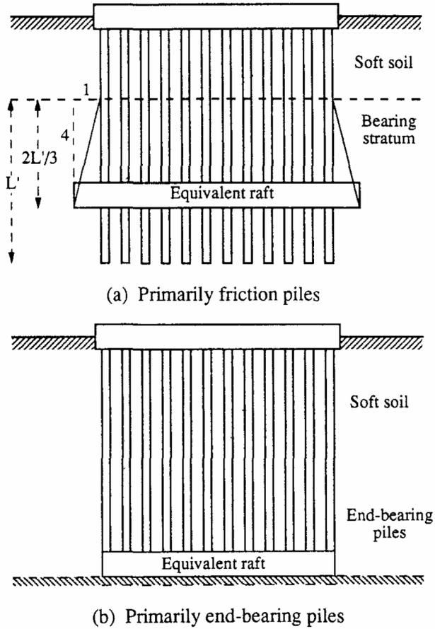
Fig 2.2 Equivalent Raft Approach for Pile Groups
