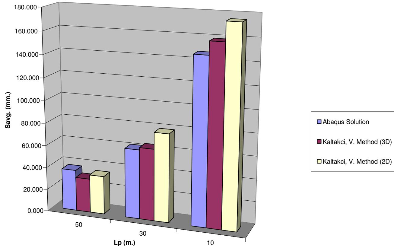
**Fig C.1  $S_{avg.}$  vs.  $L_p$  for Pile Configuration -1 ,  $n=169$  &  $V_{ult} / P_{eff} = 5$**
