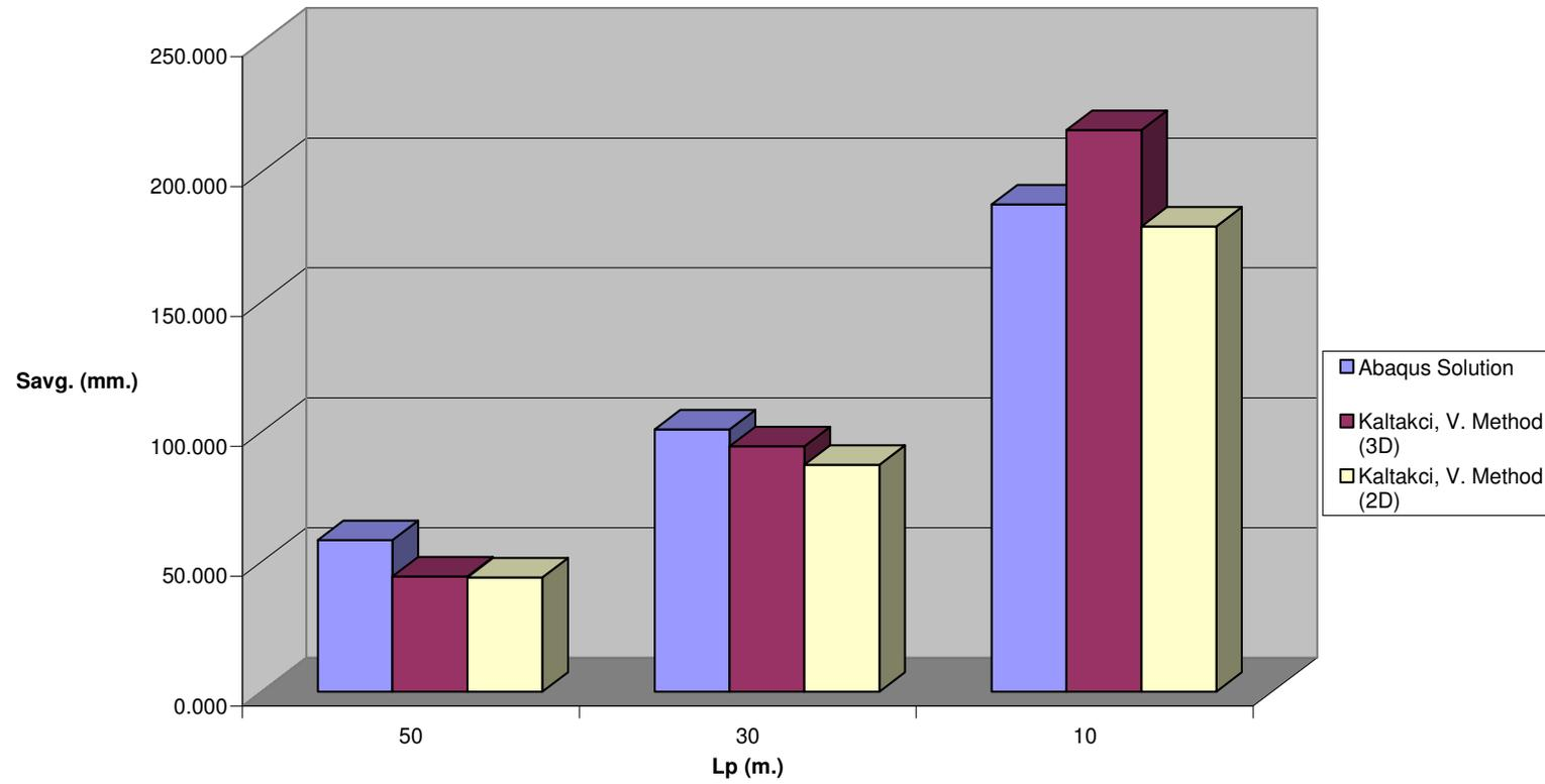
**Fig C.13  $S_{avg}$ . vs.  $L_p$  for Pile Configuration -3 ,  $n=40$  &  $V_{ult} / P_{eff} = 5$**
