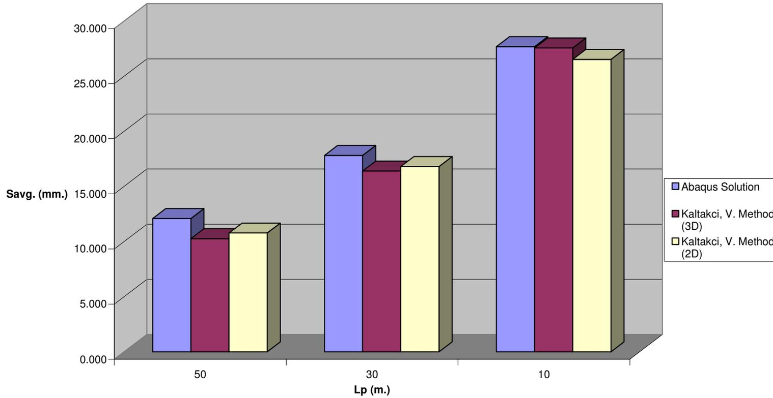
**Fig C.6  $S_{avg}$ . vs.  $L_p$  for Pile Configuration -2 ,  $n=49$  &  $V_{ult} / P_{eff} = 20$**
