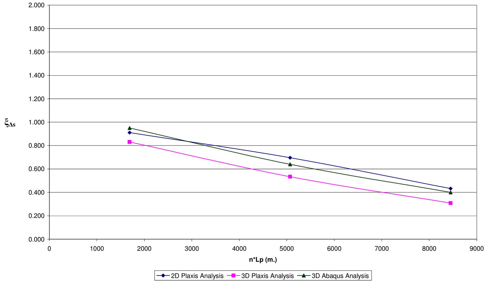
**Fig D.2  $\xi_{As}$  vs.  $n \cdot L_p$  for Pile Configuration – 1,  $n=169$  &  $V_{ult}/P_{eff} = 20$**
