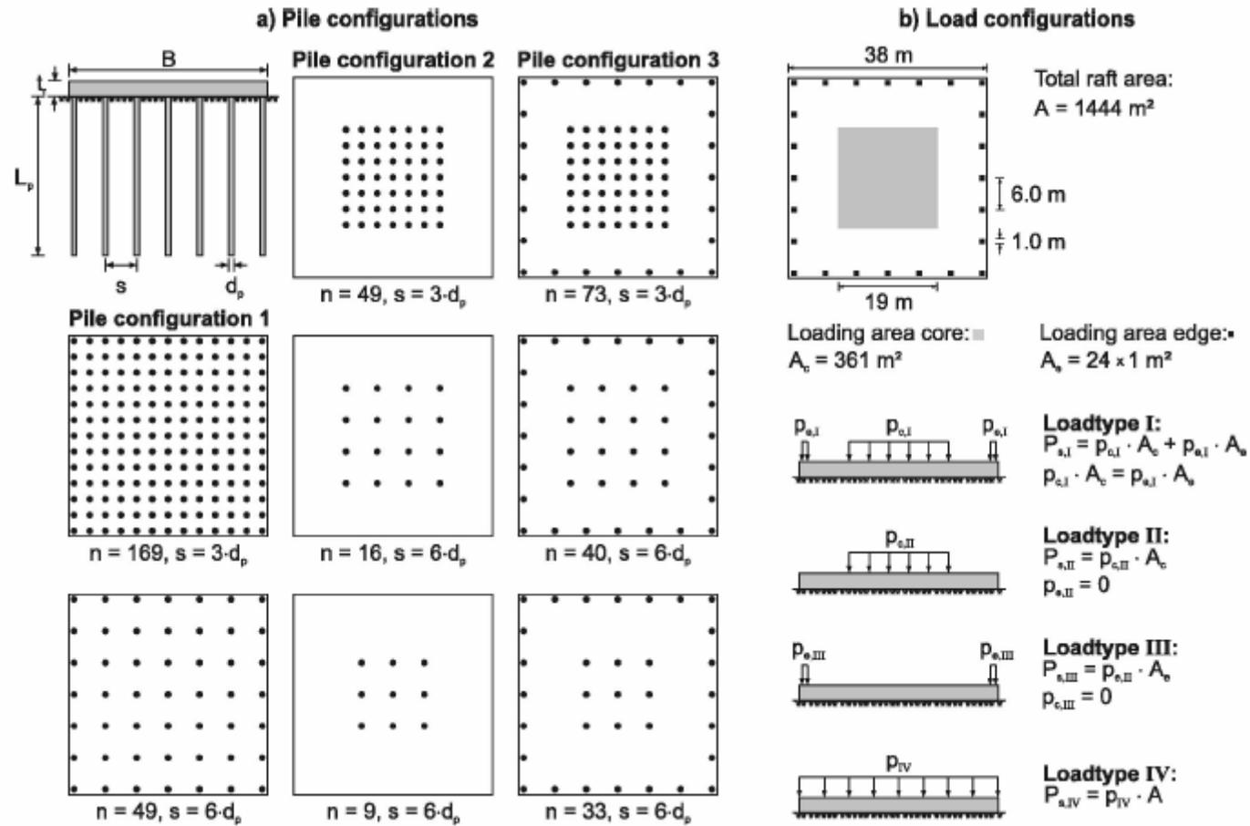
Fig 3.9 System Configurations and Load Configurations for Parametric Study
