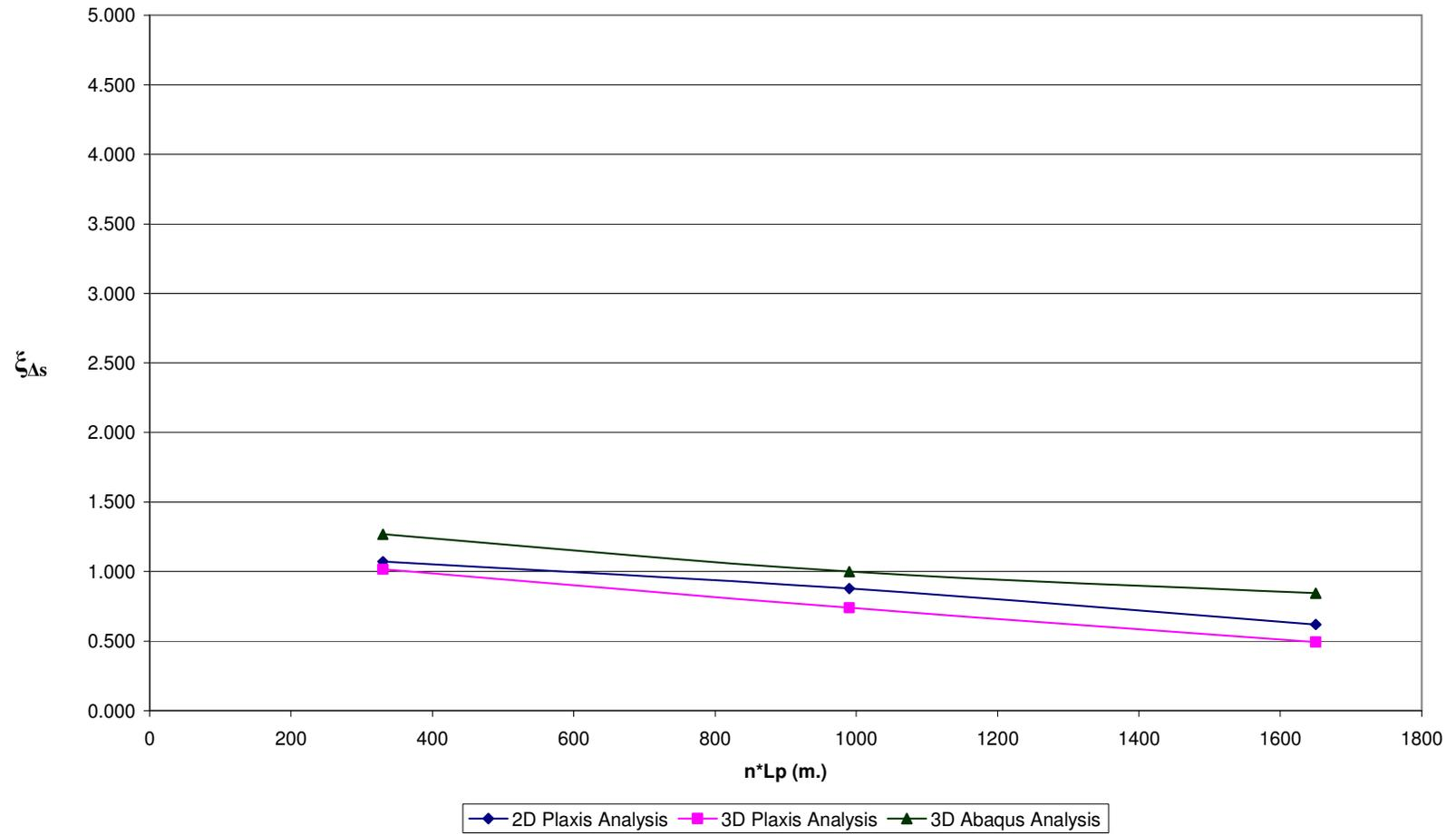
**Fig D.16  $\xi_{\Delta s}$  vs.  $n \cdot L_p$  for Pile Configuration - 3,  $n=33$ ,  $V_{ult}/P_{eff} = 20$**
