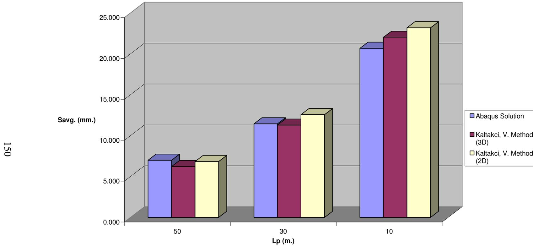
**Fig C.2 S<sub>avg.</sub> vs. L<sub>p</sub> for Pile Configuration -1 , n=169 & V<sub>ult</sub> / P<sub>eff</sub> = 20**
