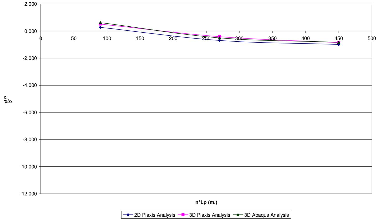
**Fig D.10  $\xi_{\Delta s}$  vs.  $n \cdot L_p$  for Pile Configuration – 2,  $n=9$  &  $V_{ult} / P_{eff} = 20$**
