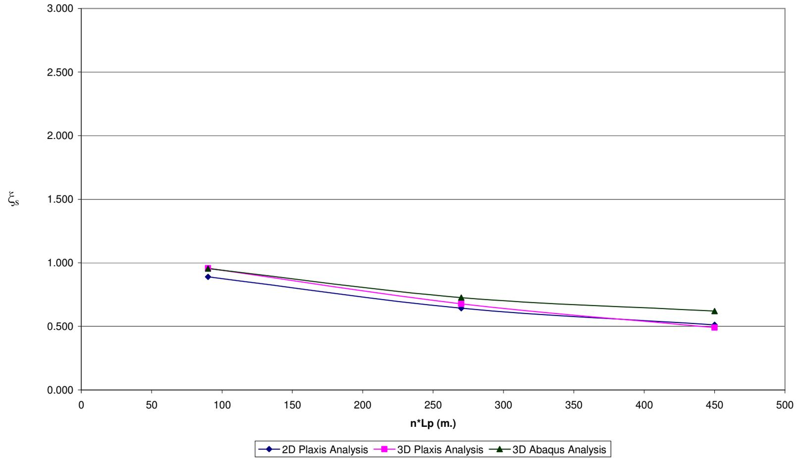
**Fig A.8  $\xi_s$  vs.  $n \cdot L_p$  for Pile Configuration – 2,  $n=9$  &  $V_{ult} / P_{eff} = 20$**
