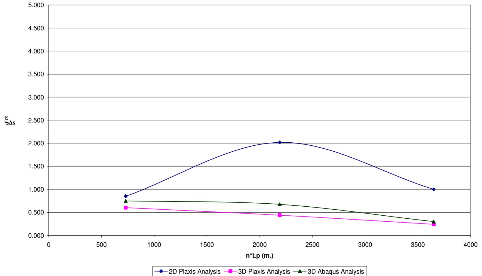
**Fig D.11  $\xi_{\Delta s}$  vs.  $n \cdot L_p$  for Pile Configuration – 3,  $n=73$  &  $V_{ult} / P_{eff} = 5$**
