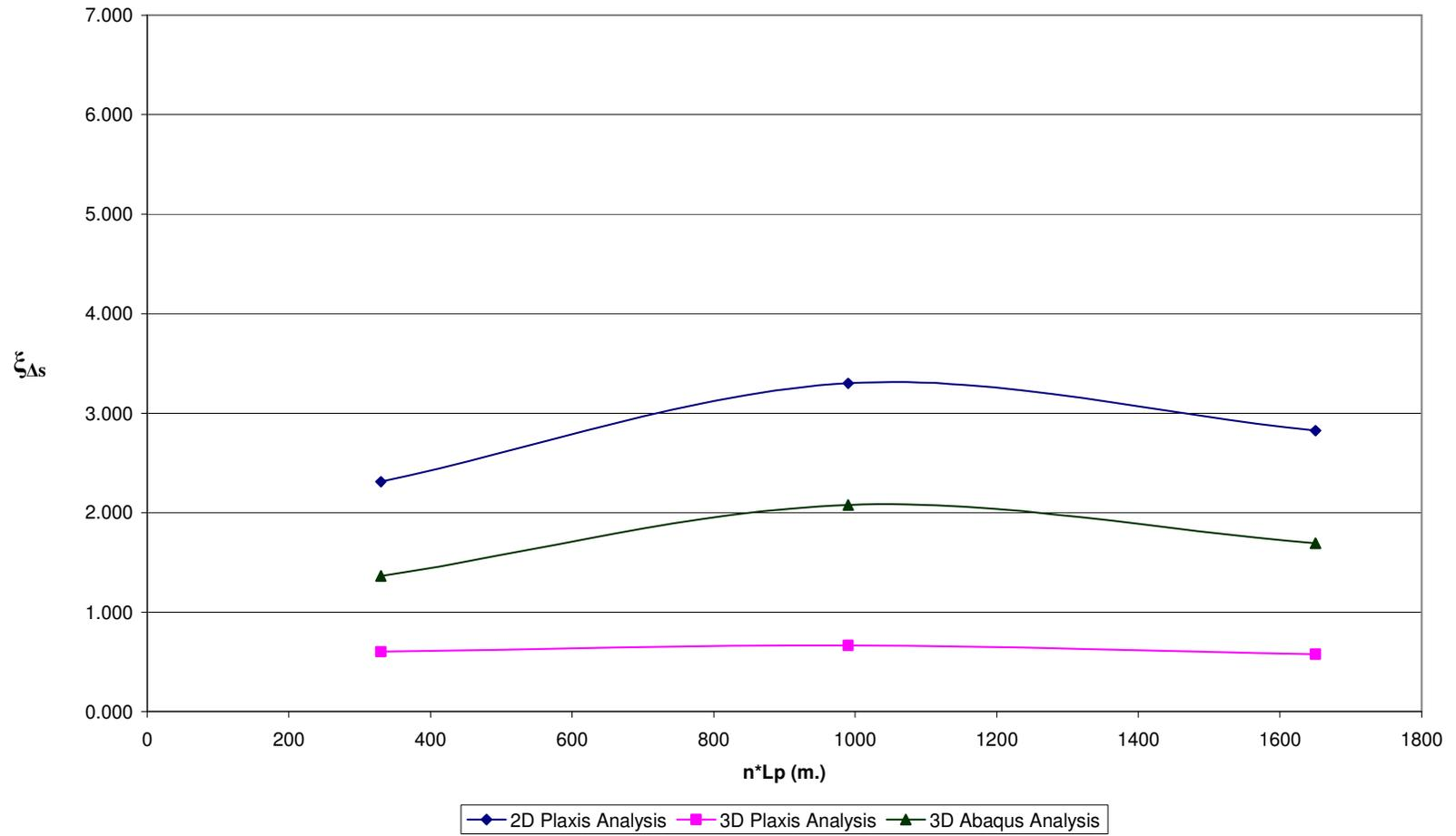
**Fig D.15  $\xi_{\Delta s}$  vs.  $n \cdot L_p$  for Pile Configuration – 3,  $n=33$  &  $V_{ult} / P_{eff} = 5$**
