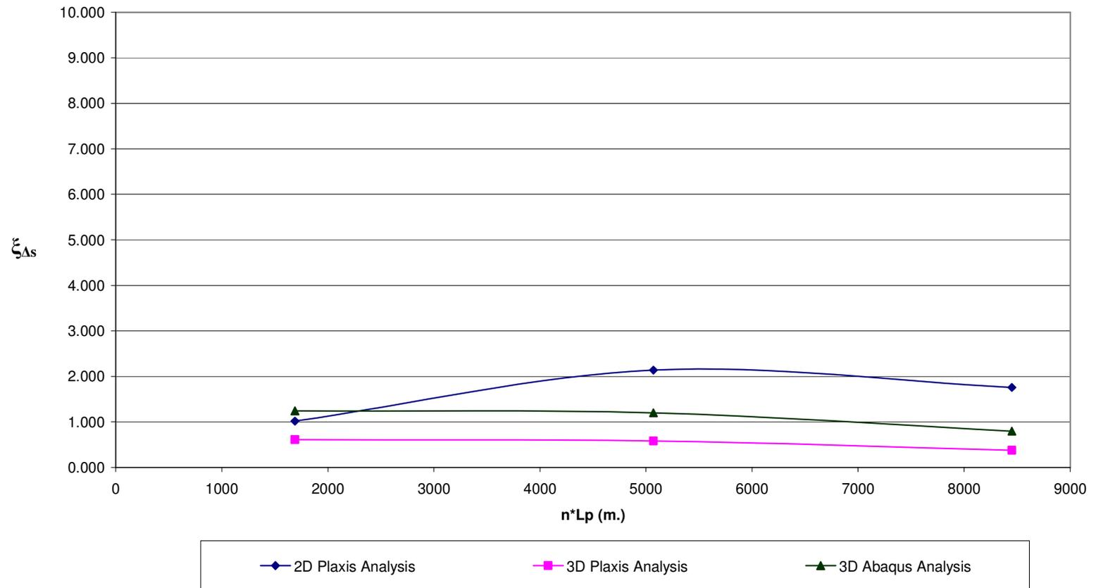
**Fig D.1  $\xi_{As}$  vs.  $n \cdot L_p$  for Pile Configuration – 1,  $n=169$  &  $V_{ult}/P_{eff} = 5$**
