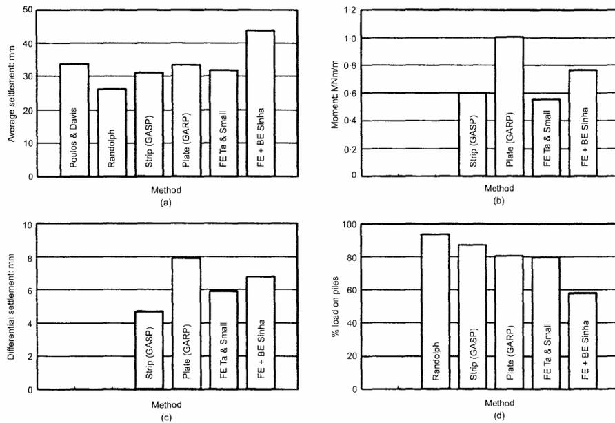
Fig 2.11 Comparative Results for Hypothetical Example ( raft with 9 piles, total load=12 MN)
