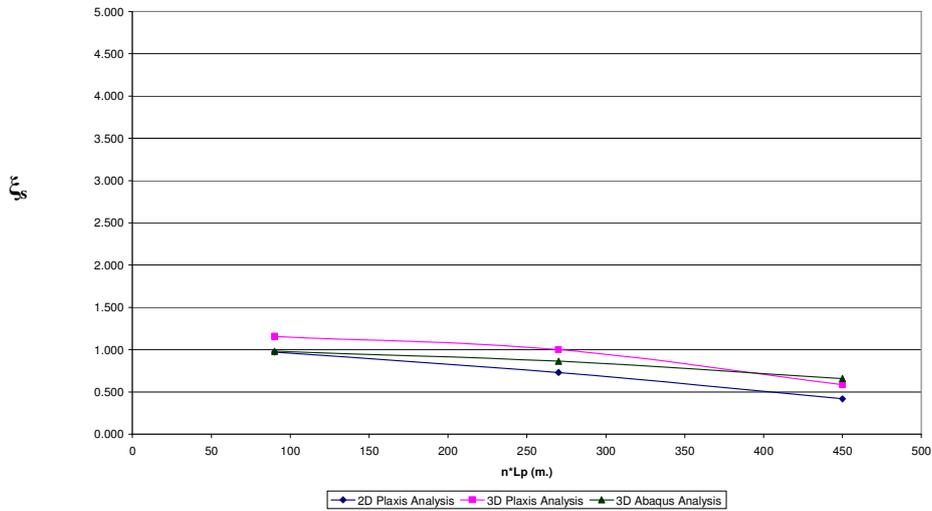
Fig 4.13  $\xi_s$  vs.  $n \cdot L_p$  for Pile Configuration – 2,  $n=9$  &  $V_{ult} / P_{eff} = 5$
