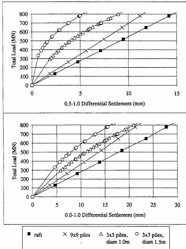
Fig 2.15 Development of Differential Settlements with Load Level
