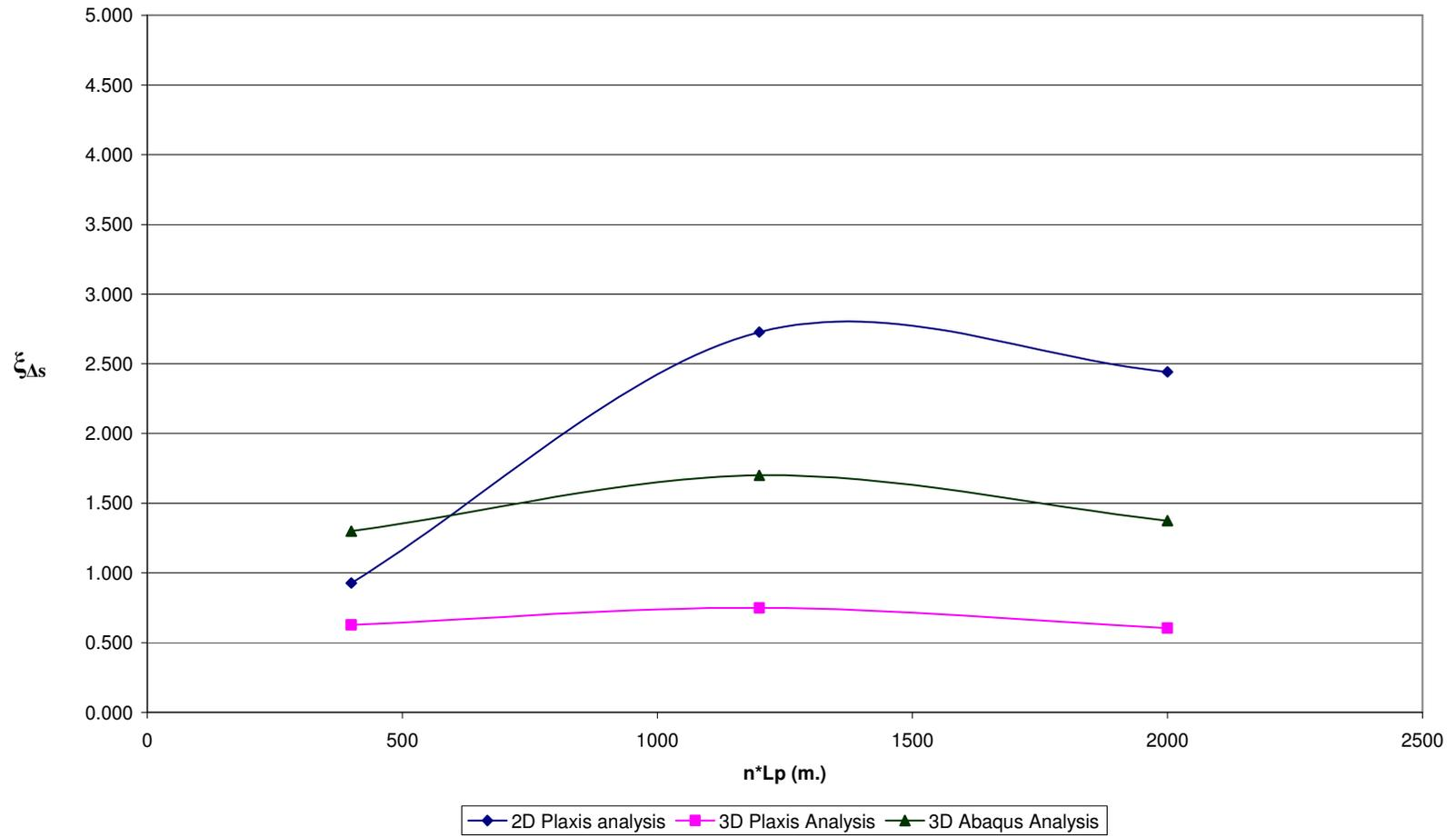
**Fig D.13  $\xi_{As}$  vs.  $n \cdot L_p$  for Pile Configuration – 3,  $n=40$  &  $V_{ult} / P_{eff} = 5$**
