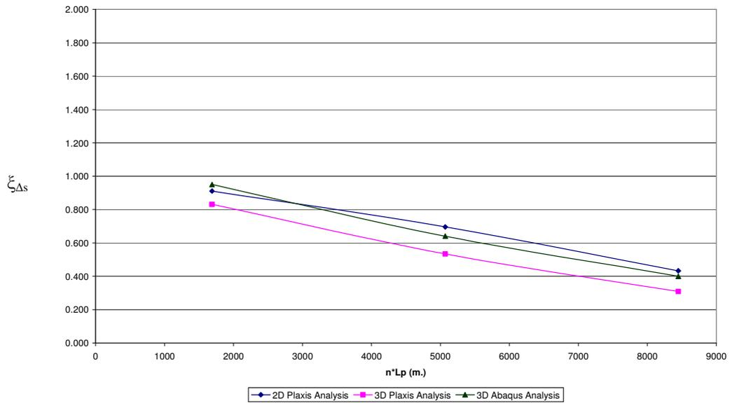
Fig 4.11  $\xi_{\Delta s}$  vs.  $n \cdot L_p$  for Pile Configuration – 1,  $n=169$  &  $V_{ult} / P_{eff} = 20$
