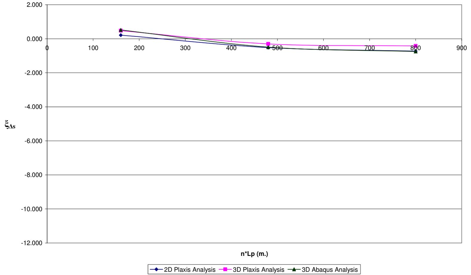
**Fig D.8  $\xi_{As}$  vs.  $n \cdot L_p$  for Pile Configuration – 2,  $n=16$  &  $V_{ult} / P_{eff} = 20$**
