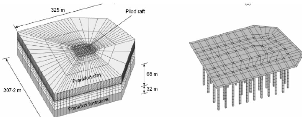
Fig 3.4 The Finite Element Mesh of the System and the Piled Raft for Westend 1
