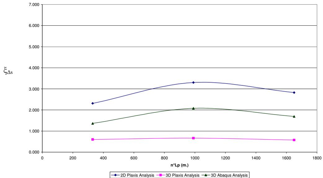
Fig 4.19  $\xi_{\Delta s}$  vs.  $n \cdot L_p$  for Pile Configuration – 3,  $n=33$  &  $V_{ult} / P_{eff} = 5$
