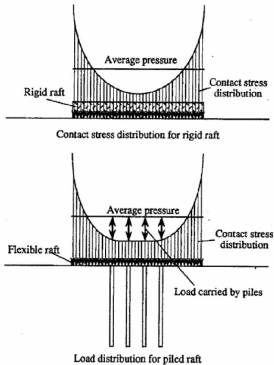
Fig 2.14 Schematic Design Approach for Settlement Reducing Piles
