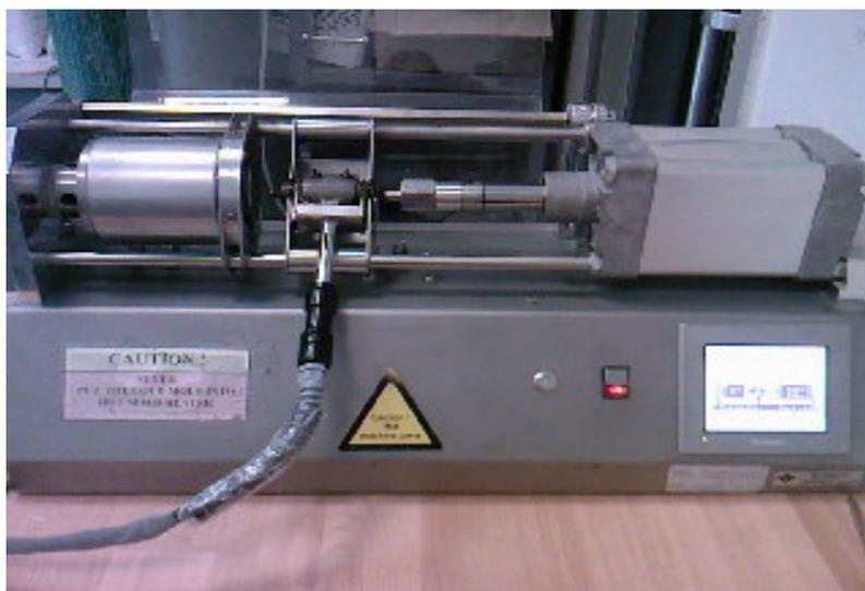
**Figure 3.8** DSM Xplore injection molding machine
