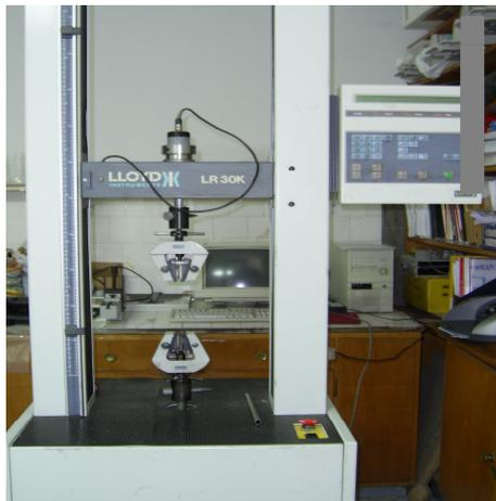
**Figure 3.11** Lloyd LR 30K Universal Testing Machine
