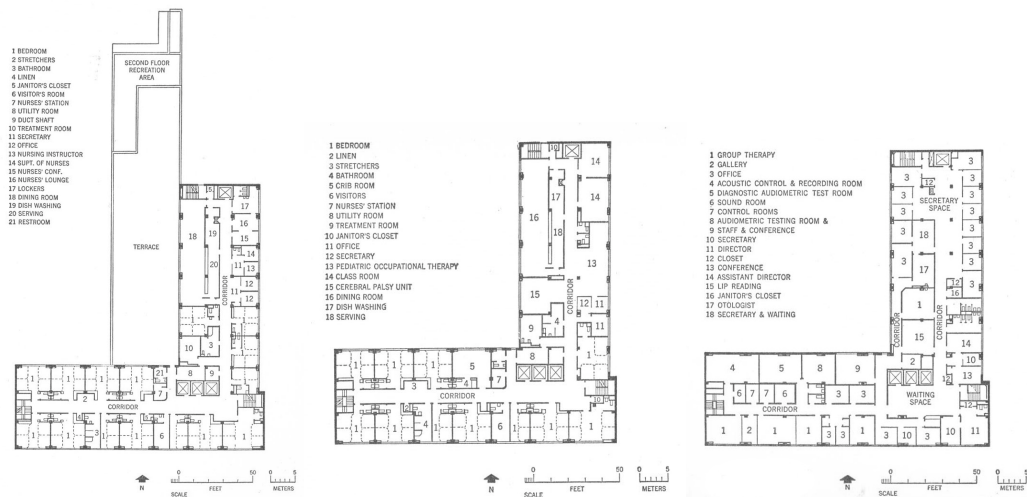
Figure 2.3. Detroit Rehabilitation Institute of Metropolitan Detroit: 3 rd , 4 th , and 5 th Floor Plans. On the third floor, there is an adult in-patient unit; on the fourth floor, pediatric in-patient unit, cerebral palsy unit; on the last floor, speech and hearing area, administrative and staff offices. W. Scott Allan. "Rehabilitation: a community challenge". New York: Wiley, 1958, pp. 54, 55.
