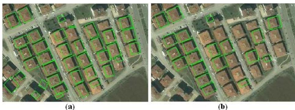
Figure 26 Effect of *Peak\_Thr* parameter on Hough transform a) *Peak\_Thr*=0.4 b) *Peak\_Thr*=0.7
