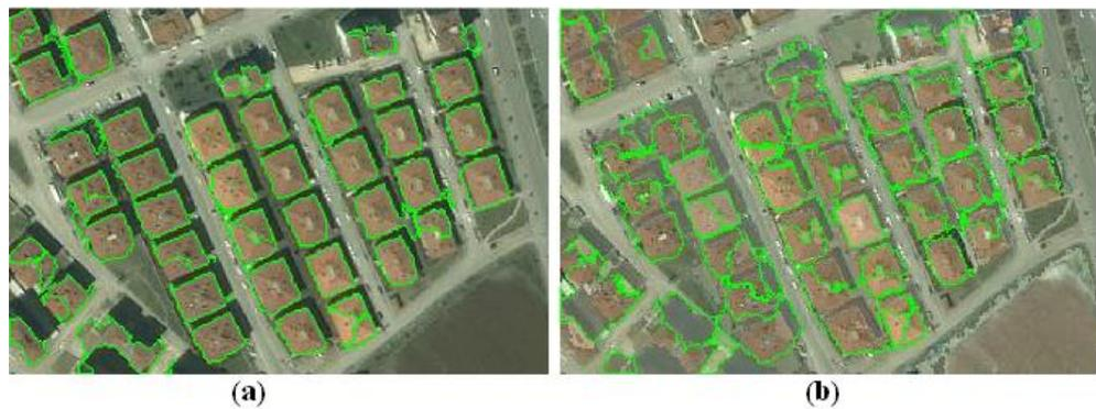
**Figure 44 Mean shift based building detection outputs a) by using original image b) by using shadow removed image**
