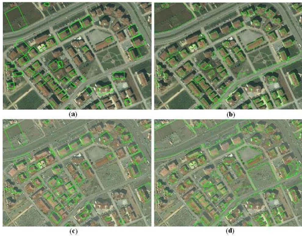
Figure 38 Test Results #7 continued a) Detected buildings by Hough based detection algorithm on original image b) Detected buildings by Mean shift based detection algorithm on original image c) Detected buildings by Hough based detection algorithm on shadow removed image d) Detected buildings by Mean shift based detection algorithm on shadow removed image
