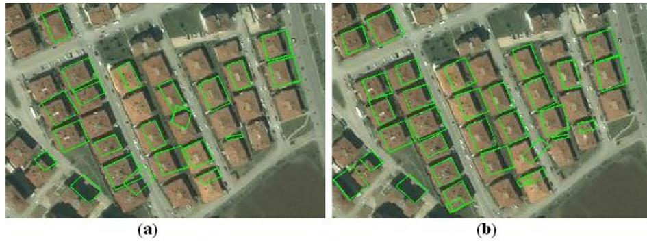
**Figure 24** Effect of *start* and *finish* parameters on Hough transform a) *start* and *finish* are set 90 deg b) *start* = 88, *finish* = 92
