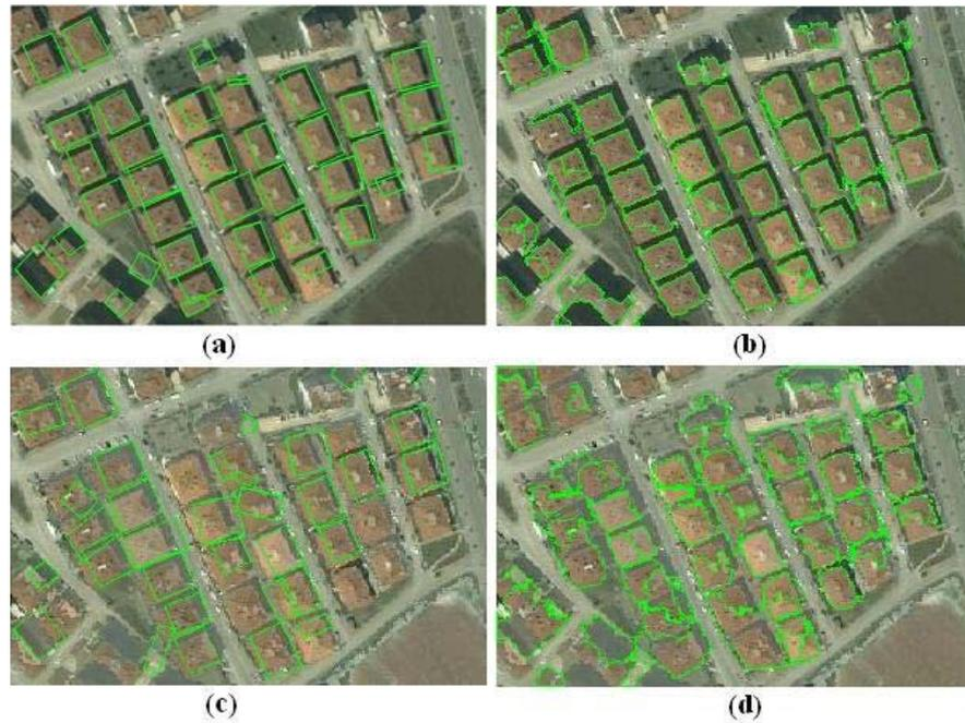
**Figure 31 Test Results #1 continued a) Detected buildings by Hough based detection algorithm on original image b) Detected buildings by Mean shift based detection algorithm on original image c) Detected buildings by Hough based detection algorithm on shadow removed image d) Detected buildings by Mean shift based detection algorithm on shadow removed image**
