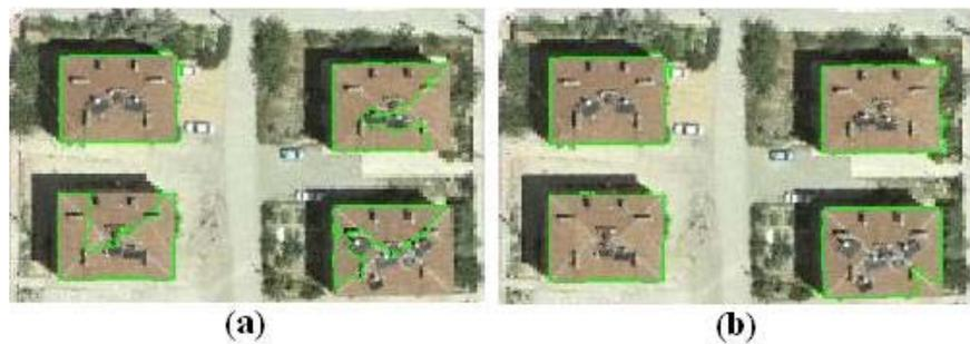
Figure 29 Effect of *THR* parameter on Mean shift based building detection algorithm a) *THR*=8 b) *THR*=15
