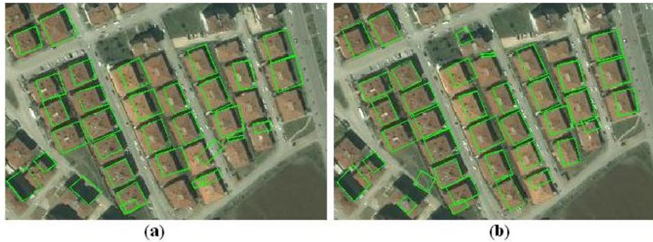
Figure 25 Effect of *Theta\_Res* parameter on Hough transform a) *Theta\_Res*=1 b) *Theta\_Res*=2
