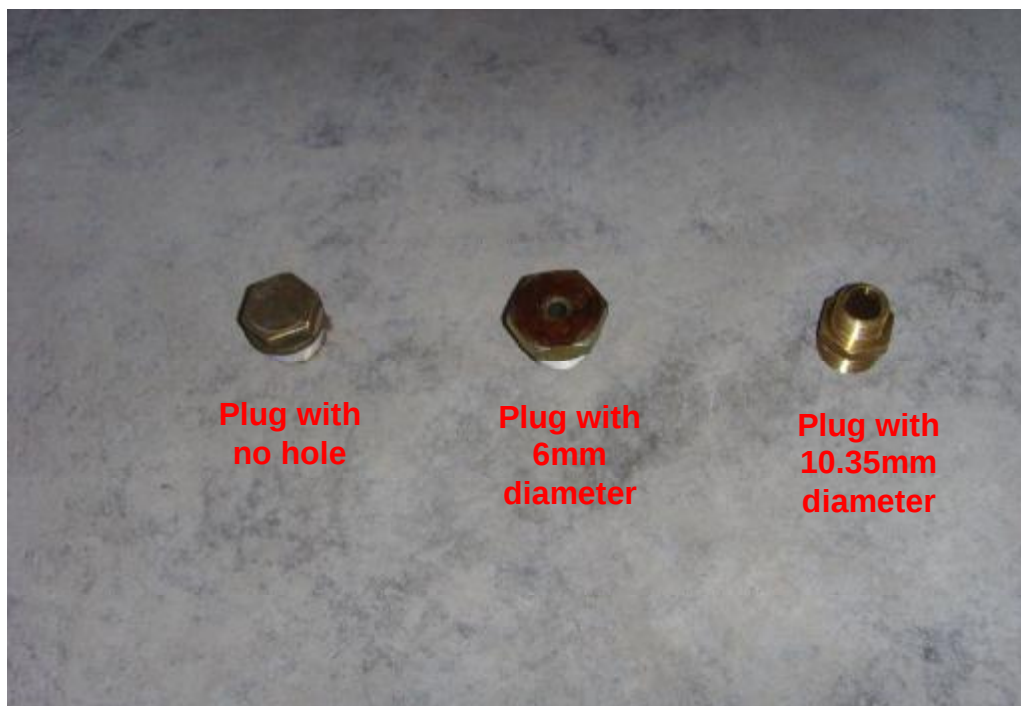
Figure 3.5 Plugs and their dimensions
