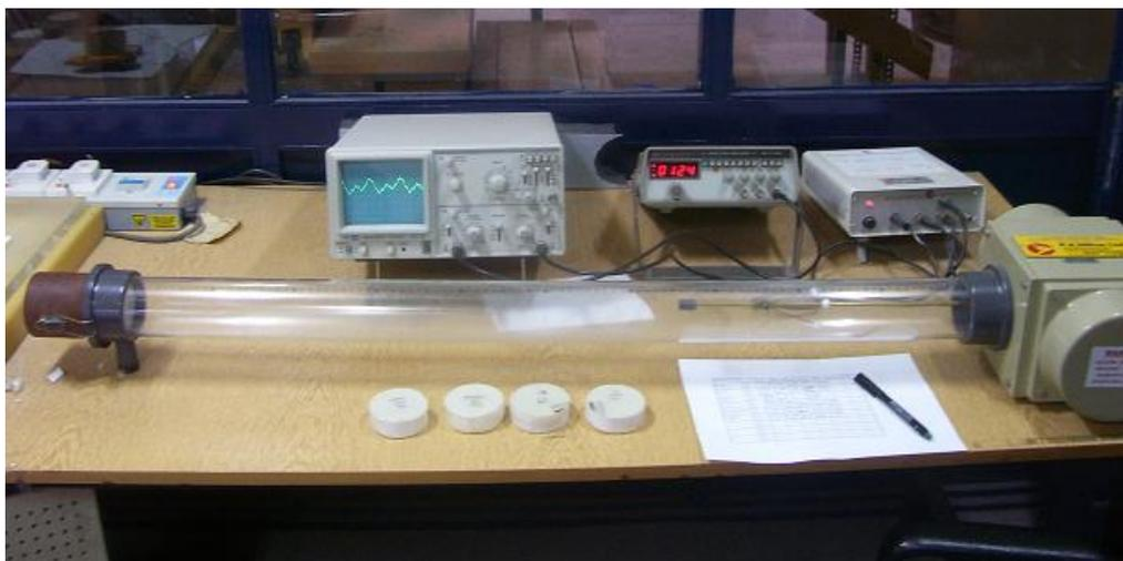
Figure 15. The experimental set-up used in impedance tube measurements
