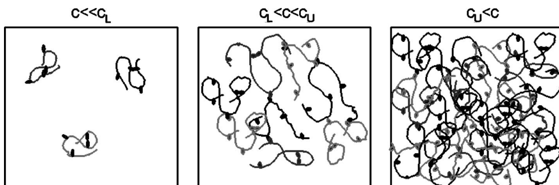
Figure 4.7: Schematic representation of possible hydrophobic interaction modes in different concentration regimes (taken from ref. [29]).
