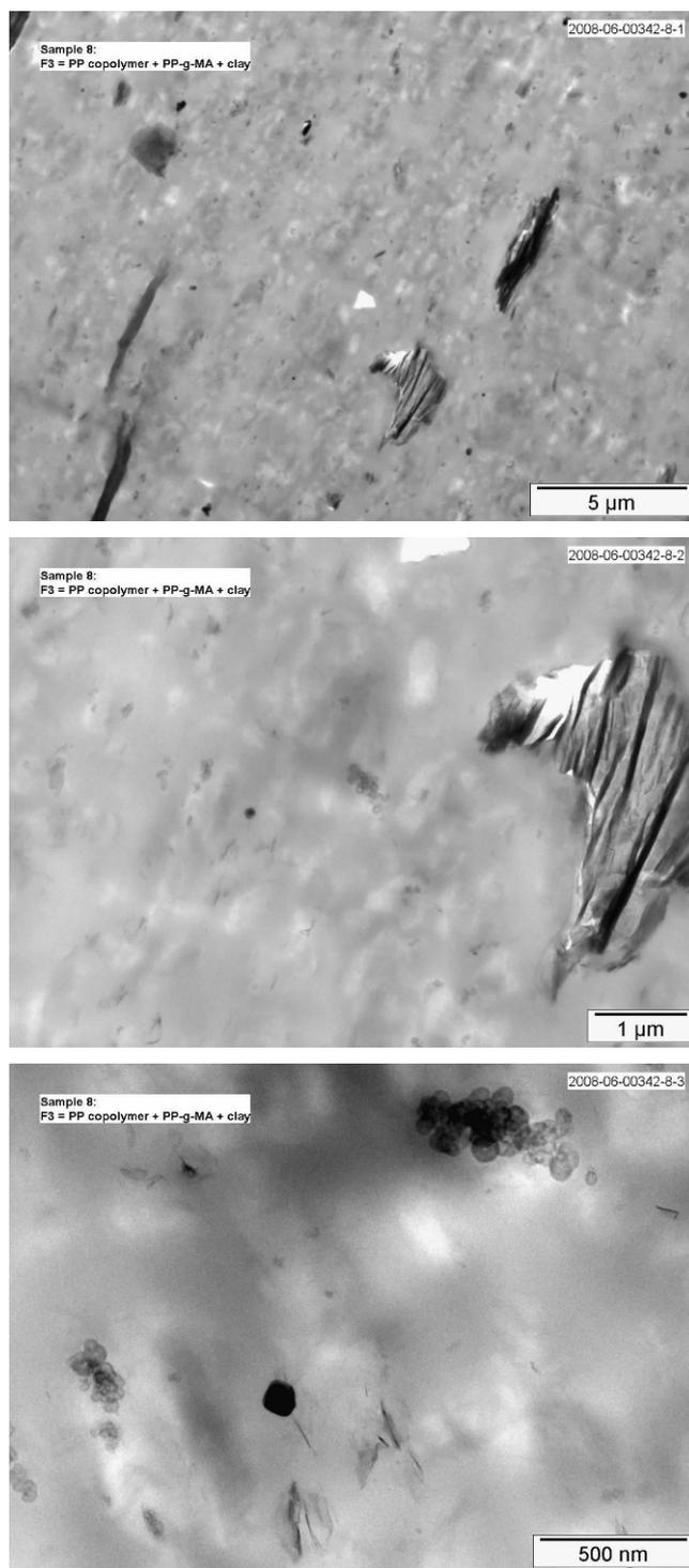
**Figure 4.22** TEM micrographs at different magnifications of the ternary nanocomposite containing recycled polypropylene, 1 wt% Cloisite® 25A and 2 wt% PP-MAH prepared with MB method at 180 °C and 350 rpm screw speed.
