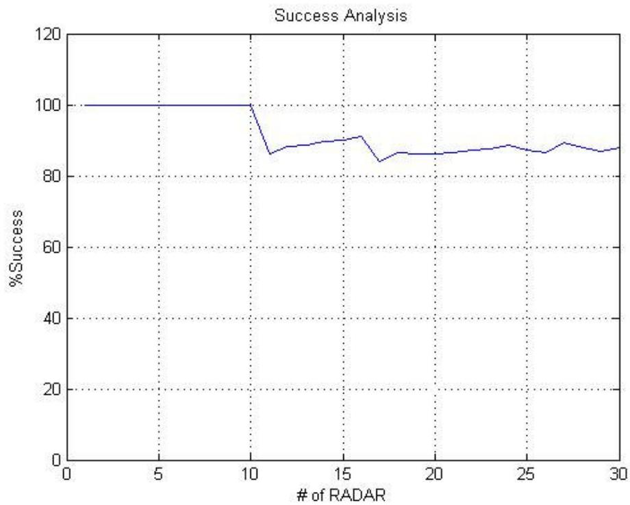
**Figure 5.7 Success Analysis for different numbers of RADARs for 5% jitter and noise rate and 10% missing pulse or false alarm rate**
