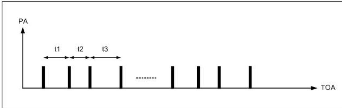
Figure 2.3 Jittered PRI Sequence where  $t_1=t \pm \delta_1$ ,  $t_2=t \pm \delta_2$ ,  $t_3=t \pm \delta_3$
