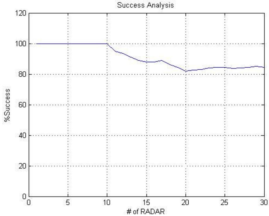
**Figure 5.6 Success Analysis for different numbers of RADARs for 5% jitter and noise rate and 2% missing pulse or false alarm rate**
