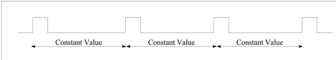
**Figure 3.7 Stable PRI Mode Pulse Sequence**
