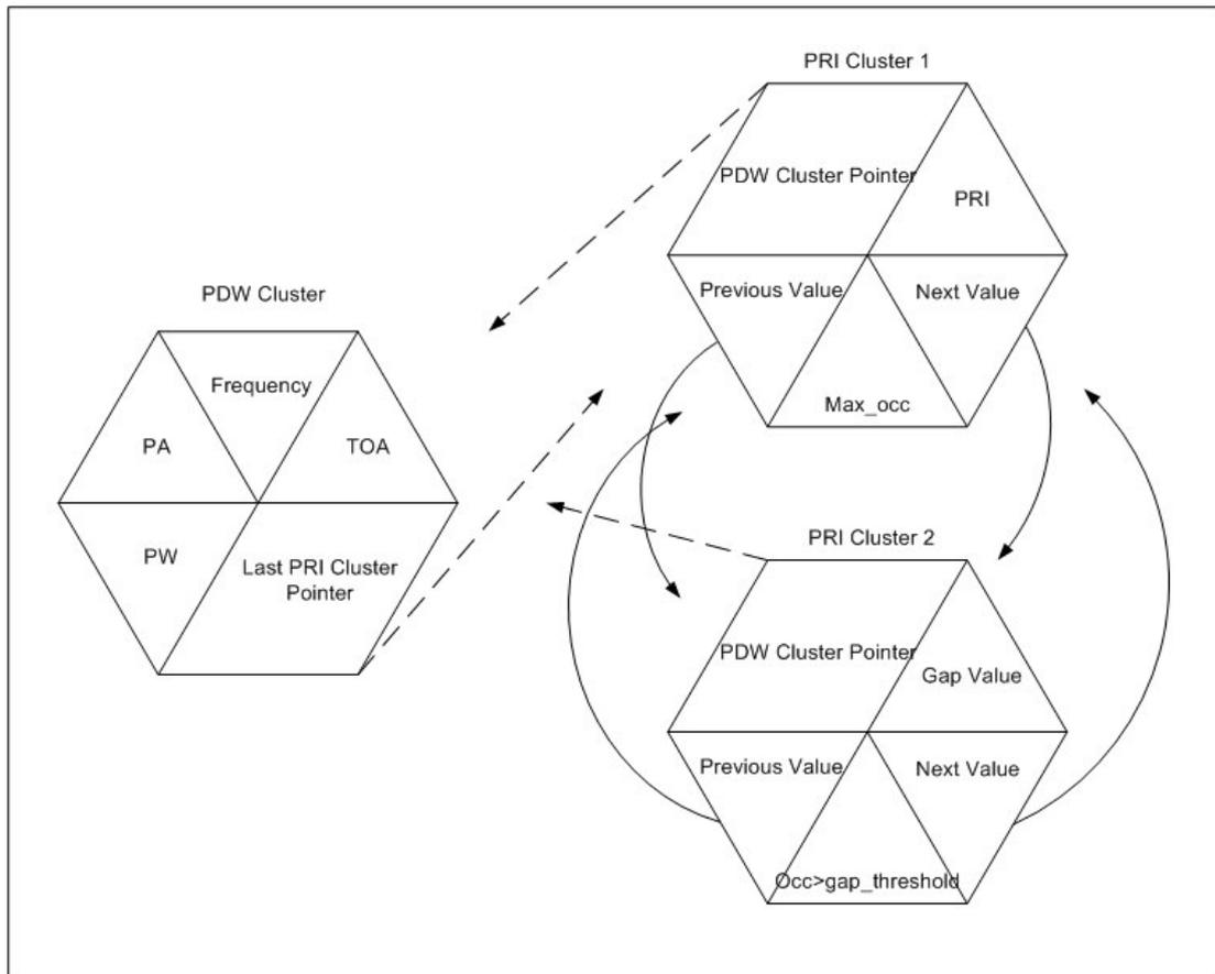
**Figure 3.9 PRI and PDW Clusters of a Dwell PRI mode sequence**
