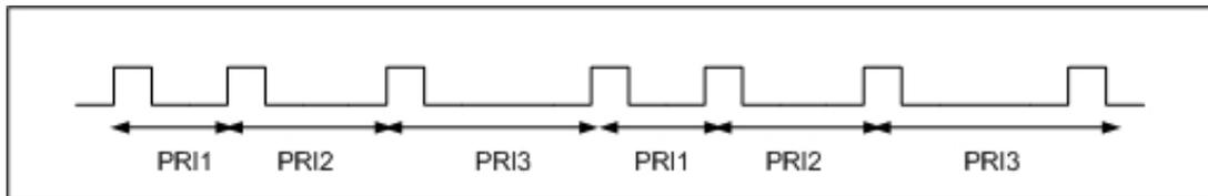
Figure 3.10 Stagger PRI Mode Pulse Sequence
