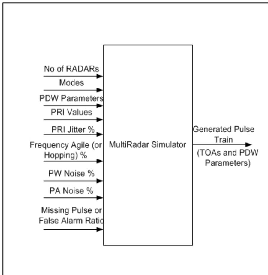
**Figure 5.1 Block Diagram of MultiRadar Simulator**
