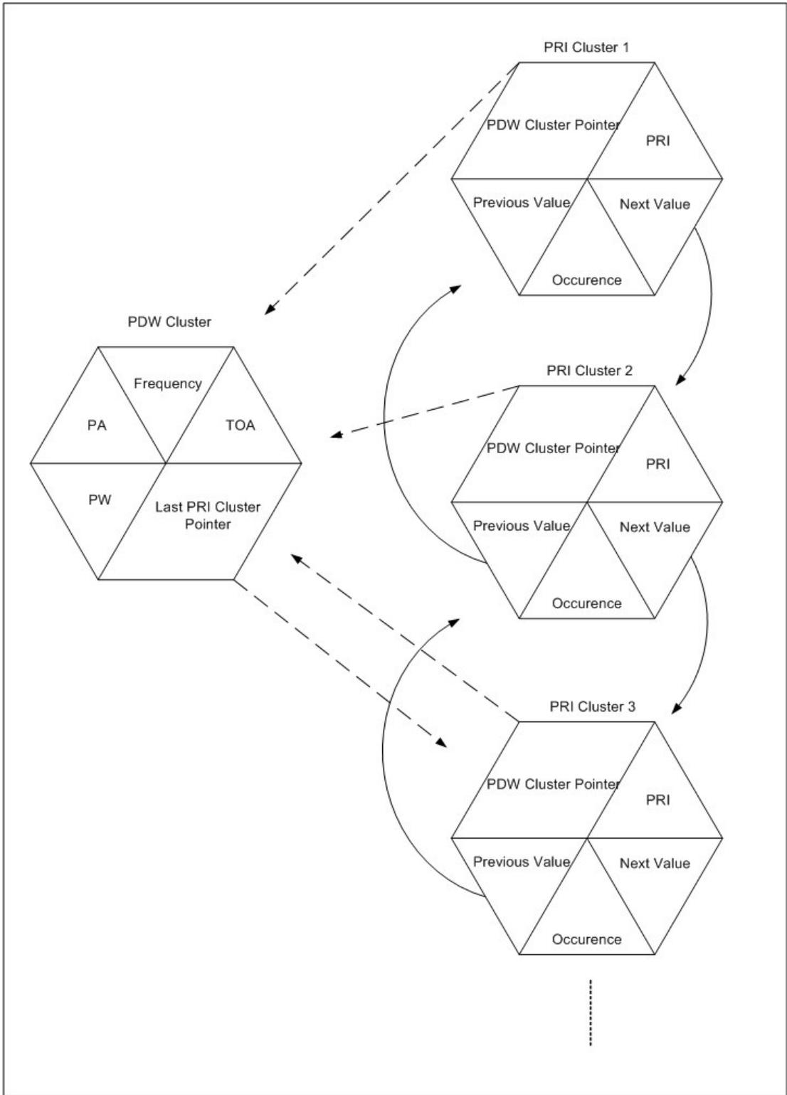
**Figure 3.5 PRI clusters, which are formed by pulses that have matched PDWs**
