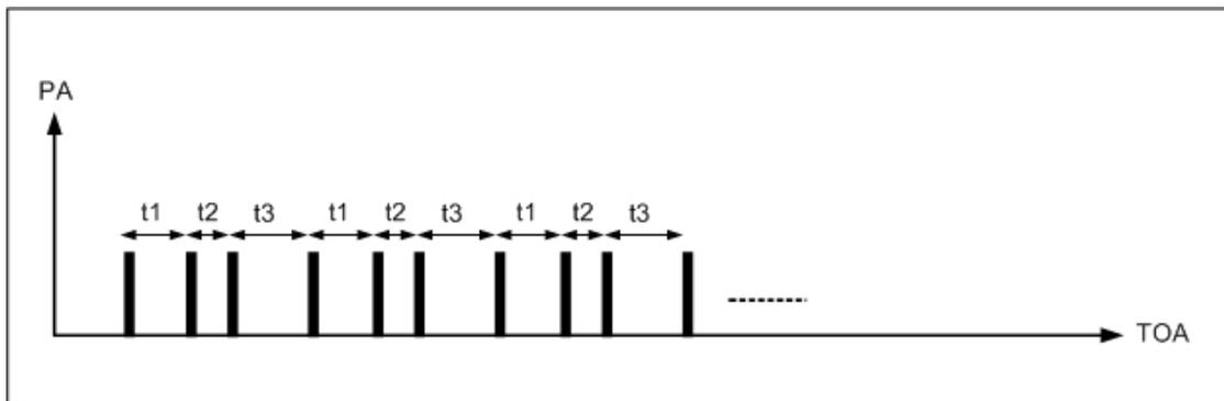
Figure 2.6 Level 3 Stagger PRI Mode pulse sequence
