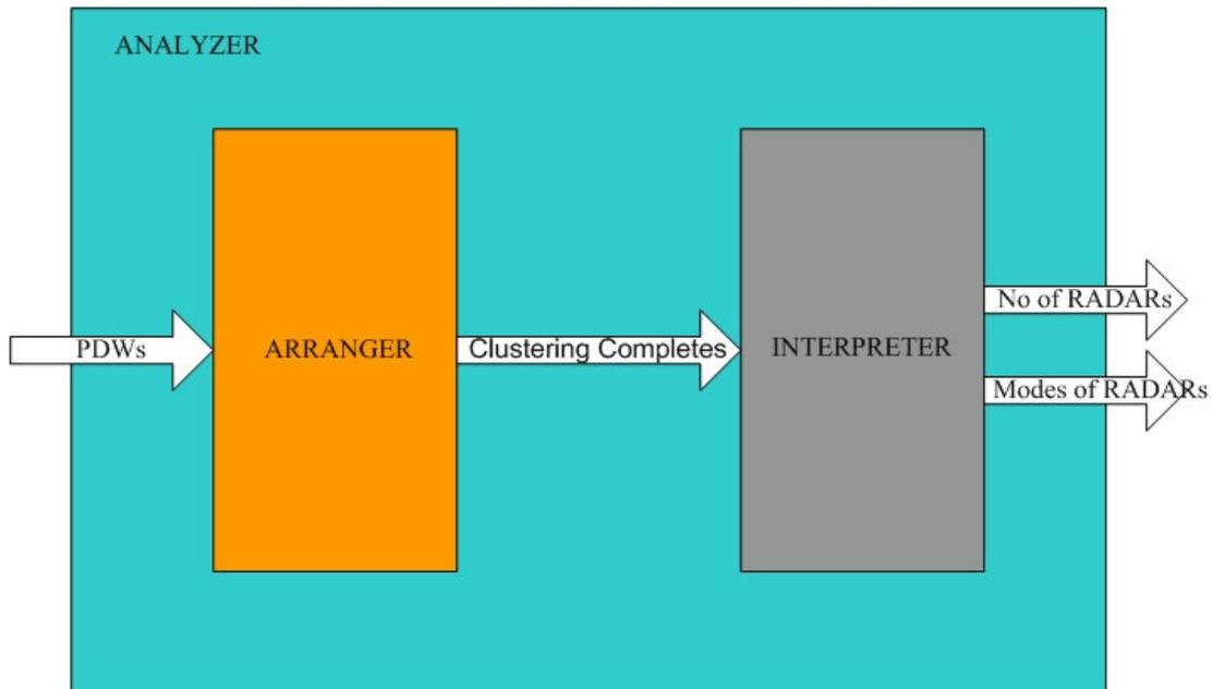
Figure 3.1 The Block Diagram of the Analyzer
