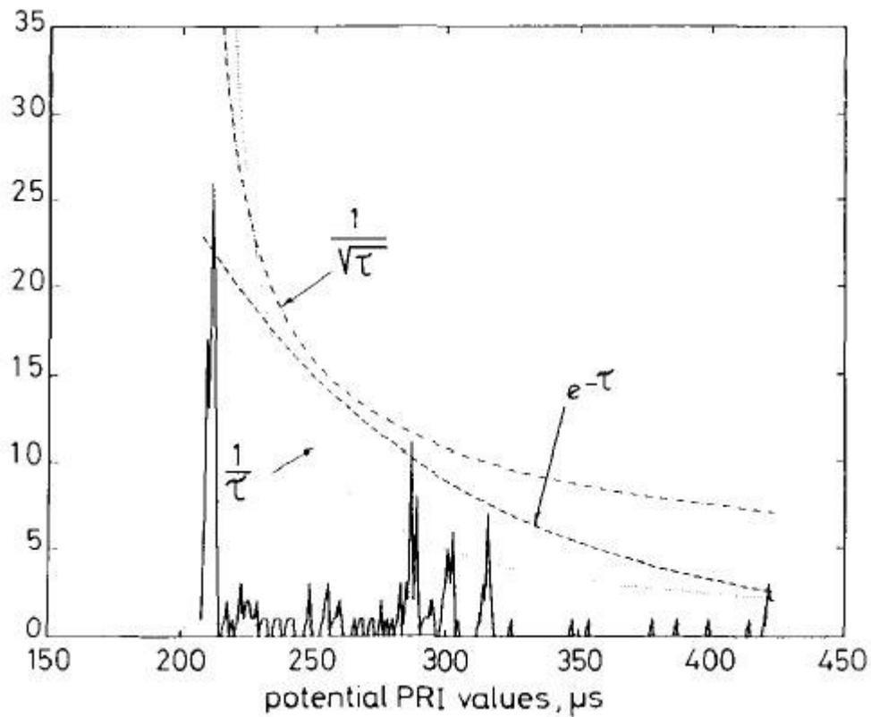
**Figure 4.8 Different forms of threshold in SDIF histogram [8]**
