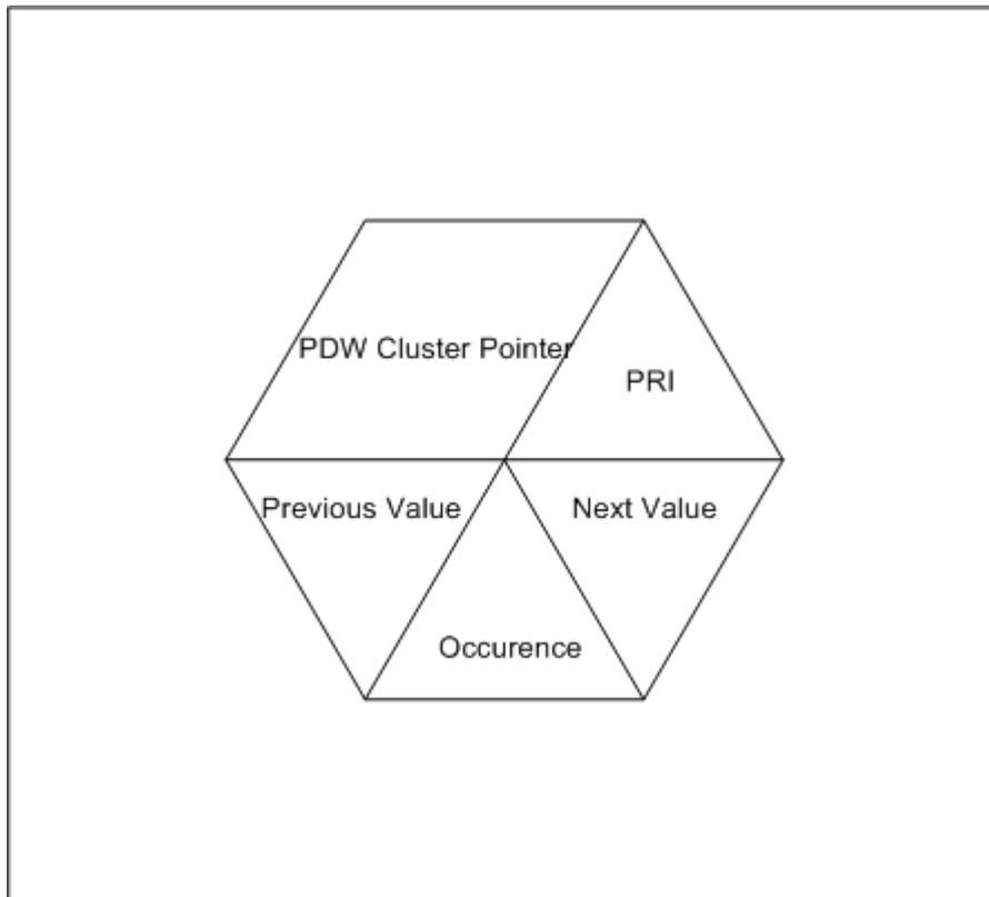
**Figure 3.4 The Basic Structure of a PRI Cluster**
