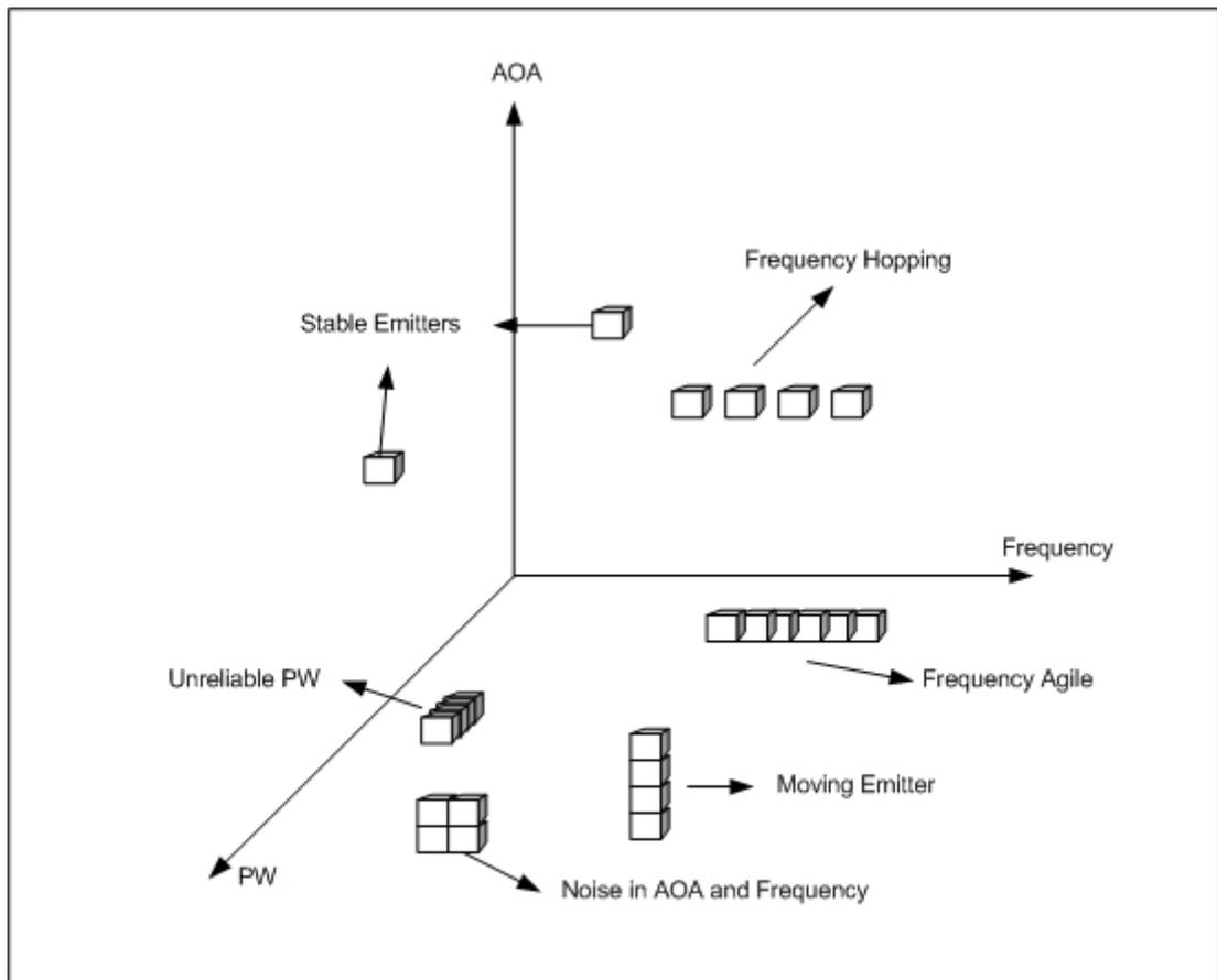
**Figure 2.1 Pulse Separation in AOA, Frequency and PW**
