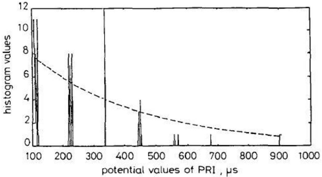
Figure 4.5 SDIF histogram of the TOA first difference in a complex radar environment [8]
