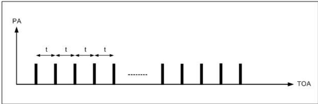
Figure 2.4 Stable PRI Mode pulse sequence
