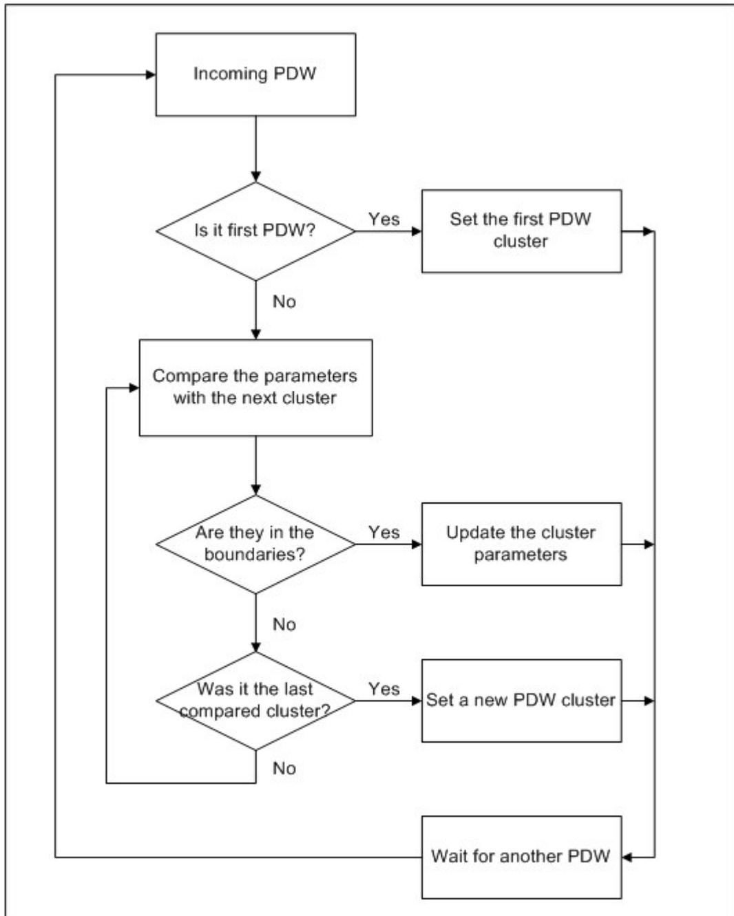
Figure 3.3 The Flowchart of PDW Clustering
