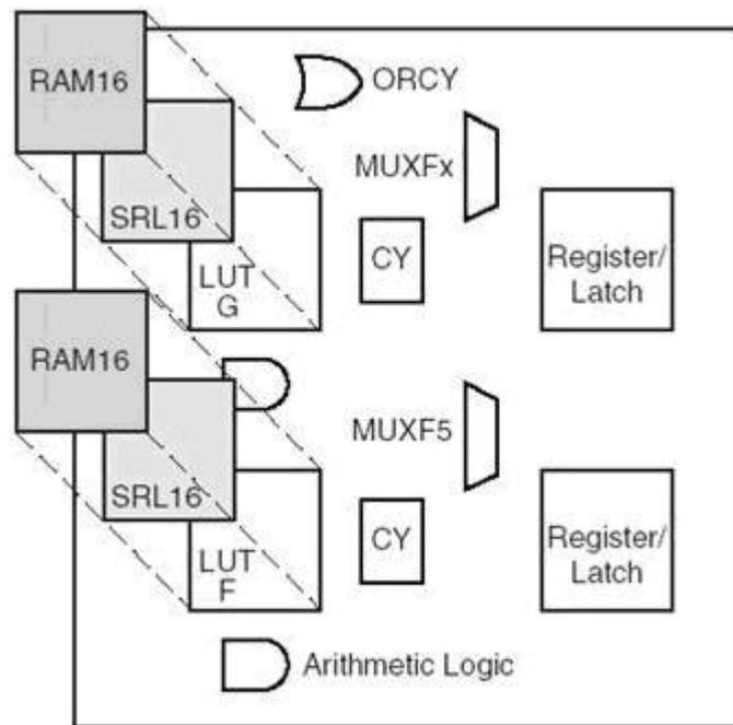
**Figure A.0.1 Virtex Family FPGA Logic Slice**
