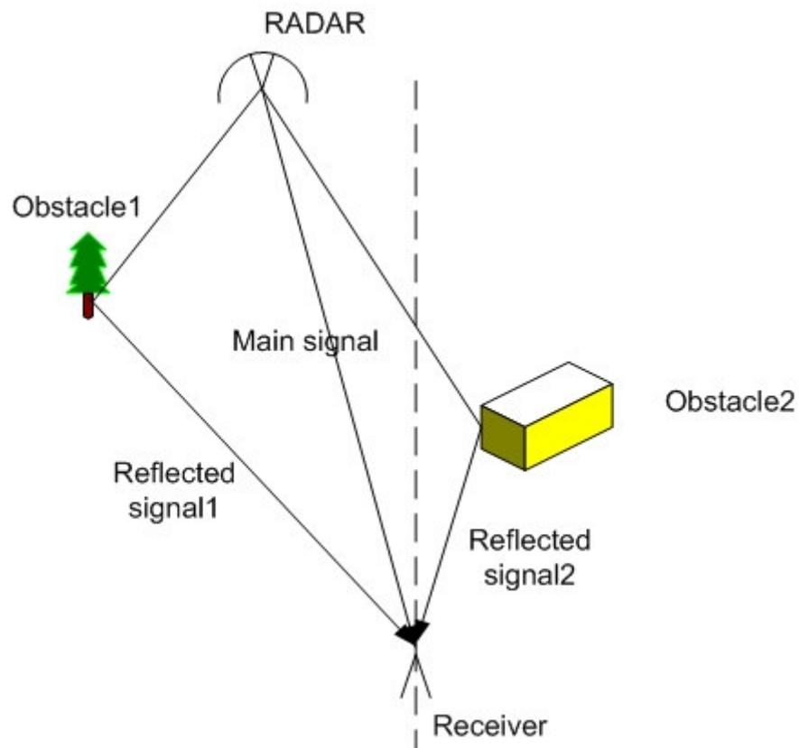
**Figure 2.2 Reflection of Main Signal (corruption of AOA measurement)**
