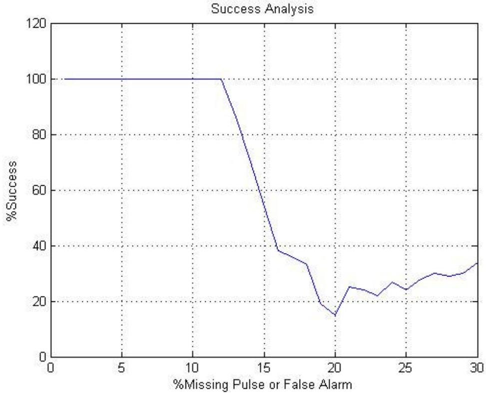
**Figure 5.3 Success Analysis for variable values of missing pulse or false alarm rate**
