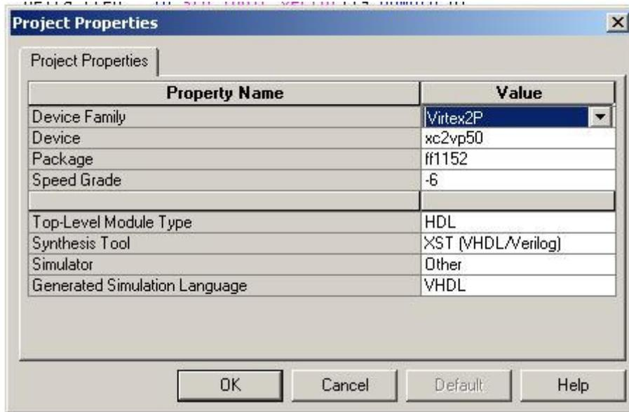
**Figure 6.1 Project Properties of Analyzer**
