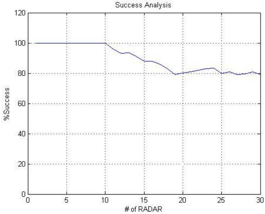
**Figure 5.4 Success Analysis for different numbers of RADARs for 2% jitter and noise rate and 5% missing pulse or false alarm rate**
