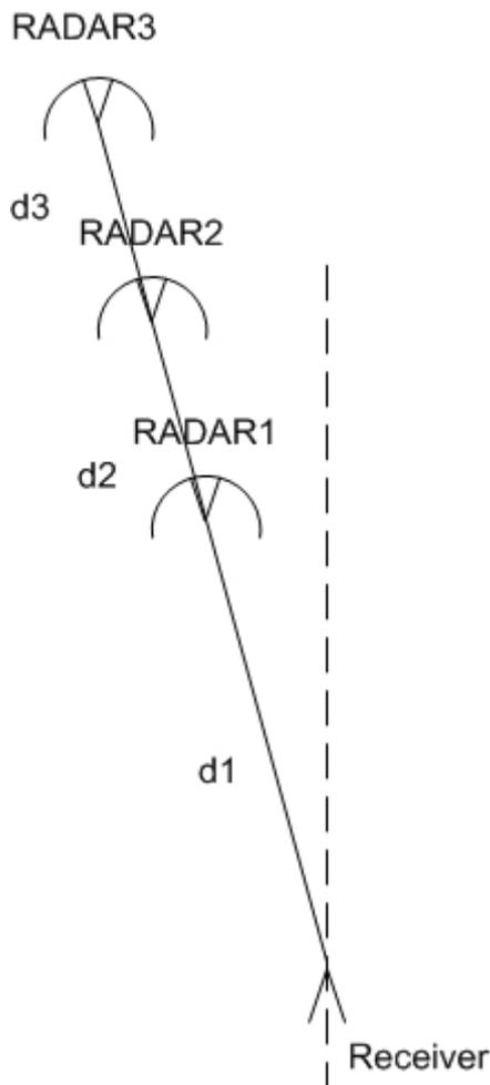
**Figure 5.9 Same RADARs with different distances and same angle to receiver**
