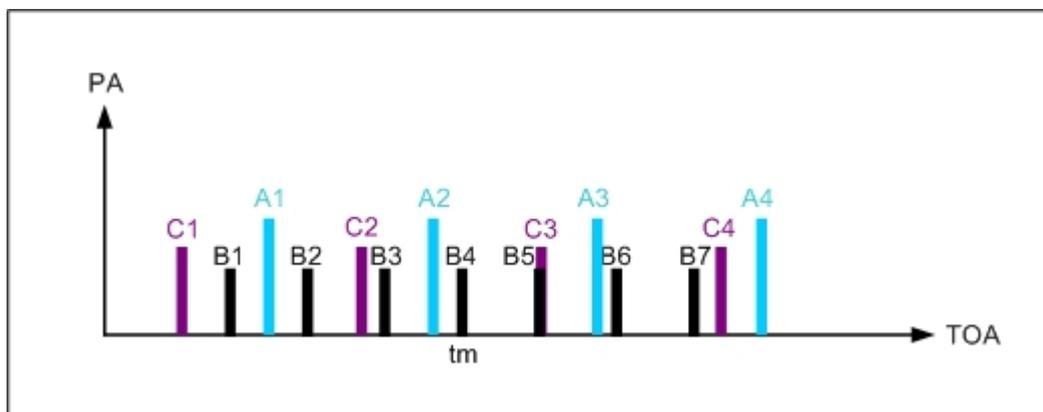
Figure 4.1 3 interleaved stable PRI sequences
