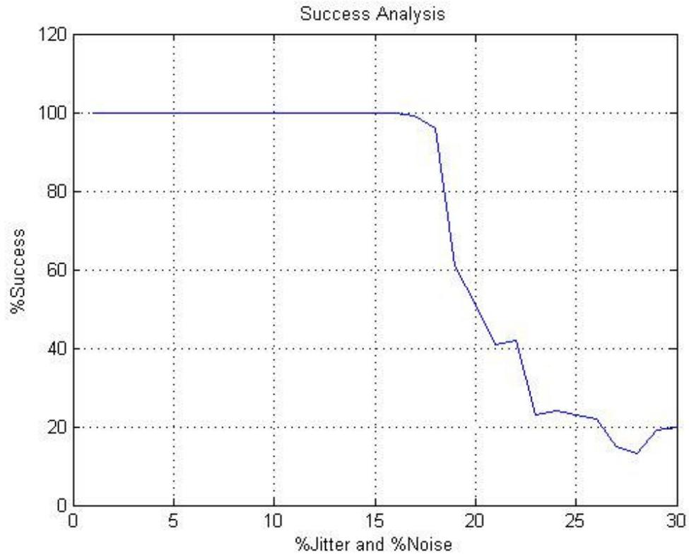
**Figure 5.2 Success Analysis for variable values of jitter and noise rate**
