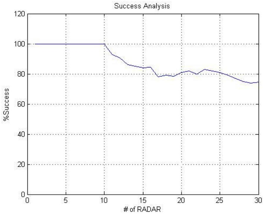
**Figure 5.5 Success Analysis for different numbers of RADARs for 2% jitter and noise rate and 10% missing pulse or false alarm rate**
