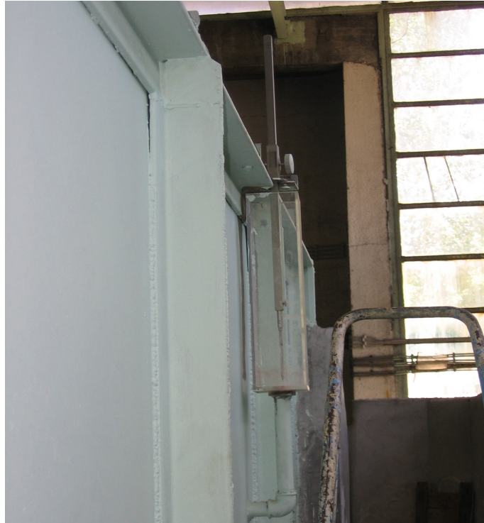
Figure 4.4 Photograph of the point gage used in discharge measurement
