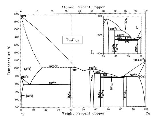
Figure 4.4 Equilibrium binary phase diagram of Ti-Cu.
