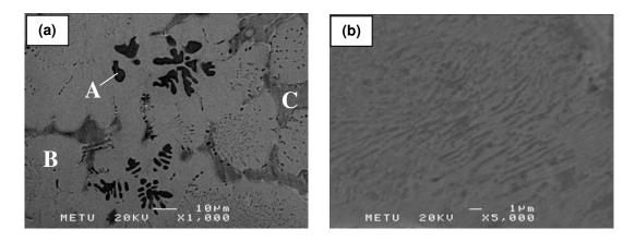
**Figure 4.6** Microstructure of alloy A1 from region 1 at magnification of (a) 1000 and (b) 5000.
