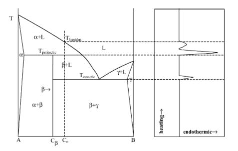
**Figure 2.3** Schematic phase diagram and DSC curve for a hypothetical binary alloy which melts through a sequence of eutectic and peritectic reactions [20].
