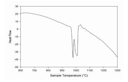
**Figure 4.8** DSC heating curve for alloy A1 obtained with a heating rate of 20°C/min.
