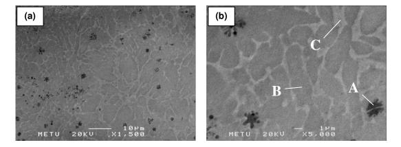
**Figure 4.11** Microstructure of alloy C1 from region X at magnification of (a) 1500 and (b) 5000.
