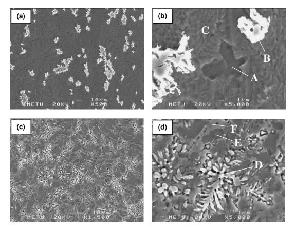
**Figure 4.28** Microstructure of alloy A7 from (a) and (b) region 1. Microstructure of alloy C7 from (d) and (e) region X.
