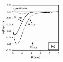
**Figure 4.1** Partial ordering energies, W(R), between pair of constituting element atoms for (a)  $Ti_{64}Cu_{35}Ag_1$ , (b)  $Ti_{64}Cu_{35}Au_1$ , (c)  $Ti_{64}Cu_{35}Al_1$ , (d)  $Ti_{64}Cu_{35}Ni_1$  and (e)  $Ti_{64}Cu_{35}Mn_1$  ternary alloy systems. ( $R_{Ti-Cu}$ =5.1786 at.u.)
