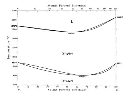
Figure A. 1 Equilibrium binary phase diagram of Ti-Zr.
