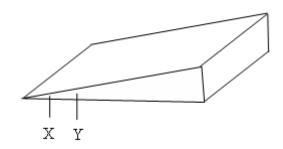
**Figure 4.10** Shape of a centrifugally cast alloy. Thickness changes along the length of the specimen.
