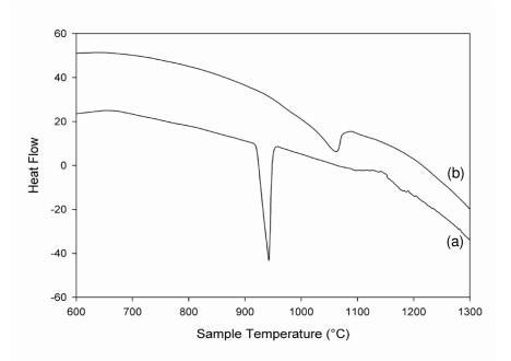
**Figure 4.29** DSC heating curves for (a) alloy A7, and (b) alloy C7 obtained with a heating rate of 20°C/min.
