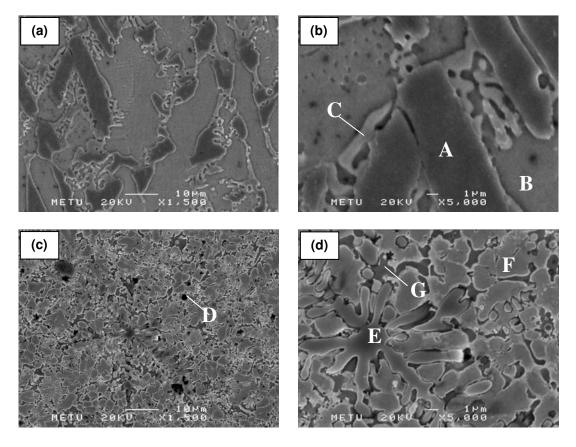
**Figure 4.19** Microstructure of alloy A4 from region 1 at magnification of (a) 1500 and (b) 5000, alloy C4 from region X at magnification of (c) 1500 and (d) 5000.
