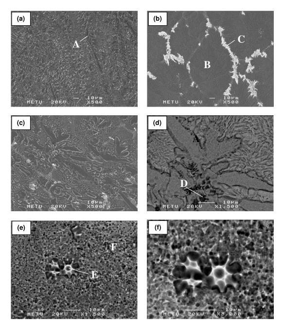
**Figure 4.13** Microstructure of alloy A2 from (a) region 1, (b) region 2, (c) region 3, and (d) region 3 in back scattered electron mode. Microstructure of alloy C2 from region X at magnification of (e) 1500, and (f) 3000.
