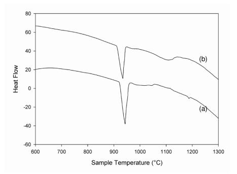
**Figure 4.23** DSC heating curves for (a) alloy A5, and (b) alloy C5 obtained with a heating rate of 20°C/min.
