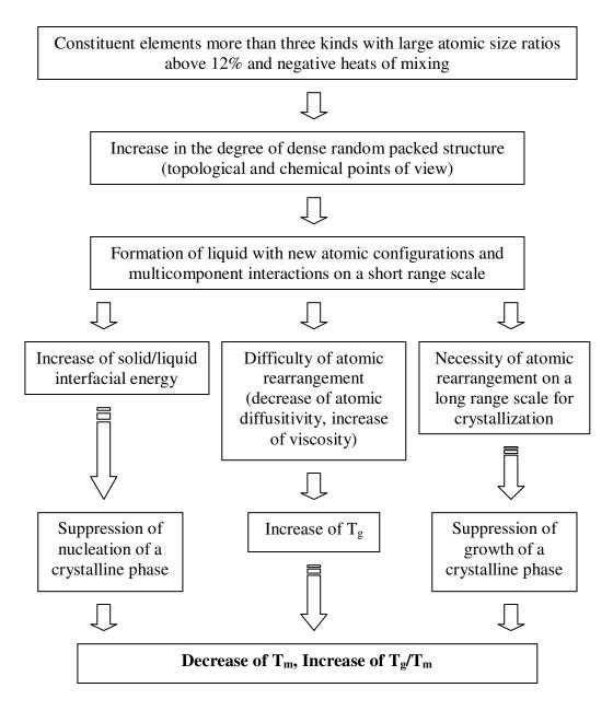
**Figure 2.4** Mechanisms for the stabilization of supercooled liquid and high glass forming ability for the multicomponent alloys which satisfy the rules of semi empirical approach [4].
