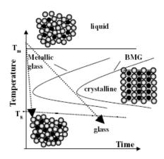
Figure 2.1 Schematic time temperature transformation diagram of structure formation during quenching from the melt [56].
