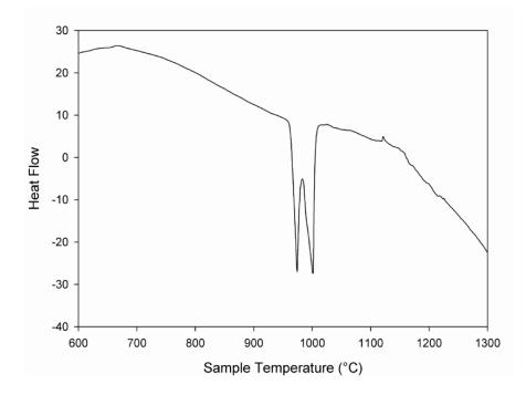
**Figure 4.12** DSC heating curve for alloy C1 obtained with a heating rate of 20°C/min.
