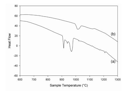
**Figure 4.17** DSC heating curves for (a) alloy A3, and (b) alloy C3 obtained with a heating rate of 20°C/min.
