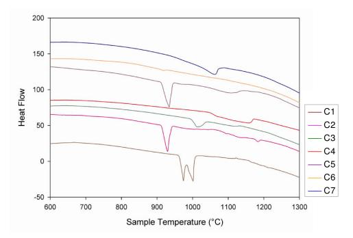
Figure 4.32 Comparison of DSC patterns of centrifugal cast alloys.
