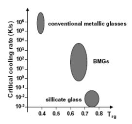
**Figure 2.2** Critical cooling rate versus reduced glass transition temperature  $T_{rg}$  for conventional metallic glasses, silicate glasses and bulk metallic glasses [56].
