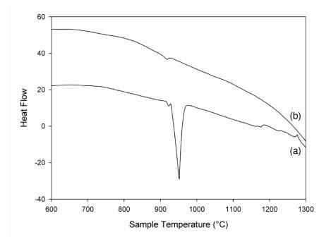
**Figure 4.26** DSC heating curves for (a) alloy A6, and (b) alloy C6 obtained with a heating rate of 20°C/min.
