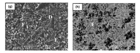
**Figure 4.22** Microstructure of alloy A5 from (a) and (b) region 1, (c) region 2, (d) region 2 in back scattered electron mode, (e) region 3 and (f) region 3 in back scattered electron mode. Microstructure of alloy C5 from (g) region X and (h) region X in back scattered electron mode.
