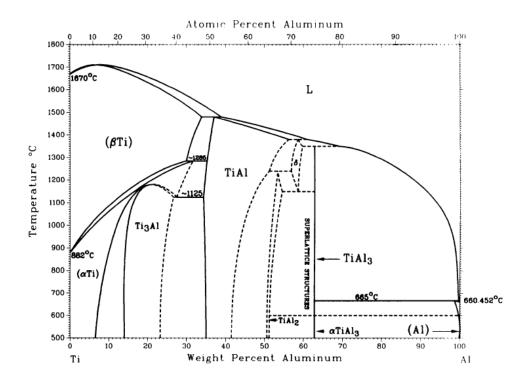
Figure A. 5 Equilibrium binary phase diagram of Ti-Al.
