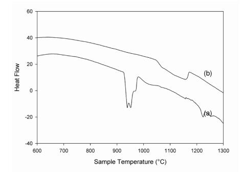
**Figure 4.20** DSC heating curves for (a) alloy A4, and (b) alloy C4 obtained with a heating rate of 20°C/min.
