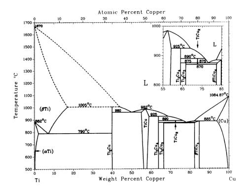
Figure A. 3 Equilibrium binary phase diagram of Ti-Cu.
