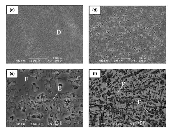
**Figure 4.25** Microstructure of alloy A6 from (a) and (b) region 1, (c) region 3. Microstructure of alloy C6 from (d) and (e) region X, (f) region X in back scattered electron mode.
