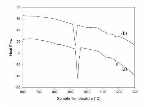
**Figure 4.14** DSC heating curves for (a) alloy A2, and (b) alloy C2 obtained with a heating rate of 20°C/min.
