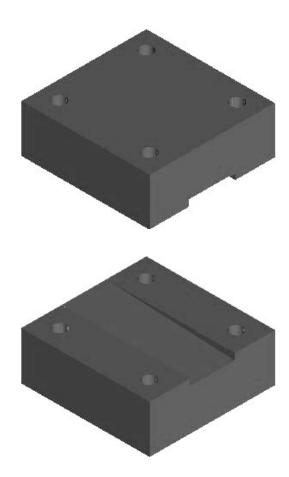
Figure 3.2 Schematic view of copper mold.
