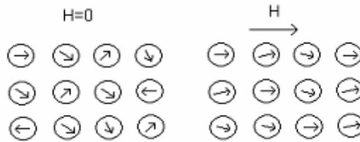
**Figure 4** The atomic dipole configuration for a paramagnetic material with or without a magnetic field [30].
