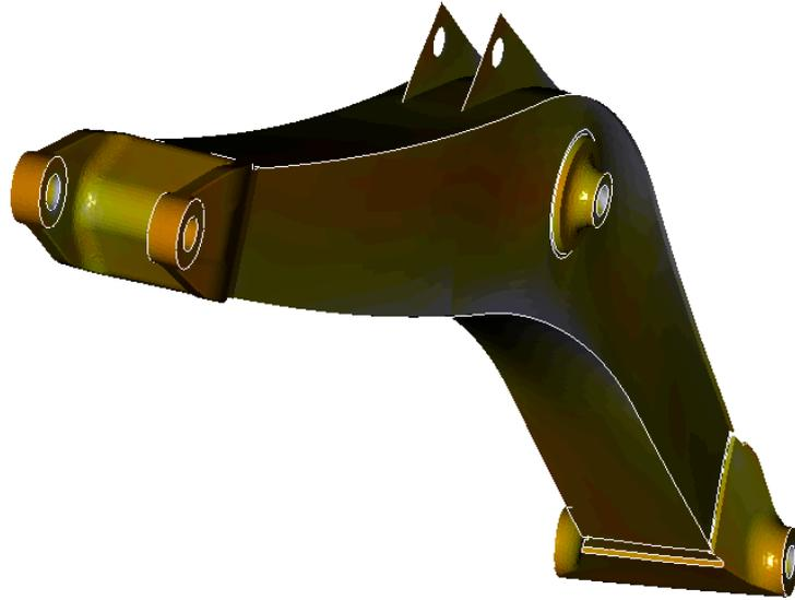
Figure 1.5 – Deformation shape of the excavator boom which is subjected to arm breakout force and lateral force.
