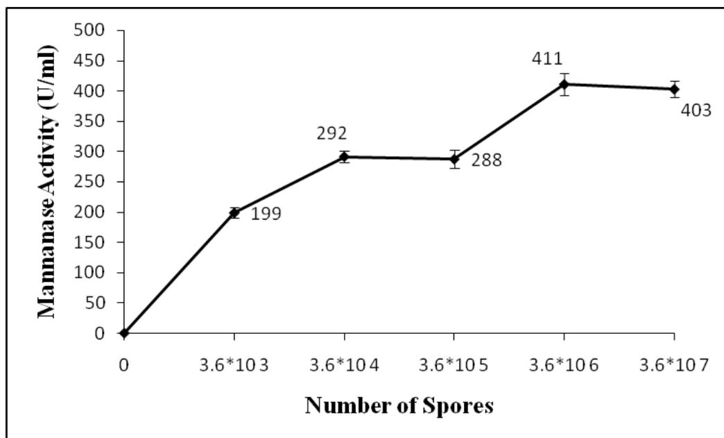
**Figure 3.10** Effect of number of spores on mannanase production by AsT1 grown in the modified YpSs medium containing 2.24 % carbon, 0.43 %  $\text{NH}_4\text{NO}_3$ , 0.1%  $\text{K}_2\text{HPO}_4$ , 0.05%  $\text{MgSO}_4$ , at 30 °C, 210 rpm.
