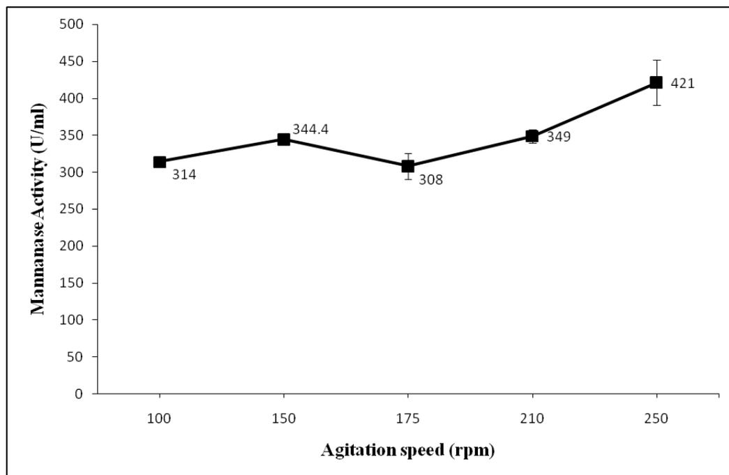
**Figure 3.15** Mannanase activities in the modified YpSs medium containing (w/v), 2.24% sucrose, 0.43%  $\text{NH}_4\text{NO}_3$  at 30 °C, at different agitation rates.
