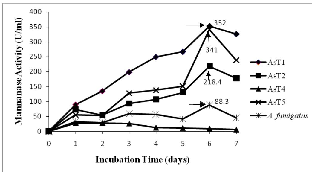
**Figure 3.1** Comparison of mannanase production of *A. sojae* transformants and *A. fumigatus* IMI 385708 in modified YpSs medium with 2% glucose (*A. sojae*) and 2% LBG (*A. fumigatus*), at 30 °C, 155 rpm.
