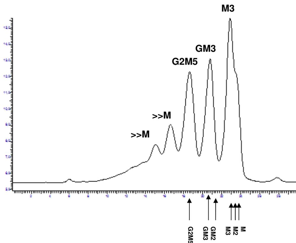
**Figure 3.25** HPLC Chromatogram of the Hydrolysis Products. 900  $\mu$ l of (% 0,5, w/v) locust-bean gum solution was incubated with 100  $\mu$ l crude mannanase enzyme (40 Unit), 50  $^{\circ}$ C for 48 hours.
