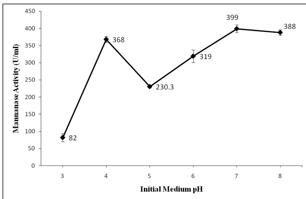
**Figure 3.11** Effect of initial pH of medium on the mannanase production by AsT1 in the modified YpSs medium (2.24% sucrose), 0.43 %  $\text{NH}_4\text{NO}_3$ , 0.1%  $\text{K}_2\text{HPO}_4$ , 0.05%  $\text{MgSO}_4$ , at 30 °C, 210 rpm.
