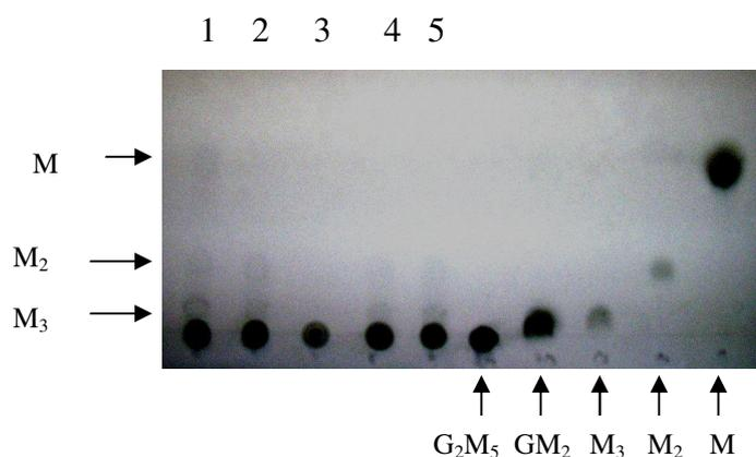
**Figure 3.24** TLC Analysis of the LBG Hydrolysis Products; M, M<sub>2</sub>, M<sub>3</sub> can be observed on the TLC plate as a result of incubation of 10 ml of (% 0,5, w/v) LBG with 2 ml crude mannanase enzyme (600 Unit) after: 1) 48 h; 2,3) 24 h; 4,5) 16 h.
