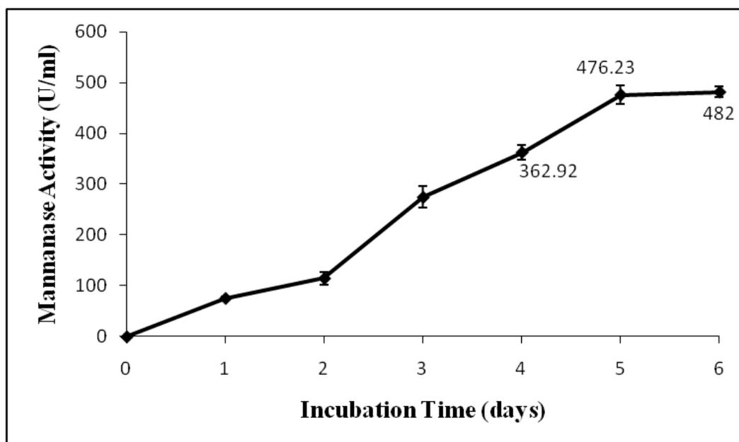
**Figure 3.23** Time course of mannanase production by AsT1 under the predicted optimum conditions; modified YpSs medium (7% molasses, 0.43%  $\text{NH}_4\text{NO}_3$ , 0.1%  $\text{K}_2\text{HPO}_4$ , 0.05%  $\text{MgSO}_4$ , w/v) at 30 °C, 207 rpm.
