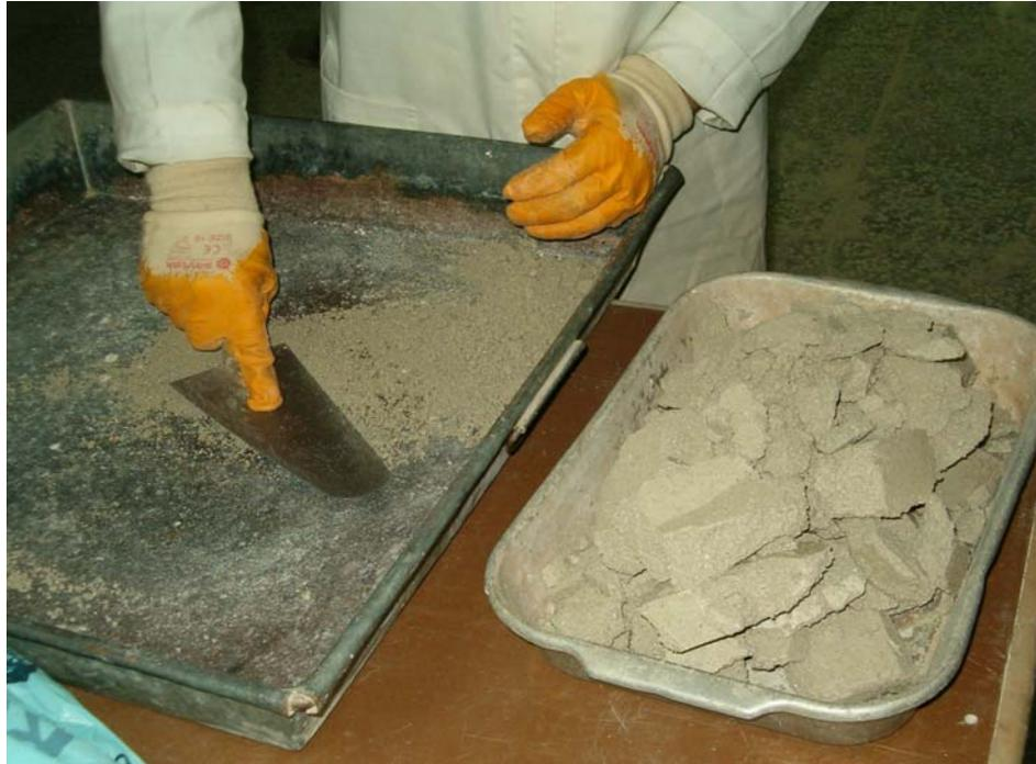
Figure 4.11 Crumbling of the soil after the test
