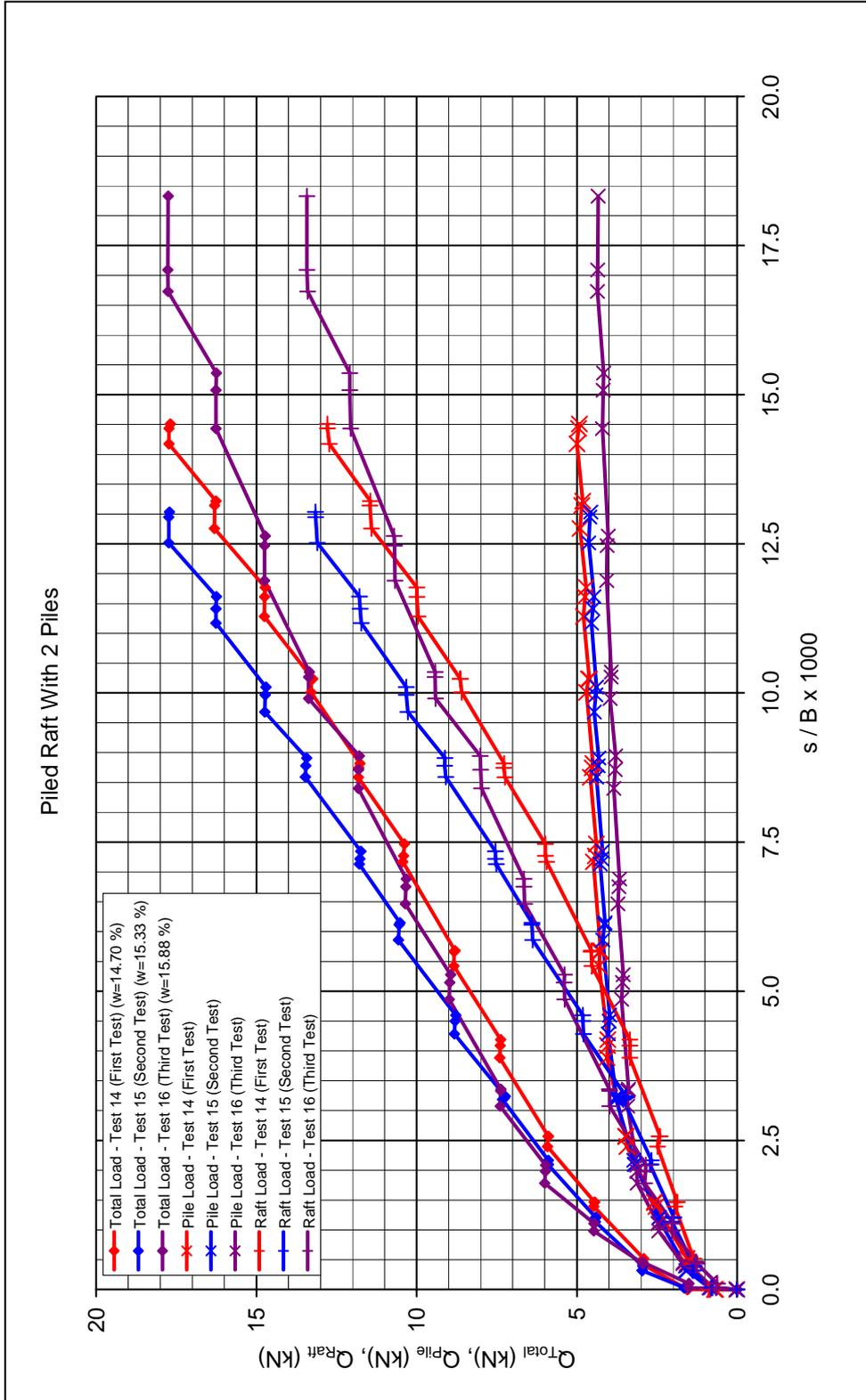
Figure 6.10 Load-settlement relationship of piled raft with 2 piles
