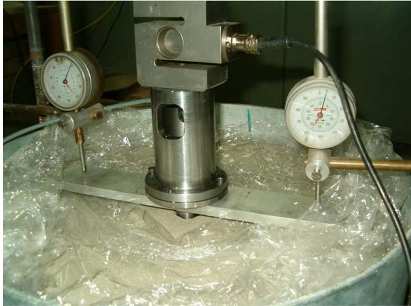
Figure 5.5 Single pile test setup
