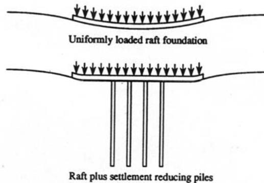
Figure 2.3 Central piles to reduce differential settlement (Randolph, 1994)
