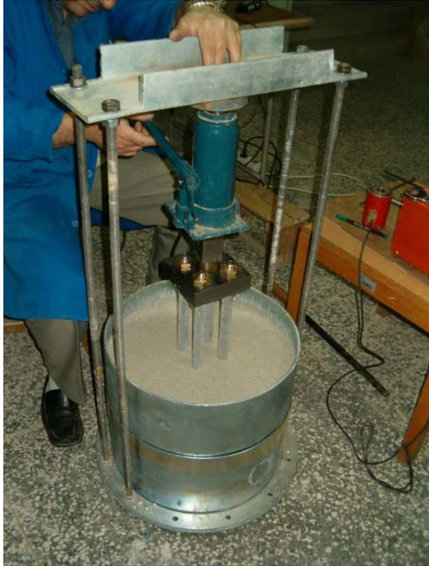
Figure 4.9 Placement of the model piled raft in the container
