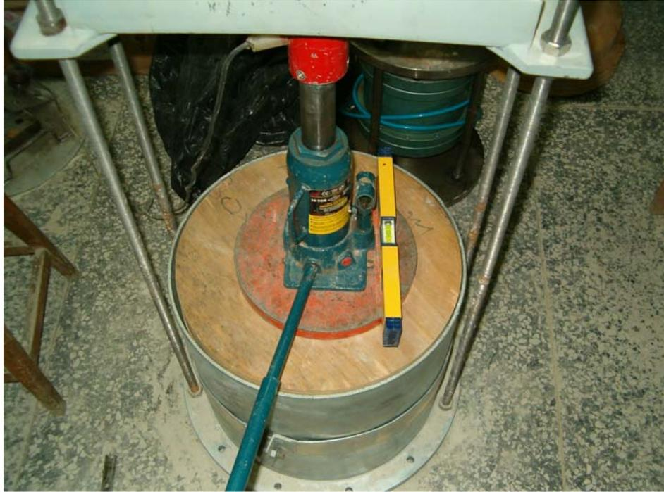
Figure 4.2 Compressing of the soil layers
