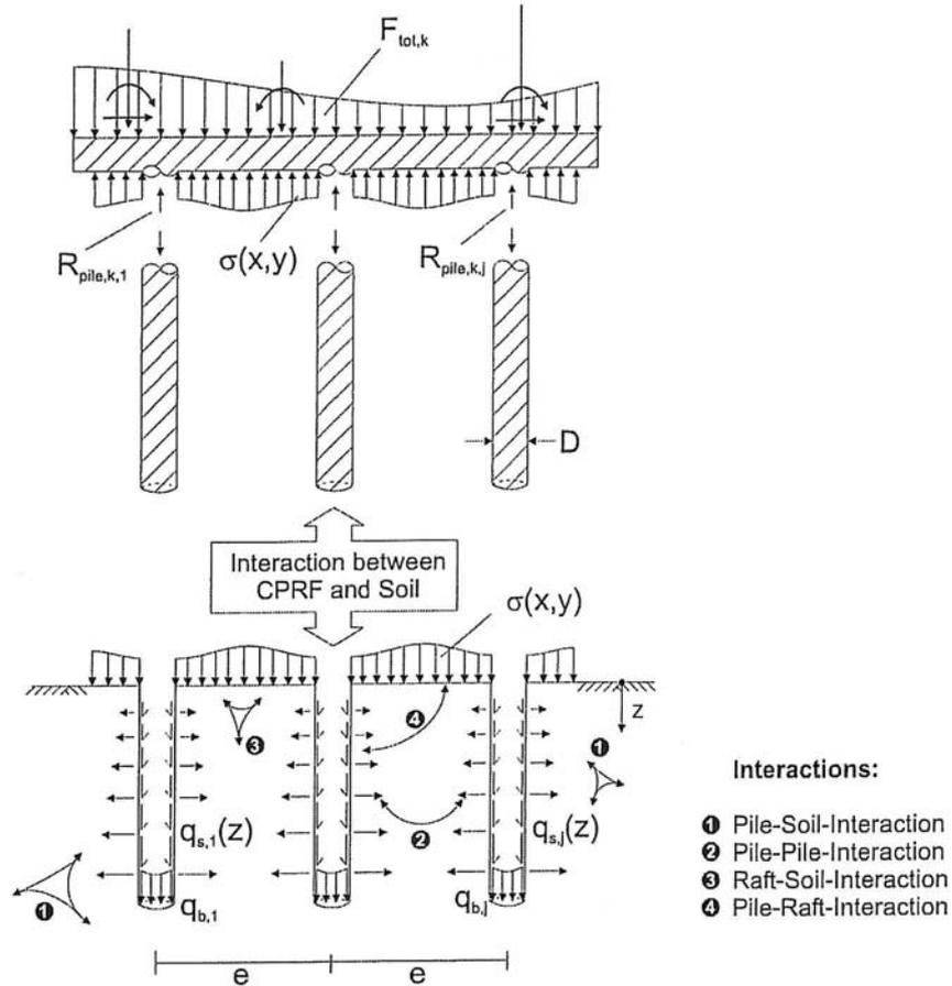
Figure 2.1 Soil-structure interaction of piled rafts (Katzenbach et al., 2004)
