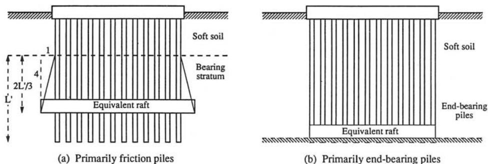
Figure 2.5 Equivalent raft approach for pile groups (Randolph, 1994)
