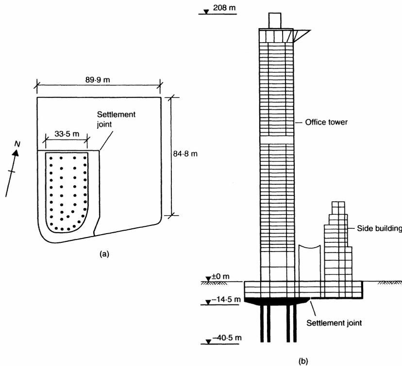
Figure 2.12 DG-Bank building: a) ground plan, b) sectional elevation
