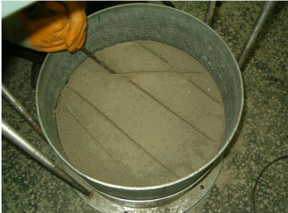
Figure 4.3 Scratching of the soil layer surface
