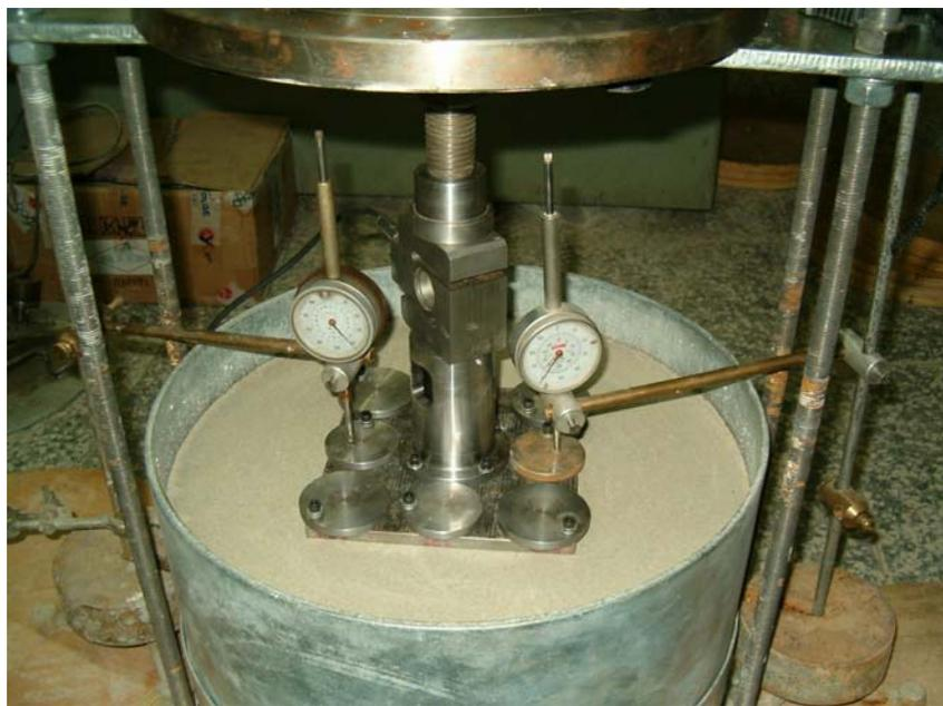
Figure 5.2 Plain raft test setup
