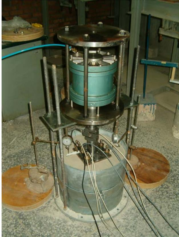
Figure 4.7 Pneumatic air cylinder and the loading system
