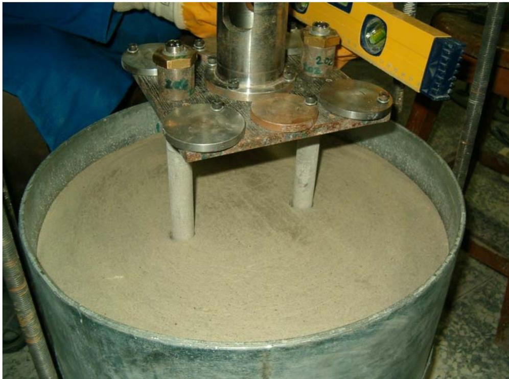
Figure 5.8 Model piled raft with 2 piles
