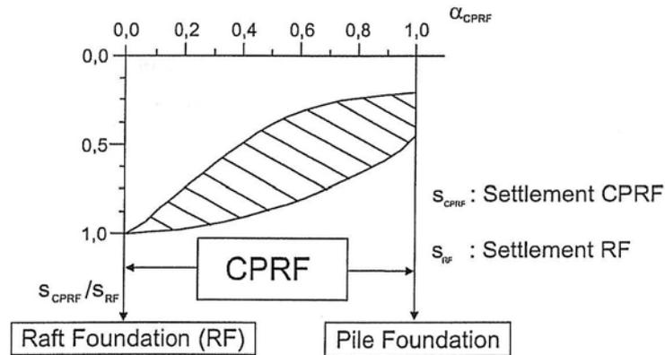
Figure 2.2 Foundation settlements as a function of piled raft coefficient
