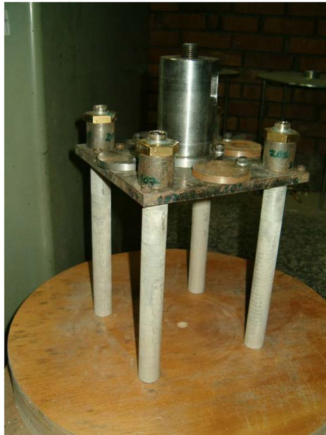
Figure 5.13 Model piled raft with 4 piles
