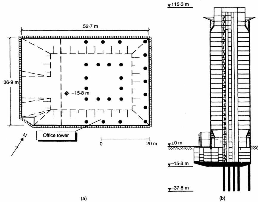
Figure 2.13 Japan-Centre building: a) ground plan b) sectional elevation
