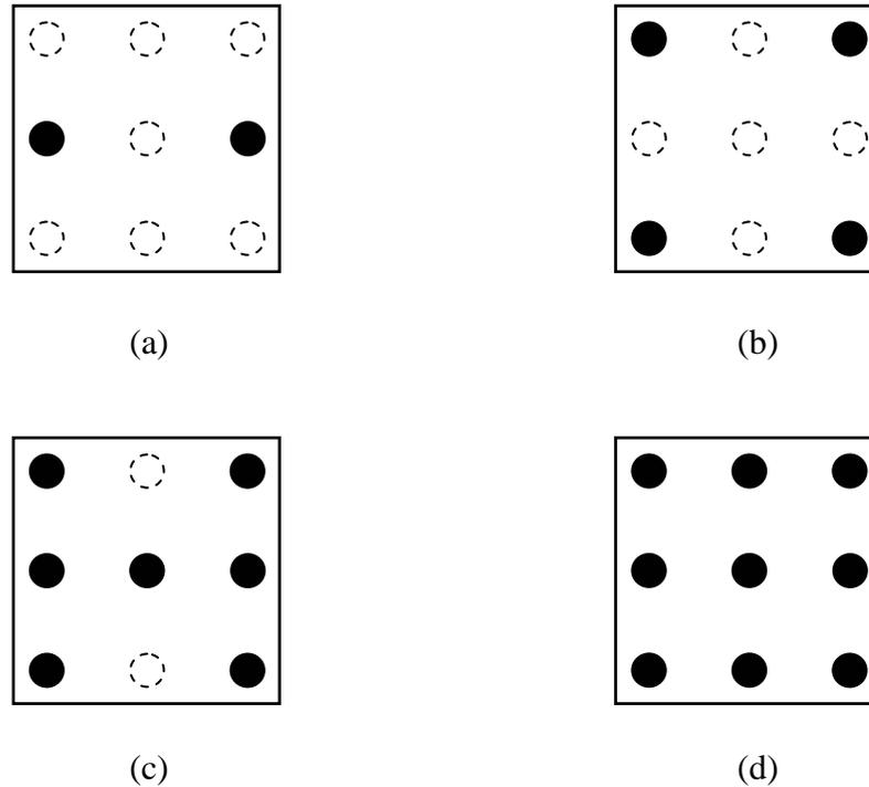
Figure 5.1 Model piled raft configurations: a) piled raft with 2 piles, b) piled raft with 4 piles, c) piled raft with 7 piles, d) piled raft with 9 piles
