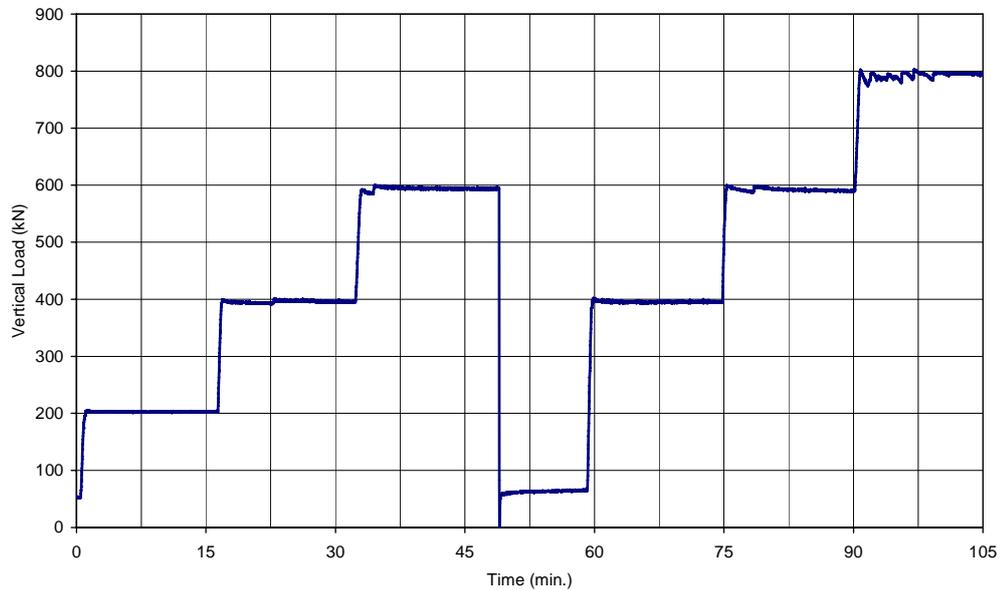
Figure 3.6 Vertical loading sequence of model piled raft foundation
