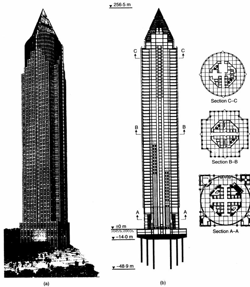
Figure 2.11 Messeturm building: a) elevation, b) cross-sections
