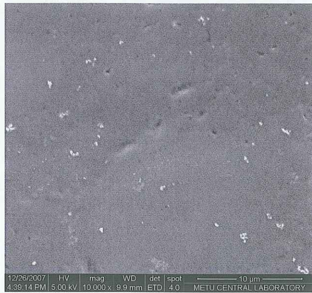
Figure 3.20 SEM image of surface area of wheat gluten film containing 1.6% TiO 2 .
