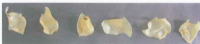
Figure 3.31 Films coated by the 1/2, 1/5, 1/10, 1/20, 1/50, 1/100 diluted \text{TiO}_2 solution from left to right.
