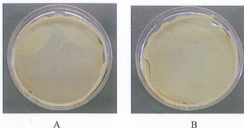
Figure 3.37 After drying of the wheat gluten films coated by the fifth method, pH adjusted to 11 by (A) KOH (B) NaOH.
