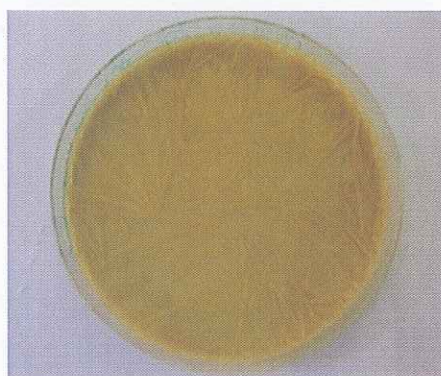
Figure 3.3 Photograph of film casted from cotton stalk xylan-lignin solution at pH 11 without removal of lignin and adjustment of pH.
