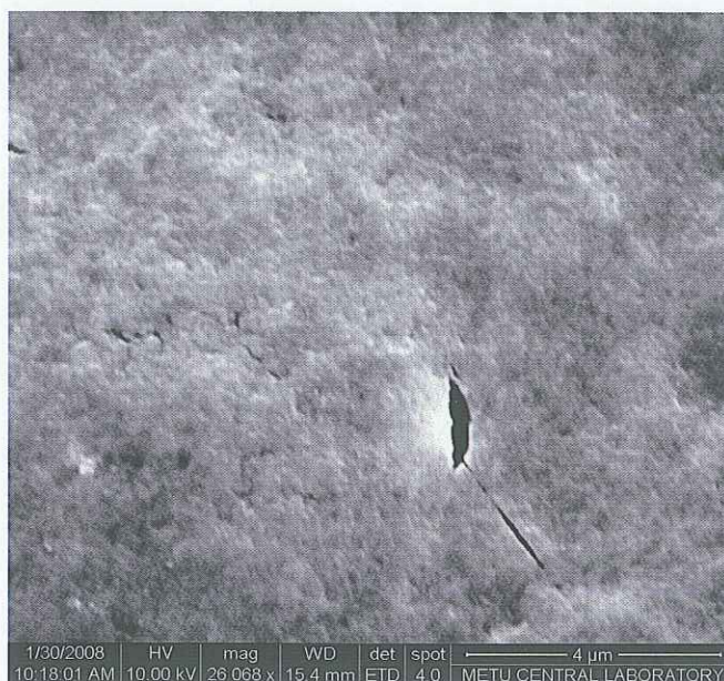
Figure 3.42 SEM image of the surface area of the procedure 5 coated wheat gluten film, which had pH adjustment by KOH.
