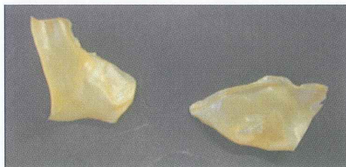
Figure 3.32 Wheat gluten film coated with third procedure.
