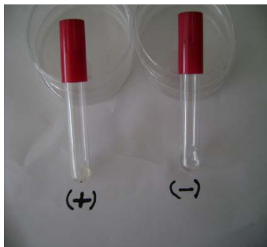
Figure E. 5: Coagulase test (Positive and Negative result)
