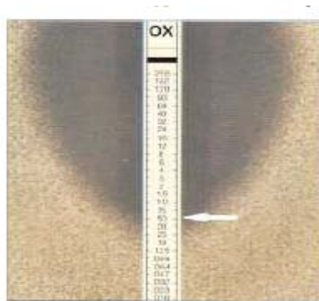
Figure 2.1 Susceptible strain. MIC 0.5 µg/ml.
