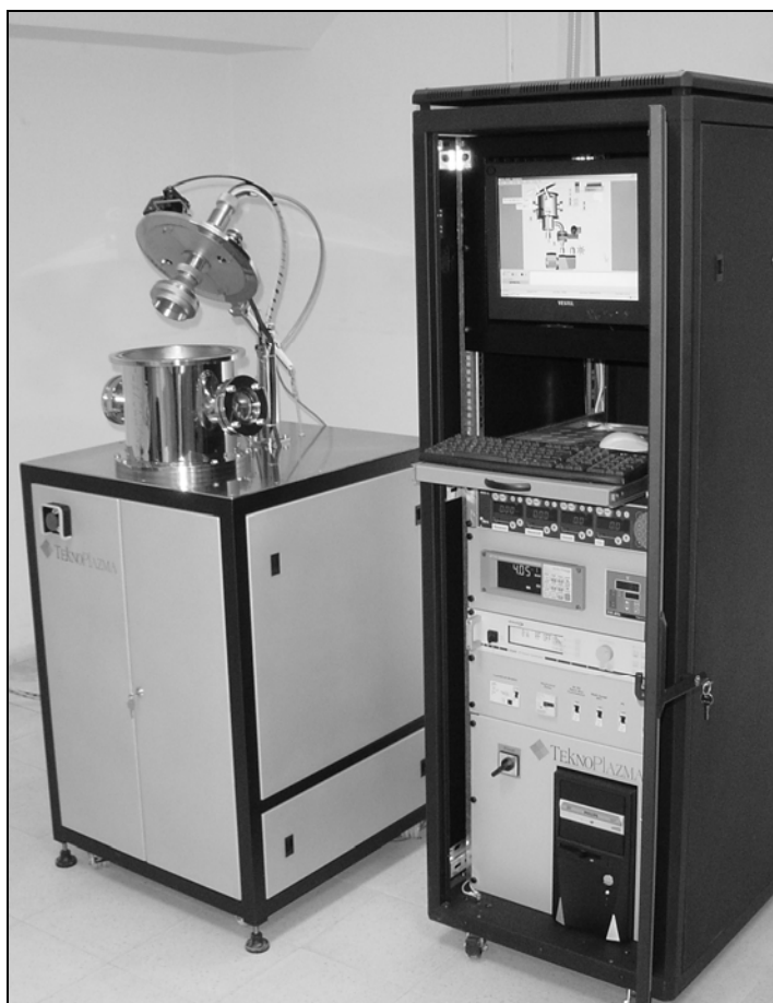
Figure 19 TPVD-300/PG System is in the course of diagnostic tests.
