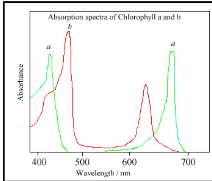
Figure 2.2 Absorption Spectra of Chlorophyll a and b (URL 9).
