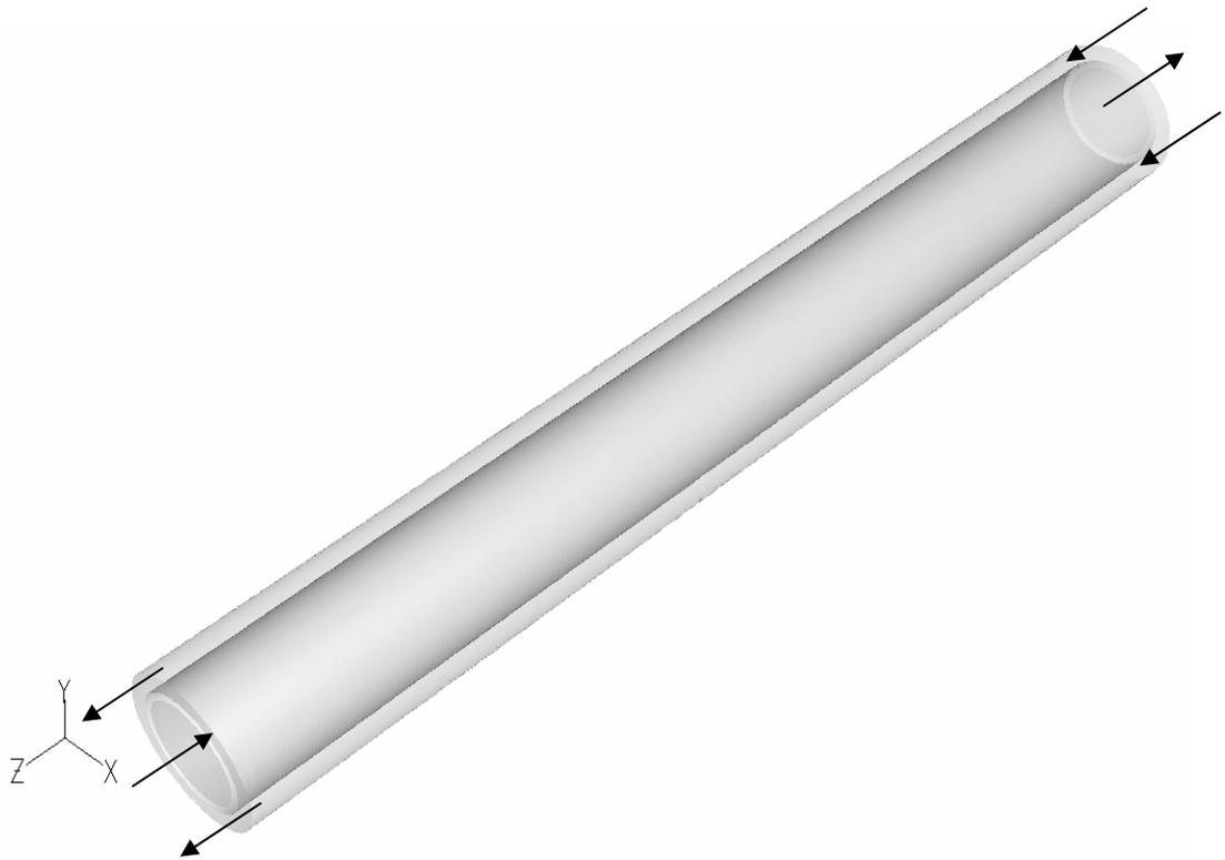
Figure 3-23 Double pipe heat exchanger without inlet nozzles
