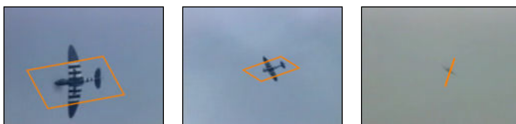
Figure 6.90 Test 2 LK – Air08 Sequence: Lucas-Kanade managed to track successfully until the 411 th frame which is shown on the right. The other two frames are the 52 nd (left) and 148 th (middle).
