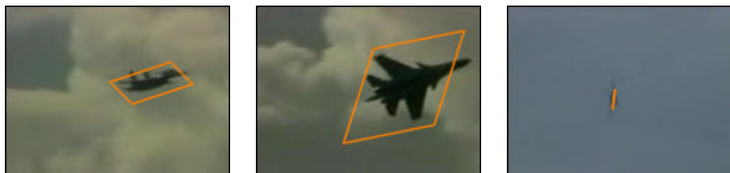
Figure 6.87 Test 1 LK – Air02 Sequence: Lucas-Kanade managed to track successfully until the 190 th frame which is shown on the right. The other two frames are the 25 th (left) and 67 th (middle).
