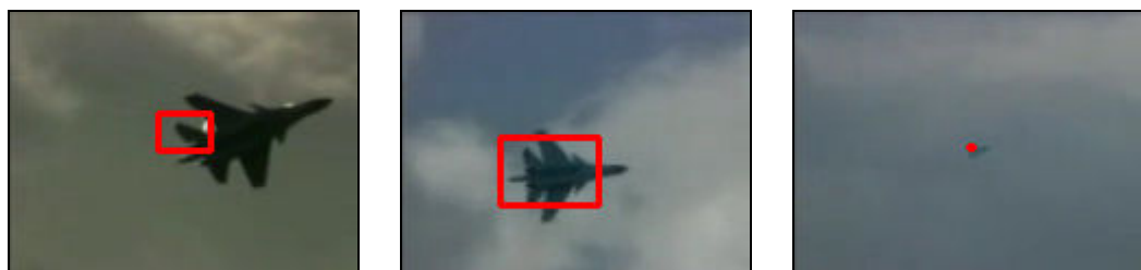
Figure 6.88 Test 1 MS – Air02 Sequence: The Mean Shift Tracker managed to track the target successfully until the last frame. Representative frames from the tracking sequence are shown, which are from left to right, the 59 th , 123 rd , and 681 st (last frame).
