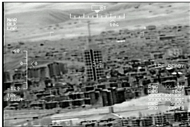
Figure 1.1 An example image of a typical Automatic Video Tracking System (AVTS). The target is maintained in the center of the field of view of the sensor. For this example, the source is an infrared imaging source mounted on an aircraft.
