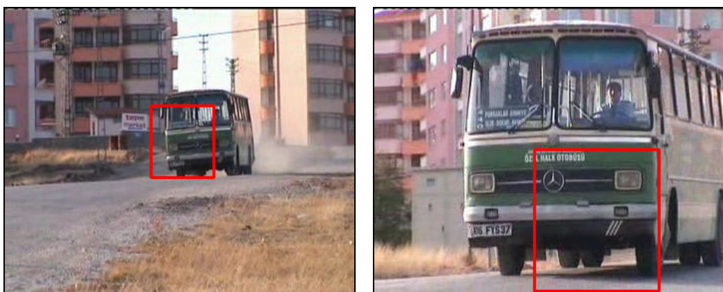
Figure 6.100 Test 5 MS – Pursaklar03 Color: The Mean Shift Tracker managed to track the target until the 208 th frame. It also had difficulties in maintaining the track gate on the target and updating the size accordingly. Representative frames from the tracking sequence are the 52 nd (left) and 208 th (right).
