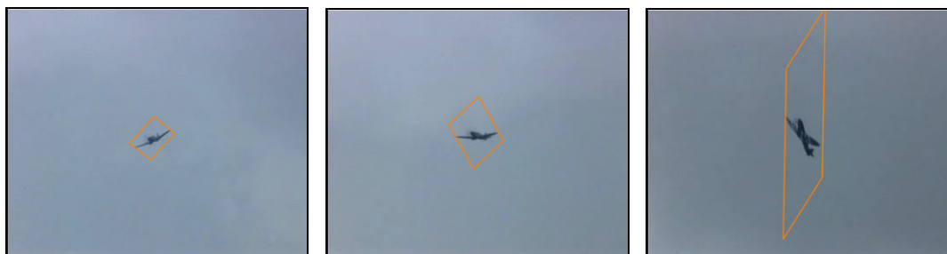
Figure 6.93 Test 3 LK – Air09 Sequence: Lucas-Kanade managed to track successfully until the 140 th frame which is shown in the middle. From then on the track gate started to grow more than necessary. The other two frames are the 102 nd (left), and 220 th (right).
