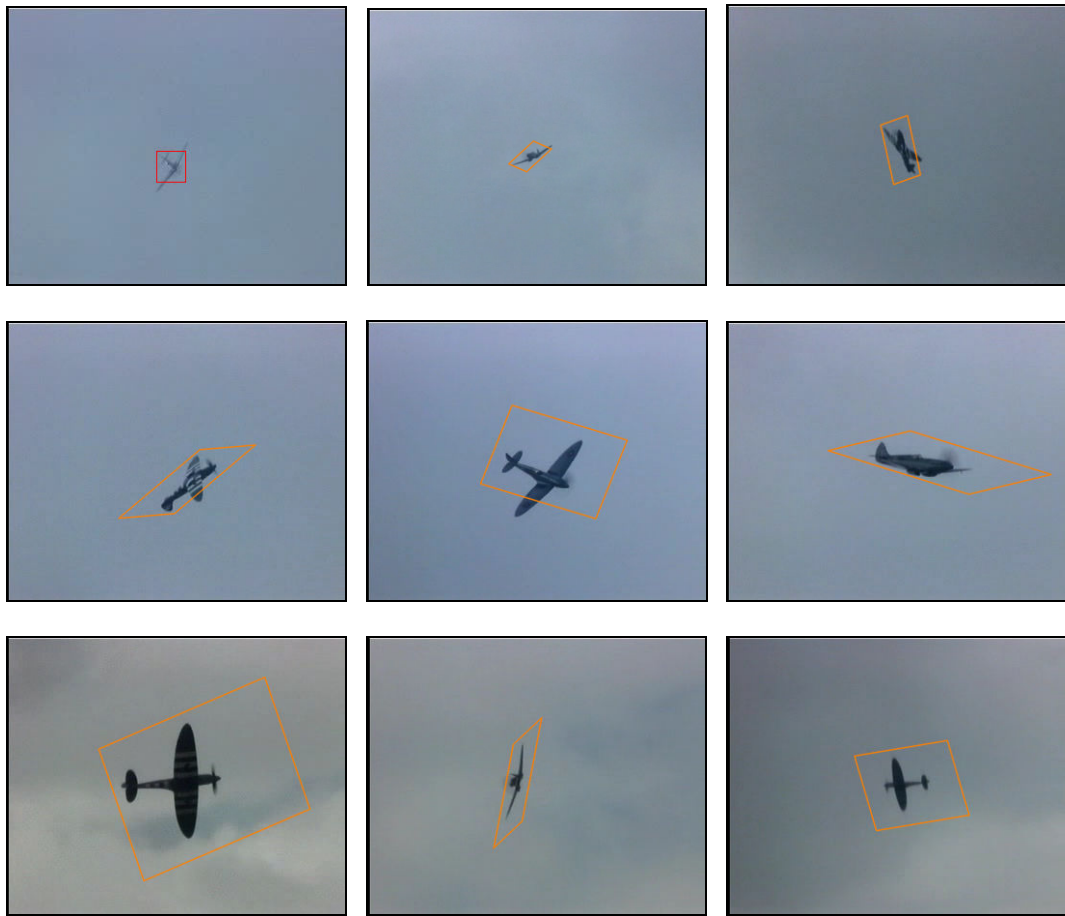
Figure 6.92 Test 3 CWT – Air09 Sequence: A total of 887 frames. The size of the target selected on the first frame (upper left) is 31 \times 33 pixels. The representative frames from left to right and top to bottom are 1 st , 102 nd , 220 th , 319 th , 478 th , 552 nd , 623 rd , 713 th , and 887 th . The target is tracked successfully until the last frame.
