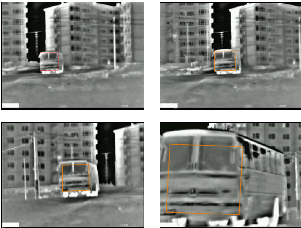
Figure 6.95 Test 4 CWT – Pursaklar03 Infrared: The tracking sequence is 269 frames. The representative frames show the 1 st , 42 nd , 138 th and 269 th (last) frame of the sequence.
