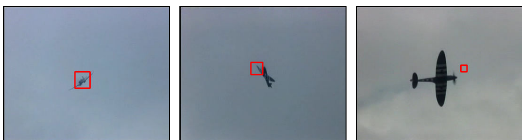
Figure 6.94 Test 3 MS – Air09 Sequence: The Mean Shift Tracker managed to track the target successfully until the 627 th frame which is shown on the right. Representative frames from the tracking sequence are shown, which are from left to right, the 70 th , 319 th , and 627 th (last frame).
