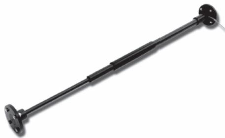
**Figure 5.9: Fill-extensometer**
