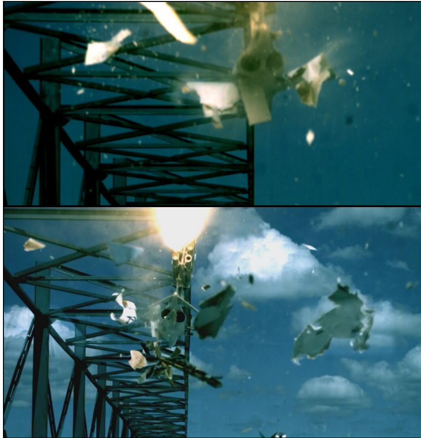
Figure 60 – A View of Failure of the Composite Aircraft Model
