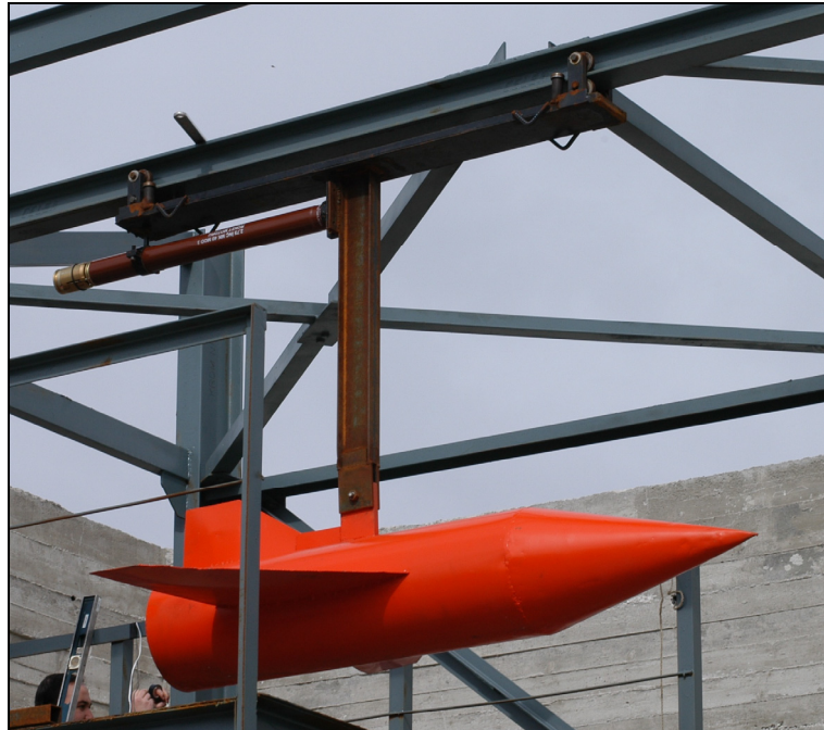
Figure 71 – Dummy Test Setup with R5 Rocket Engine
