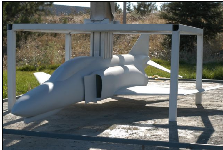
Figure 45 – A View of Composite Test Aircraft Model with Sting
