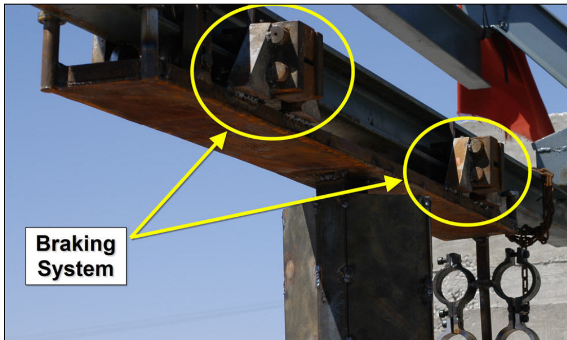
Figure 70 – A View of Installed Braking System
