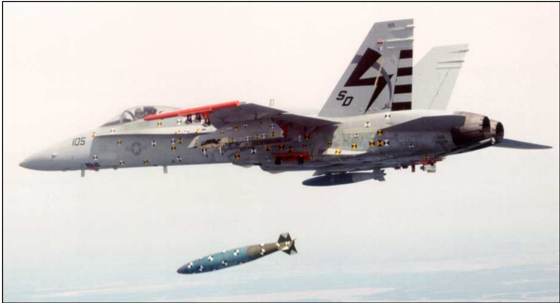
Figure 2 – A View of Separation of a Bomb from Aircraft in Flight Test
