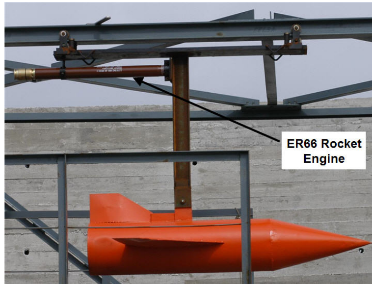
Figure 64 – R5 Installed on Conceptual Carriage
