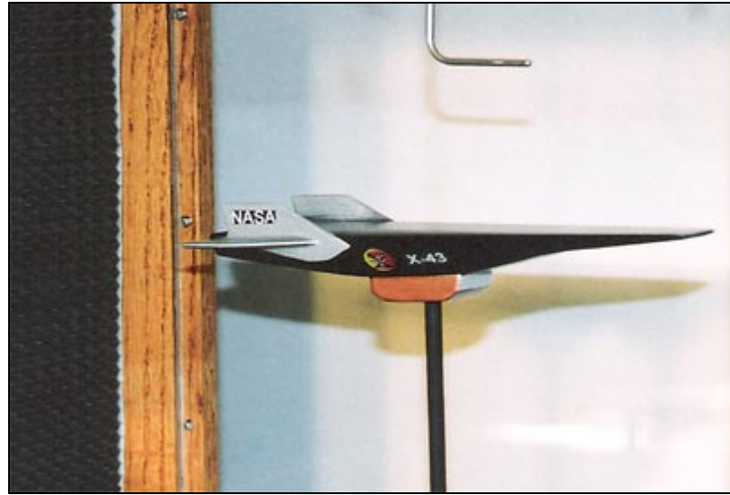
Figure 20 – A View of Sting Usage in a Wind Tunnel(Holding From Middle)
