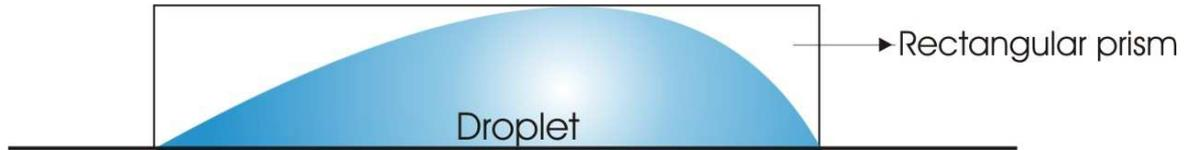
Fig. 4.8 Method used to calculate the mass of the droplet
