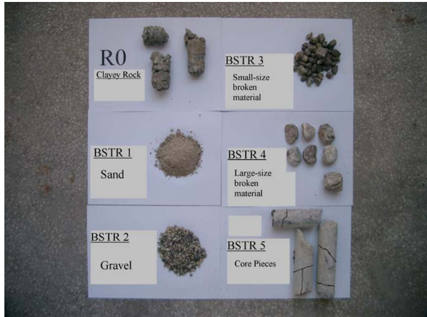
Figure 3-5 Various types of Broken Structural Domain (BSTR), METU's Rock Mechanics Laboratory
