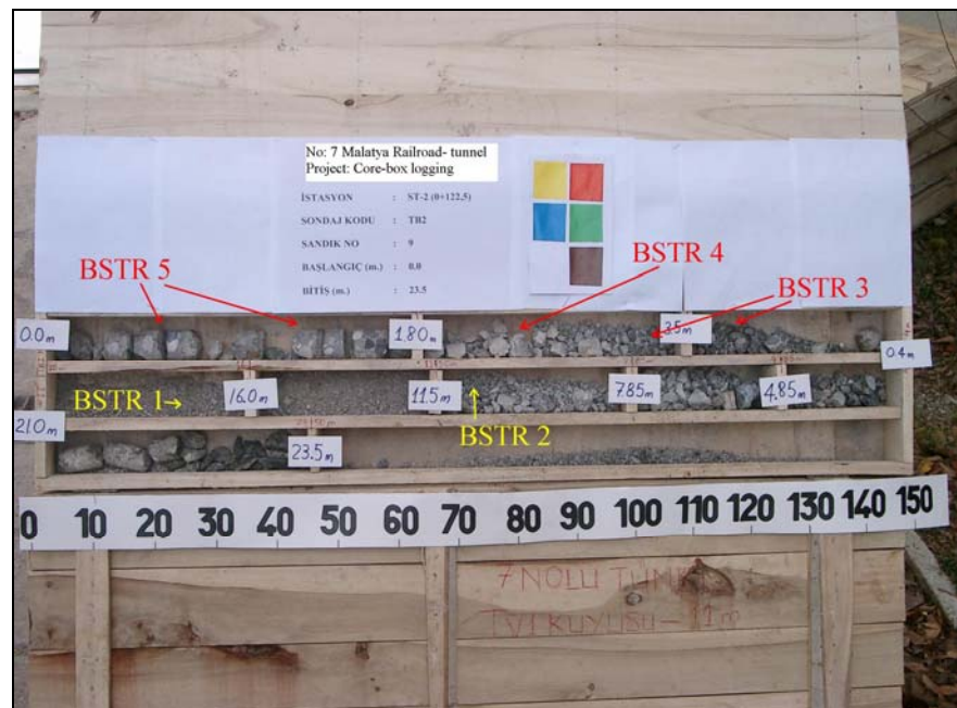
Figure 3-6 Core-box surveying for No:7 Malatya Railway tunnel project. Various types of BSTR are marked, METU's Rock Mechanics Laboratory, (Osgoui & Ünal, 2005b)
