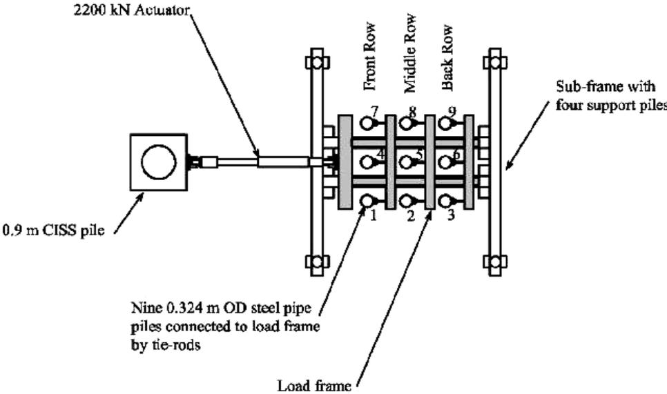
Figure 2.3. Lateral load test setup in the study of Rollins (2001)
