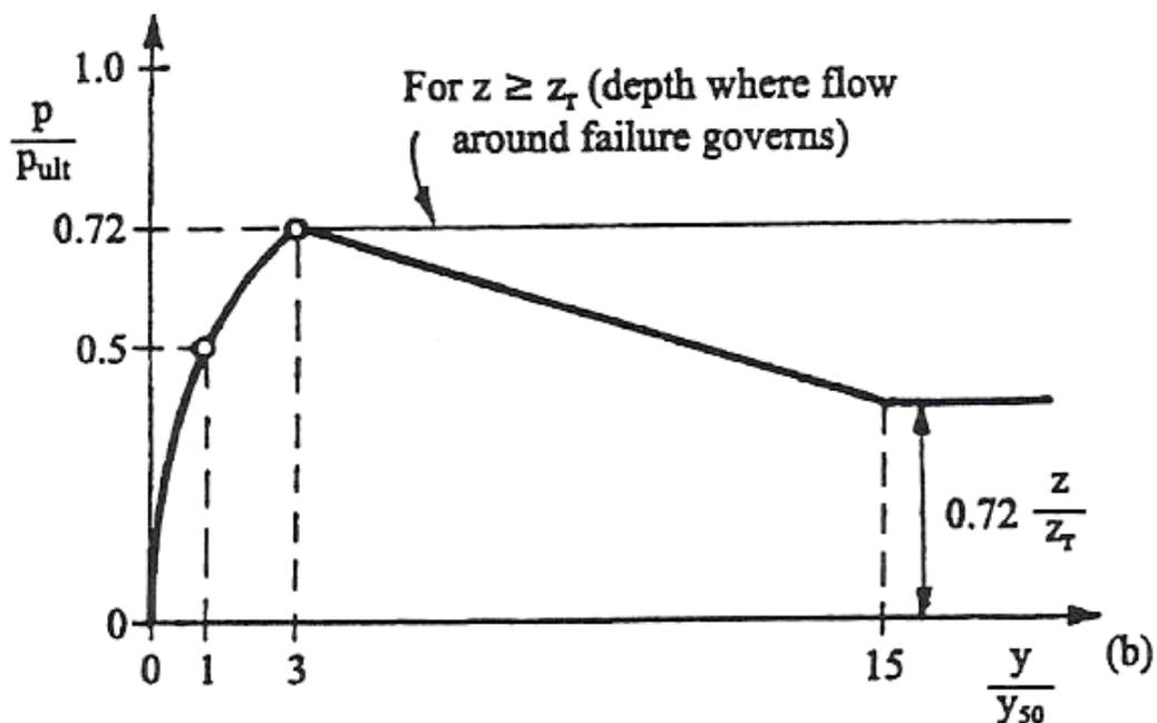
**Figure A-2:** Illustration of p-y curve for soft clay for cyclic loading
