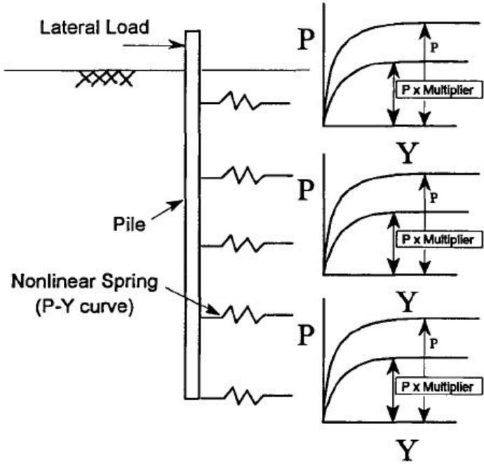
**Figure 2.6.** P-y multiplier approach for individual rows.
