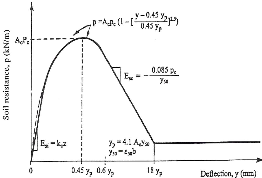
**Figure A-5:** Illustration of p-y curve for stiff clay for cyclic loading
