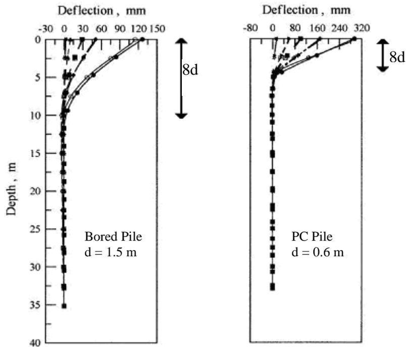
**Figure 2.9.** Depth of fixity depending on the pile diameter (Huang, 2001)
