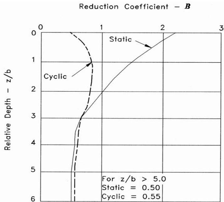
**Figure A-8:** Coefficient B for soil resistance vs depth (Reese et al., 1974)
