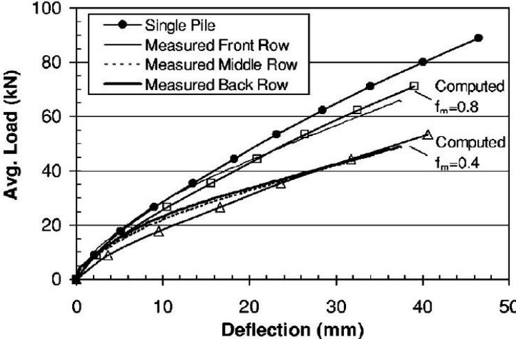
Figure 2.4. Average load – deflection curves for single pile and each row in the group (Rollins, 2001)
