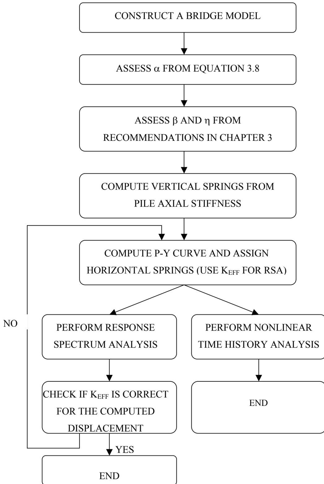
**Figure 4.6.** Algorithm for analysis
