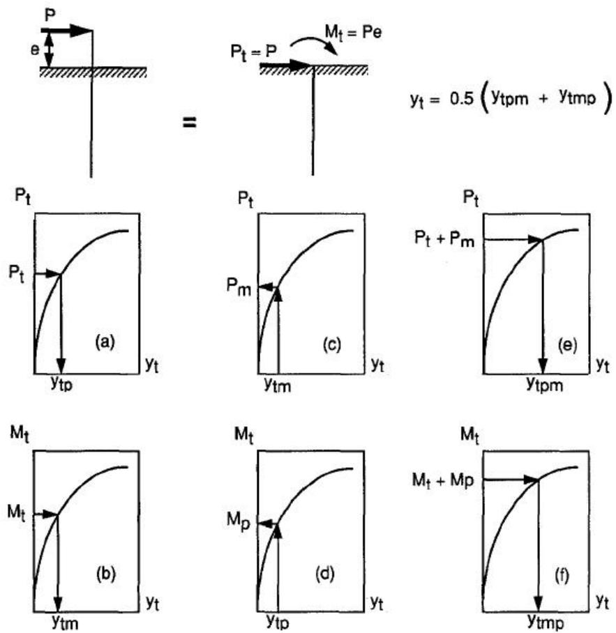
**Figure 2.10.** Nonlinear superposition procedure for a load applied above ground
