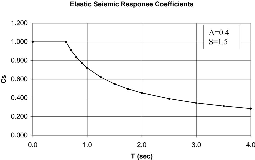
**Figure 4.7.** AASHTO response spectrum curve
