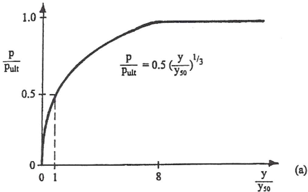
**Figure A-1:** Illustration of  $p$ - $y$  curve for soft clay for static loading (Matlock, 1970)
