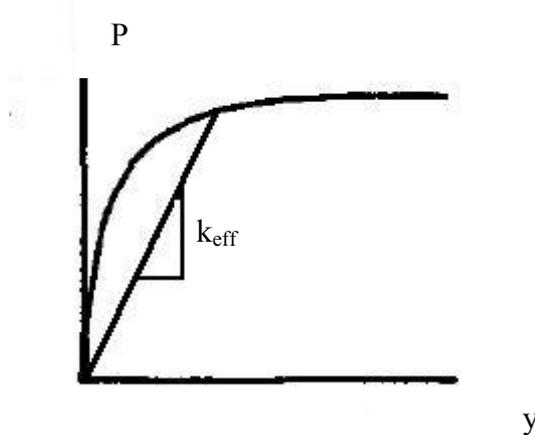
**Figure 4.1.** Spring stiffness for response spectrum analysis
