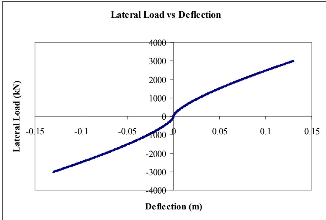
**Figure 3.4.** p-y curve computed by proposed method
