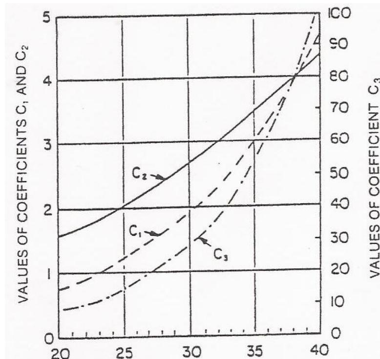
**Figure A-9:** Empirical constants for computation of ultimate bearing capacity (API, 1993)
