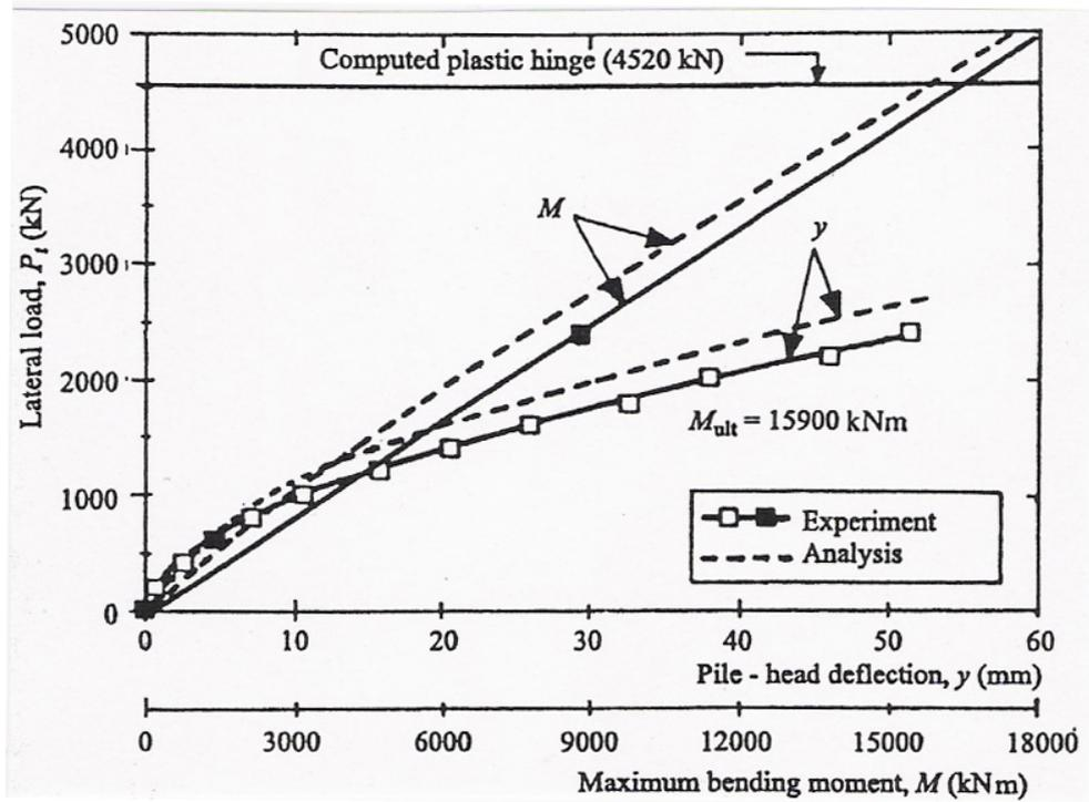
**B.9 Taiwan Test (Single Pile) (Huang et. al., 2001)**
