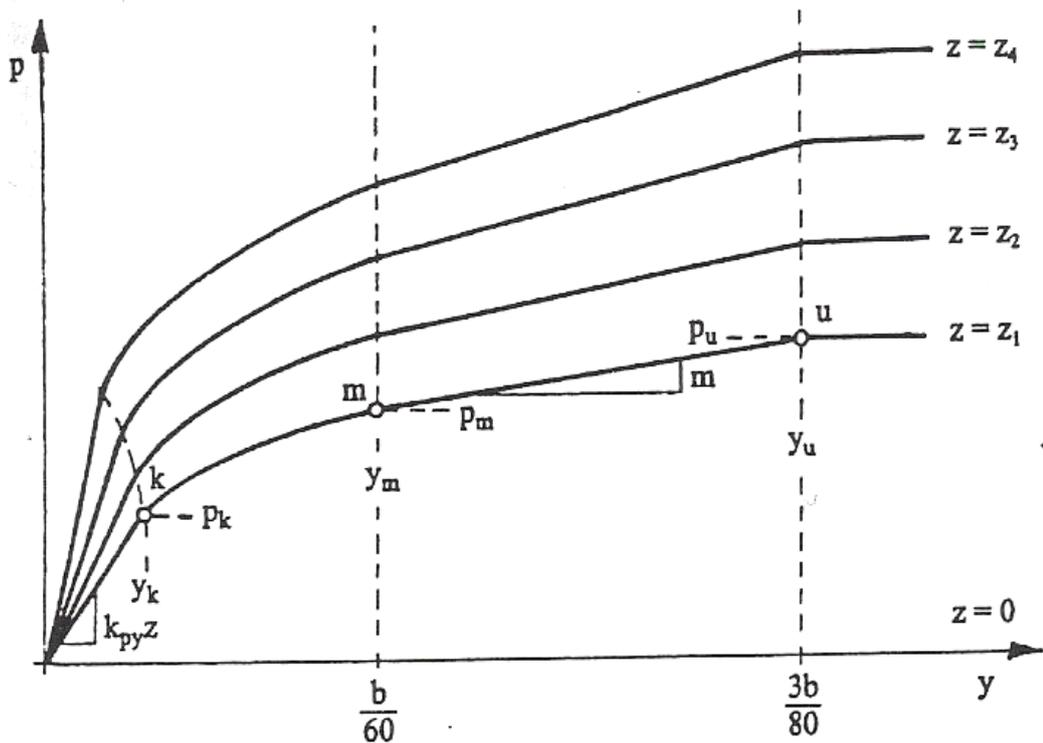
Figure A-6: Illustration of p-y curve for sands (Reese et al., 1974)
