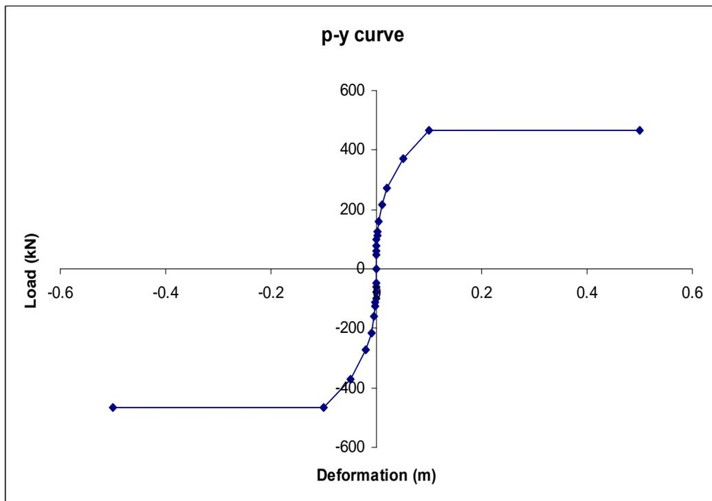
**Figure 4.9.** P-y curve at 3 m depth (Calculated by the method of Matlock (1970))
