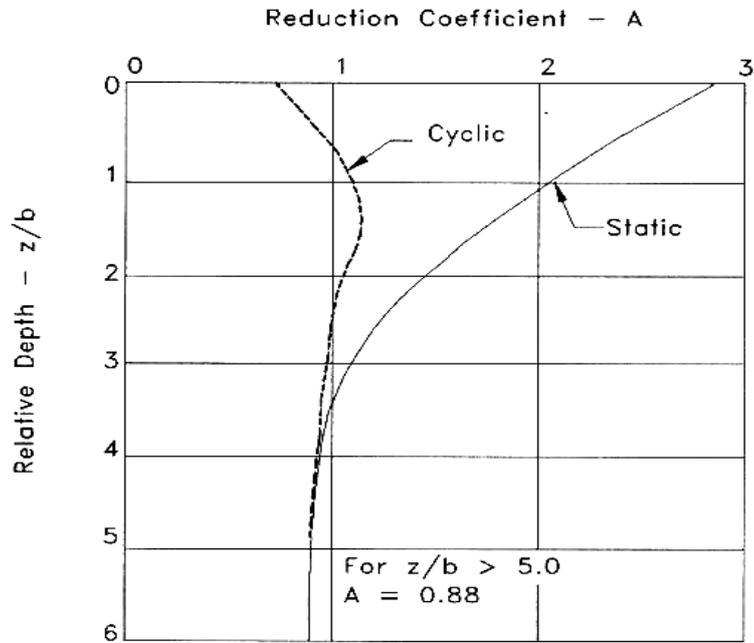
**Figure A-7:** Values of coefficients  $A_s$  and  $A_c$  (Reese et al., 1974)
