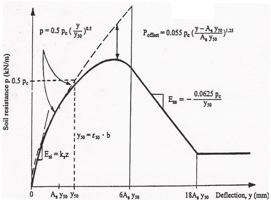
**Figure A-3:** Illustration of p-y curve for stiff clay for static loading
