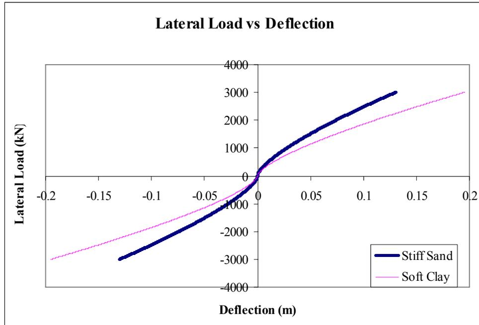
**Figure 3.5.** Illustration of the effect of soil type ( $\beta$  factor) for the proposed method
