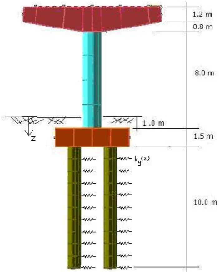
**Figure 4.4.** Pier elevation
