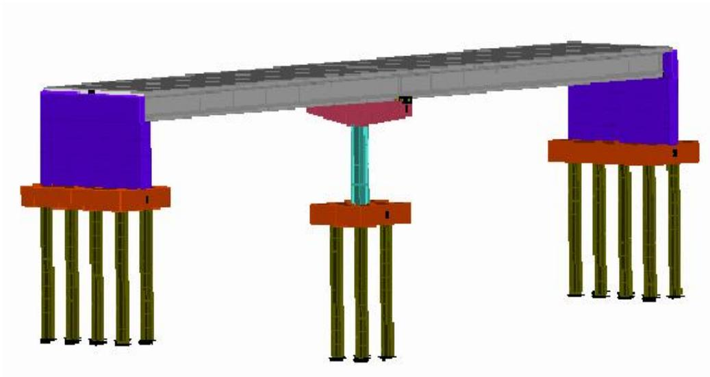
**Figure 4.2.** A sample bridge model with abutments
