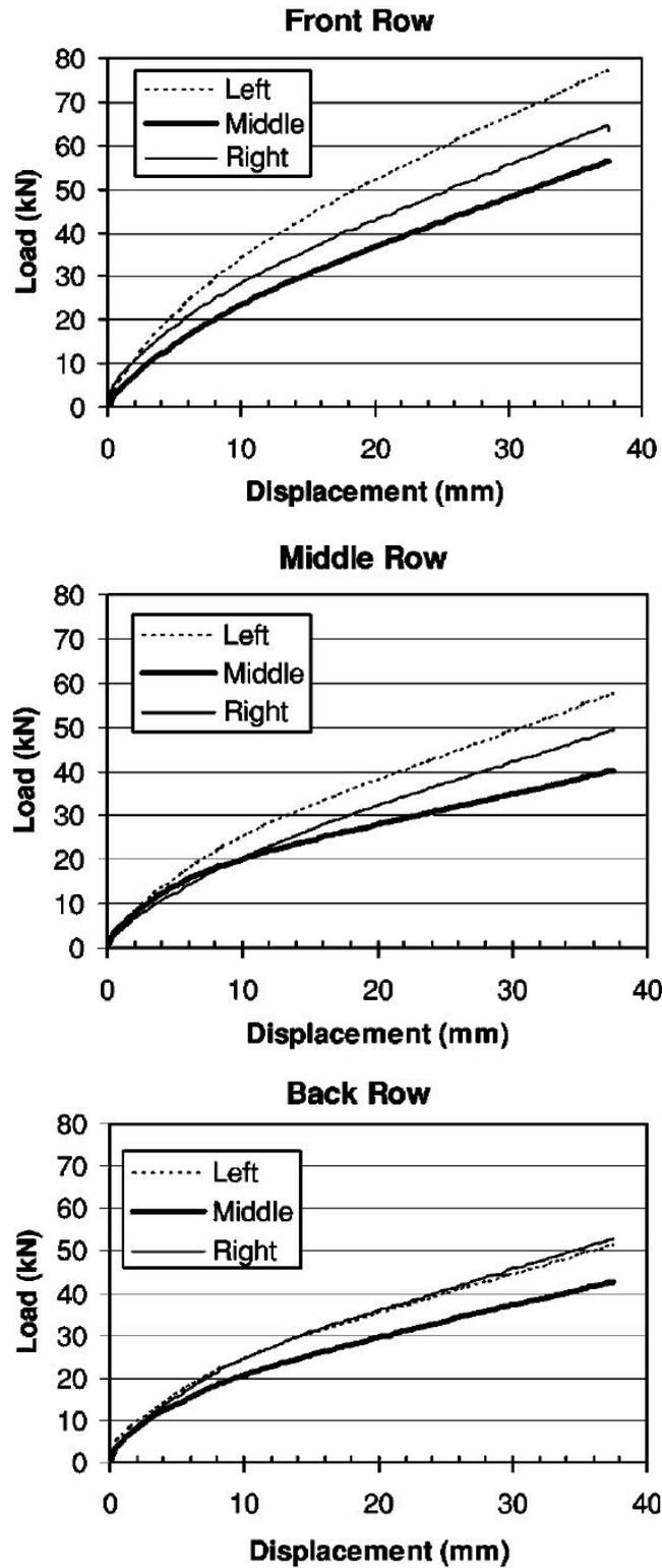
**Figure 2.5.** Measured load – deflection curves for left, middle and right piles in each row, Rollins (2001)
