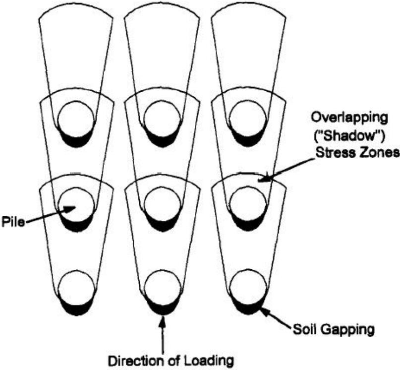
**Figure 2.2.** Schematic view of overlapping failure zones (Shadowing Effect) (Rollins, 1998)
