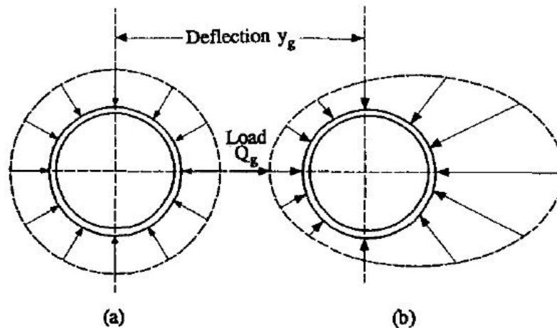
**Figure 2.7.** Distribution of soil reaction around a pile: a) before lateral load; b) after lateral load (Prakash & Kumar, 1996)
