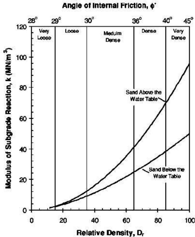
**Figure 2.1.** Recommendation for modulus of subgrade reaction for sands by API (1993)
