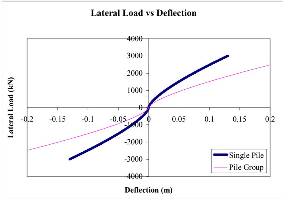
**Figure 3.6.** Illustration of the effect of group reduction ( $\eta$  factor) for the proposed method
