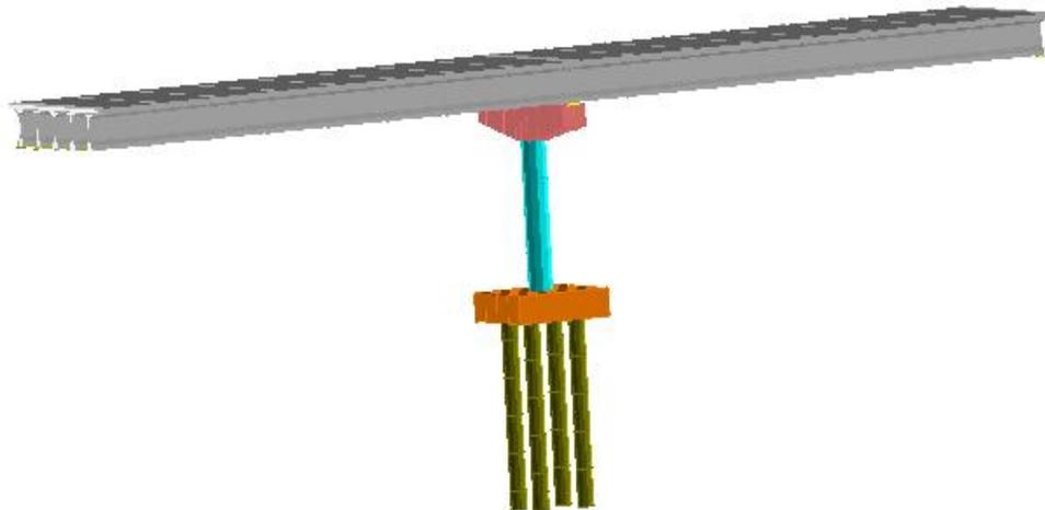
**Figure 4.3.** Bridge model with simplified abutment model
