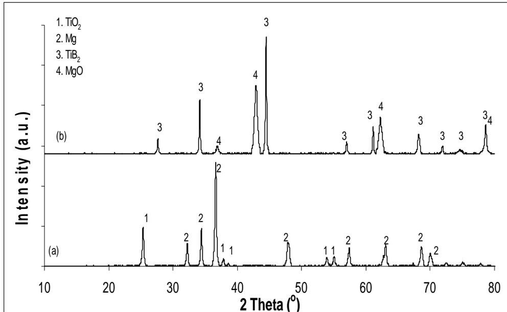
Fig.4.17 XRD pattern of (a) Sample ball milled for 5 hours, (b) Sample ball milled for 15 hours
