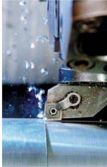
Fig.2.2 Metal tip coated with  $TiB_2$  while machining aluminum alloy [36]
