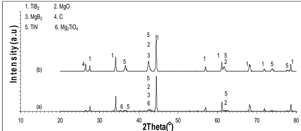
Fig.4.11 Effect of 40% excess Mg on the XRD patterns of leached samples. (a) Sample containing stoichiometric amount Mg after ignition, ball milling for 7 h in ethanol and leaching for 15 h in 1 M HCl, (b) Sample containing 40% excess Mg after ignition, ball milling and leaching with the same conditions
