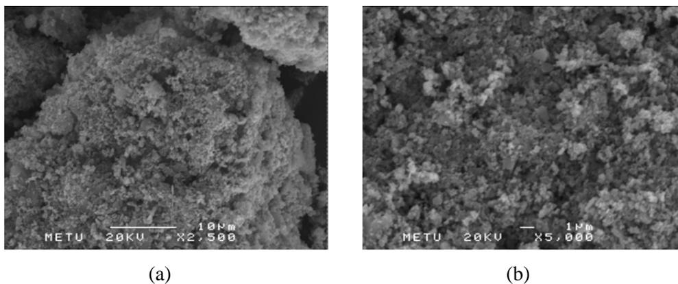
Fig.4.9 SEM micrographs of (a) Sample leached for 15 h in 1 M HCl after furnace ignition, (b) Sample furnace ignited, ball milled for 7 h with 150 rpm in ethanol and leached for 15 h in 1 M HCl
