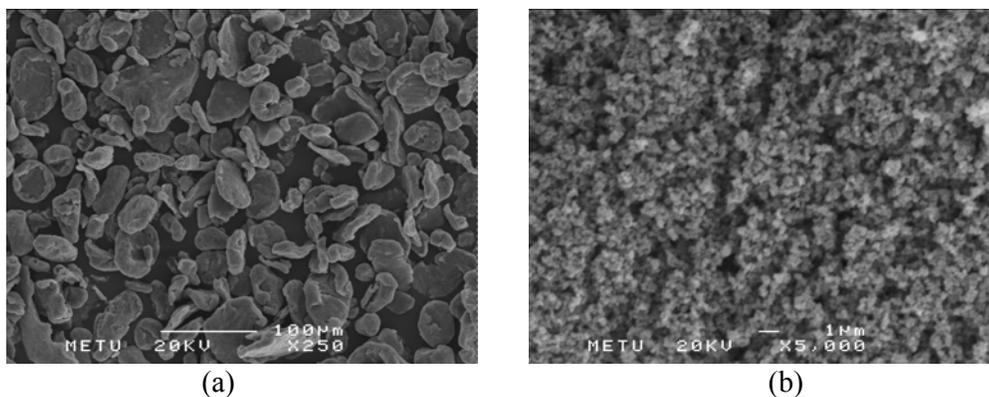
Fig.3.1 SEM micrographs of (a) Mg powder bought from Aldrich, (b) TiO<sub>2</sub> powder
