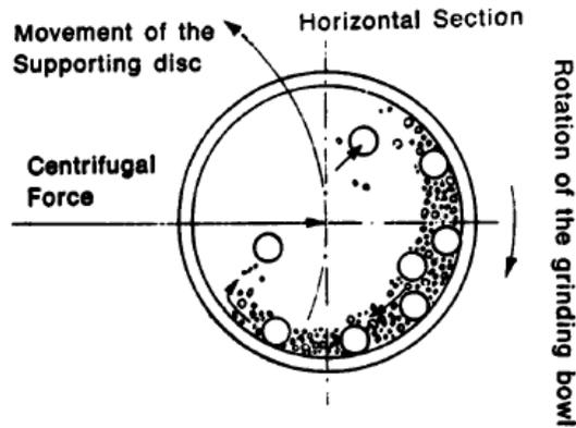
Fig.3.6 Ball motions in the planetary ball milling machine [73]
