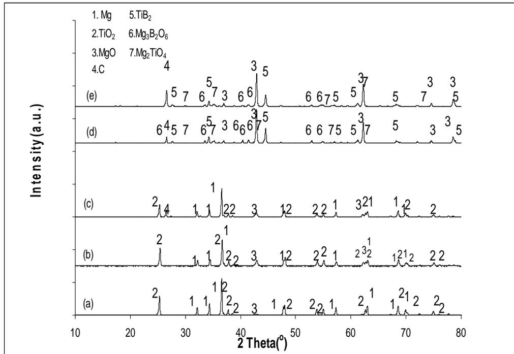
Fig.4.1 Effect of temperature on  $\text{TiB}_2$  production from  $\text{H}_3\text{BO}_3 + \text{Mg} + \text{TiO}_2$  mixtures (a) 600 °C, (b) 700 °C, (c) 725 °C, (d) 750 °C, (e) 800 °C
