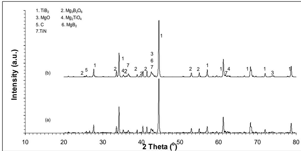
Fig.4.7 Effect of ball milling process performed after ignition (a) Sample ignited, leached for 15 h in 1M HCl, (b) Sample ignited, ball milled for 7 h and leached for 15 h in 1M HCl
