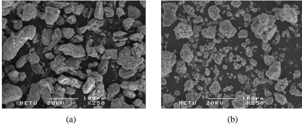
Fig.4.20 SEM micrographs of (a) Mg + TiO<sub>2</sub> + B<sub>2</sub>O<sub>3</sub> reactant mixture, (b) Mg + TiO<sub>2</sub> + B<sub>2</sub>O<sub>3</sub> reactant mixture after dry ball milling
