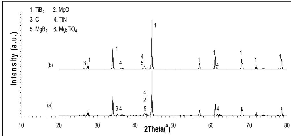
Fig.4.12 Effect of concentration of HCl on the leached products (a) Sample ignited, ball milled for 7 h in ethanol and leached for 15 h in 1 M HCl, (b) Sample ignited, ball milled for 7 h in ethanol and leached for 15 h in 3 M HCl
