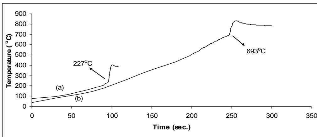
Fig.4.22 Ignition temperatures of (a) Ignited sample after ball milling, (b) Ignited sample without ball milling operation before ignition (plot (a) was shifted 50 °C up for clarity)
