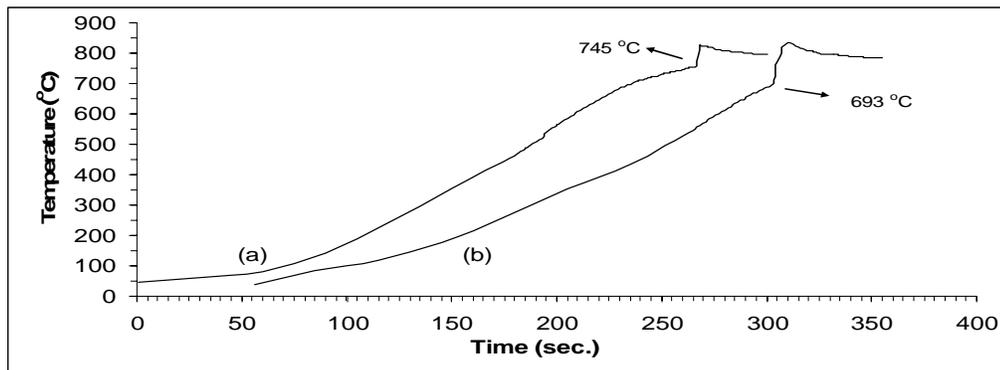
Fig.4.2 Effect of using (a) H<sub>3</sub>BO<sub>3</sub>, (b) B<sub>2</sub>O<sub>3</sub> on ignition temperature (plot (b) was shifted 55 seconds to right for clarity)
