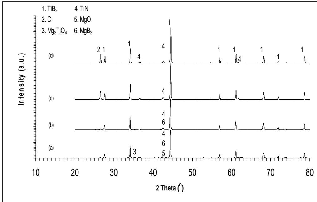
Fig.4.14 XRD pattern of sample ignited, ball milled for 7 h in ethanol, leached for 15 h in (a) 1 M HCl, (b) 3 M HCl, (c) 5 M HCl and (d) 7 M HCl
