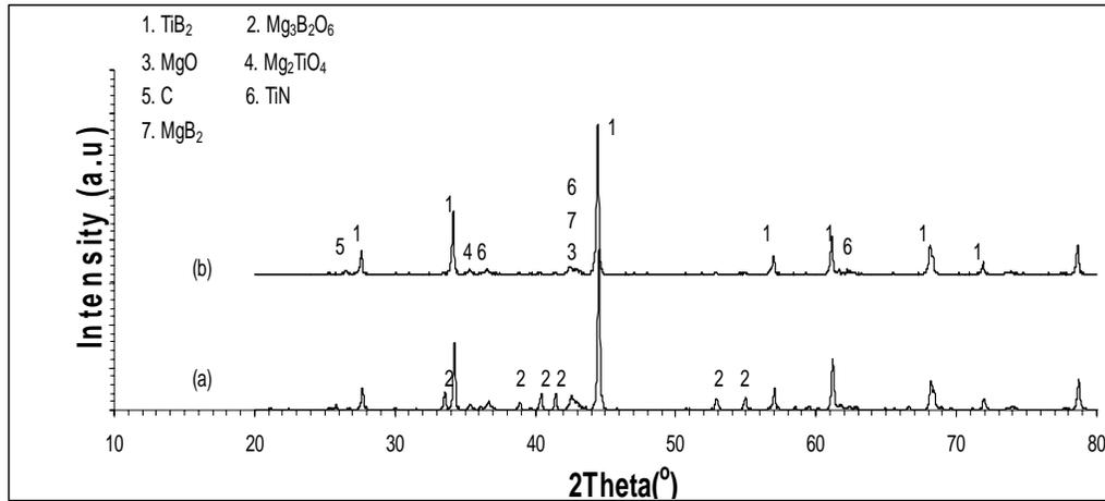
Fig.4.8 Effect of ball milling with ethanol medium after ignition (a) XRD of sample ignited, ball milled and leached in the 1M HCl, (b) Sample ball milled in ethanol, leached in the same condition with other sample after ignition again with the same conditions
