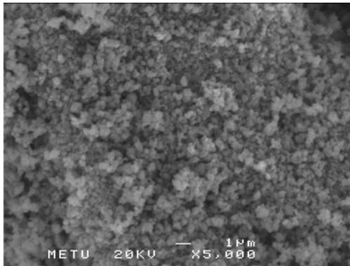
Fig.4.19 SEM micrograph of a MCP sample leached for 3 minutes
