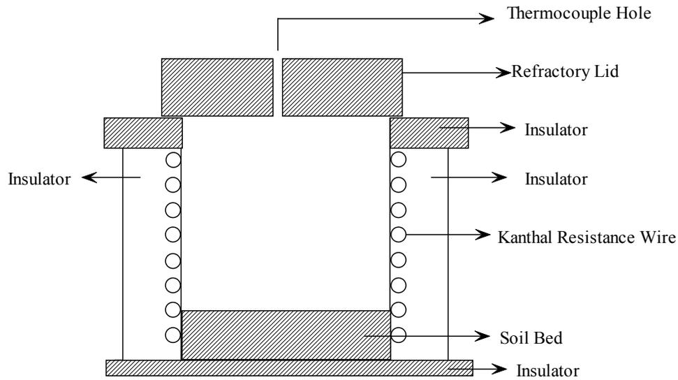
Fig.3.2 Pot furnace used during experiments.
