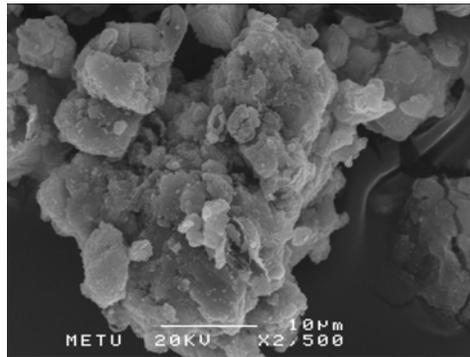
Fig.4.21 Structure of an agglomerate in the Mg + TiO<sub>2</sub> + B<sub>2</sub>O<sub>3</sub> reactant mixture after dry ball milling
