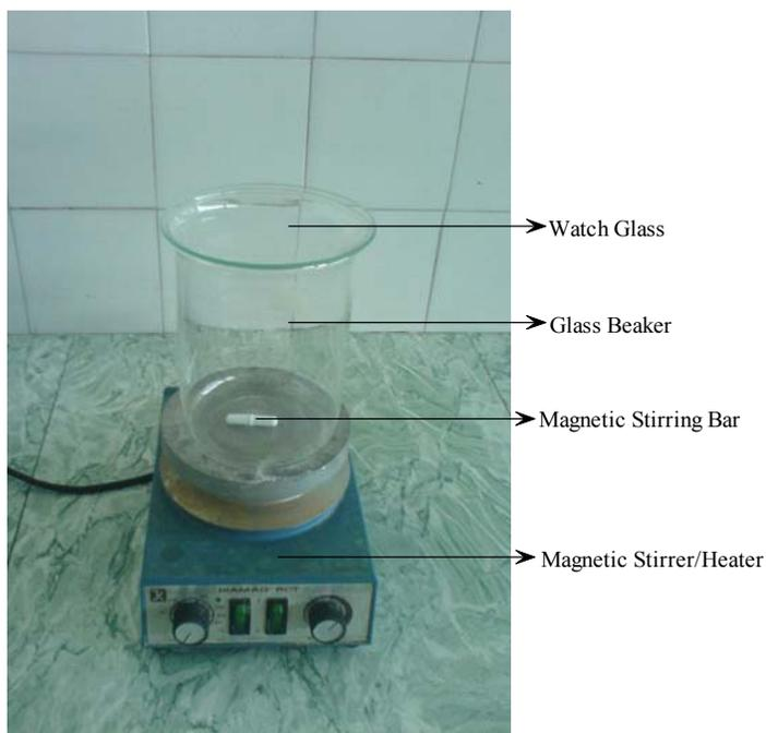
Fig.3.9 Experimental set-up of leaching without heating
