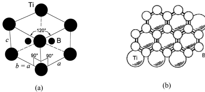
Fig.2.1 (a) The hexagonal unit cell of single crystal TiB<sub>2</sub>,  $a=b \neq c$ ,  $\alpha=\beta=90^\circ$ ,  $\gamma=120^\circ$
