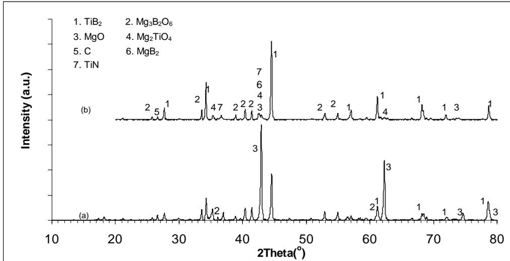
Fig.4.5 XRD pattern of (a) Sample ignited in furnace preheated to 800 °C, (b) Sample in (a) leached in the 1M HCl solution for 15 hours
