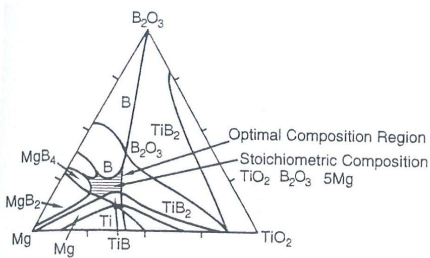
Fig.2.4 Diagram showing possible phases which can form in the system of  $\text{TiO}_2\text{-B}_2\text{O}_3\text{-Mg}$  [27]
