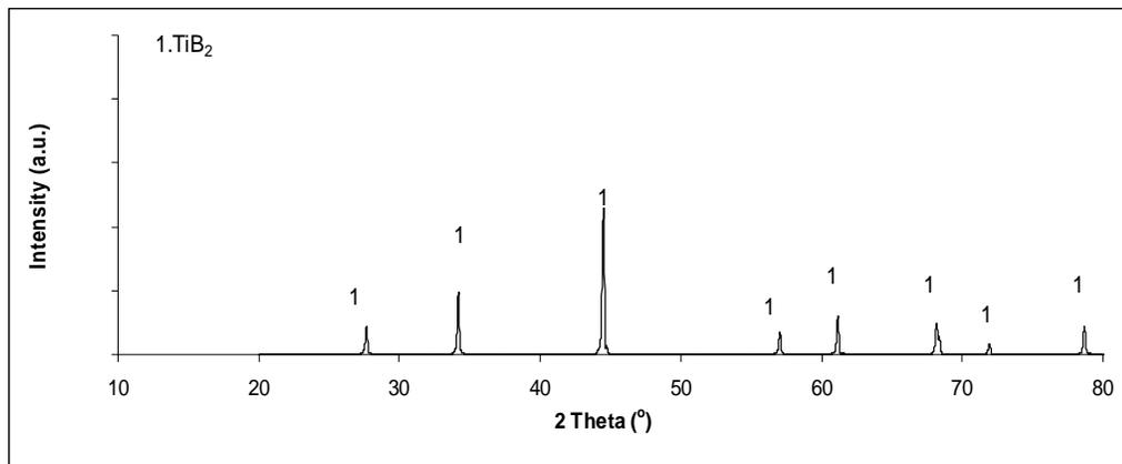
Fig.4.18 XRD pattern of sample ball milled for 15 hours and leached for 3 minutes in 0.5 M HCl solution
