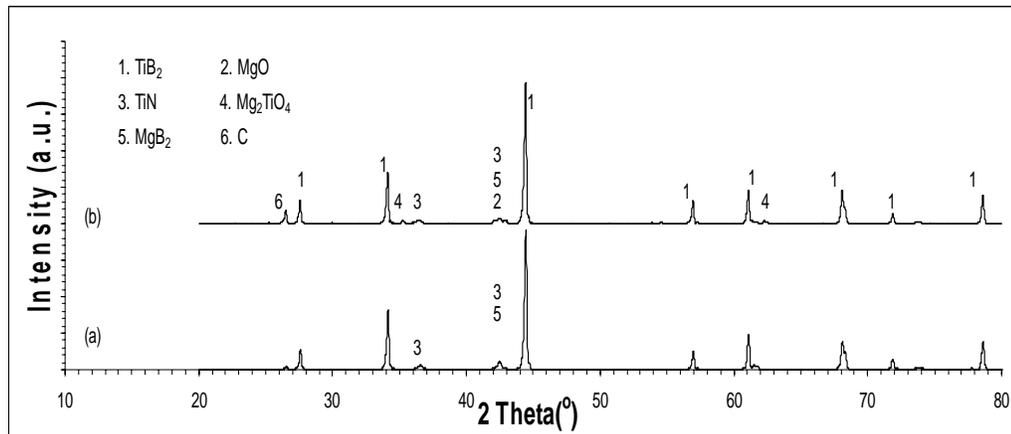
Fig.4.13 XRD pattern of (a) Sample ignited, ball milled for 7 h in ethanol and leached for 15 h in 3 M HCl, (b) Sample containing 10 % excess  $\text{TiO}_2$  and 20 % excess  $\text{B}_2\text{O}_3$  after ignition, ball milling for 7 h in ethanol and leached for 15 h in 3 M HCl
