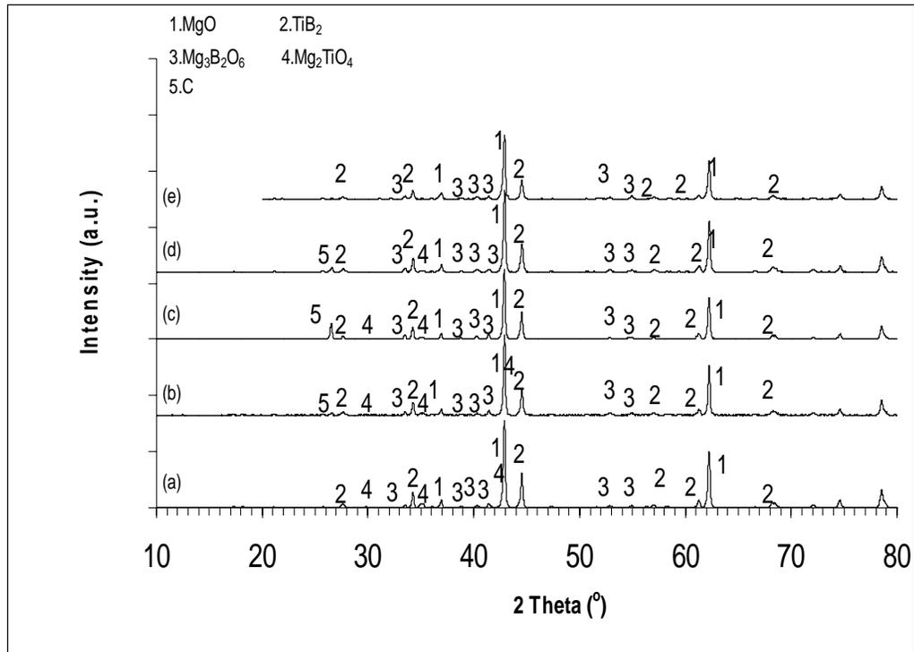
Fig.4.3 Effect of excess Mg addition on minor phases (a) Stoichiometric amount Mg, (b) 10% excess Mg, (c) 20% excess Mg, (d) 30% excess Mg, (e) 40% excess Mg
