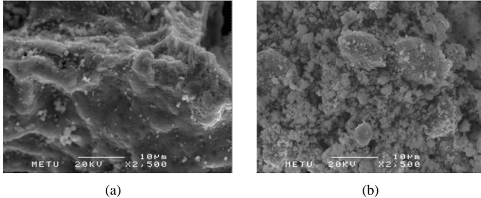
Fig.4.6 SEM micrographs of (a) Sample ignited in the furnace preheated to 800 °C, (b) Sample dry ball milled for 7 h with 150 rpm after ignition in the same conditions
