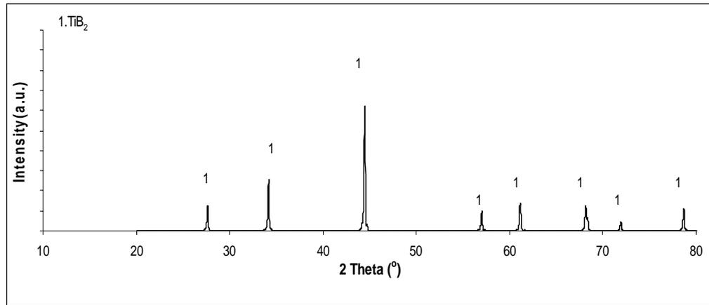
Fig.4.15 XRD pattern of sample ignited under argon atmosphere, ball milled in the ethanol medium and leached in 5 M HCl solution
