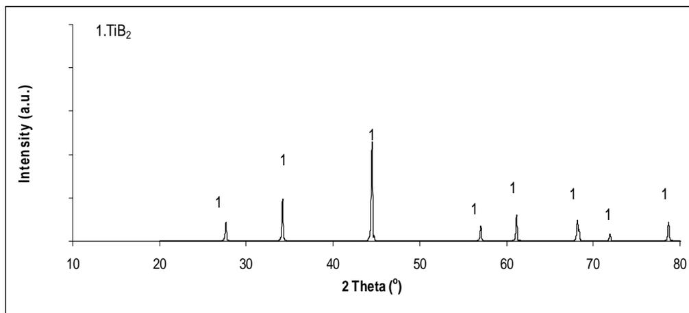
Fig.4.16 XRD pattern of sample ignited in argon and leached in 5 M HCl for 15 hours at 75 °C
