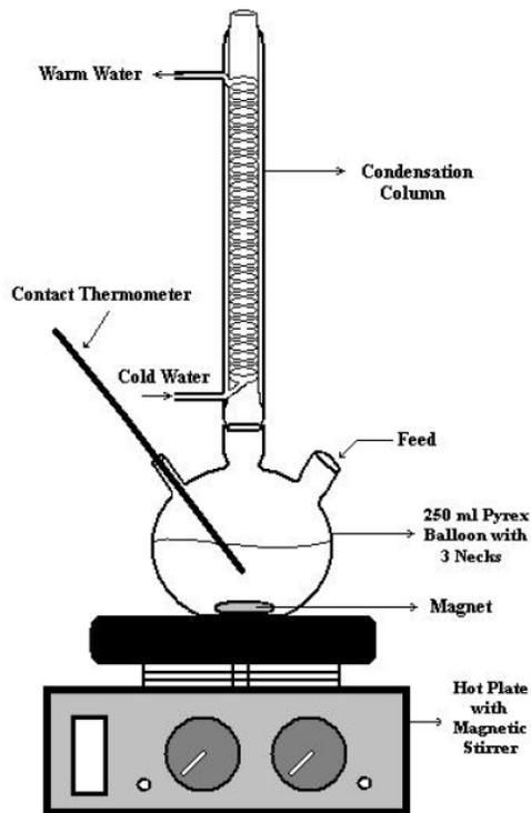
Fig.3.11 Experimental set-up of leaching with heating
