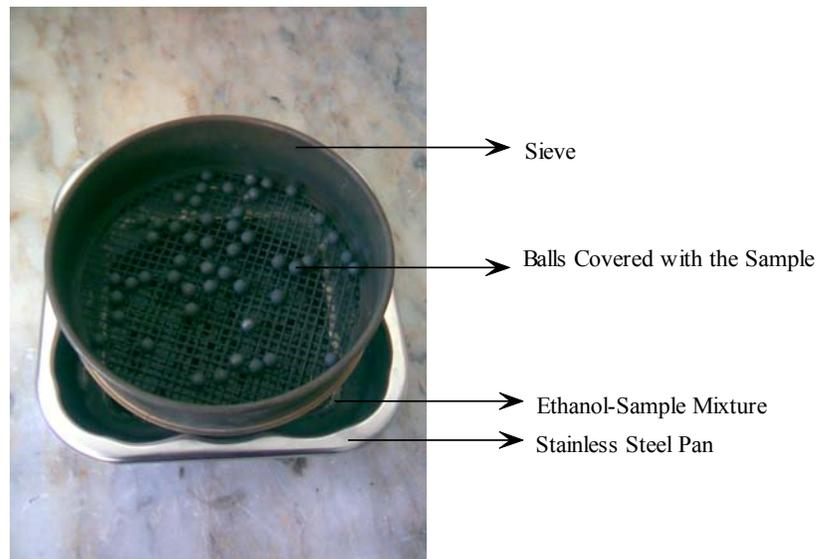
Fig.3.8 Sieve, pan, and balls after ethanol ball milling
