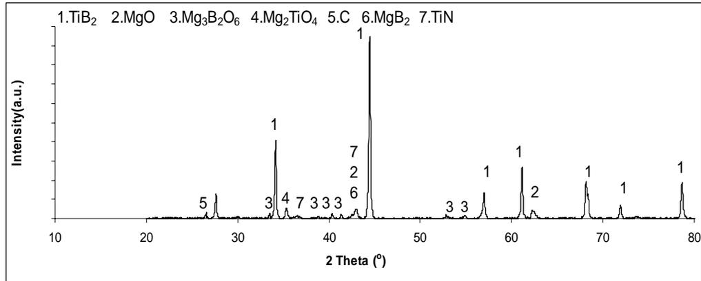
Fig.4.23 XRD pattern of the sample ball milled for 5 h, ignited in air at 800 °C and leached in 1 M HCl for 15 h at room temperature
