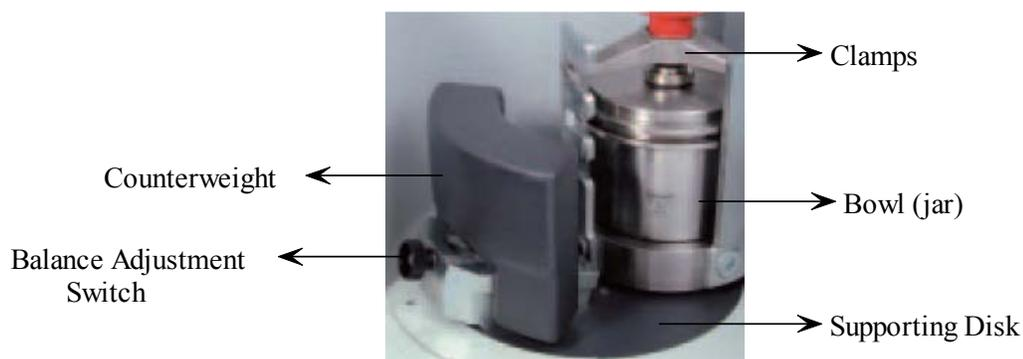
Fig.3.7 Balance adjustment [76]
