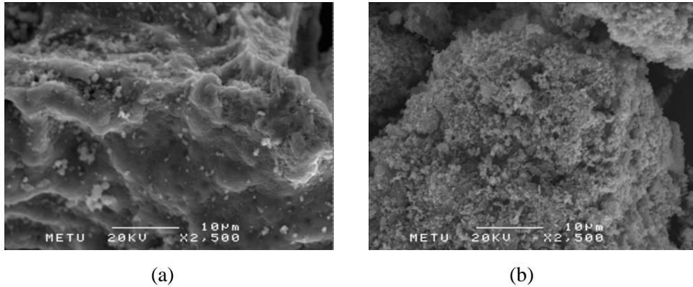
Fig.4.4 SEM micrographs of (a) Ignited sample in the furnace preheated to 800 °C, (b) Sample leached for 15 hours in the 1M HCl solution after ignition
