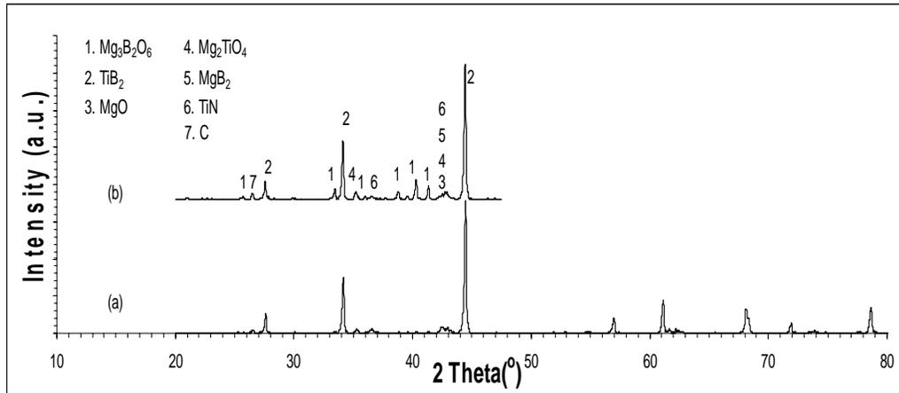
Fig.4.10 (a) Sample ignited, ball milled in ethanol and leached in the 1M HCl for 15 h, (b) Sample ignited, stirred in ethanol, filtered, leached 1 M HCl for 15 h
