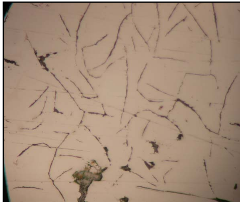
Figure 4.6 Microstructure of specimen, with 4Ae code, Treated with FeSiMg-Cermish metal, Mg/S: 2, Section size: 10 mm, A type FG, Magnification \times 500 ,
