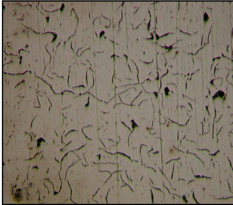
Figure 4.3 Microstructure of specimen, with 1Af code, Treated with FeSiMg-Cermish metal, Mg/S: 0.5, Section size: 20 mm, A type FG, Magnification \times 100 ,
