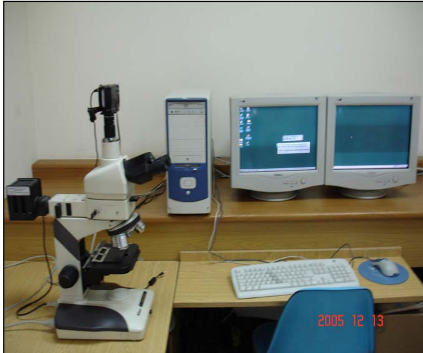
Figure 3.6. CLEMEX image analyzer system.
