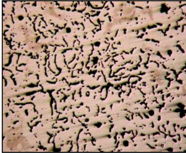
Figure 4.29 Microstructure of specimen, with 7Bf code, Treated with FeSiMg, Mg/S:5.3, Section size: 20 mm, 98.6 % CG, Magnification \times 100 ,
