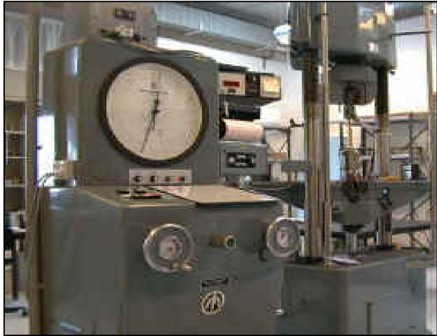
Figure 3.10 ALSA universal testing machine used for tensile test
