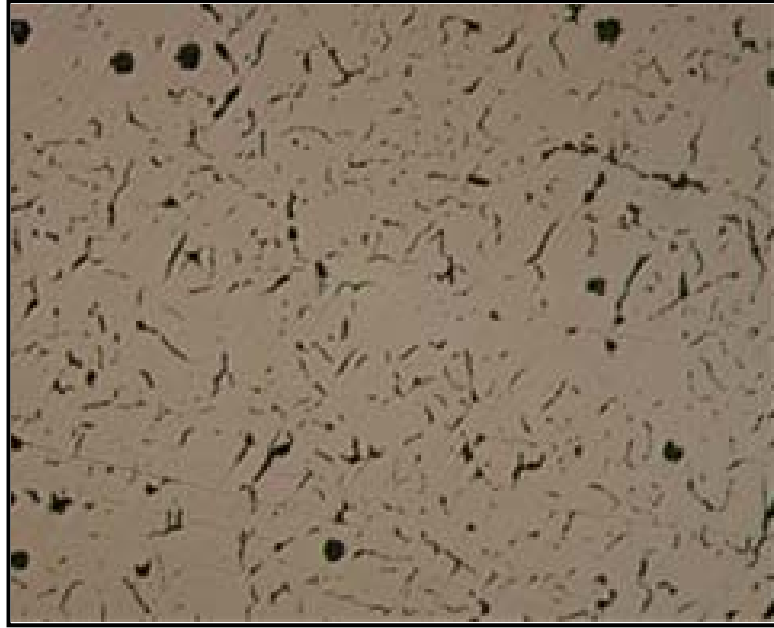
Figure 4.19 Microstructure of specimen, with 5Bf code, Treated with FeSiMg, Mg/S: 3, Section size: 20mm, 99.5% CG Magnification \times 100 ,
