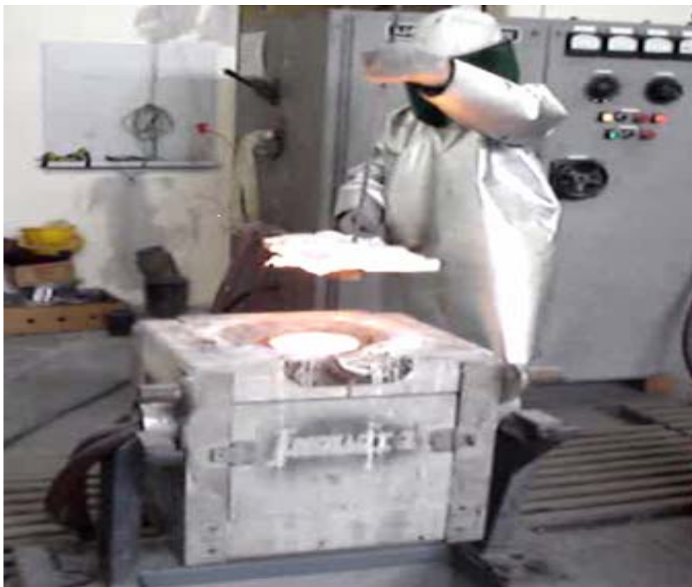
Figure 3.3 Plunger method used for CG iron production
