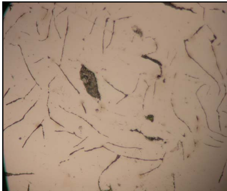
Figure 4.8 Microstructure of specimen, with 4Ag code, Treated with FeSiMg-Cermish metal, Mg/S: 2, Section size: 20 mm, A type FG, Magnification \times 500 ,
