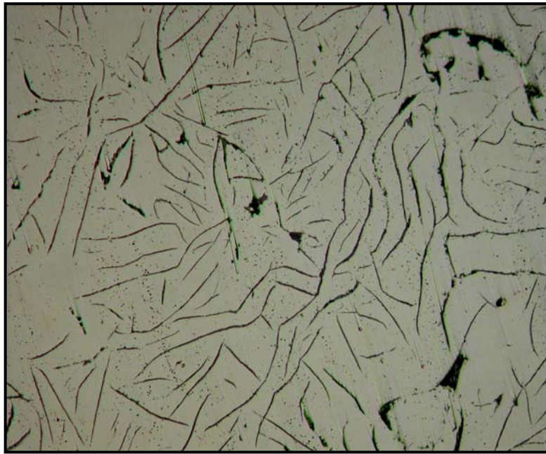
Figure 4.9 Microstructure of specimen, with 4Bd code, Treated with FeSiMg, Mg/S: 2, Section size: 5 mm, A type FG, Magnification \times 500 ,
