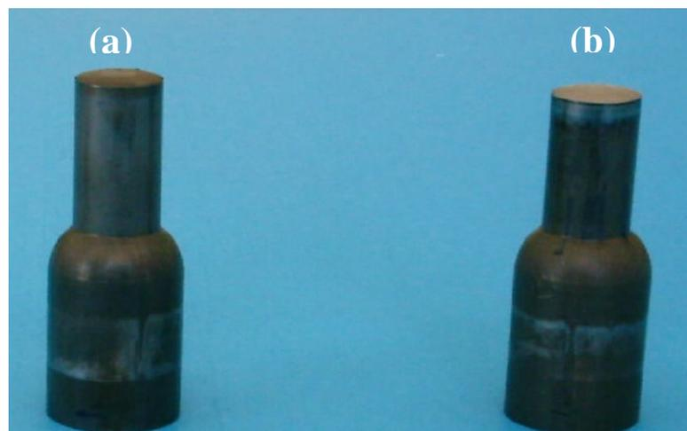
**Figure 5.44.** Extruded specimens **a)** Phosphate and soap layer on the shear surface **b)** Shiny surface at the tip of the specimen means this region had exposed to high friction [75]
