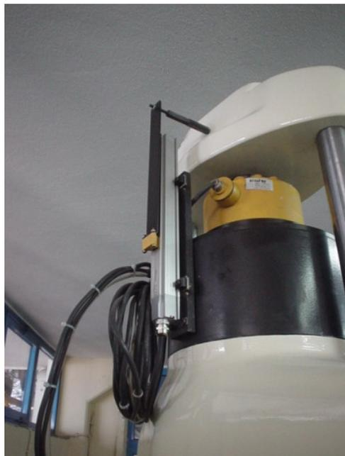
**Figure 4.4.** 40 tons tensile test machine (*left*), Displacement sensor (*right*)
