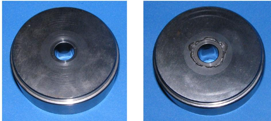
**Figure 4.78.** Unused (*left*) and failed (*right*) second
