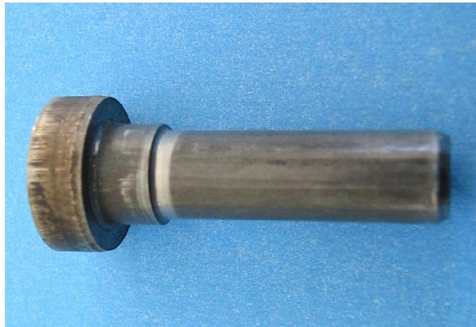
**Figure 4.57.** M10 Cylinder head stepped bolt
