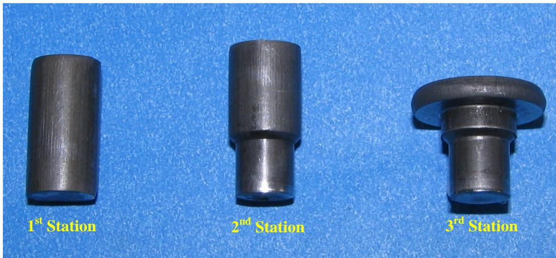
**Figure 4.75.** Forged parts in each station
