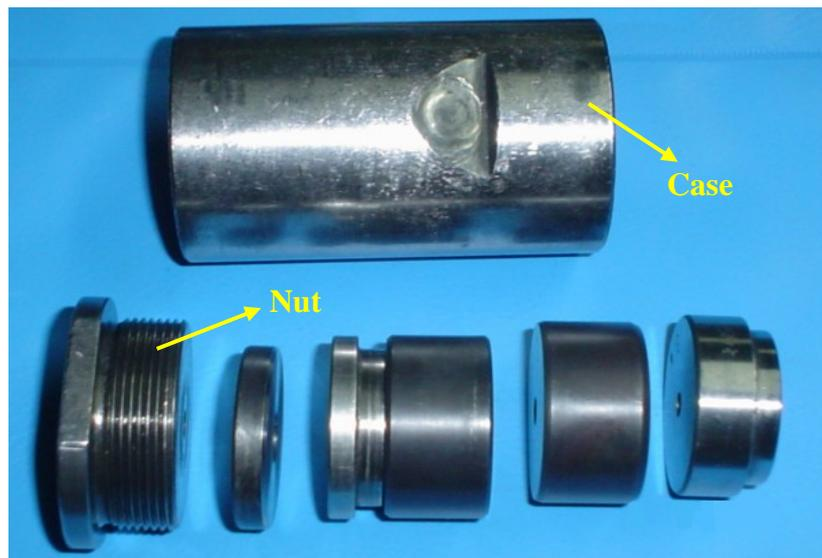
**Figure 4.43.** Axial prestressed extrusion die set
