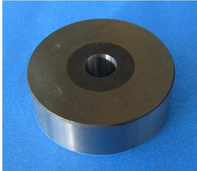
**Figure 3.15.** Assembled bolt forming die
