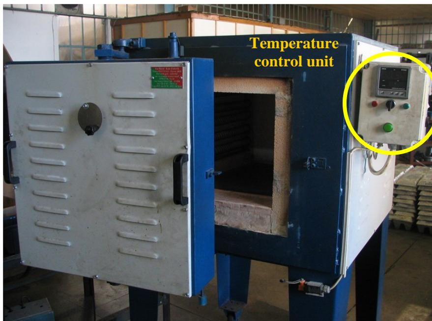
**Figure 3.14.** Temperature controlled furnace
