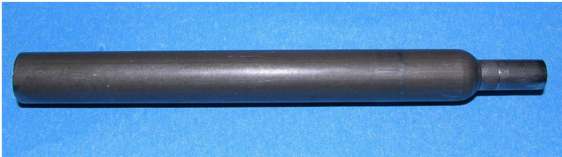
**Figure 5.57.** Extruded part with  $h/d = 8.5$  and  $\varphi = 1.05$
