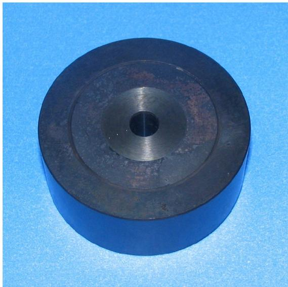
**Figure 4.38.** Tool after assembly of insert and two rings
