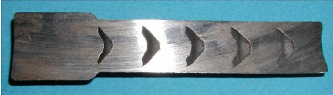
**Figure 1.6.** Central burst in extrusion (Chevron crack) [7]
