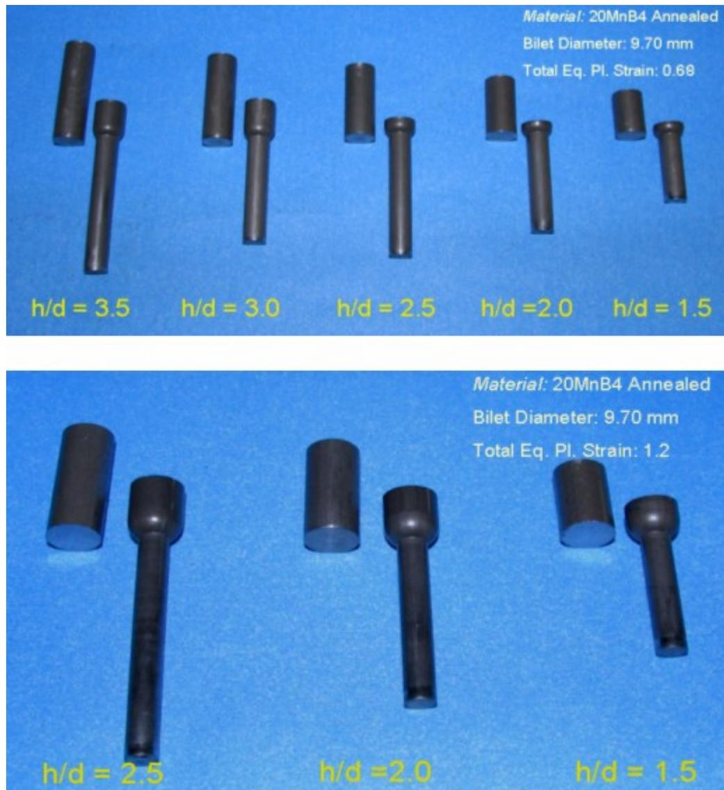
**Figure 5.17.** Extrusion test specimens
