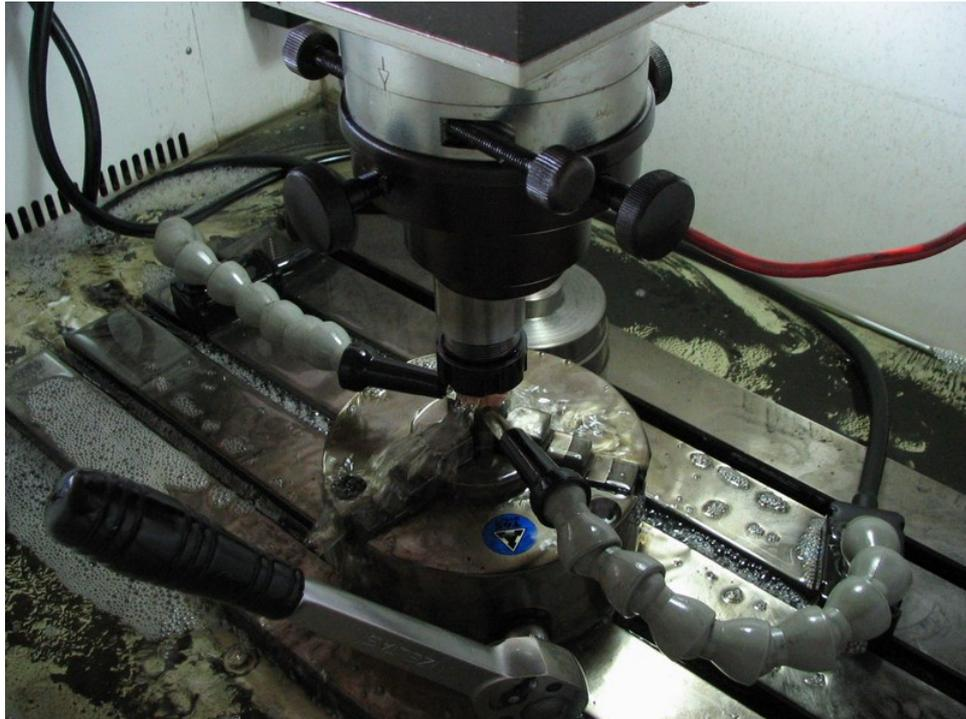
**Figure 3.6.** EDM of forming die
