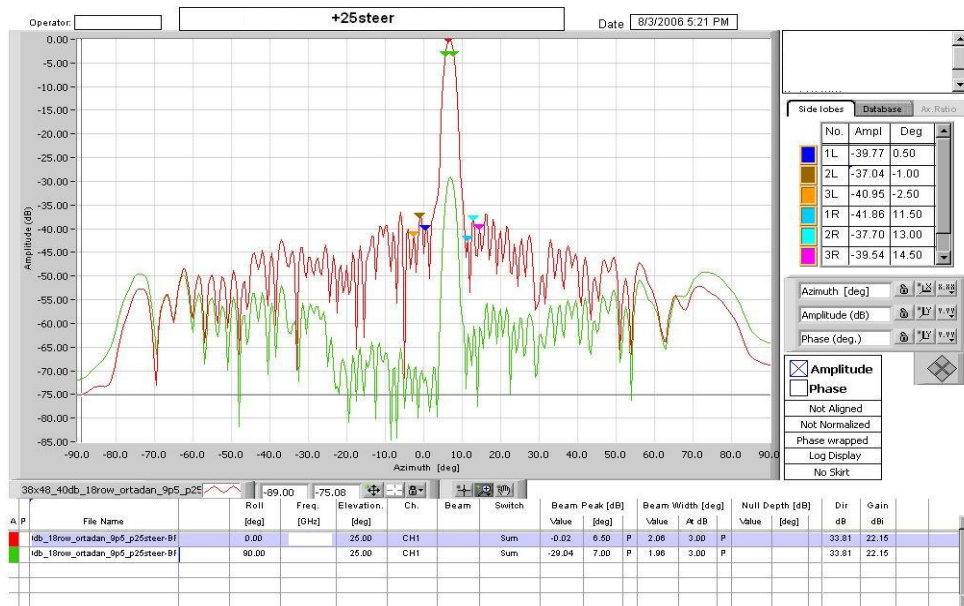
Figure 6.12 Measured azimuth ( \theta = 90^\circ ) co and cross - polarized patterns of the planar SR-SWGA antenna with baffles at +25 degrees beam steering.
