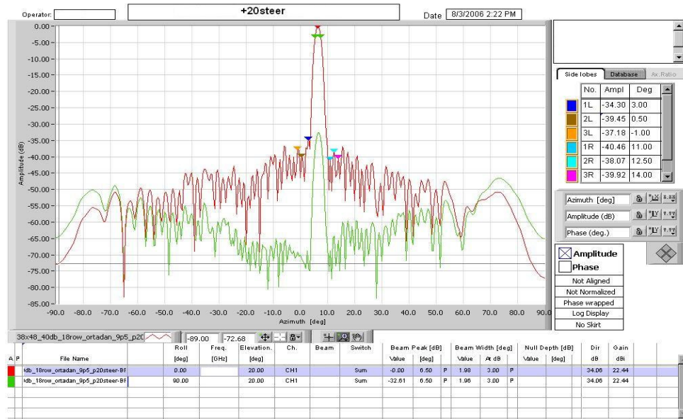
Figure 6.11 Measured azimuth ( \theta = 90^\circ ) co and cross - polarized patterns of the planar SR-SWGA antenna with baffles at +20 degrees beam steering.
