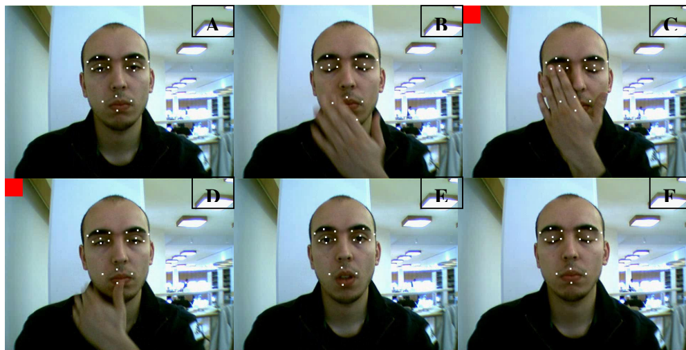
Figure 5-3 Sample Sequence of Partial Occlusion (Frames with a detected face geometry rule violation contain a red rectangle in upper left corner)
