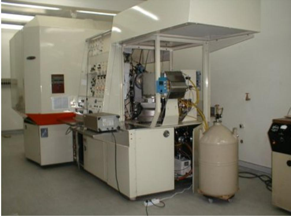
Fig.3.5. Ion implantation system in METU Physics department
