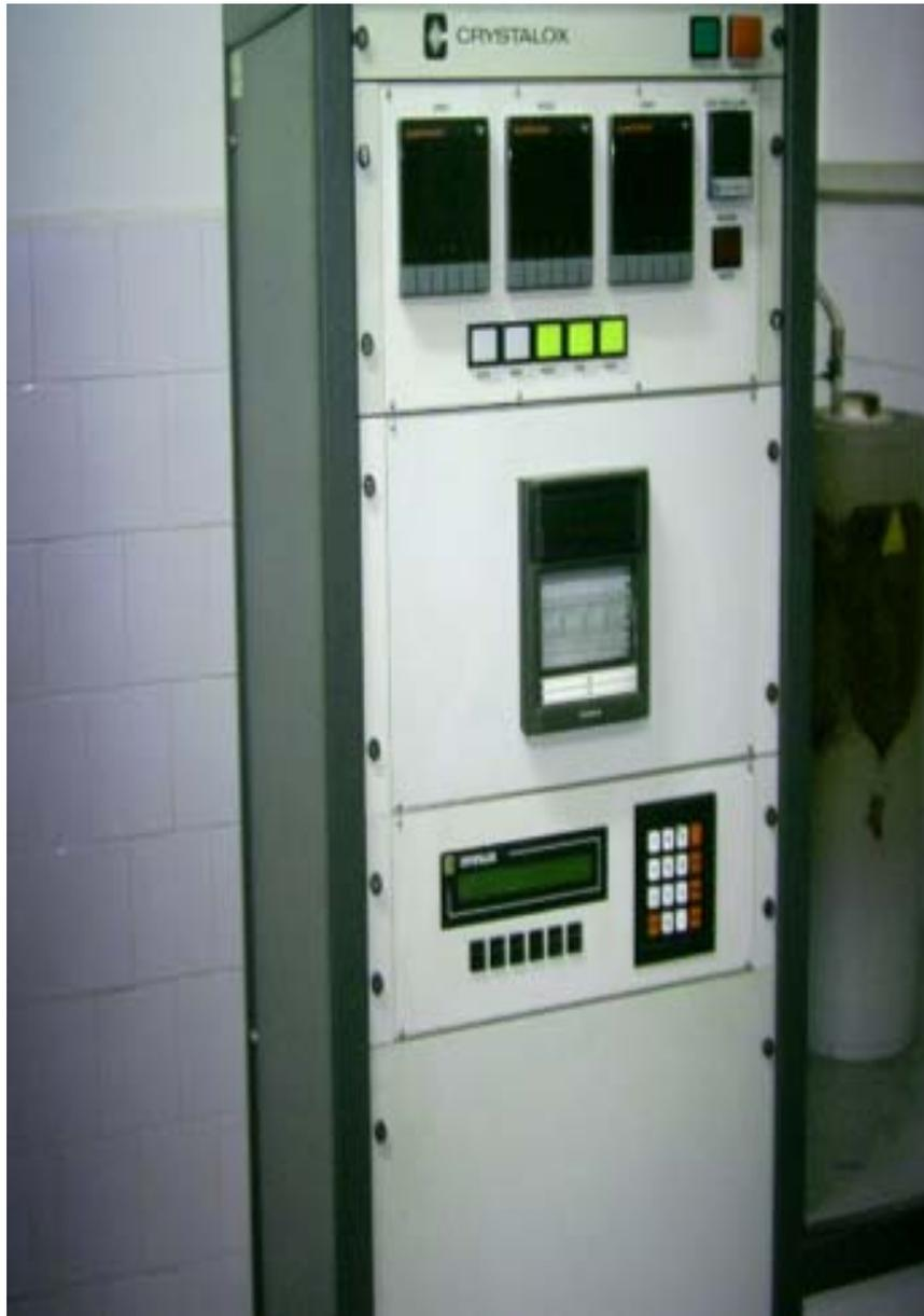
Fig.3.2. Bridgman Stockbarger System in the Crystal Growth Laboratory of Physics Department at METU
