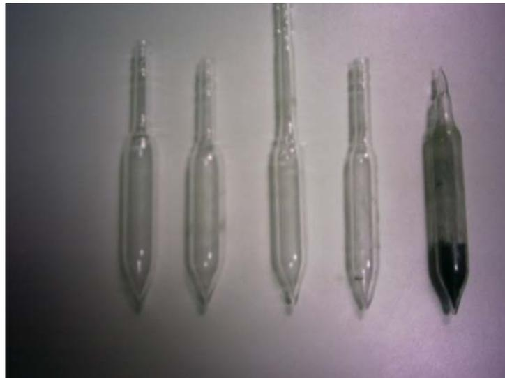
Fig.3.1. Some pointed bottom crucible with different diameters
