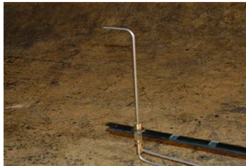
Figure 3.4 Pitot Tube Used in Experimental Measurements.
