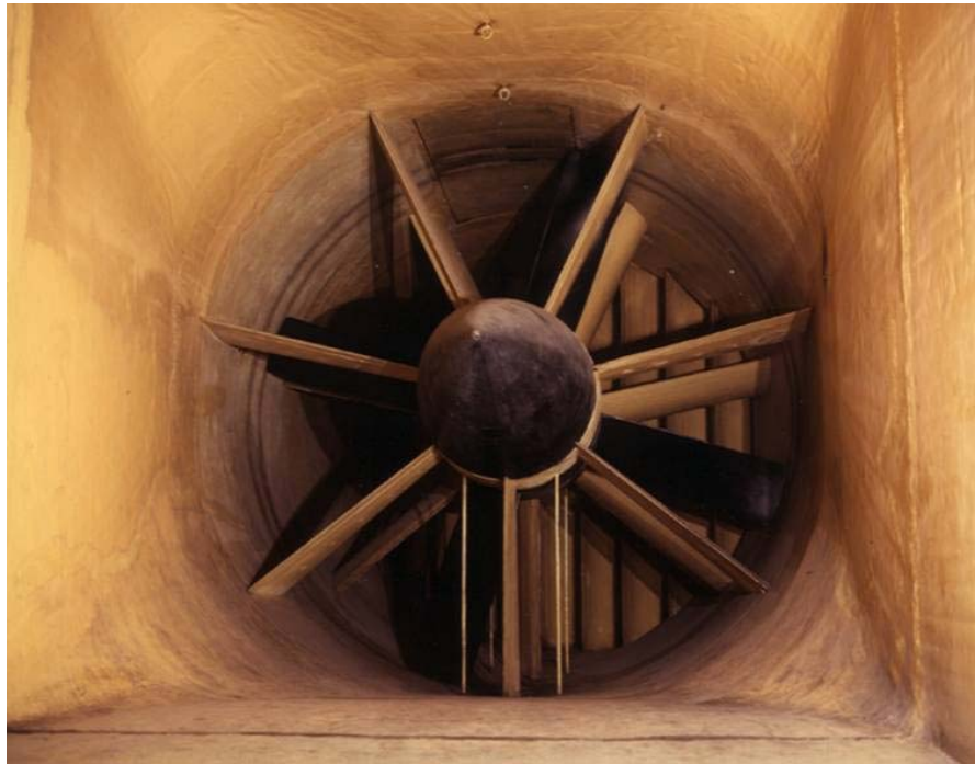
Figure 1.7 Ankara Wind Tunnel Fan (Looking From Downstream).
