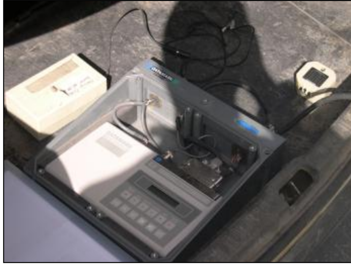
Figure 4.23. General view of the DATAMARK LS-8000 WD with 24 bit resolution A/D type data recorder and its associated equipment used for microtremor measurements in the field investigation.
