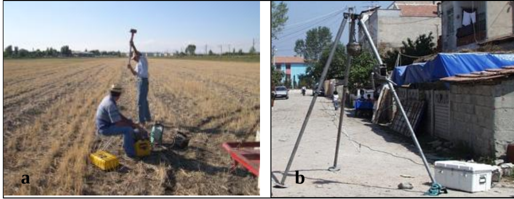
Figure 4.7. Field applications of the seismic energy sources, such as sledge hammer and striker plates (a) and weight-drop (b).
