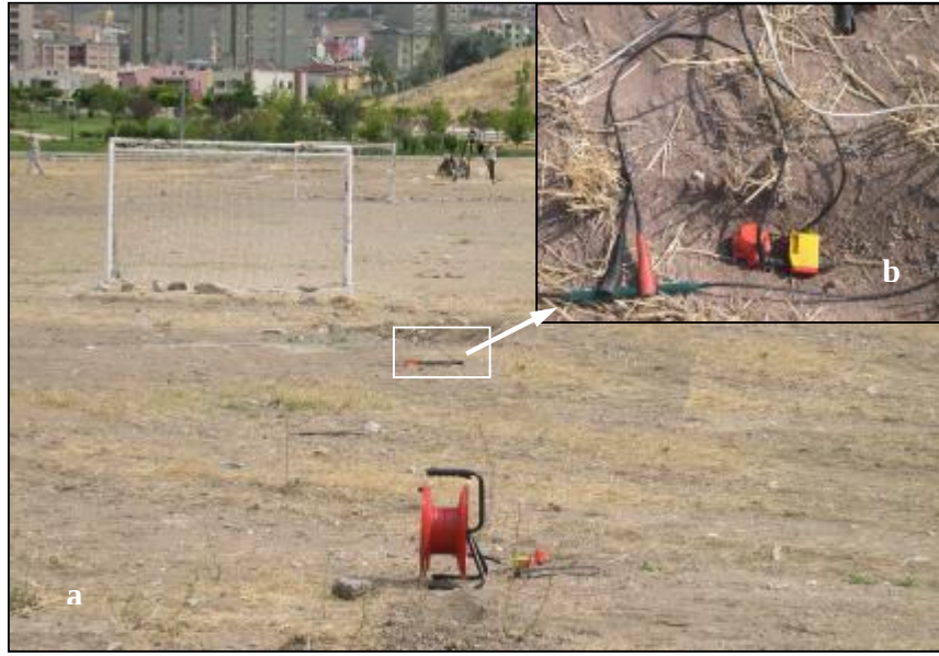
Figure 4.8. General view of the some of the equipments, particularly geophones, geophone cables and geophone extension cables that are necessary to perform refraction survey in the field, (a). Figure 4.8b shows a close up view of the P (20 Hz) and S wave (14 Hz) geophones.
