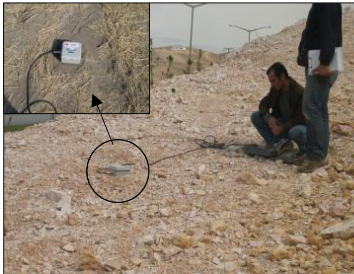
Figure 4.22. General view of microtremor measurements and a close-up view of the Akashi JEP-6A3 three component built-in acceleration seismometer (small figure) during the field investigation.
