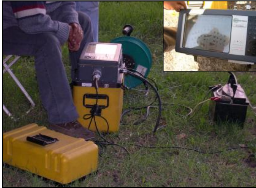
Figure 4.9. A general and close up view of the 12-channel signal-enhancement seismograph (GEOMETRICS, SmartSeis-26325-01) and its' associated equipment (i.e., power supply, integrated extension cables for connecting the geophones and seismic energy source).
